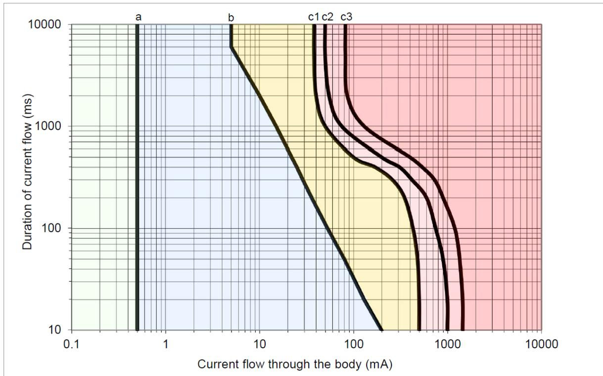
**Figure 2: Time/Current zones of effects of alternating currents (15Hz to 100Hz) for a current path left hand to feet**
