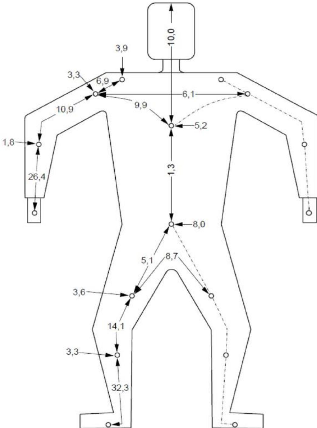
Figure 1: Internal Partial Impedances of the Human Body (from Figure 1 IEC TS 60479-1 Ed4.0)
