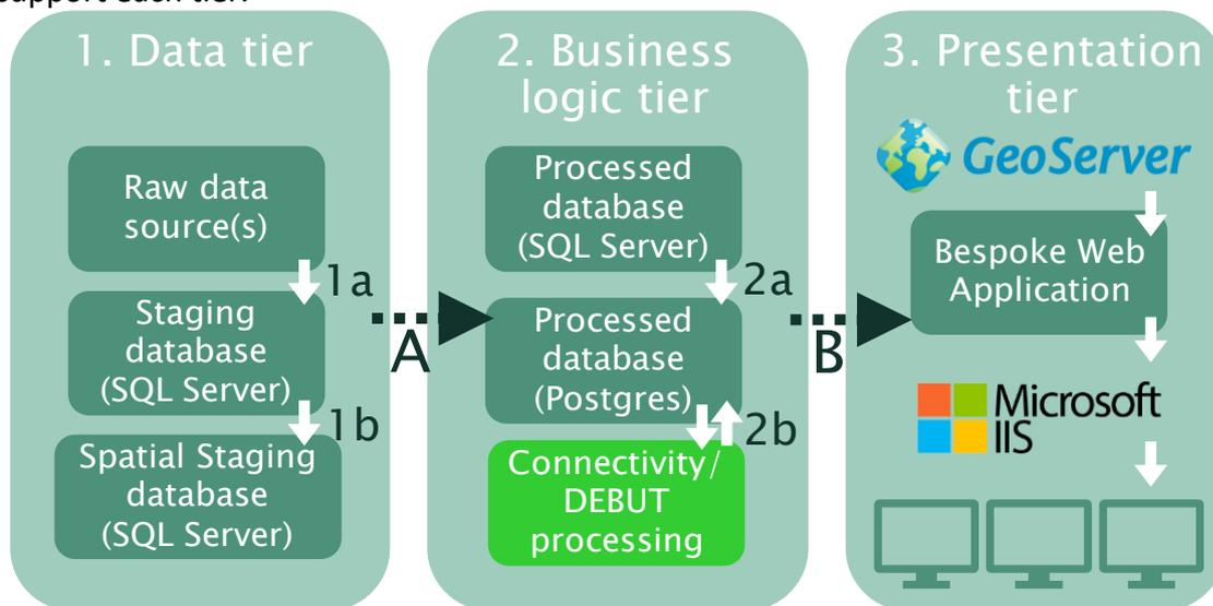
Figure 7. three distinct elements of software architecture
