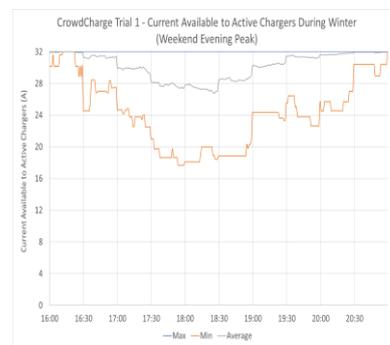
**Figure 4. Current allocated to chargers in demand management**
