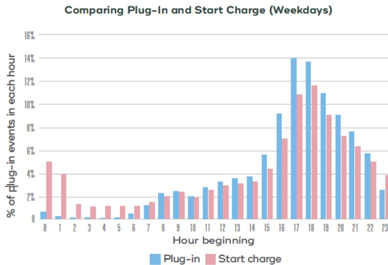
**Figure 9. Plug in times vs charge start times**
