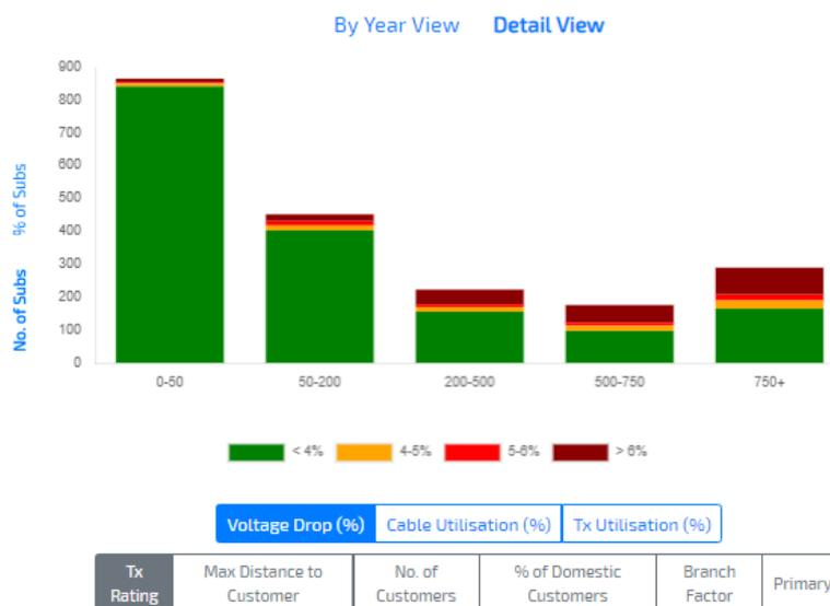
**Figure 19. Detailed results breakdown graph**
