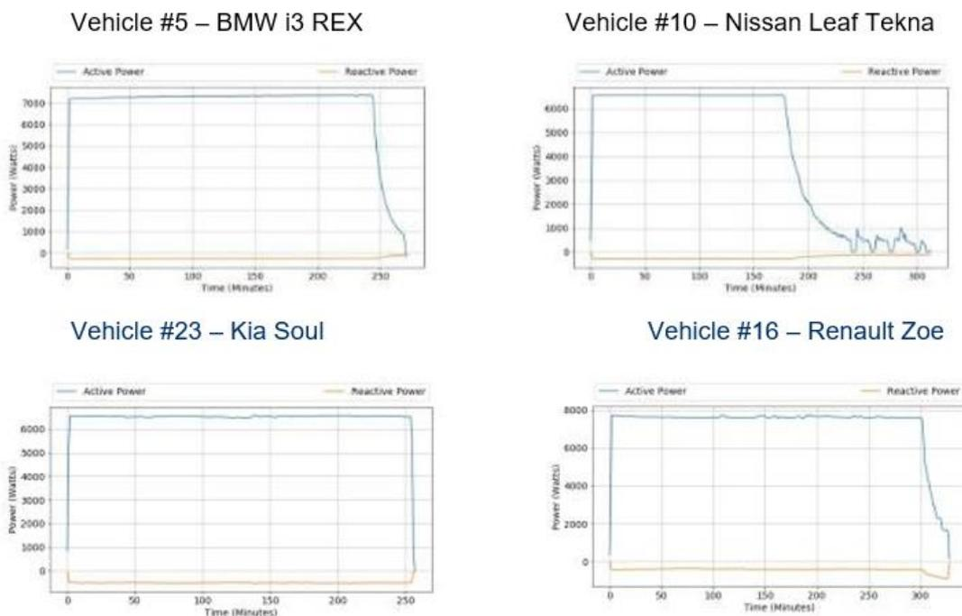
**Figure 1. Showing four of the charging profiles observed**
