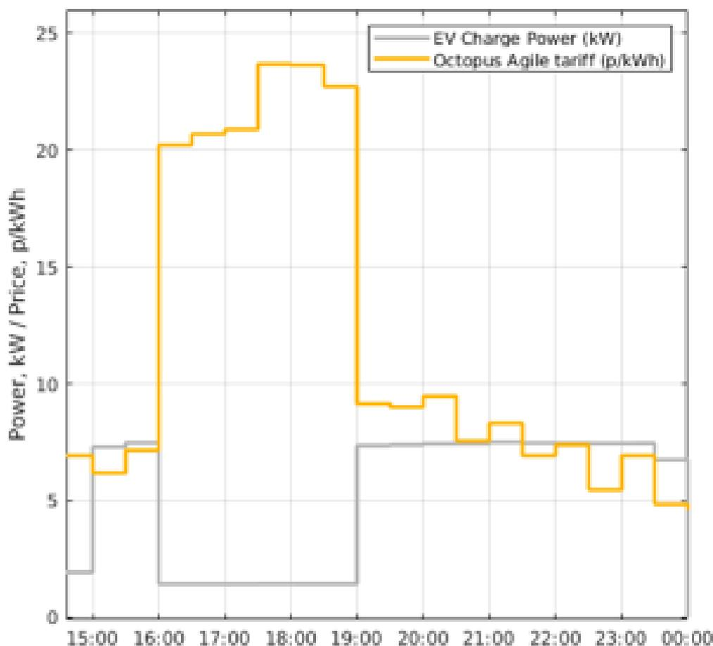
Figure 2-9 - Constraining EV charging on Octopus Agile tariff (Home 4)
