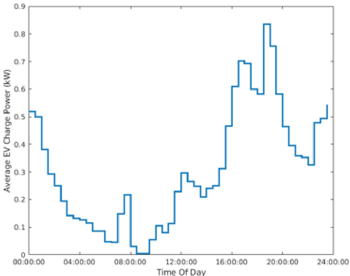
Figure 2-5 - Average EV charge power across the day for the MADE homes (Homes 2,3,4 & 5, 01/12/2019 - 15/01/2020. Note that Home 1 was not included in this analysis since the charge point was installed at a later date.)
