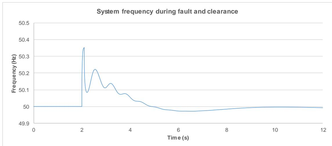
**Figure 2-6 Frequency during fault and clearance - Min load**
