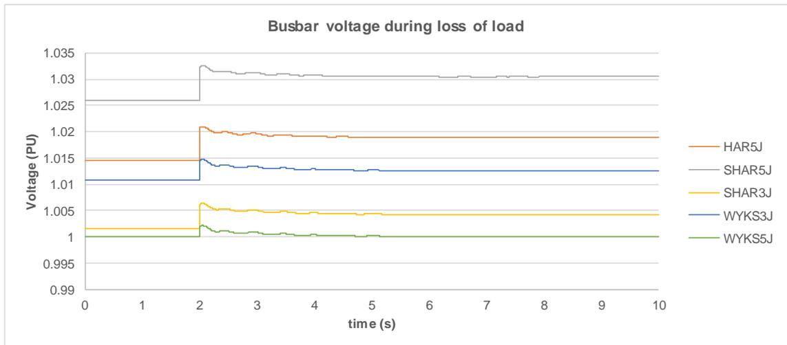
**Figure 2-13 Busbar voltage following loss of Sharnbrook 11kV feeder**
