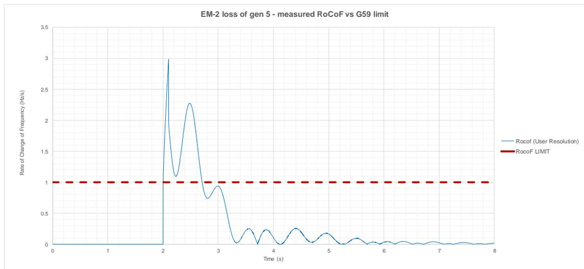
**Figure 2-28 Rate of change of system frequency following loss of Generator 5**
