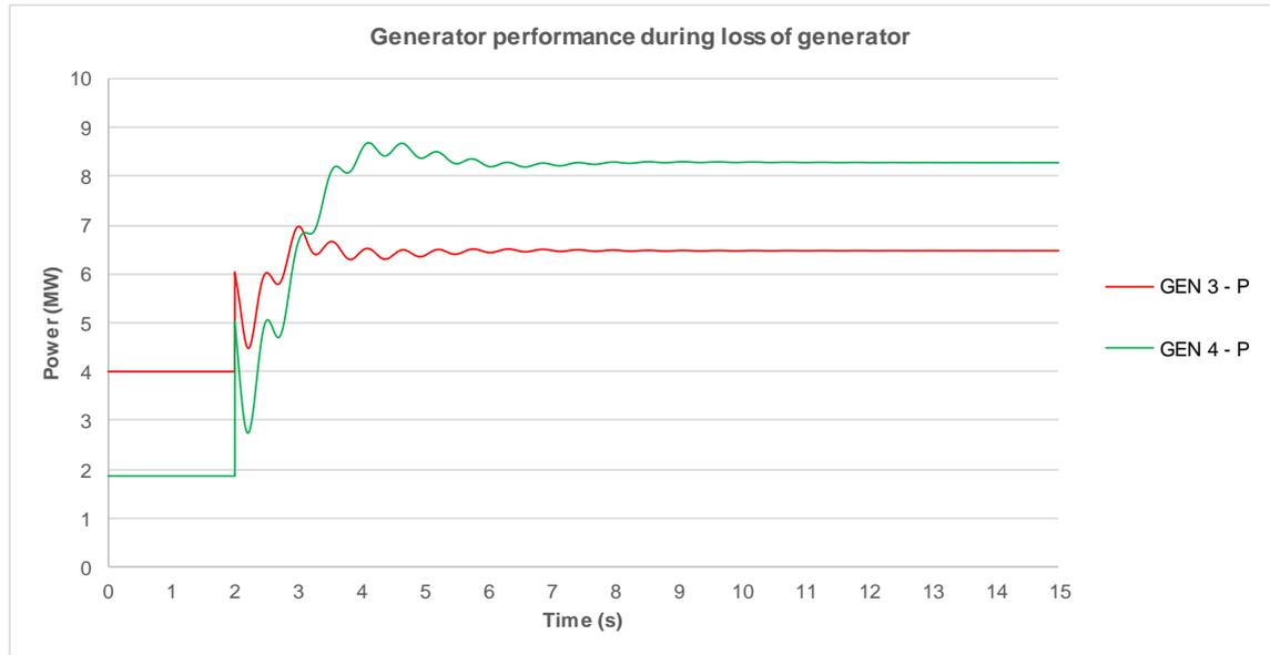
**Figure 2-27 Active power response following loss of Generator 5**
