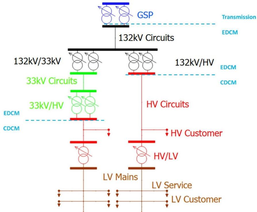
**Figure 4.6 Single line diagram showing charging methodology boundaries [36]**
