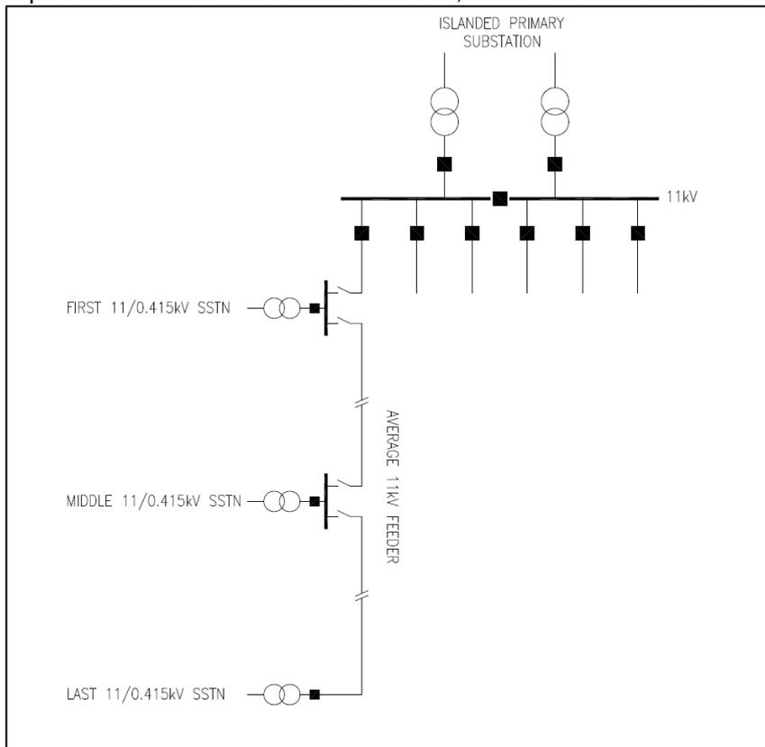
**Figure 1-3 Distribution substations on 11kV feeder**
