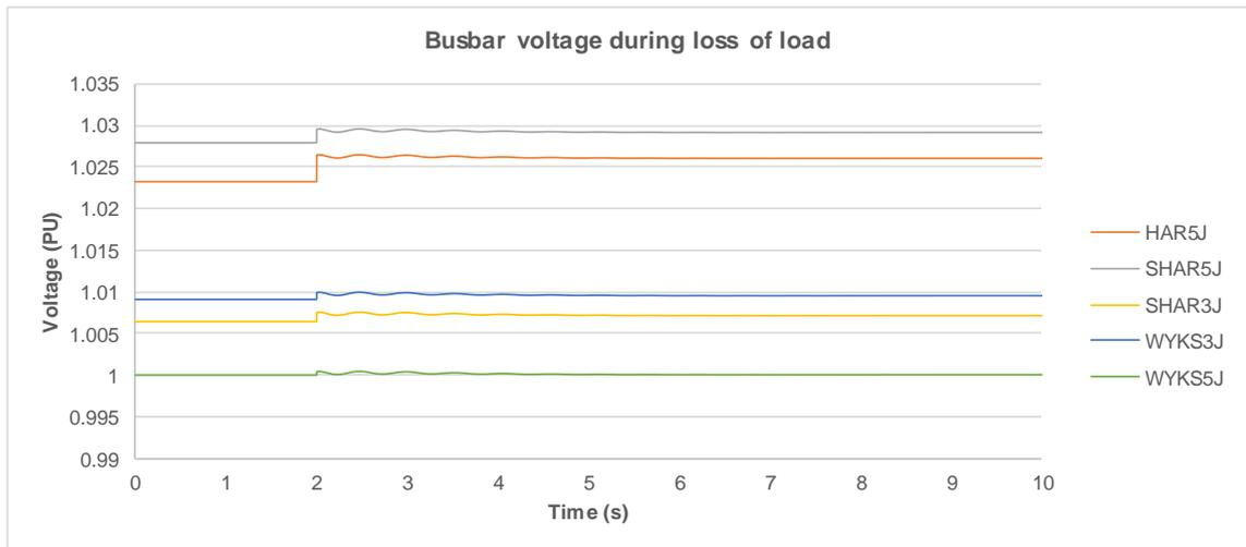
**Figure 2-11 Busbar voltage following loss of Harrold 11kV feeder**
