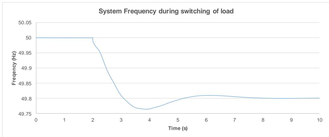
**Figure 2-32 Frequency following connection of Little Irchester 11kV feeder**
