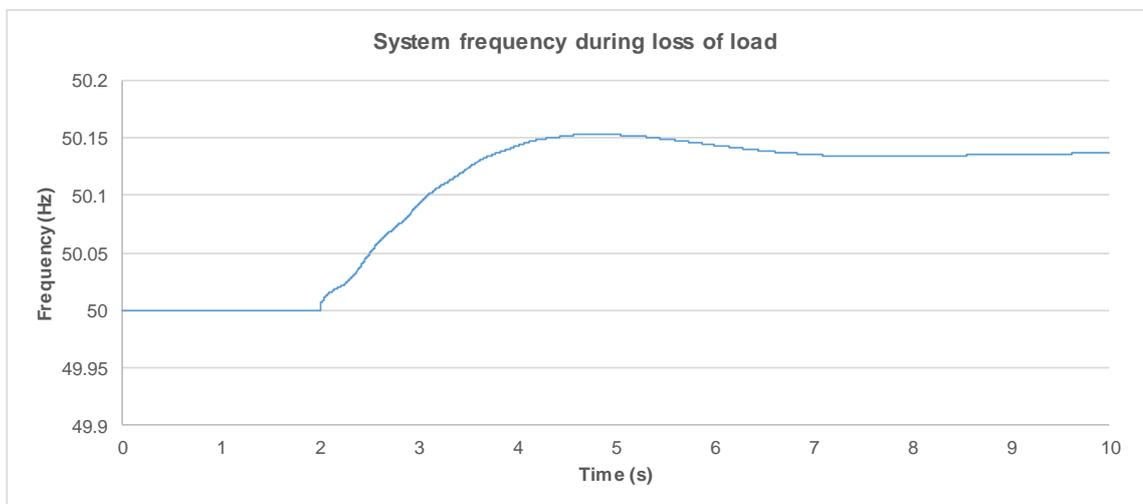
**Figure 2-14 Frequency following loss of Sharnbrook 11kV feeder**
