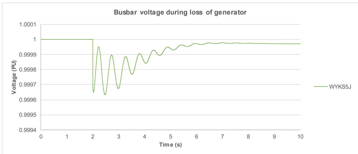
**Figure 3.3 Voltage response after loss of a generator on EM1**
