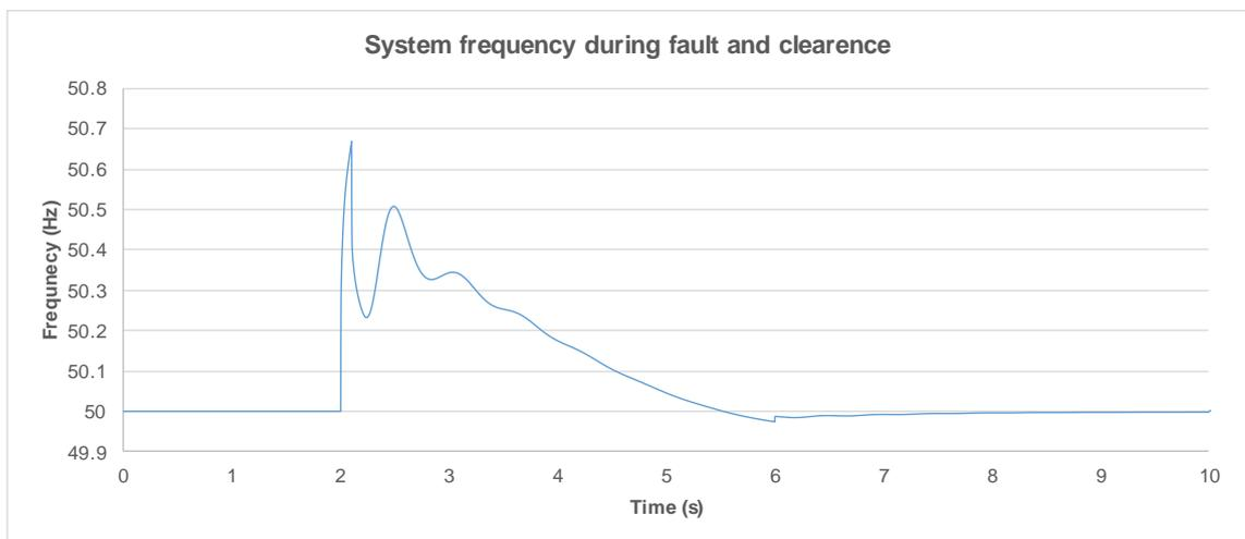
**Figure 2-22 Frequency during fault and clearance – Max load**
