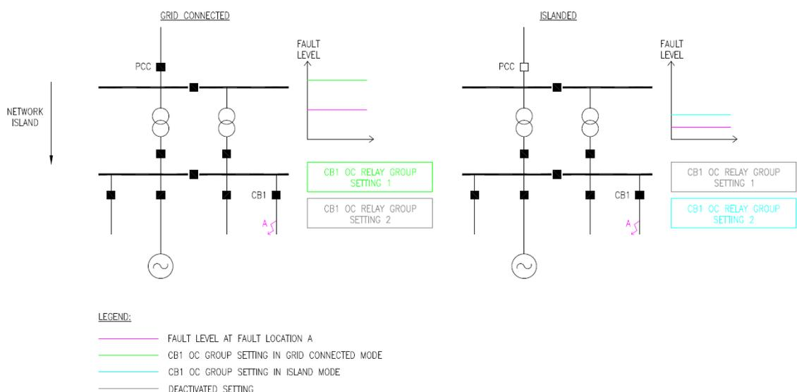
**Figure 2.1 Overcurrent group settings in grid-connected and island modes**
