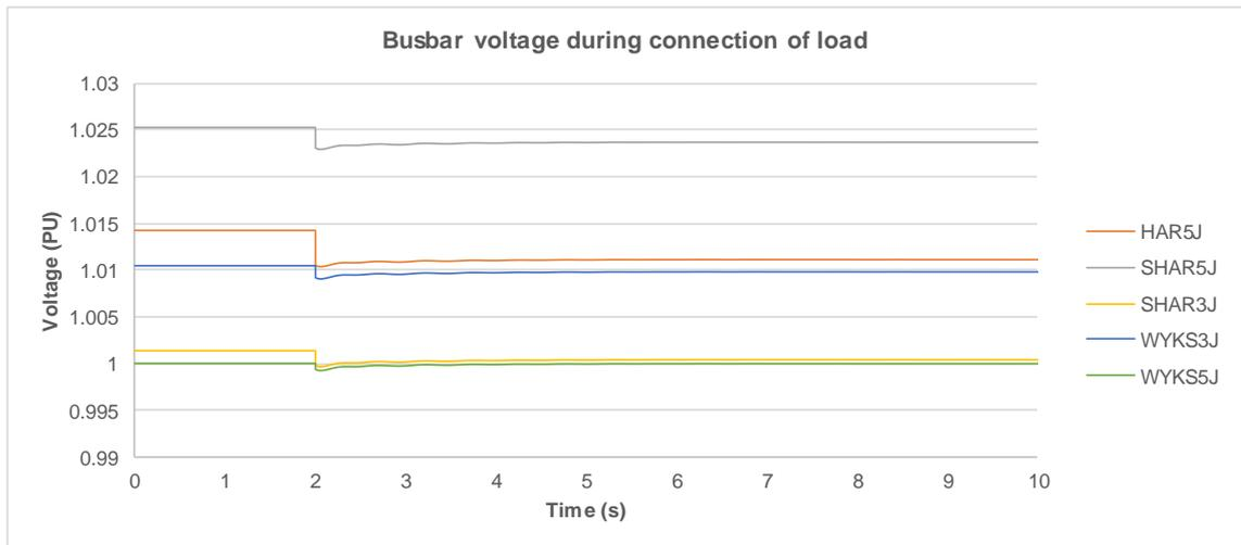
**Figure 2-15 Busbar voltage following connection of Harrold 11kV feeder**
