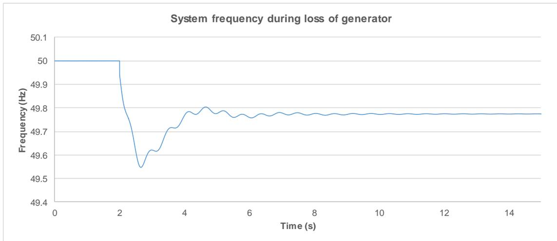
**Figure 2-8 Frequency following loss of generator 5**
