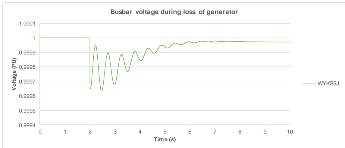
**Figure 2-7 Busbar voltage following loss of Generator 5**
