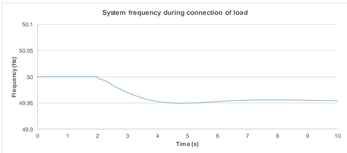
**Figure 2-16 Frequency following connection of Harrold 11kV feeder**
