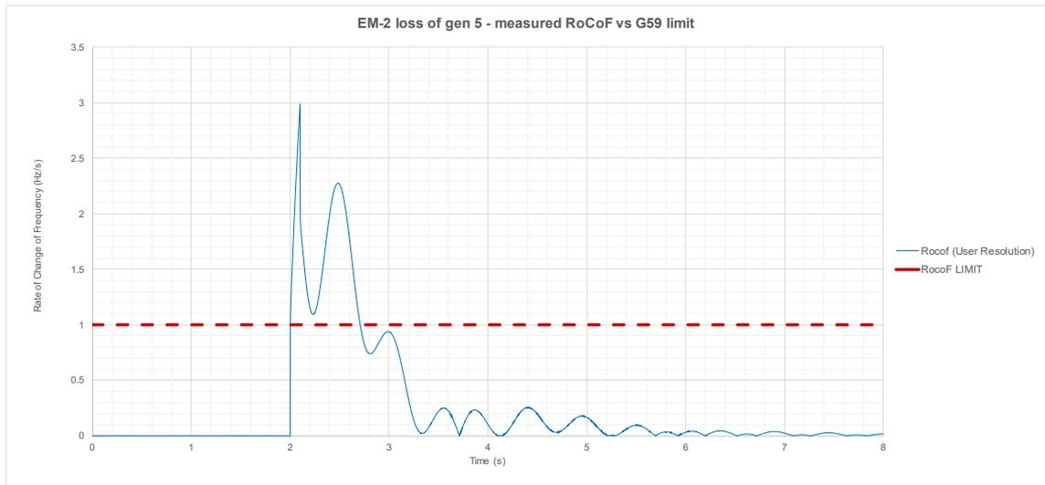
**Figure 3.4 Rate of Change of Frequency (RoCoF) simulation for EM2**
