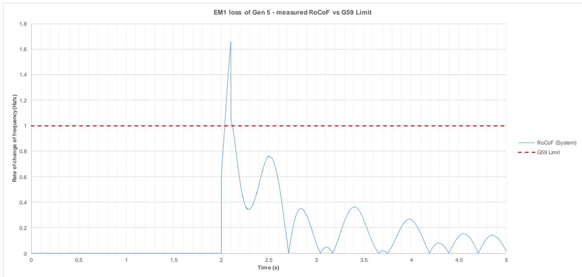
**Figure 2-10 Rate of change of system frequency following loss of Generator 5**
