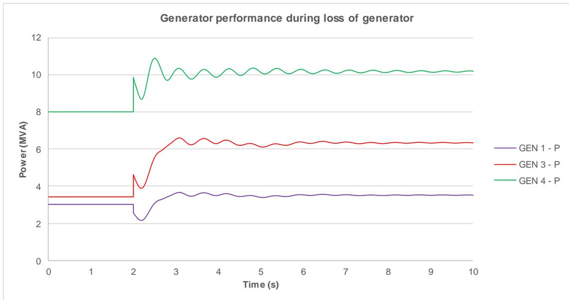
**Figure 2-9 Active power response following loss of Generator 5**
