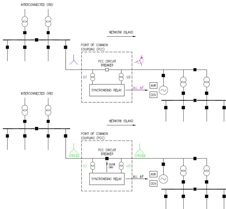
**Figure 2.3 Seamless reconnection of island to the main interconnected grid**
