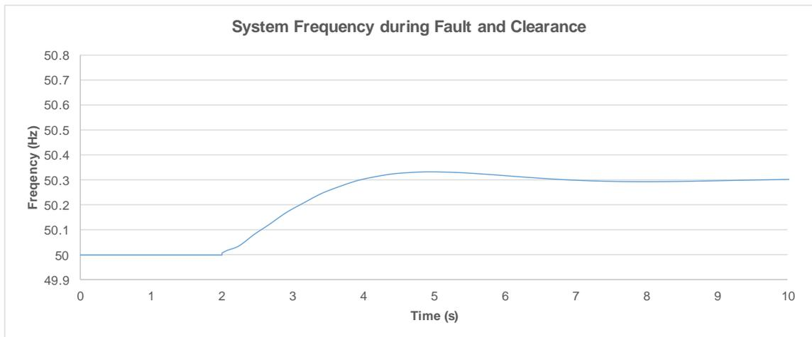
**Figure 2-30 Frequency following loss of Little Irchester 11kV feeder**
