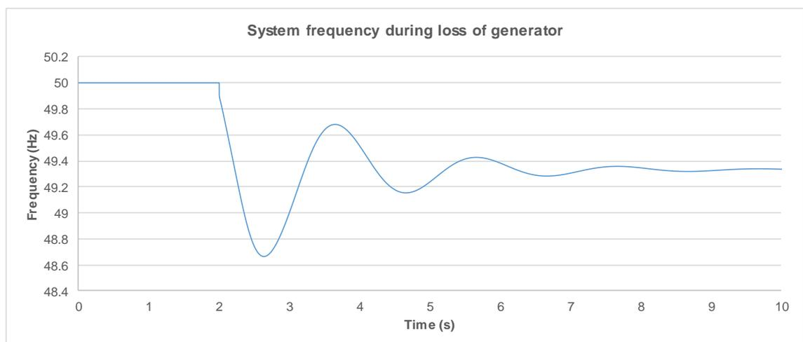
**Figure 2-26 Frequency following loss of Generator 5**
