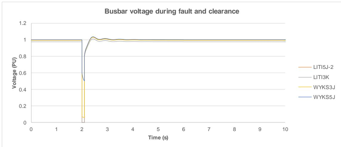
**Figure 2-21 Busbar voltage during fault and clearance – Max load**
