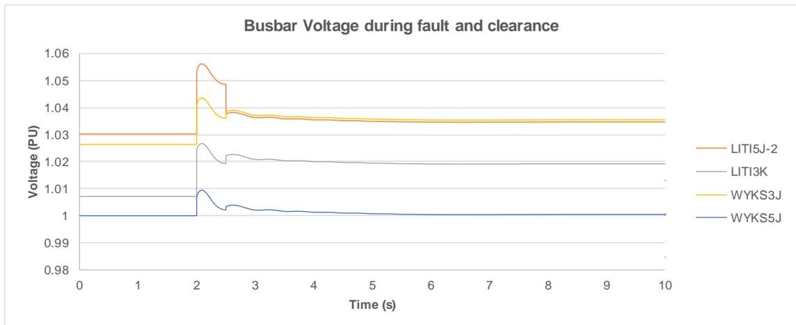
**Figure 2-29 Busbar voltage following loss of Little Irchester 11kV feeder**
