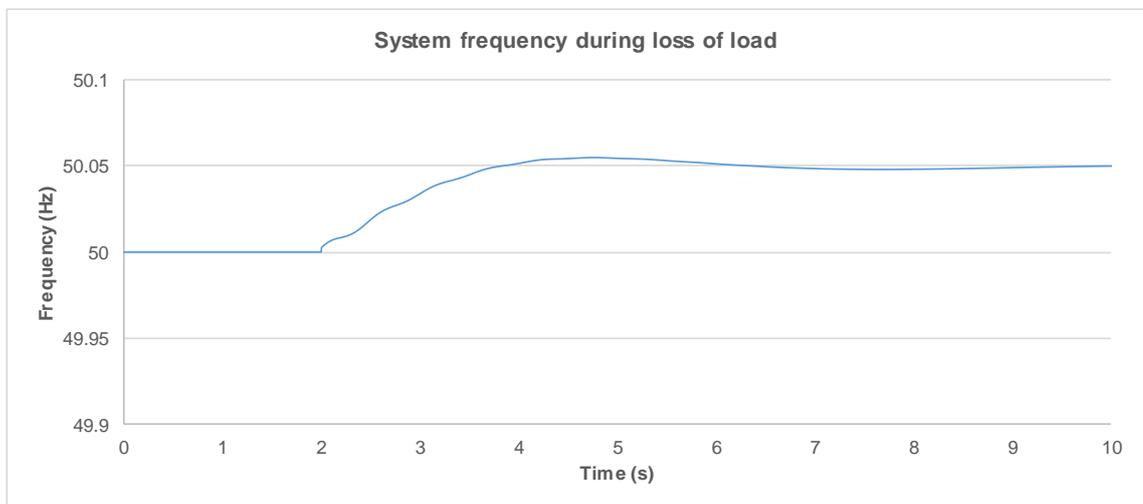
**Figure 2-12 Frequency following loss of Harrold 11kV feeder**
