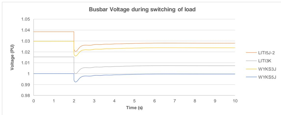
**Figure 2-31 Busbar voltage following connection of Little Irchester 11kV feeder**
