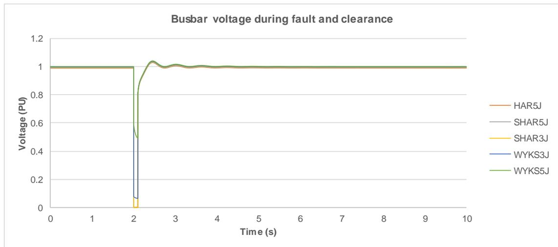
**Figure 2-5 Busbar voltage during fault and clearance - Min load**
