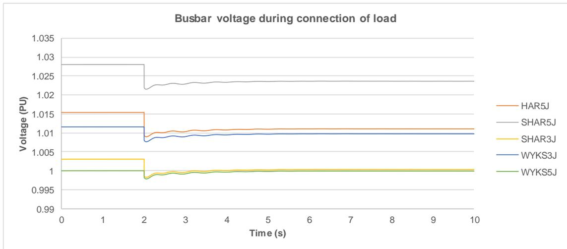
**Figure 2-17 Busbar voltage following connection of Sharnbrook 11kV feeder**
