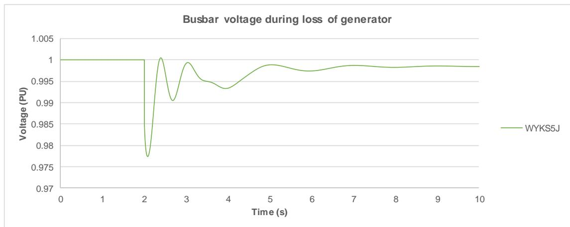
**Figure 2-25 Busbar voltage following loss of Generator 5**
