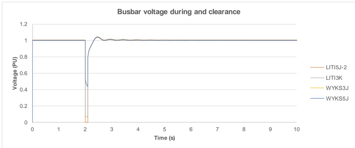
**Figure 2-23 Busbar voltage during fault and clearance – Min load**
