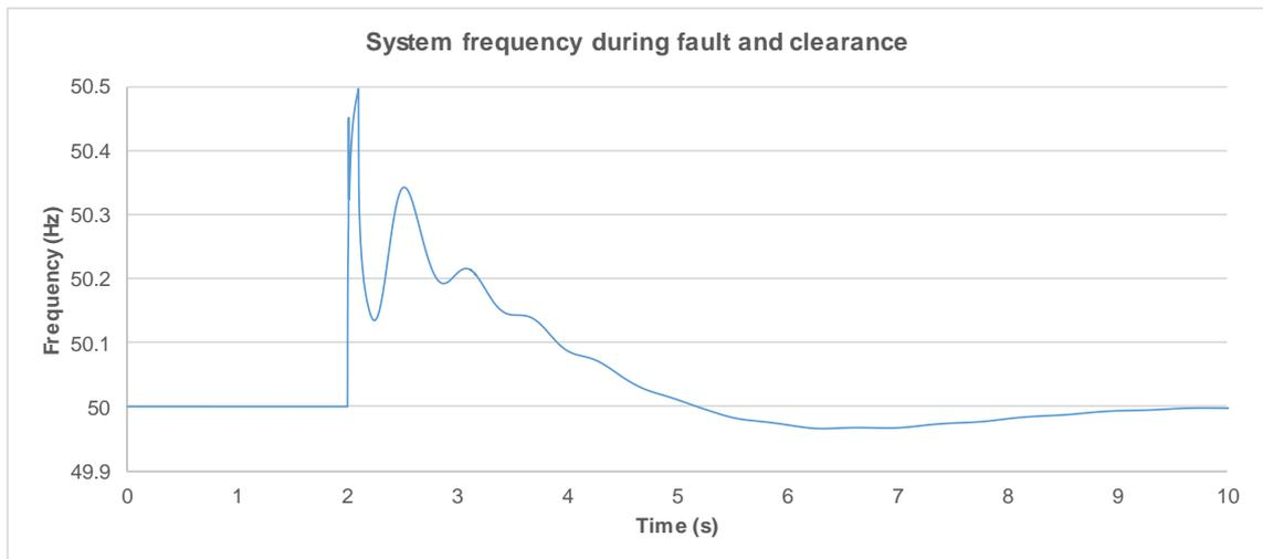
**Figure 2-4 Frequency during fault and clearance - Max load**
