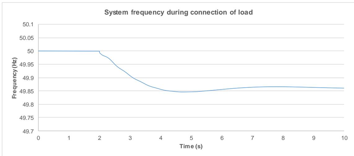
**Figure 2-18 Frequency following connection of Sharnbrook 11kV feeder**
