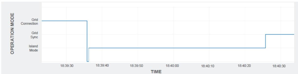
**Figure 36: Simulation of loss of grid at Taunton**
