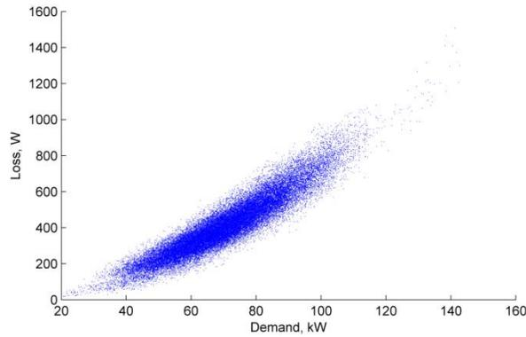
Figure 89 Aug 2018 2017 Loss, kW vs demand, 10 min. av. (Peel A I&C LV feeder)
