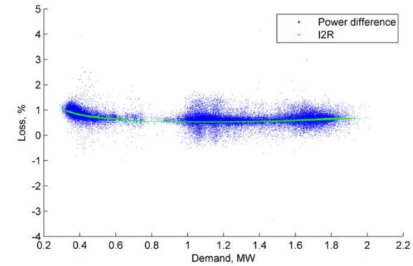
Figure 50 Aug 2018 Loss, % vs demand (Amway Tongwell HV feeder)
