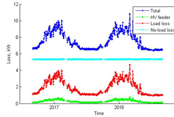
Figure 36 Long term mean daily ( $I^2R$ ) loss (Wavendon Gate Local HV feeder)
