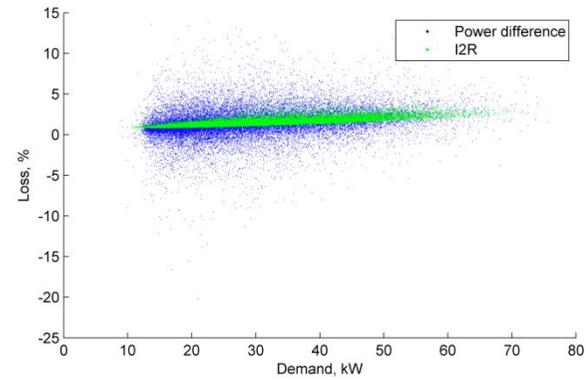
Figure 86 Aug 2018 Loss, % vs demand, 1 min. av. (Tromode Dom. LV feeder)
