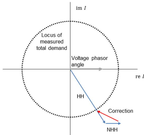
Figure 118 Corrections applied to non-half-hourly demand where the amplitude of the primary substation current due to half-hourly demand is greater than the measured current at the primary.
