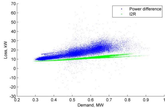
Figure 69 Aug 2018 Loss, kW vs demand (Wolverton HV feeder)
