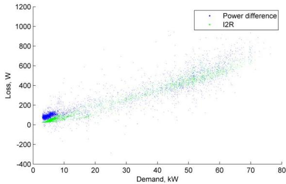
Figure 101 Aug 2018 Loss, kW vs demand, 10 min. av. (Braddan I&C LV feeder)
