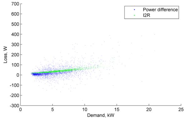
Figure 105 Aug 2018 Loss, kW vs demand, 10 min. av. (Santon OH LV feeder)
