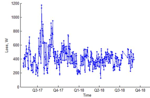
Figure 88 Long term mean daily ( $I^2R$ ) loss (Peel A I&C LV feeder)
