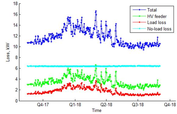
Figure 68 Long term mean daily (I<sup>2</sup>R) loss (Wolverton HV feeder)
