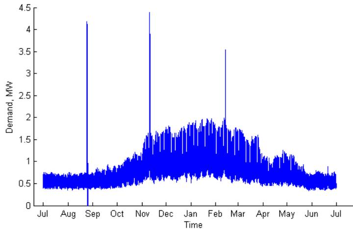
HV feeder demand. Spikes illustrate temporary changes in feeder configuration.
