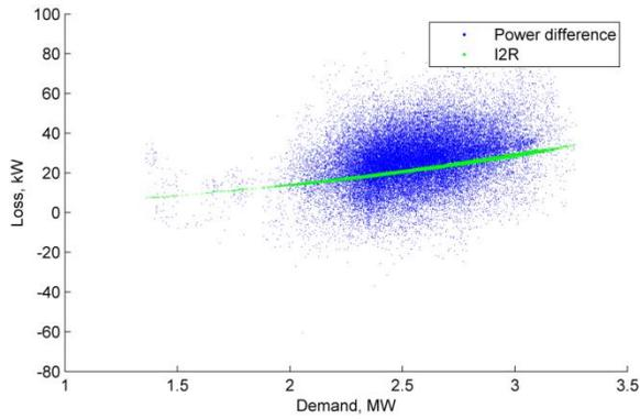
Figure 45 Aug 2018 Loss, kW vs demand (Crawley Road Tee Howard Way HV feeder)
