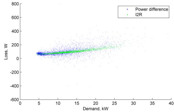
Figure 81 Aug 2018 Loss, kW vs demand, 10 min. av. (Ramsey Dom. LV feeder)
