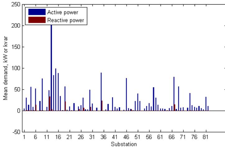
Mean distribution substation loads for substations supplied by the HV feeder. In this case emphasising the high number of connected transformers.
