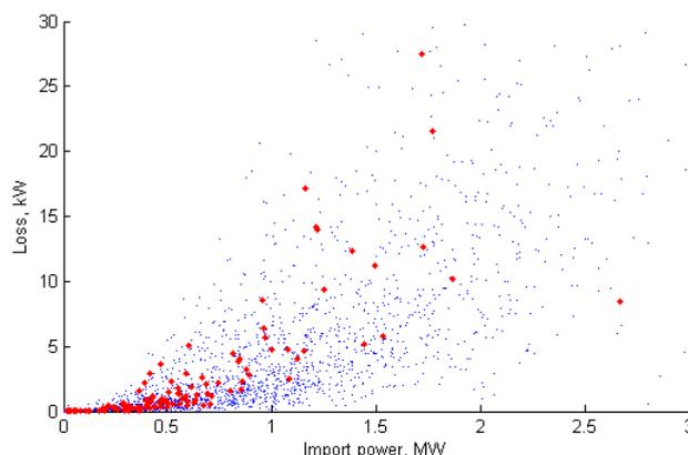
Figure 12 Line loss vs. network import power coloured for voltage (blue: 11 kV, red 6.6 kV).
