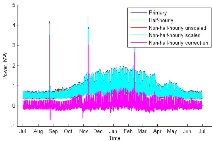
Scaled and unscaled modelled substation load.
