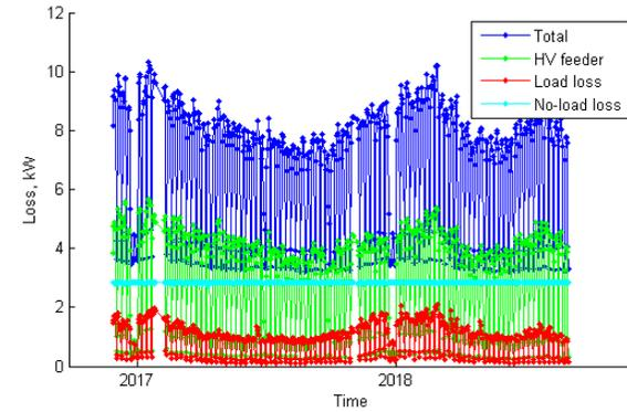
Figure 48 Long term mean daily ( $I^2R$ ) loss (Amway Tongwell HV feeder)
