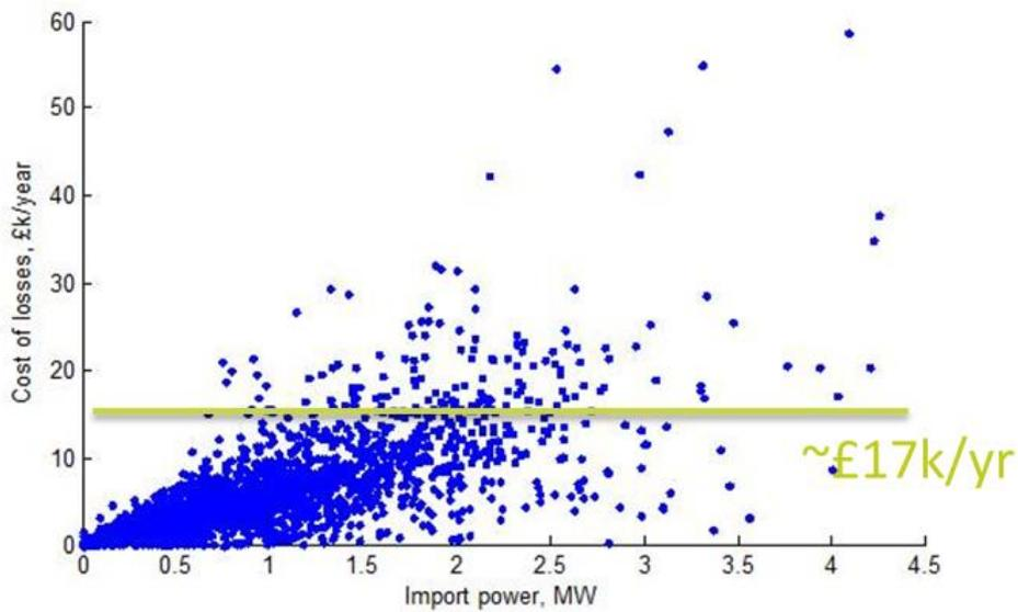
Figure 20 Cost of feeder losses scatter plot showing £17k/yr. threshold.
