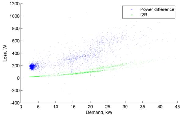
Figure 97 Aug 2018 Loss, kW vs demand, 10 min. av. (Ballasalla I&C LV feeder)
