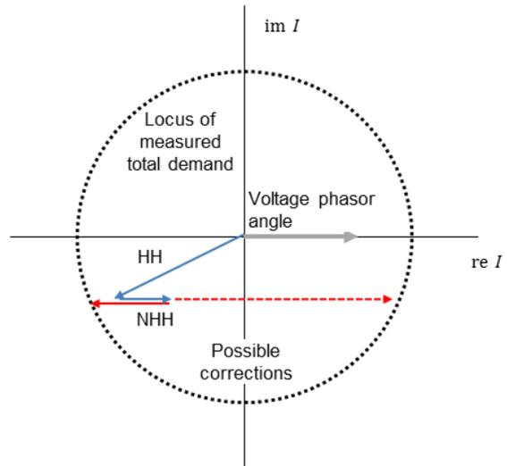
Figure 117 Corrections applied to non-half-hourly demand where the amplitude of the primary substation current due to half-hourly demand is less than the measured current at the primary, with half-hourly demand as generation.
