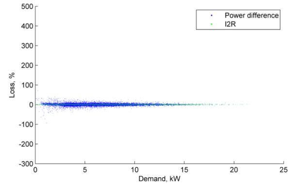
**Figure 74 Aug 2018 2017 Loss, % vs demand, 1 min. av. (Dom. Pilot LV feeder)**
