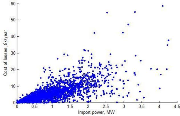
**Figure 6 Cost of feeder losses vs. feeder load.**
