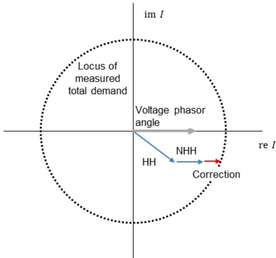
Figure 116 Corrections applied to non-half-hourly demand where the amplitude of the primary substation current due to half-hourly demand is less than the measured current at the primary, and with half-hourly, with non-half-hourly demand as loads.
