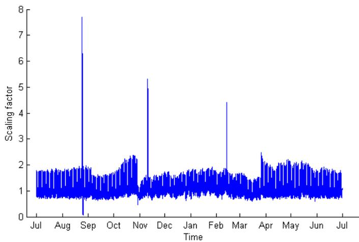
NHH demand scaling factor to match profile load estimate to SCADA current data.
