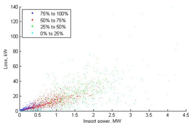
Figure 8 Loss vs. network import power coloured for proportion of losses due to transformer no-load losses.
