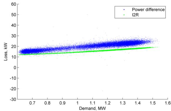
Figure 61 Aug 2018 Loss, kW vs demand (Riverside Park HV feeder)
