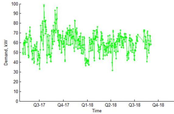
Figure 87 Long term mean daily feeder demand (Peel A I&C LV feeder)
