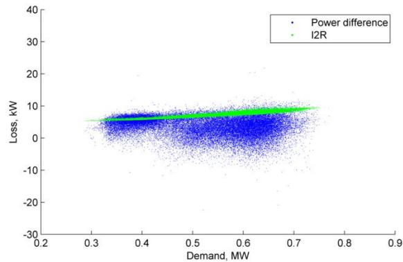
Figure 53 Aug 2018 Loss, kW vs demand (Ackerman Tongwell Aldrich Drive Tee HV feeder)
