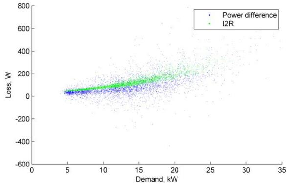
Figure 113 Mar & Apr 2018 Loss, kW vs demand, 10 min. av. (Ramsey OH LV feeder)
