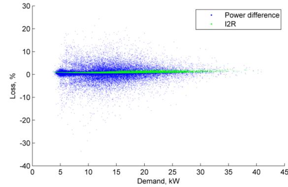
Figure 114 Mar & Apr 2018 Loss, % vs demand, 1 min. av. (Ramsey OH LV feeder)
