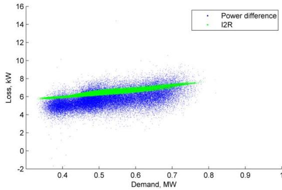
Figure 37 Aug 2018 Loss, kW vs demand (Wavendon Gate Local HV feeder)
