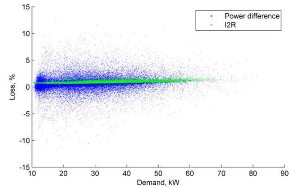
Figure 78 Aug 2018 Loss, % vs demand, 1 min. av. (Laxey Dom. LV feeder)
