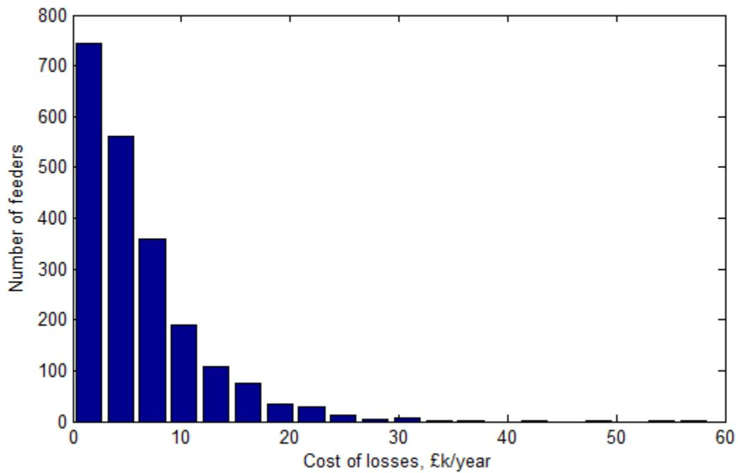
Figure 120 Cost of losses for feeders with accepted results, based on £48/MWh
