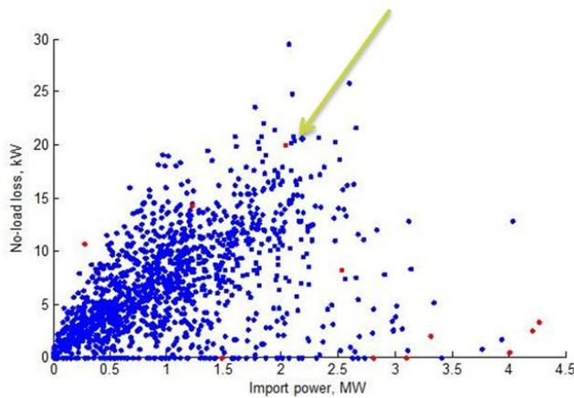
Scatter plot of HV feeder transformer no-load losses, showing that this feeder has one of the highest levels of aggregate transformer no-load loss
