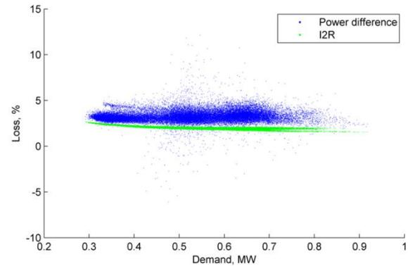
Figure 70 Aug 2018 Loss, % vs demand (Wolverton HV feeder)
