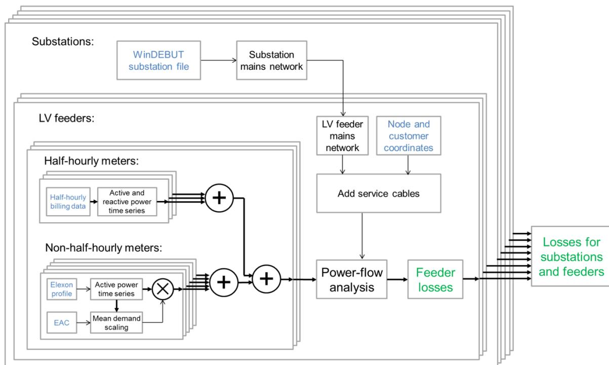
Figure 21 Outline of the LV feeder loss estimation method.
