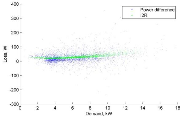
**Figure 73 Aug 2018 Loss, kW vs demand, 10 min. av. (Dom. Pilot LV feeder)**
