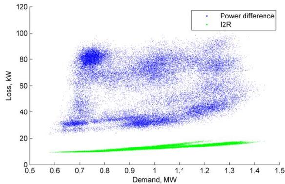
Figure 57 Aug 2018 Loss, kW vs demand (The Avenue HV feeder)
