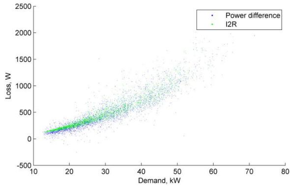
Figure 85 Aug 2018 Loss, kW vs demand, 10 min. av. (Tromode Dom. LV feeder)
