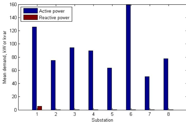
Mean distribution substation loads for substations supplied by the HV feeder.
