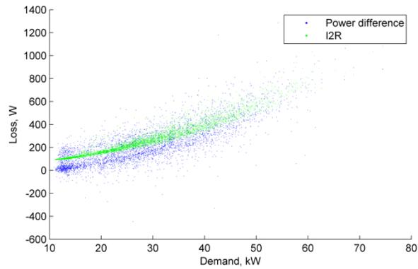
Figure 77 Aug 2018 Loss, kW vs demand, 10 min. av. (Laxey Dom. LV feeder)
