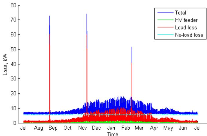
HV feeder Losses, with breakdown of losses between HV line, transformer no-load losses and transformer load losses.
