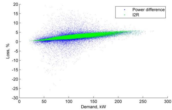
Figure 94 Aug 2018 Loss, % vs demand, 1 min. av. (Peel B I&C LV feeder)
