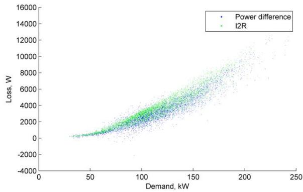
Figure 93 Aug 2018 Loss, kW vs demand, 10 min. av. (Peel B I&C LV feeder)
