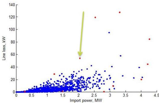
HV feeder Losses, with breakdown of losses between HV line, transformer no-load losses and transformer load losses.
