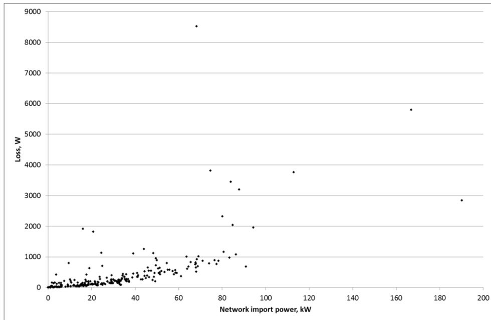
Figure 22 Loss power versus load scatter plot for all 254 processed LV feeders.
