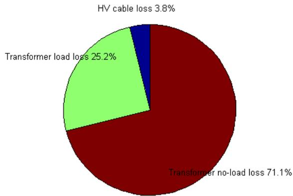
Breakdown of HV feeder mean annual losses between HV line, transformer no-load losses and transformer load losses
