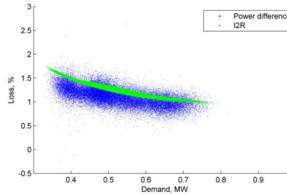
Figure 38 Aug 2018 Loss, % vs demand (Wavendon Gate Local HV feeder)
