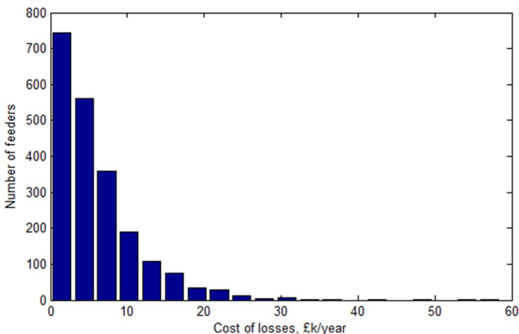
Figure 18 Cost of losses for feeders with accepted results, based on £48/MWh.
