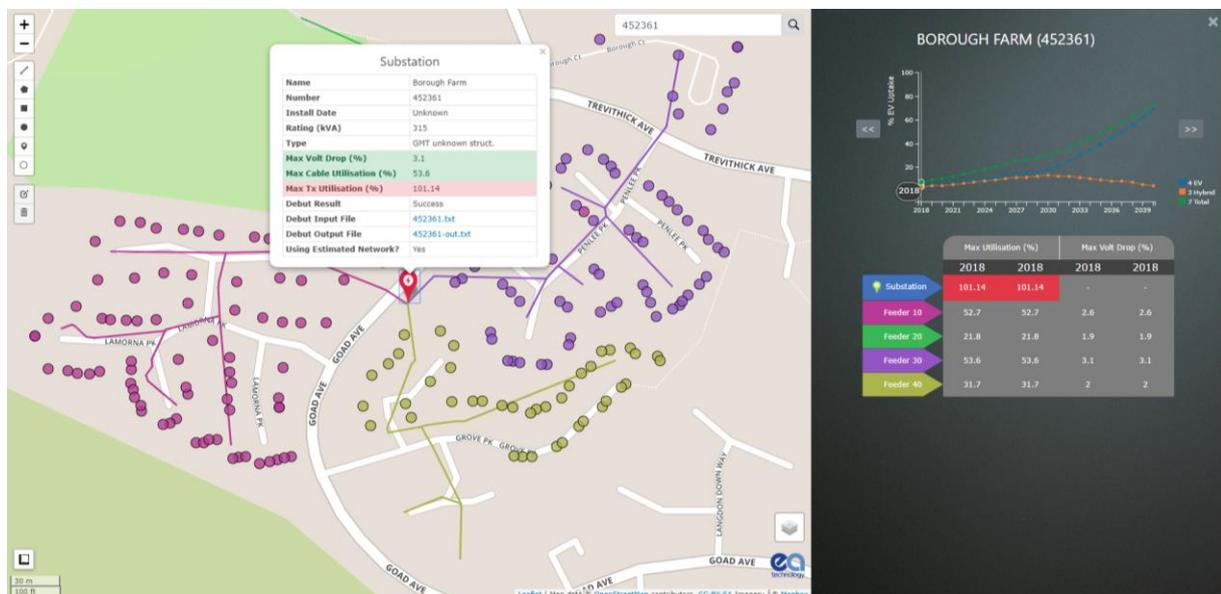
Figure 4: substation details pop-up
