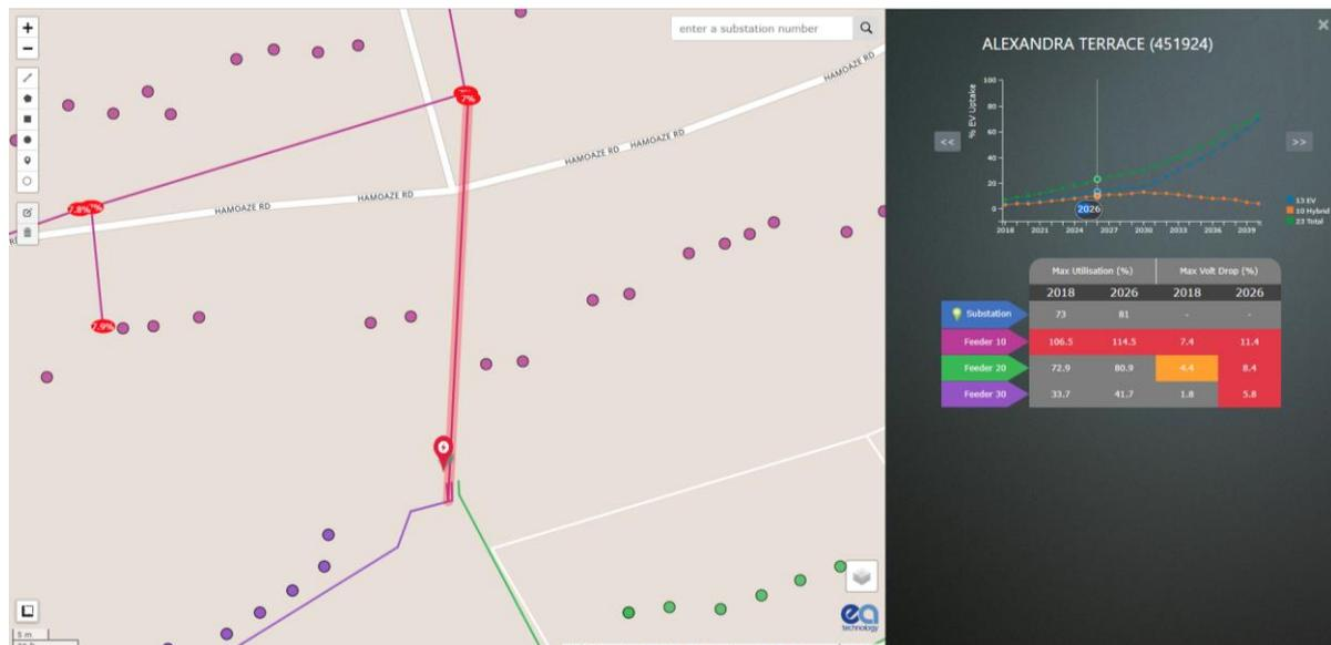
Figure 3: Example of mapped low voltage network showing over utilised cable segment highlighted
