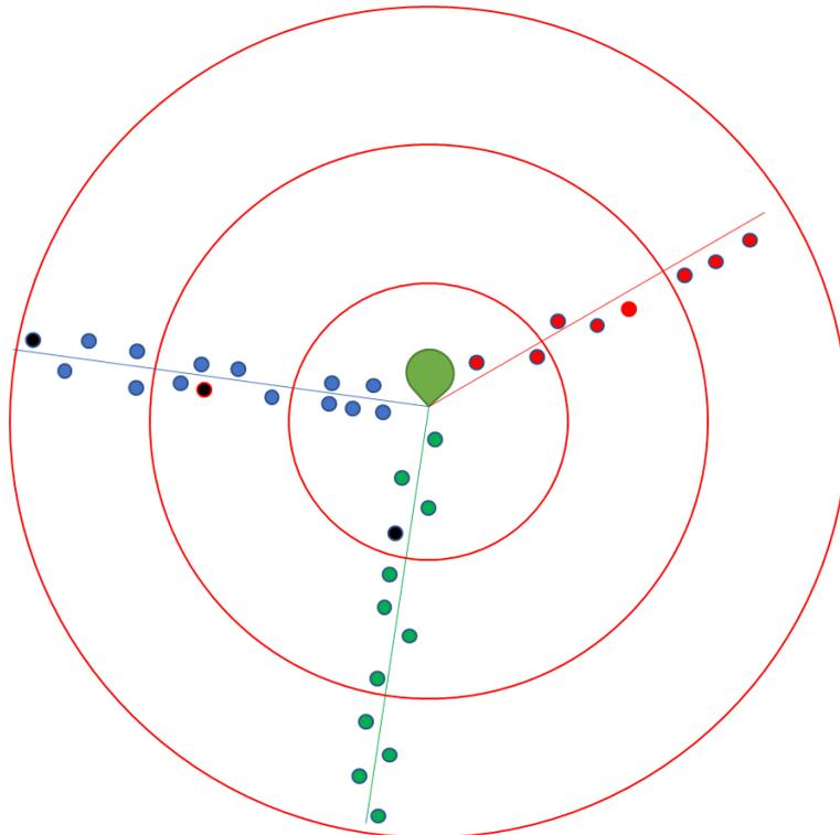
Figure 8: The first additional charger allocated to customer furthest away from substation (blue feeder) – in “furthest bucket”
