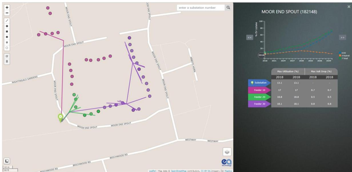
**Figure 1: Example of mapped Low Voltage network**
