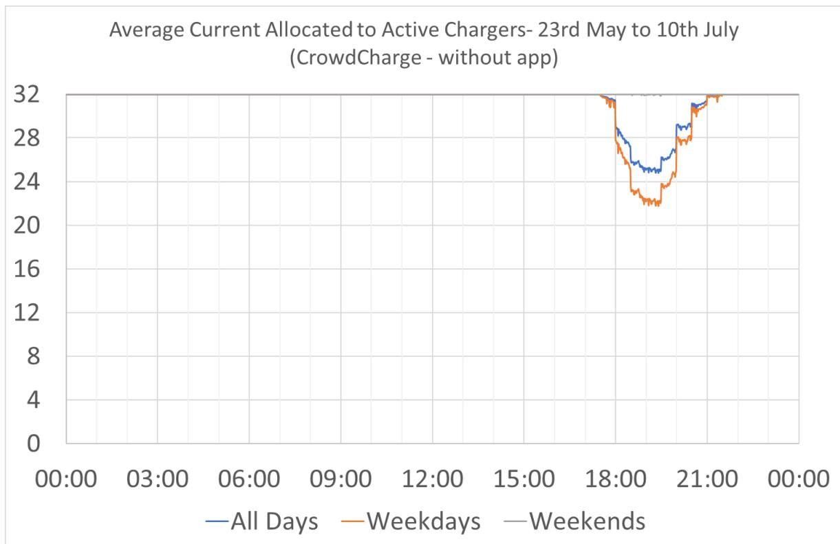
Figure 15: Average current during allocated to chargers 23<sup>rd</sup> May – 10<sup>th</sup> July 2018 (CrowdCharge)
