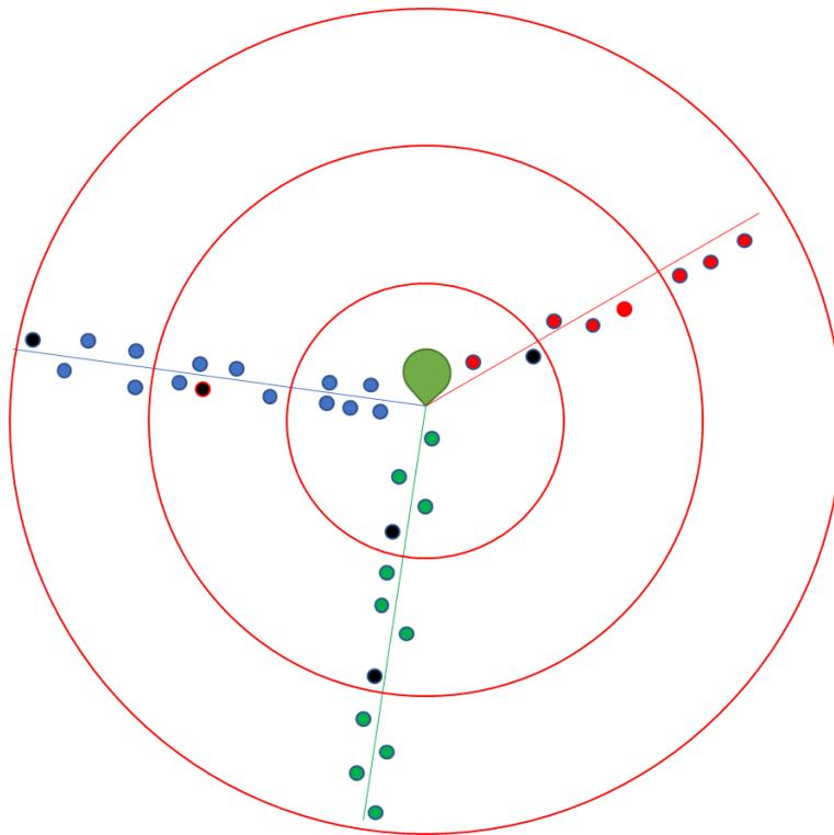
Figure 10: The third additional charger allocated to customer furthest from substation in “closest bucket” – this time on the red feeder
