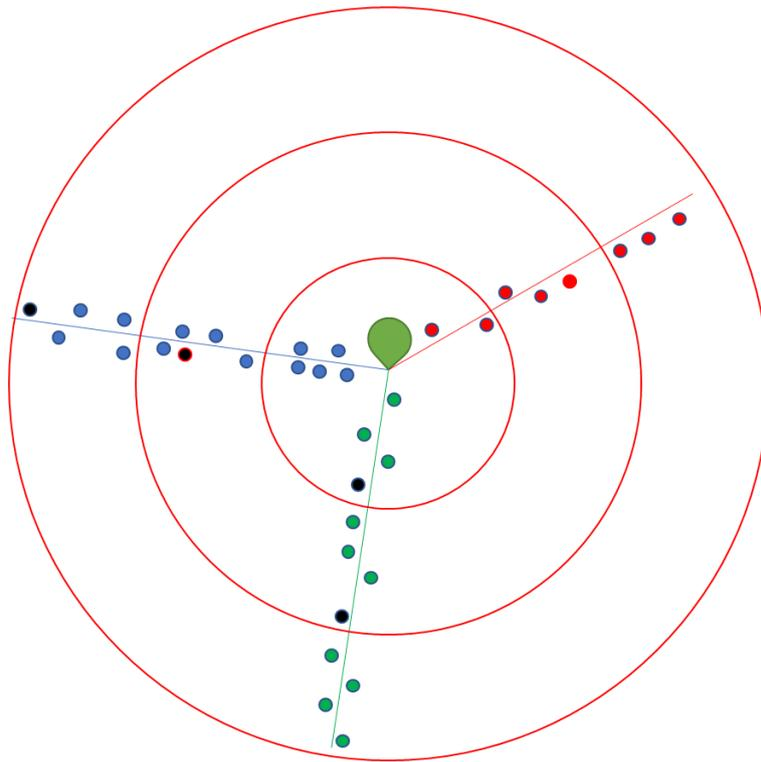
Figure 9: Second additional charger allocated to customer furthest away from substation in “middle bucket” – this time on green feeder
