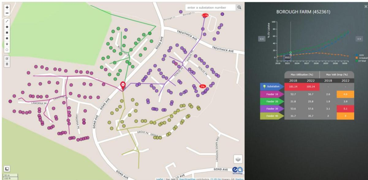
Figure 2: Example of mapped low voltage network with over-utilised substation and feeders with two near-maximum voltage drop and one over-maximum drop
