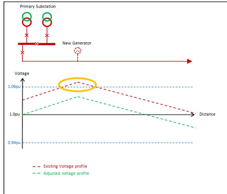
Figure 4: Traditional and amended voltage profiles
