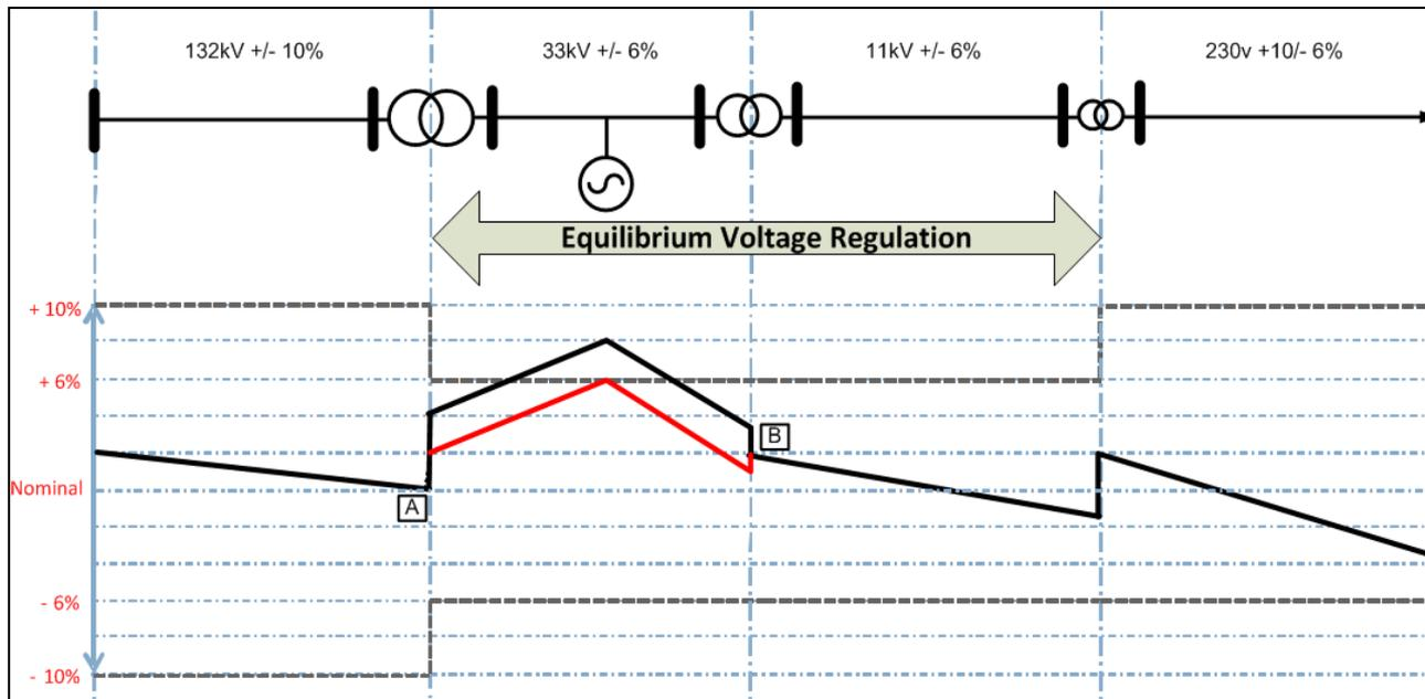
Figure 5: System Voltage Optimisation operation
