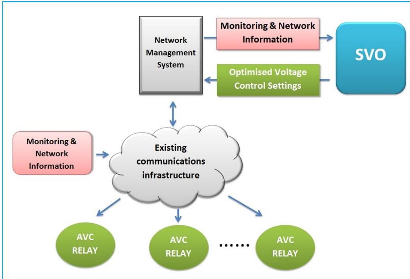
Figure 6: System Voltage Optimisation Architecture
