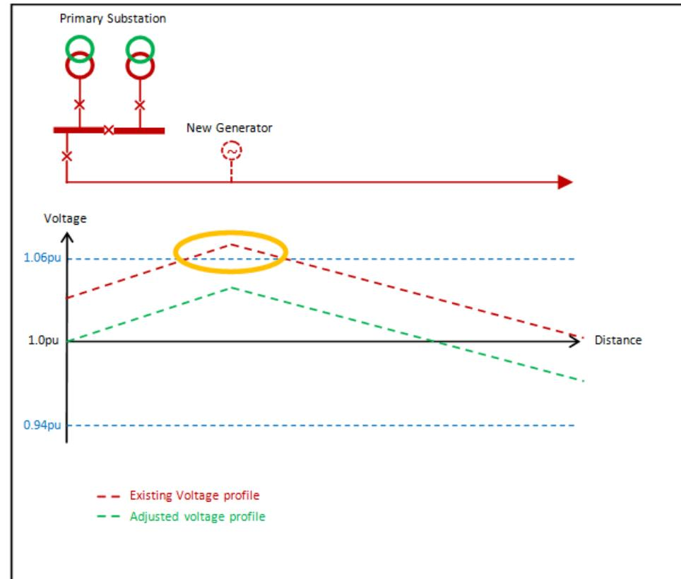
Figure 4: Traditional and amended voltage profiles
