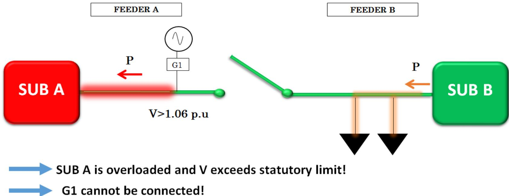
Figure 7: Thermal and voltage constraints preventing network connections.
