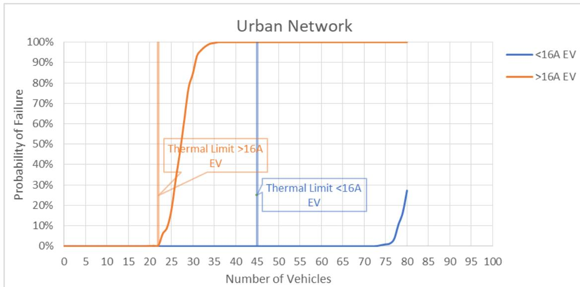
Figure 4-5: Urban network with a maximum source impedance of  $0.127+j0.068 \Omega$  with typical upper quartile EV harmonic current, WPD background harmonic distortion and  $Z_h$  calculated as per equation 2-2
