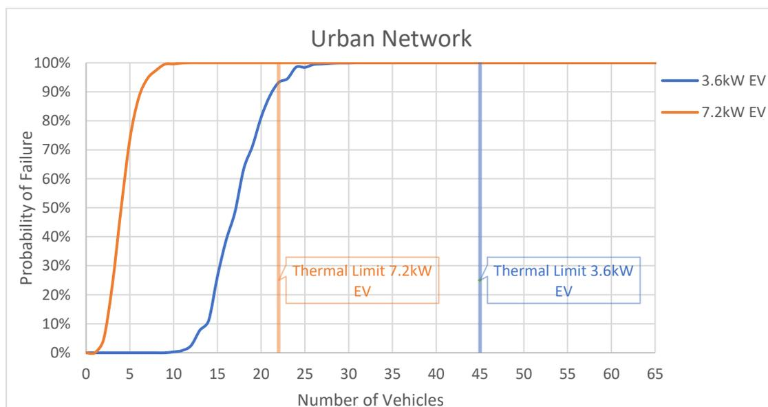
**Figure C-2: Urban network with typical upper quartile EV harmonic current, WPD background harmonic distortion and  $Z_h$  calculated as per equation 2-1**
