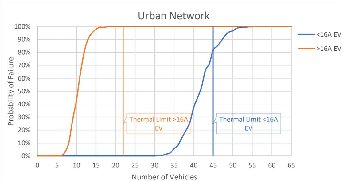
**Figure C-10:** Urban network with upper quartile EV profile, 0% background harmonic distortion and  $Z_h$  as per equation 2-2
