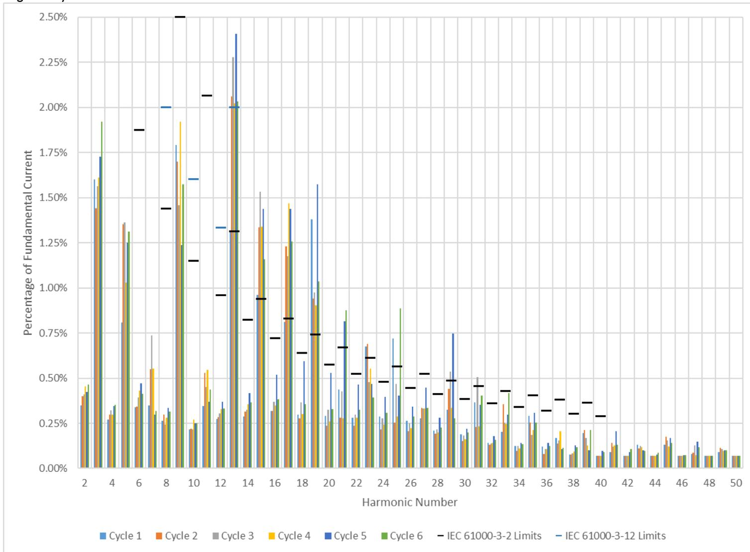
Figure 3-5: Vehicle 4 harmonic current compared against IEC 61000-3-2 and -12 limits
