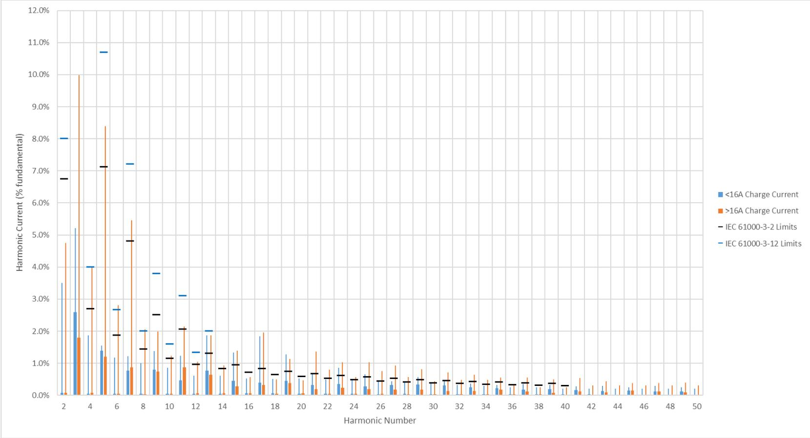
Figure 3-6: Median typical EV harmonic current assumed for <16 A and >16 A charge currents
