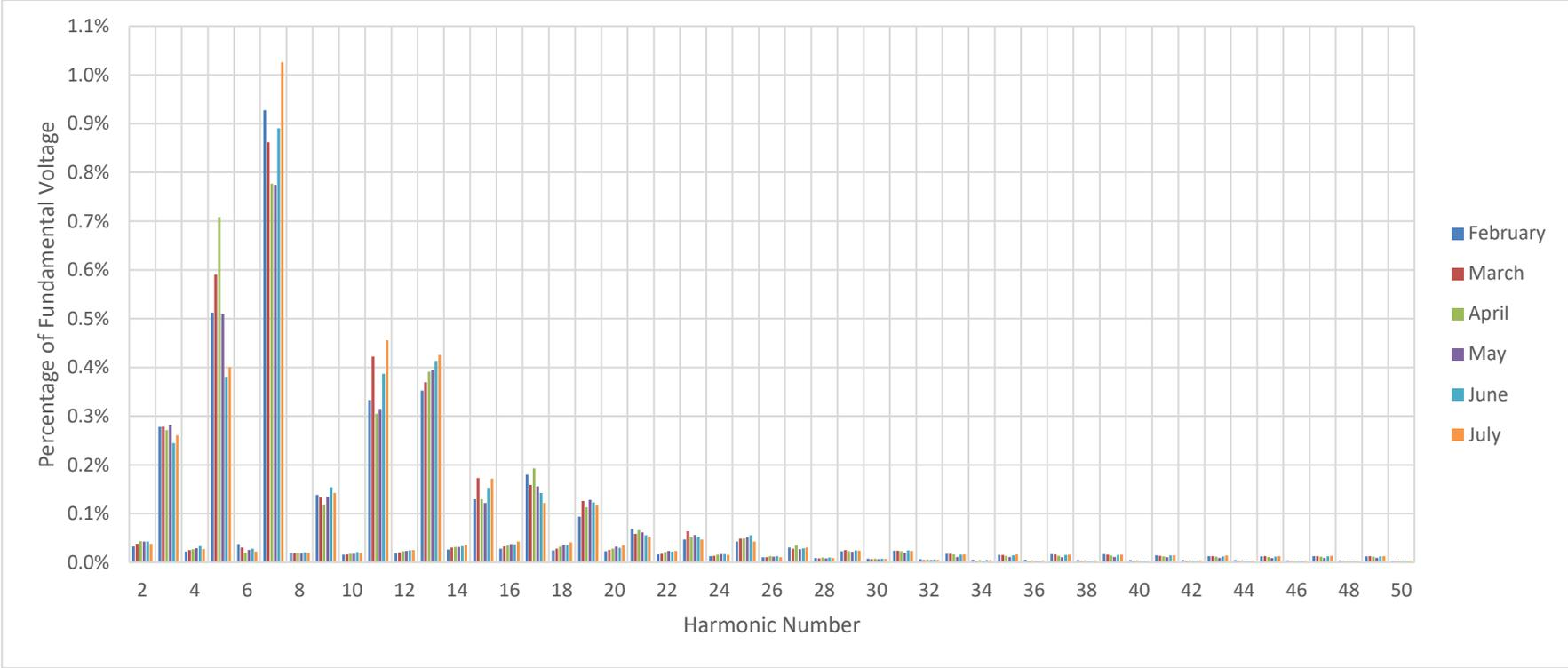
Figure 3-2: Background harmonic distortion on phase 2 during testing period
