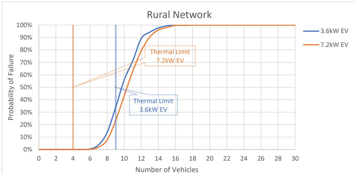
**Figure C-7: Rural network with median EV profile, 0% background harmonic distortion and  $Z_h$  as per equation 2-1**
