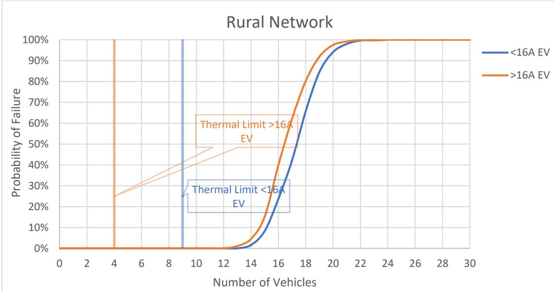
Figure 4-3: Rural network with typical median EV harmonic current, WPD background harmonic distortion and  $Z_h$  calculated as per equation 2-2
