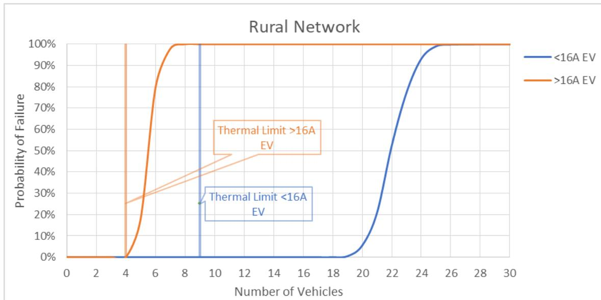
Figure 4-6: Rural network with a maximum source impedance of 0.21+j0.126 Ω with typical upper quartile EV harmonic current, WPD background harmonic distortion and Z<sub>h</sub> calculated as per equation 2-2
