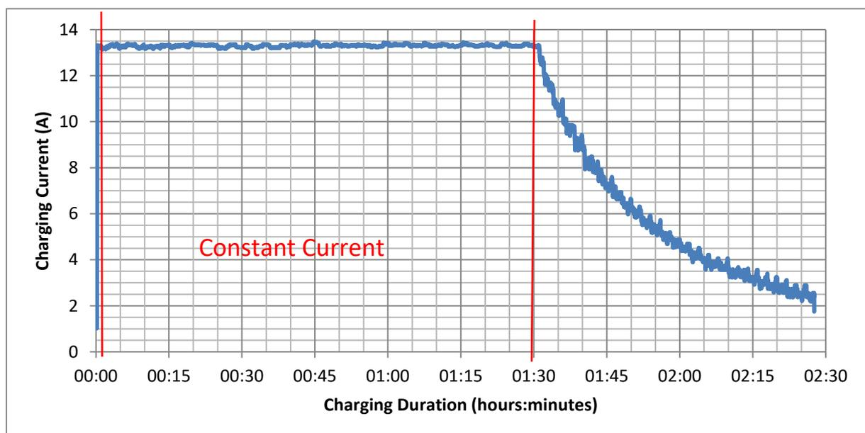
Figure 2-2: Typical 3.2 kW charging profile with extracted constant current section marked
