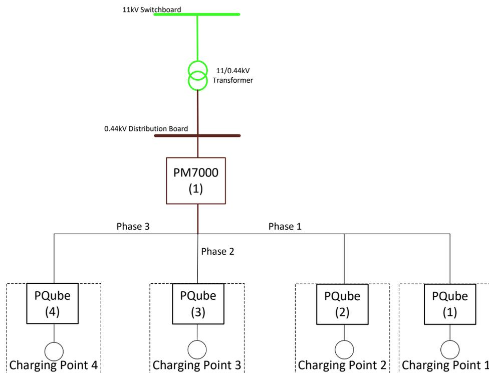
Figure 2-1: Vehicle charger and power quality measurement device arrangement
