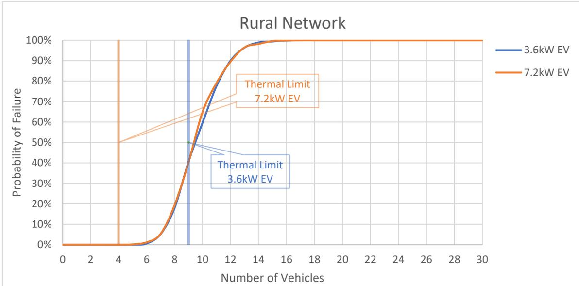
Figure C-5: Rural network with typical median EV harmonic current, WPD background harmonic distortion and  $Z_h$  calculated as per equation 2-1
