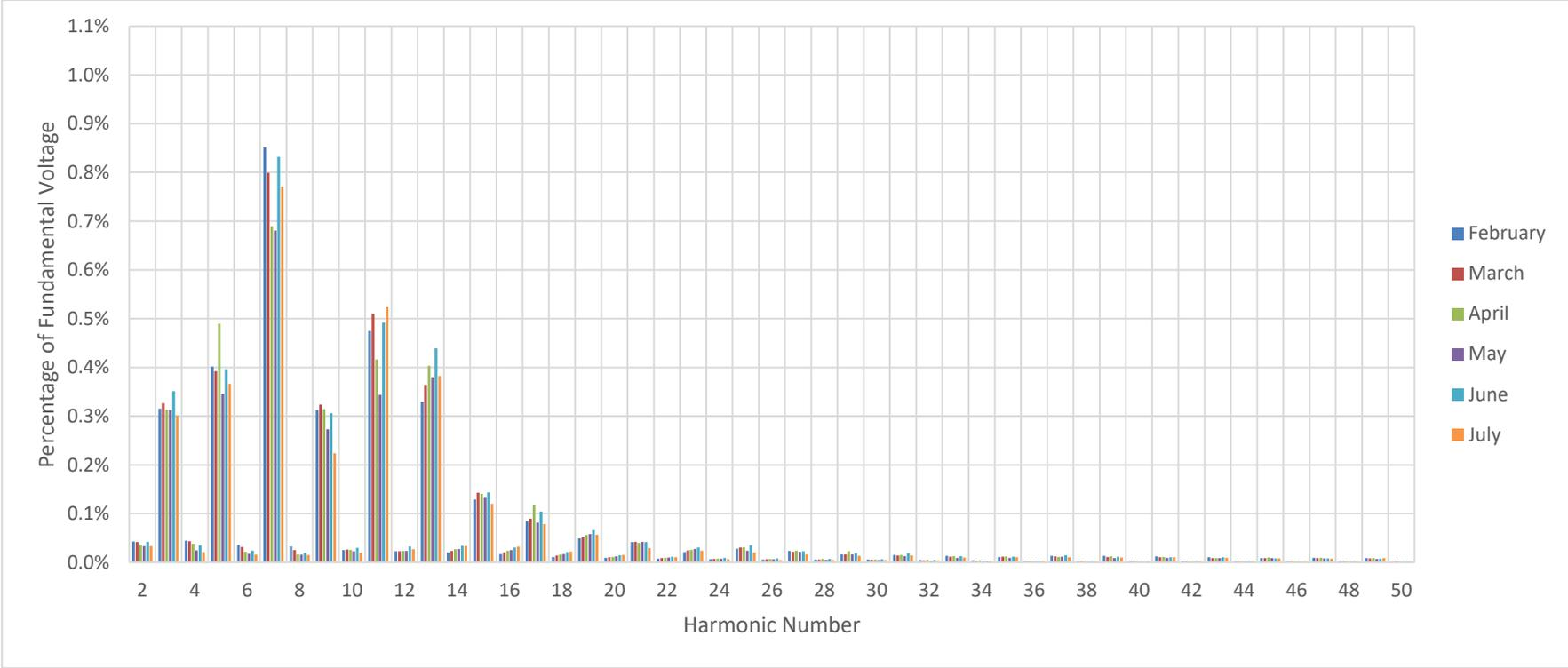
Figure 3-3: Background harmonic distortion on phase 3 during testing period
