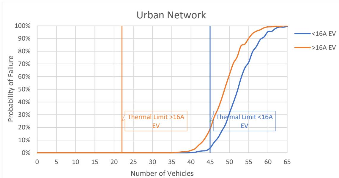
Figure 4-1: Urban network with median EV profile, WPD background harmonic distortion and  $Z_h$  as per equation 2-2
