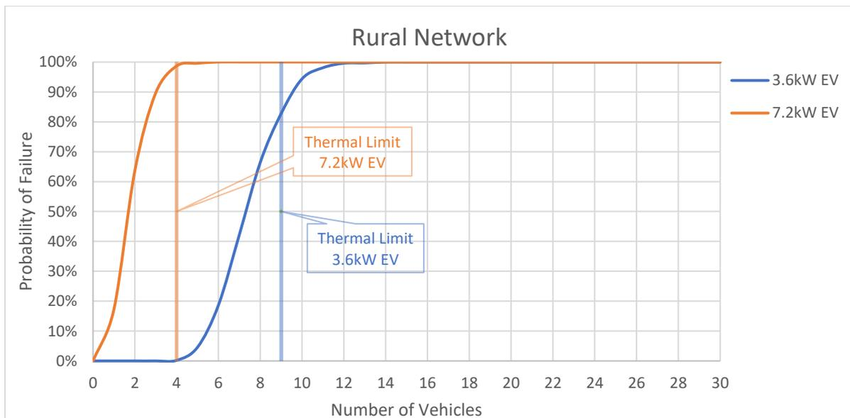
**Figure C-8: Rural network with upper quartile EV profile, 0% background harmonic distortion and  $Z_h$  as per equation 2-1**
