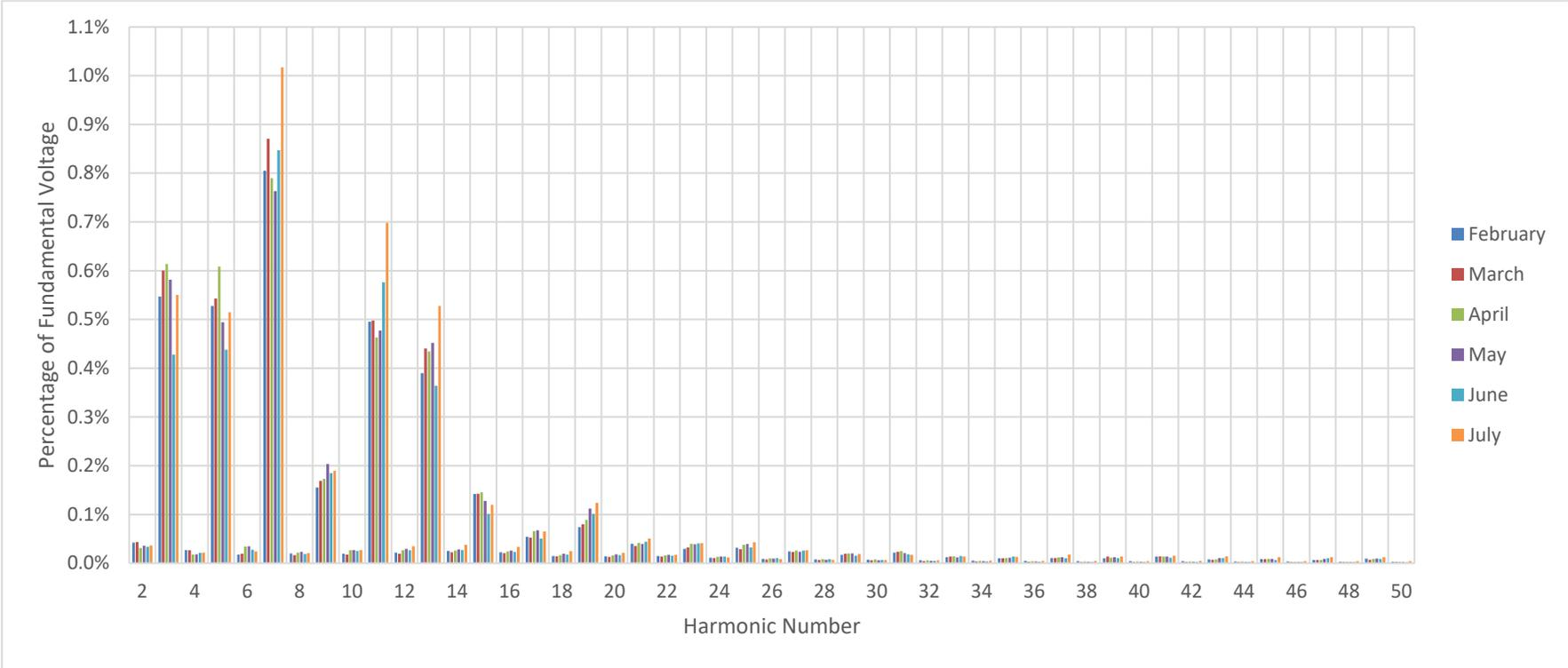
Figure 3-1: Background harmonic distortion on phase 1 during testing period
