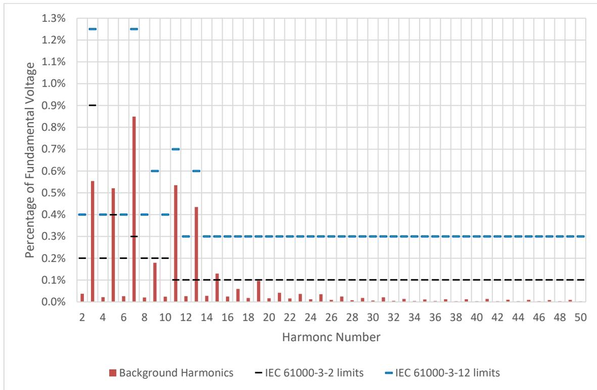
Figure 3-4: Average background voltage distortion compares against IEC 61000-3-2 and -12 limits
