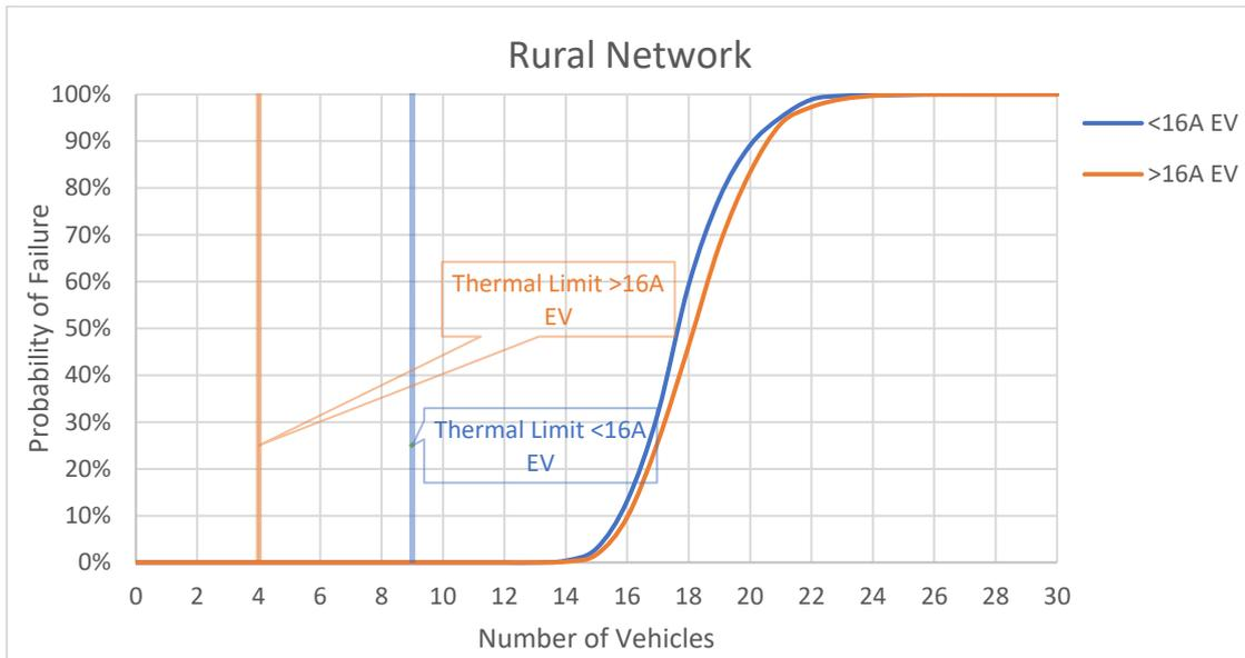
Figure C-11: Rural network with median EV profile, 0% background harmonic distortion and  $Z_h$  as per equation 2-2
