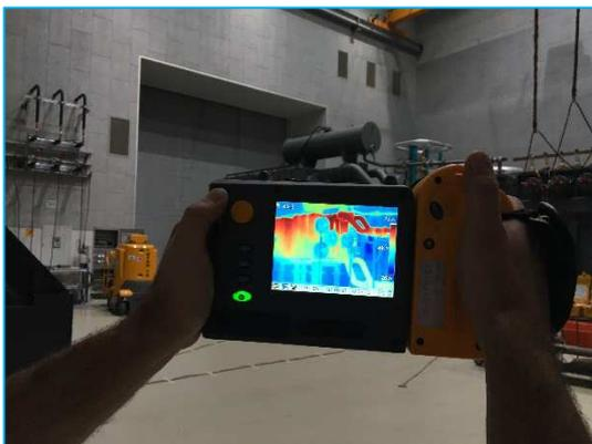
Figure 2-22: Temperature rise test
