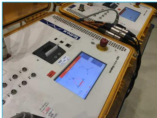
Figure 2-23: Winding resistance test
