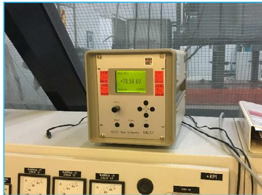
Figure 2-21: 70kV applied voltage test
