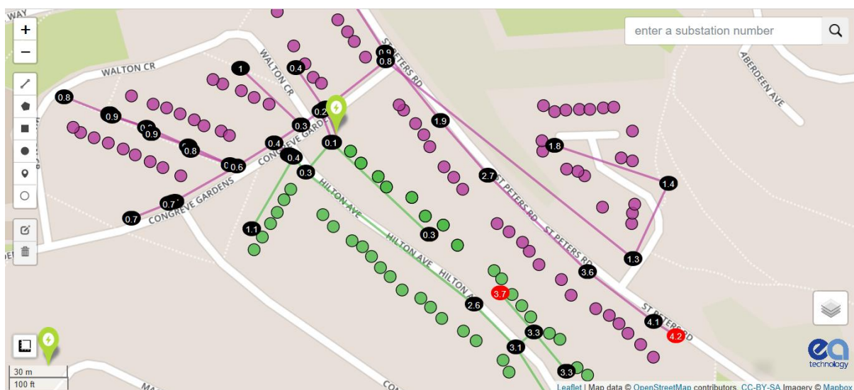
Figure 4: Substation view of the local network and associated assets and customers – colours show feeder/customer associations produced by the tool, the circled numbers show voltage drop at each cable segment node (black are intermediary, red are maximums)
