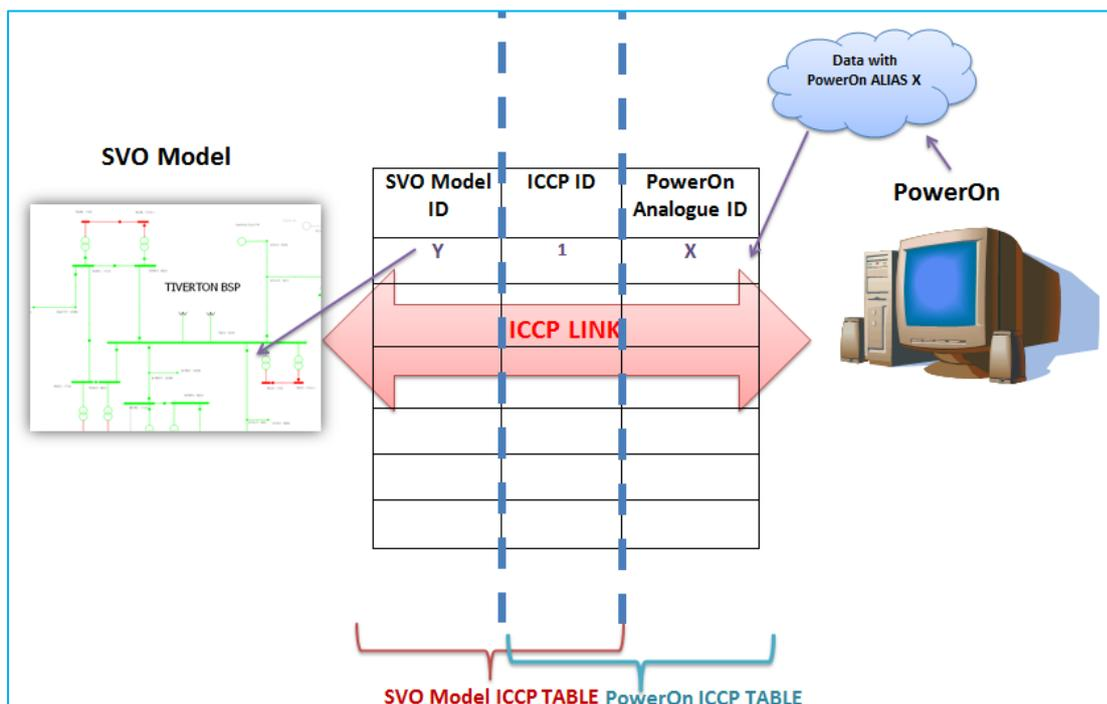
Figure 2-10 ICCP Bilateral Table and Linking of points to the network models.
