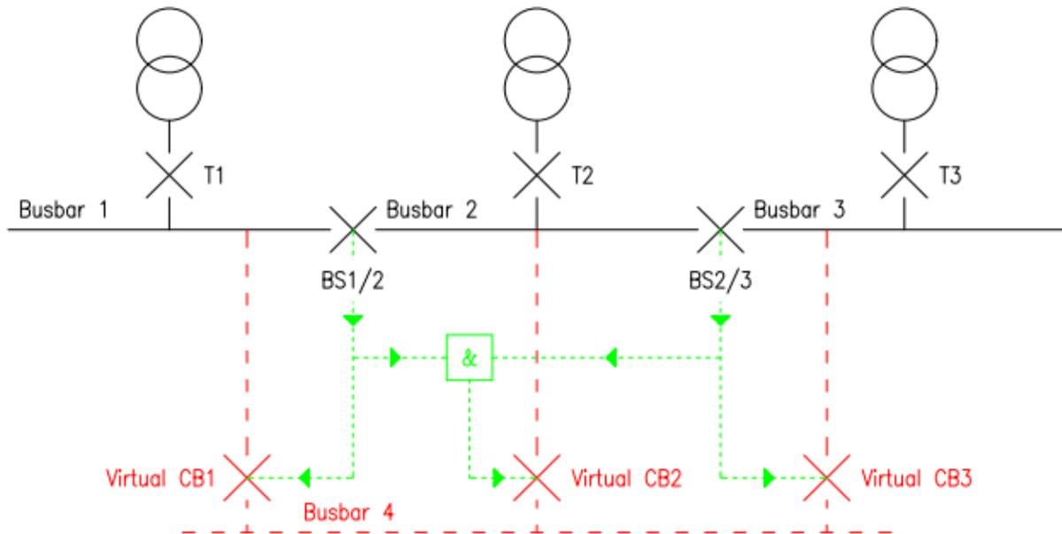
Figure 2-23: SuperTAPP SG Virtual Busbar Concept
