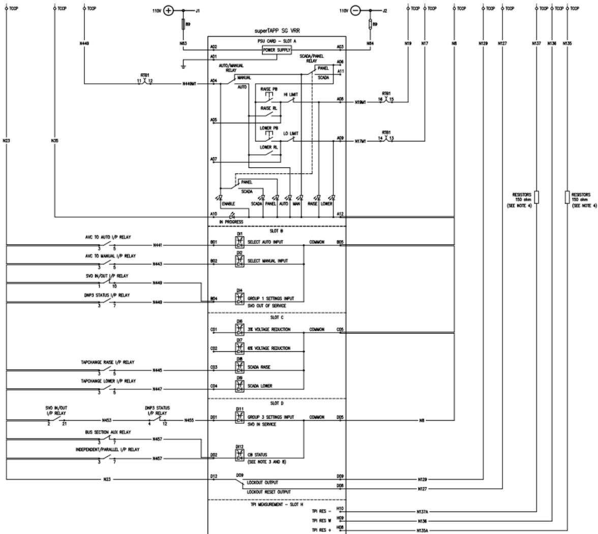
Figure 2-15: SuperTAPP SG Wiring Schematic
