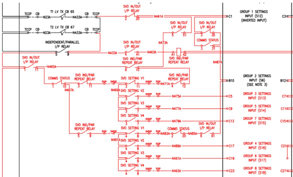
Figure 2-17: MicroTAPP Relay Interface Logic
