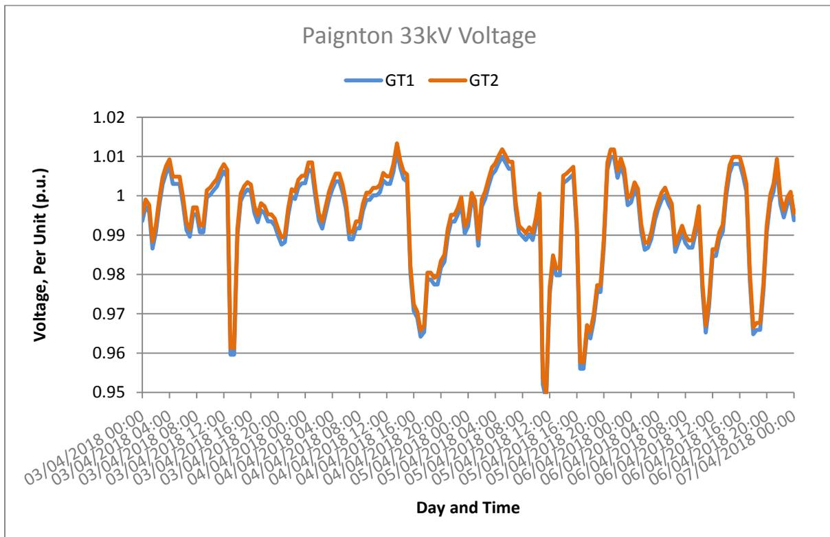
Figure 5-2 Paignton 33kV Voltage
