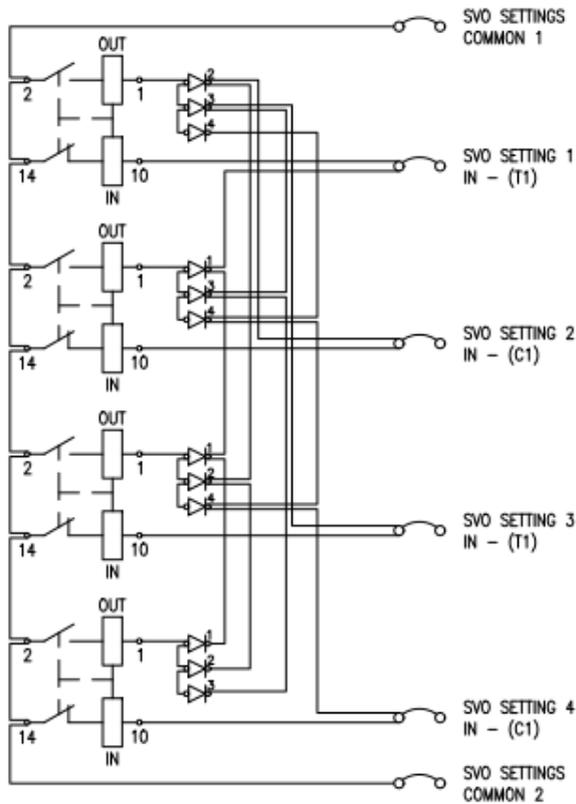
Figure 2-16: MicroTAPP SCADA Control Interface
