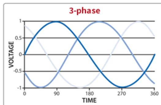
Three phase electricity is more commonly used in commercial and industrial connections.
