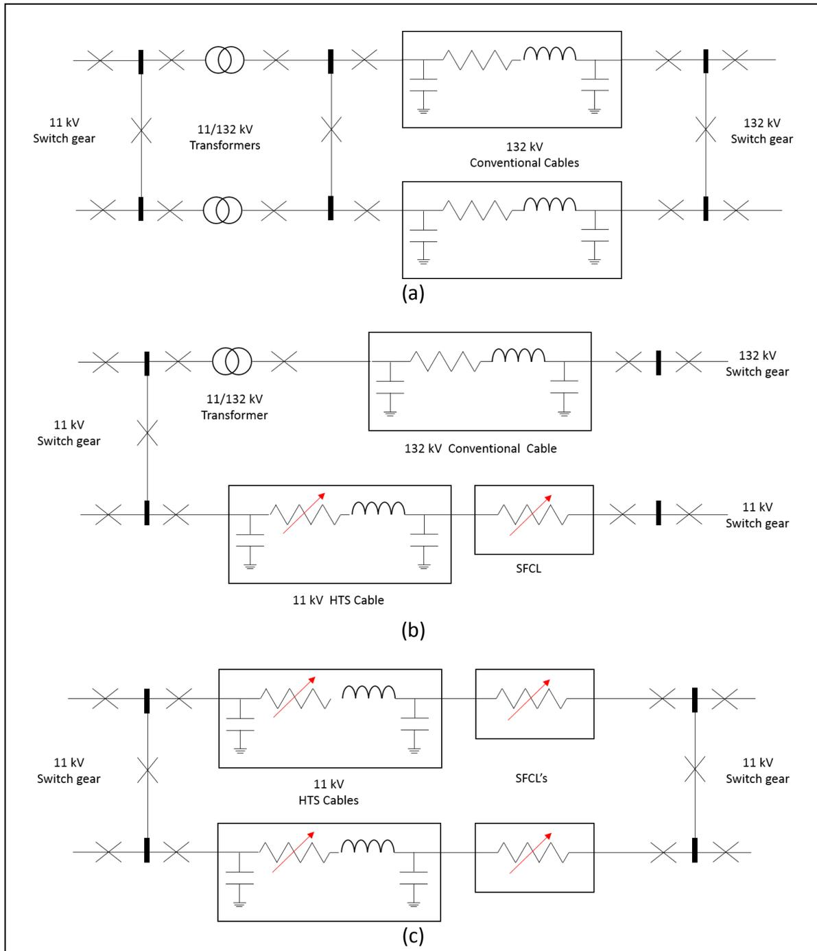
Figure 3.1: Layout diagrams for: (a) Conventional (b) Superconducting + Conventional and (c) Fully superconducting solutions.
