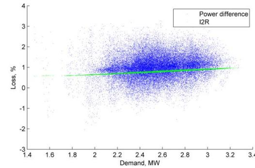
Figure 33 March 2017 Loss, % vs demand (Crawley Road Tee Howard Way HV feeder)
