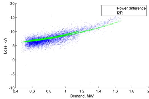
Figure 24 March 2017 Loss, kW vs demand (Wavendon Gate Local HV feeder)
