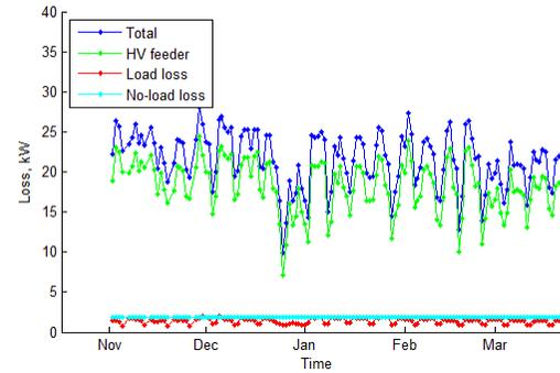
Figure 31 Long term mean daily loss (Crawley Road Tee Howard Way HV feeder)
