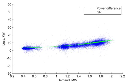
**Figure 7 March 2017 Loss, kW vs demand (Amway Tongwell HV feeder)**
