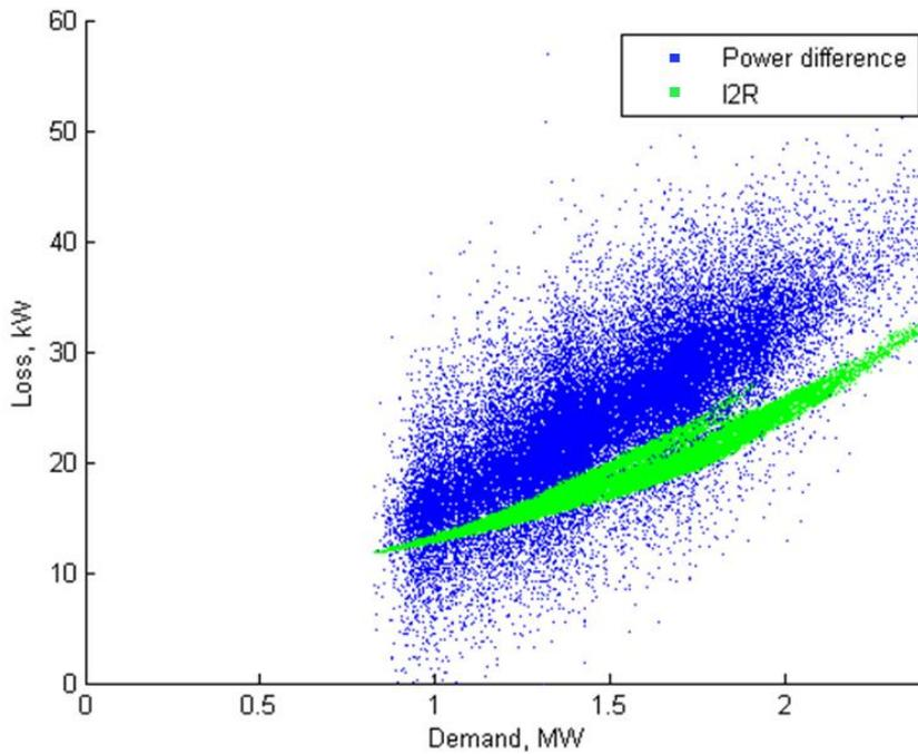
Figure 13 Pilot HV feeder losses for each 1 minute sample calculated with the power difference method and with the I<sup>2</sup>R method
