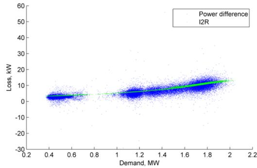
Figure 36 March 2017 Loss, kW vs demand (Amway Tongwell HV feeder)
