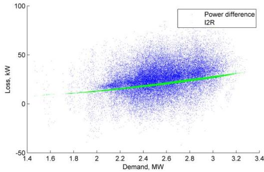
Figure 32 March 2017 Loss, kW vs demand (Crawley Road Tee Howard Way HV feeder)
