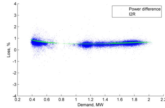
Figure 37 March 2017 Loss, % vs demand (Amway Tongwell HV feeder)
