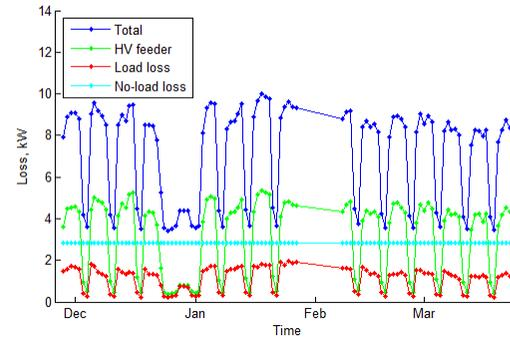
Figure 35 Long term mean daily loss (Amway Tongwell HV feeder)
