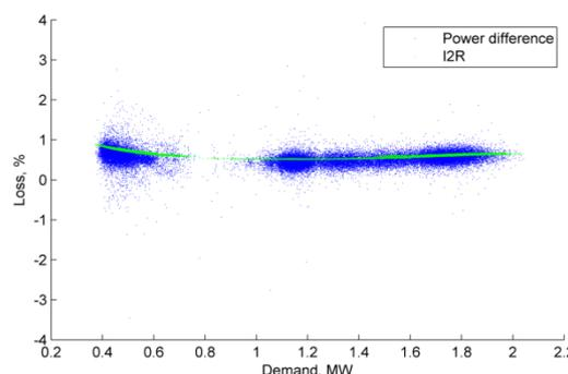
**Figure 8 March 2017 Loss, % vs demand (Amway Tongwell HV feeder)**
