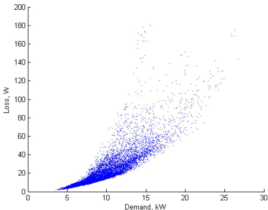
**Figure 12 Pilot LV feeder losses for each 1 minute sample calculated with I<sup>2</sup>R method**
