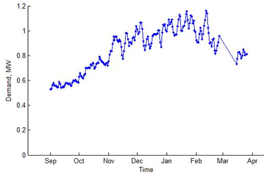
Figure 22 Long term mean daily feeder demand (Wavendon Gate Local HV feeder)
