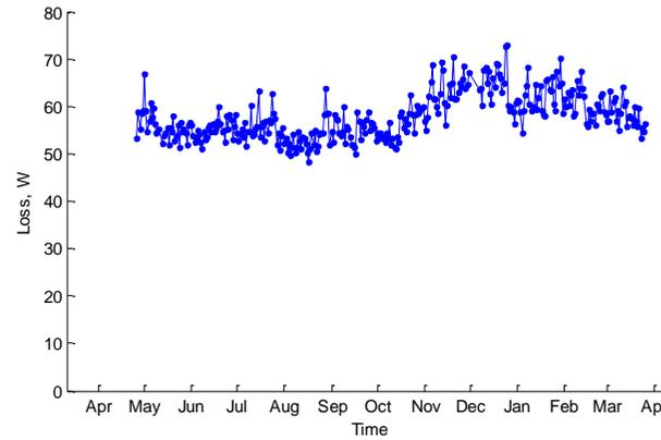
**Figure 43 Long term mean daily loss (Domestic Pilot LV feeder)**
