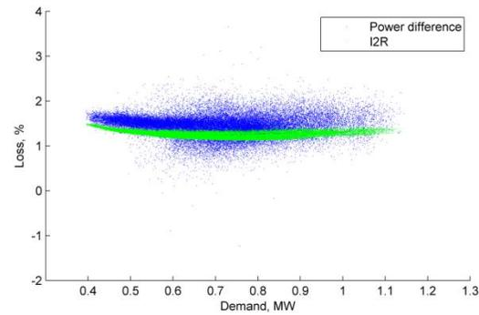
Figure 41 March 2017 Loss, % vs demand (Ackerman Tongwell Aldrich Drive Tee HV feeder)
