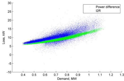
Figure 40 March 2017 Loss, kW vs demand (Ackerman Tongwell Aldrich Drive Tee HV feeder)
