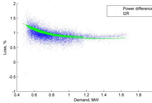
Figure 25 March 2017 Loss, % vs demand (Wavendon Gate Local HV feeder)
