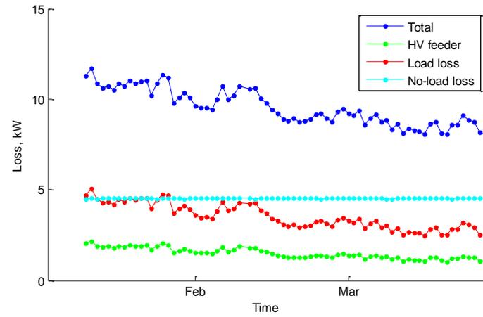
Figure 39 Long term mean daily loss (Ackerman Tongwell Aldrich Drive Tee HV feeder)
