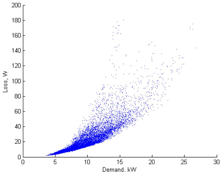
Figure 2 Pilot LV feeder losses for each 1 minute sample calculated with  $I^2R$  method
