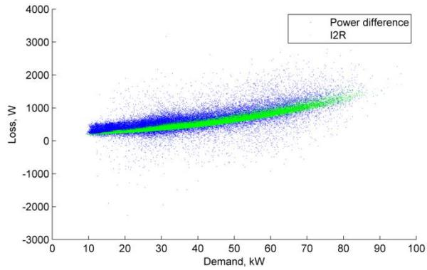
Figure 48 March 2017 Loss, kW vs demand (Laxey Domestic LV feeder)
