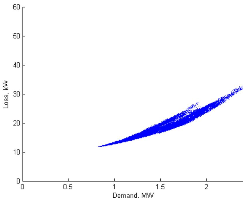
Figure 11 Pilot HV feeder losses for each 1 minute sample calculated with  $I^2R$  method
