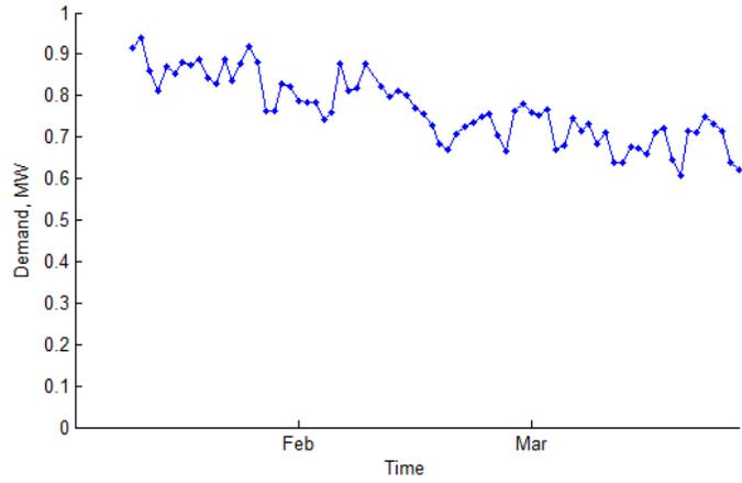
Figure 38 Long term mean daily feeder demand (Ackerman Tongwell Aldrich Drive Tee HV feeder)
