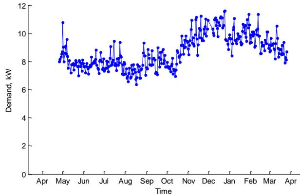
**Figure 42 Long term mean daily feeder demand (Domestic Pilot LV feeder)**
