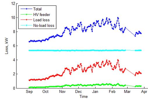
Figure 23 Long term mean daily loss (Wavendon Gate Local HV feeder)
