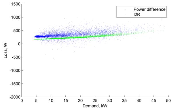
Figure 52 March 2017 Loss, kW vs demand (Ramsey Domestic LV feeder)
