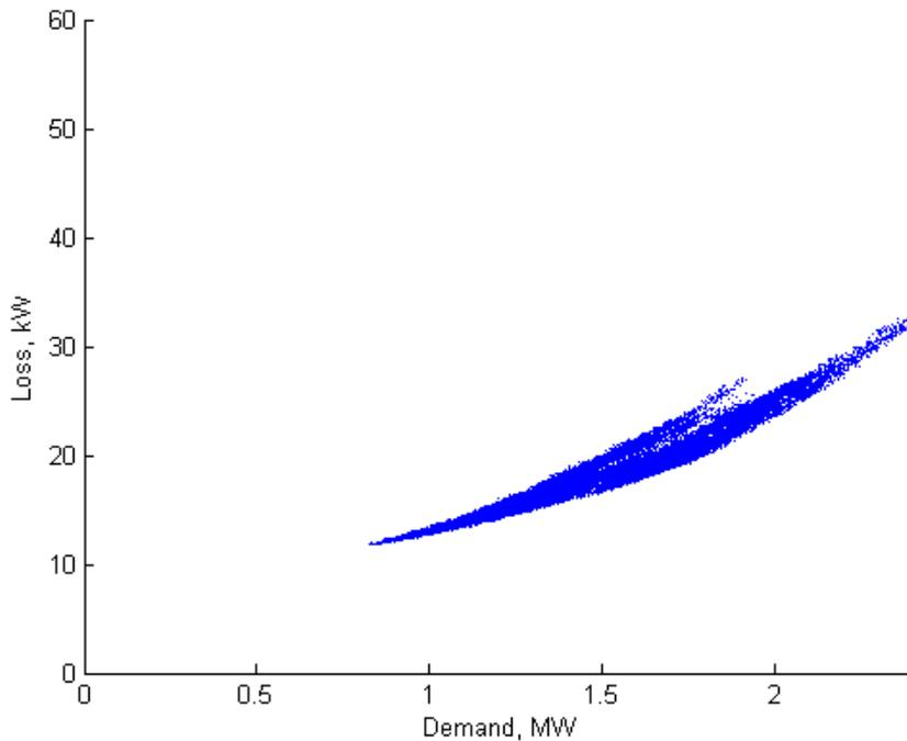
**Figure 1 Pilot HV feeder losses for each 1 minute sample calculated with  $I^2R$  method**
