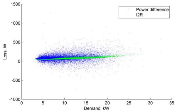
**Figure 44 March 2017 Loss, kW vs demand (Domestic Pilot LV feeder)**
