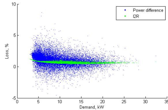
**Figure 45 March 2017 Loss, % vs demand (Domestic Pilot LV feeder)**
