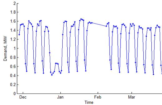
Figure 34 Long term mean daily feeder demand (Amway Tongwell HV feeder)
