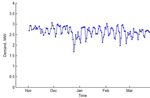
Figure 30 Long term mean daily feeder demand (Crawley Road Tee Howard Way HV feeder)
