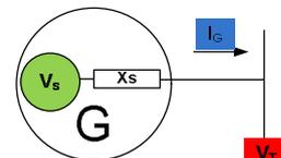
Figure 1: Thevenin model of a generator connected to the network
