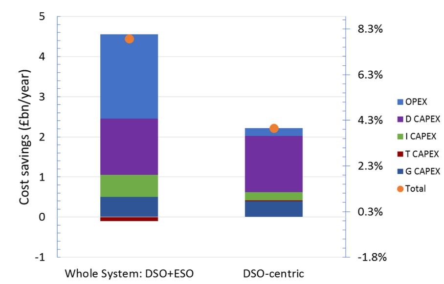
**Figure 4. Potential benefits of improved transmission and distribution control interface. Right vertical axis shows cost savings relative to total system cost without added flexibility. DSO = Distribution System Operator, ESO = Electricity System Operator**
