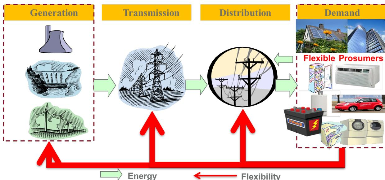
**Figure 1. Energy flows from Grid to consumers while the flexibility flows from prosumers to the grid**
