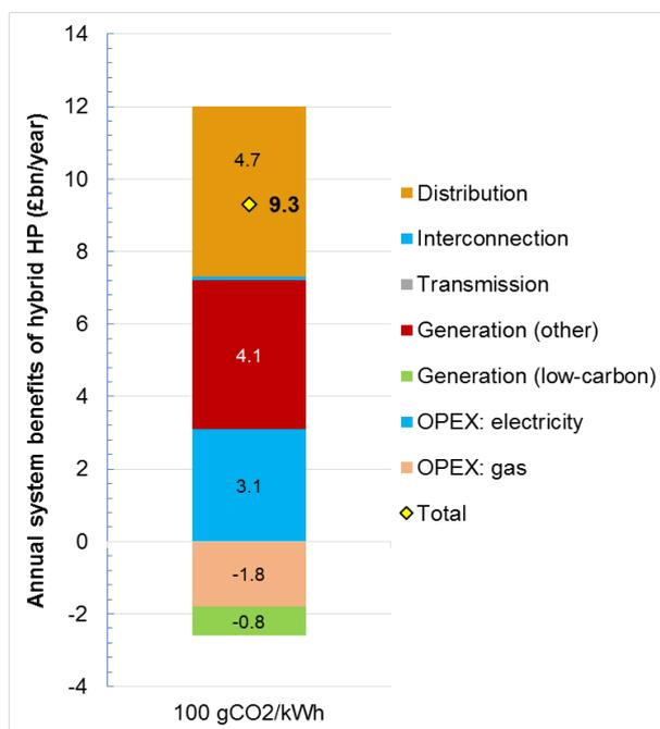
**Figure 6. System-level benefits of hybrid heat pumps in the future GB power system with the carbon target of 100 gCO<sub>2</sub>/kWh<sup>9</sup>**
