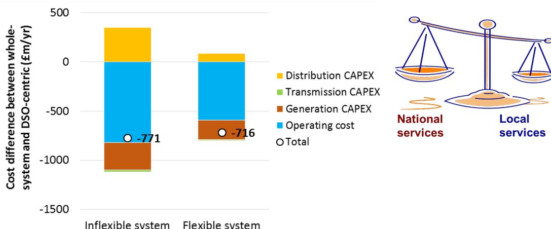
**Figure 5. Impact of generation flexibility on the role and value of demand-side flexibility. Cost differences shown are between whole-system and DSO-centric approaches, for two flexibility levels of conventional generation fleet**
