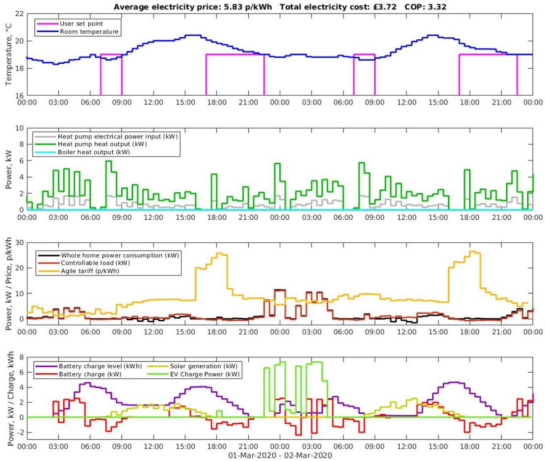
**Figure 8.3 - Full simulation run under Phase 3 control (Digital twin of Home 2, 01/03/2020 - 02/03/2020)**
