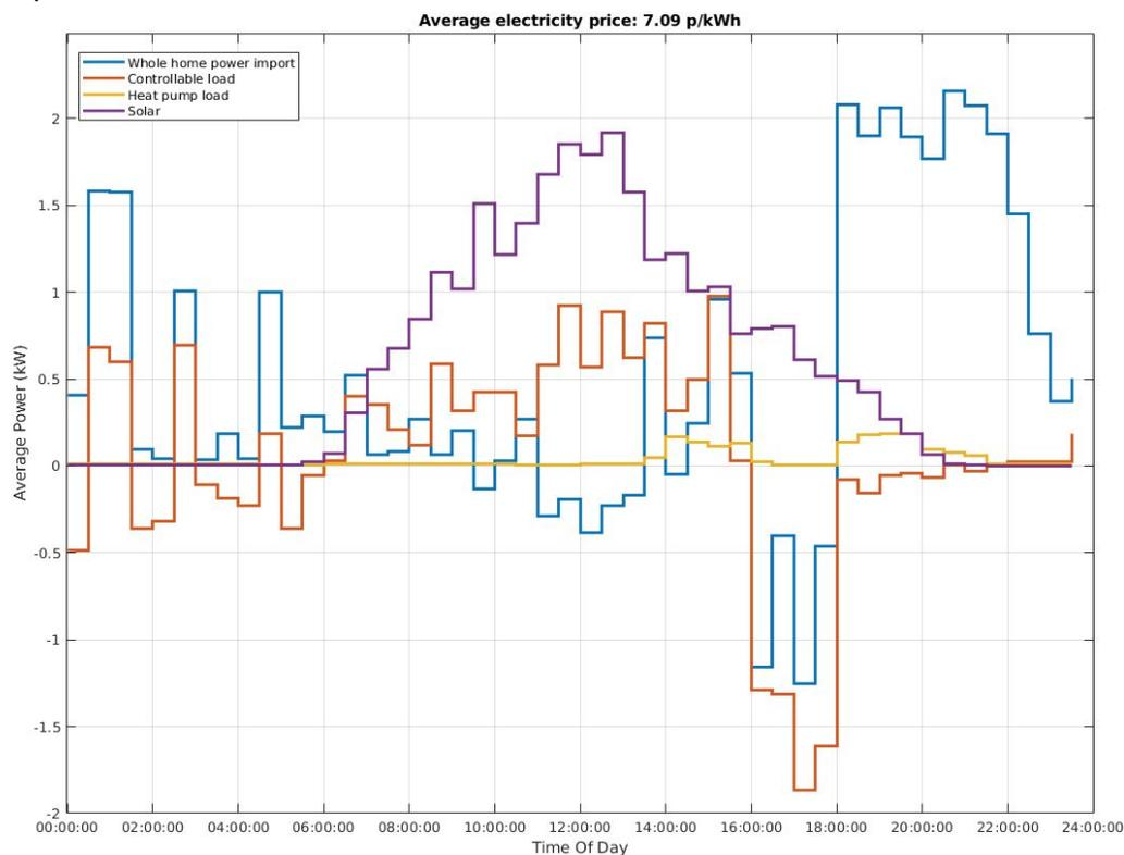
**Figure 3.24 - Average load profiles during Secure Flexible Power intervention (All homes, 08/06/2020). Controllable load is the combination of heat pump, battery and EV in this case.**
