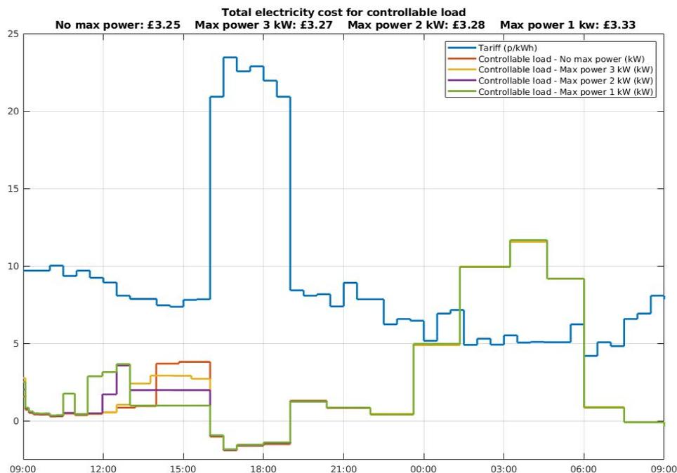
Figure 4.4 - Simulated controllable load on the Octopus Agile tariff with a range of maximum power limits between 13:00 - 16:00 (Digital twin of Home 5, 03/01/2020 - 04/01/2020)
