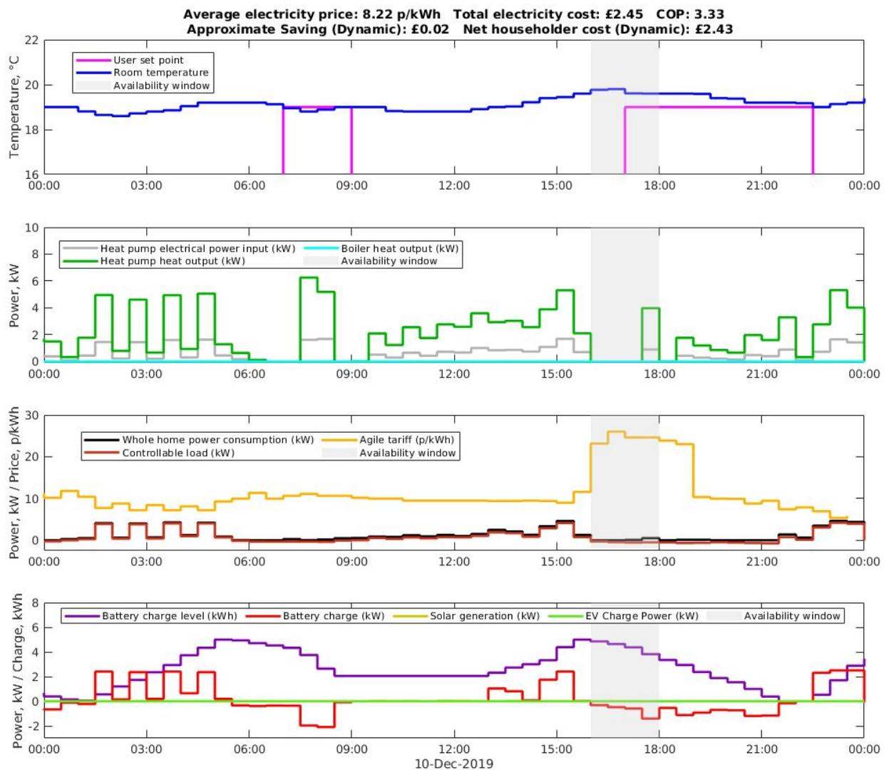
**Figure 9.2 - Full simulation run, available for 16:00 - 18:00 but request is not utilised on the Octopus Agile tariff (Digital twin of Home 2, 10/12/2019)**
