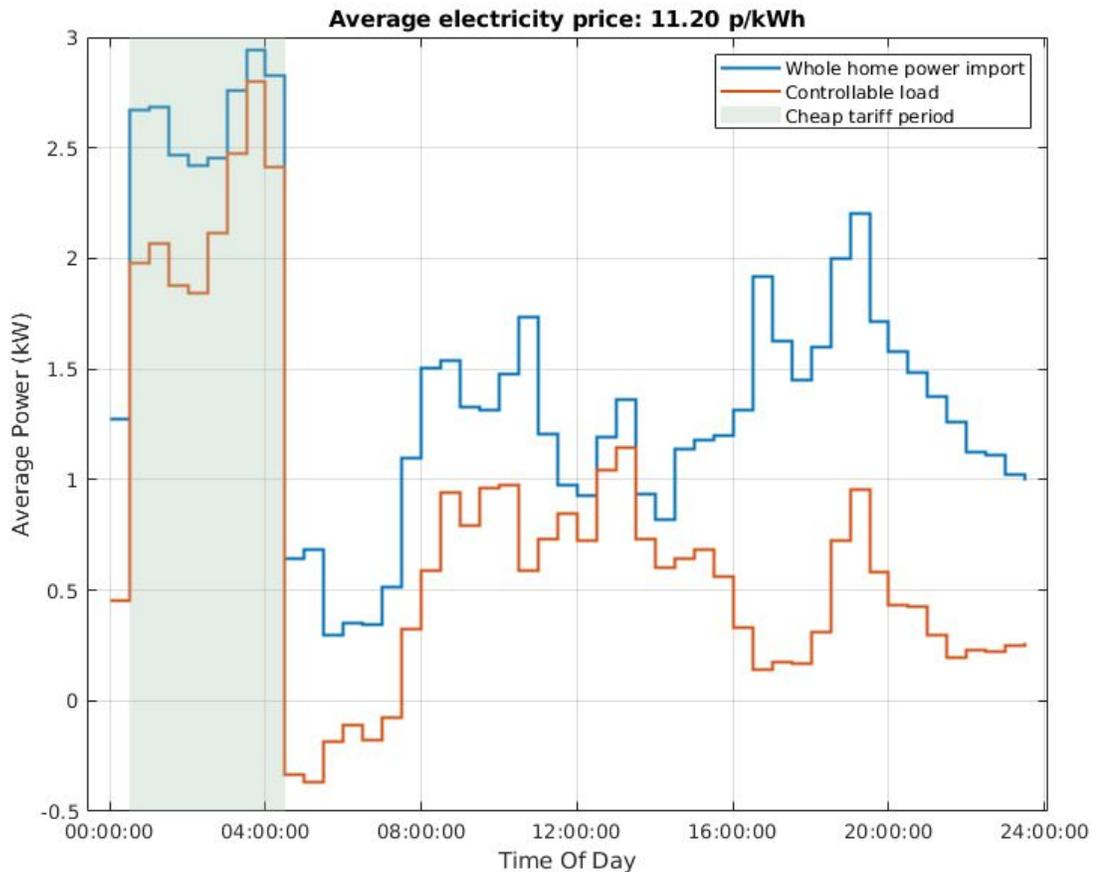
Figure 3.7 - Average load profiles for phase 2 operation on Octopus Go tariff (All homes, 18/02/2020 - 27/02/2020, note that three days worth of data were excluded from this range due to interventions which significantly affected the demand profile). Controllable load is the combination of heat pump and battery in this case. Whole home power import = import from (/export to) the grid.
