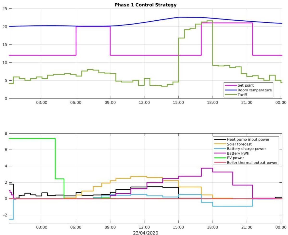
Figure 4.1- Optimisation output under Phase 1 control (Digital twin of Home 5, 23/04/2020)
