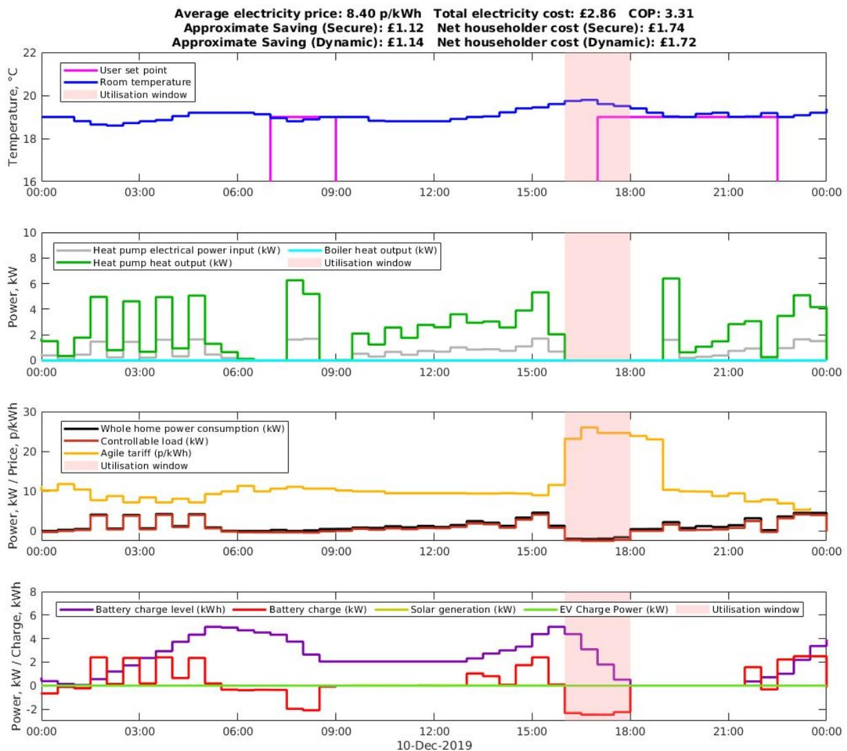
Figure 9.3 - Full simulation run, 16:00 - 18:00 request utilised on the Octopus Agile tariff (Digital twin of Home 2, 10/12/2019)
