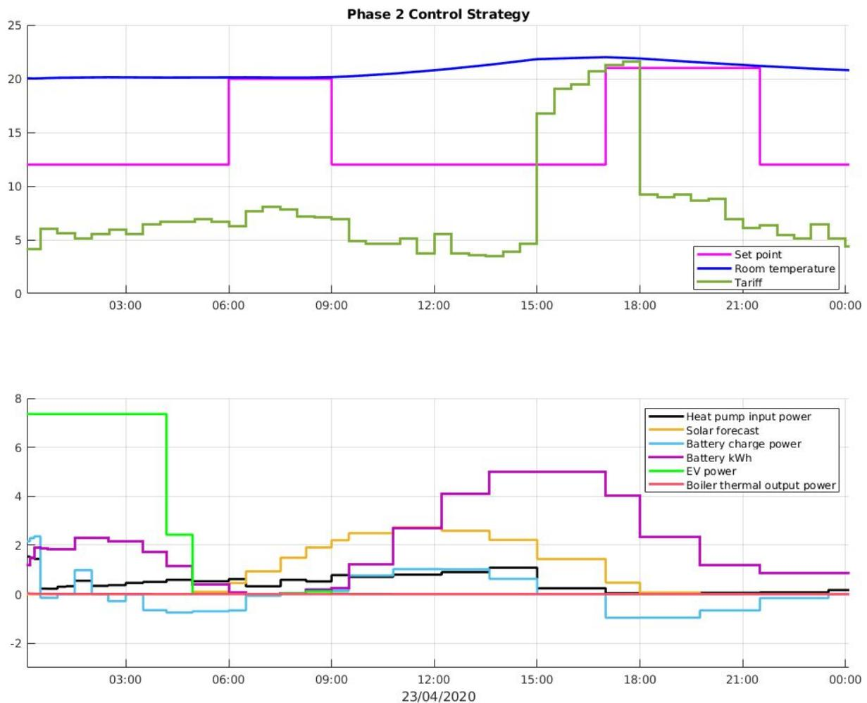
Figure 4.2 - Optimisation output under Phase 2 control (Digital twin of Home 5, 23/04/2020)
