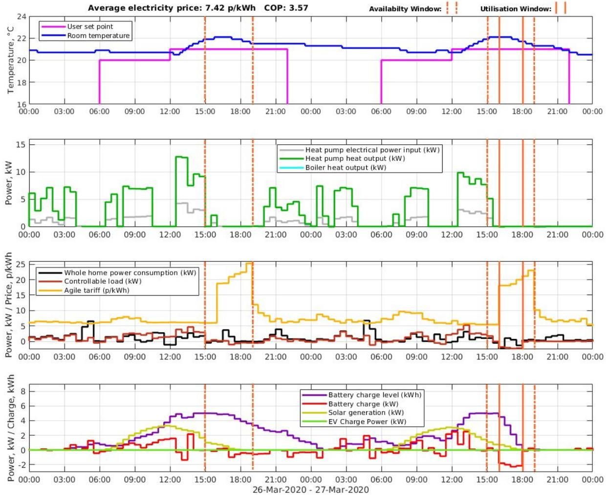
Figure 3.25 - Dynamic Flexible Power intervention (*Home 3, 26/03/2020*). Controllable load is the combination of heat pump and battery in this case.
