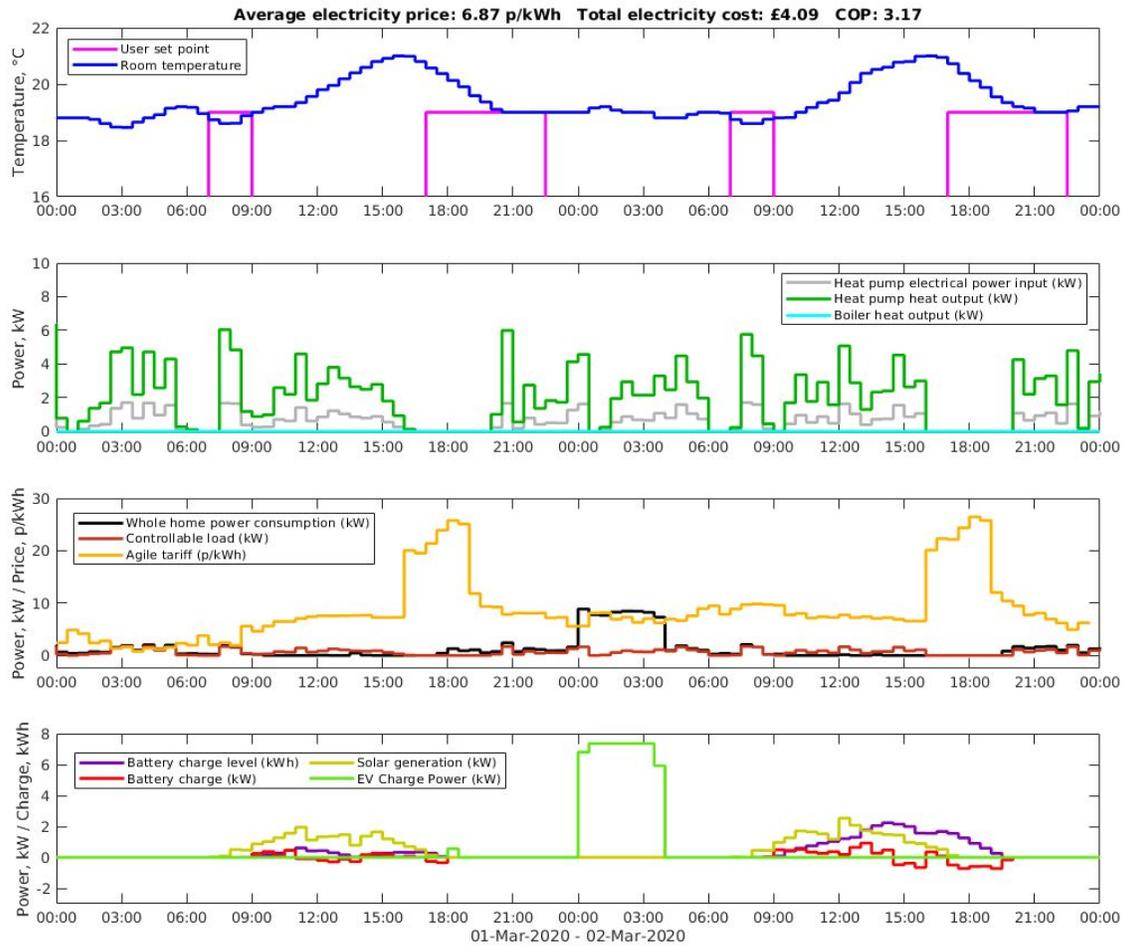
**Figure 8.1 - Full simulation run under Phase 1 control with smart EV charging (Digital twin of Home 2, 01/03/2020 - 02/03/2020)**
