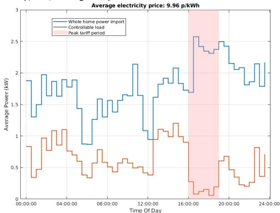
Figure 3.4 - Average load profiles for baseline operation on Octopus Agile tariff (All homes, 10/01/2020 - 16/01/2020). Controllable load is just the heat pump in this phase. Whole home power import = import from (/export to) the grid.
