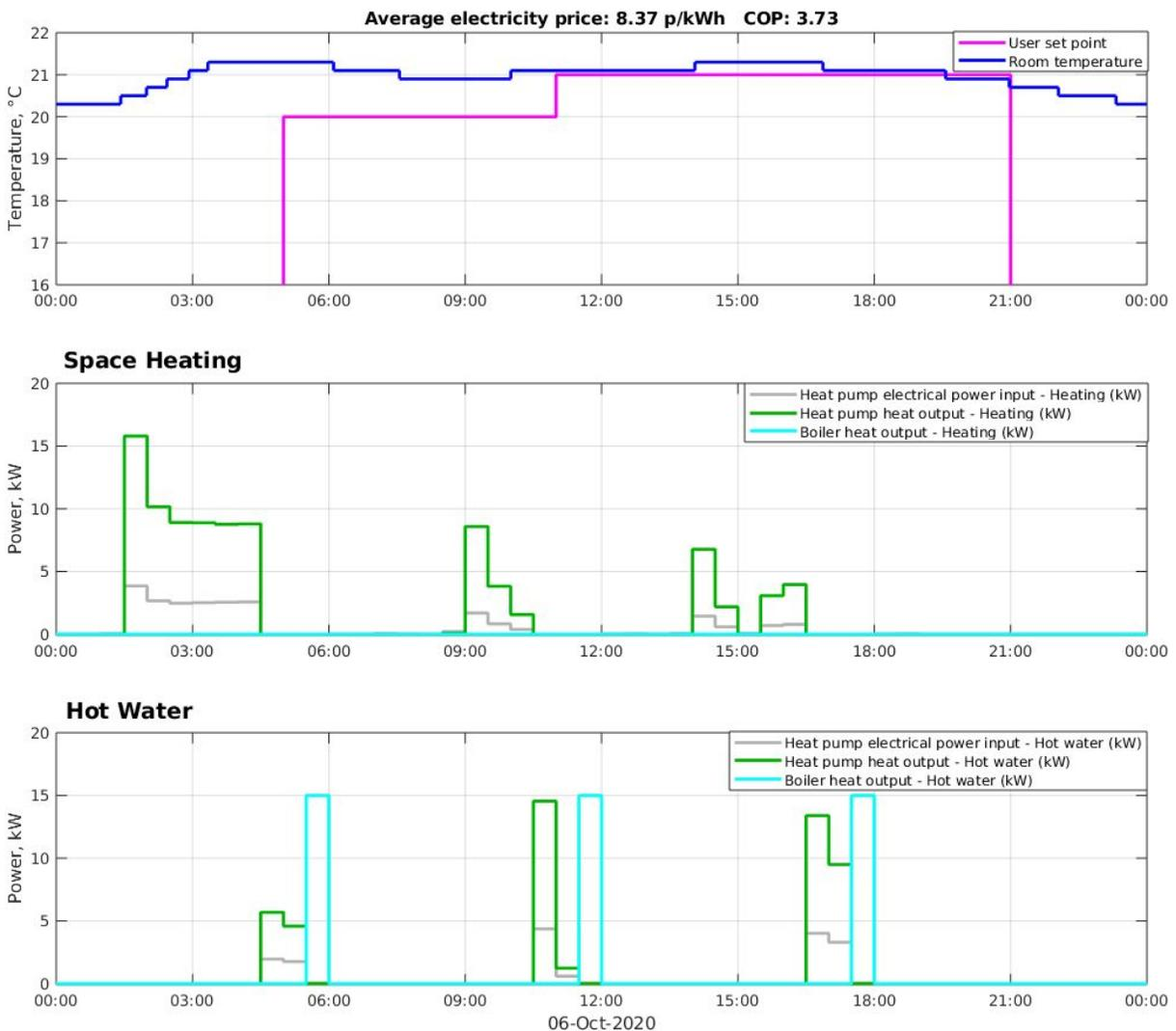
**Figure 10.4 - Hot water intervention (Home 03, 06/10/2020). Note that the boiler heat output is estimated as this home does not have a boiler heat meter.**
