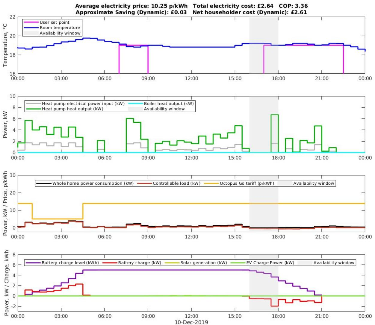
**Figure 9.5 - Full simulation run, available for 16:00 - 18:00 but request is not utilised on the Octopus Go tariff (Digital twin of Home 2, 10/12/2019)**
