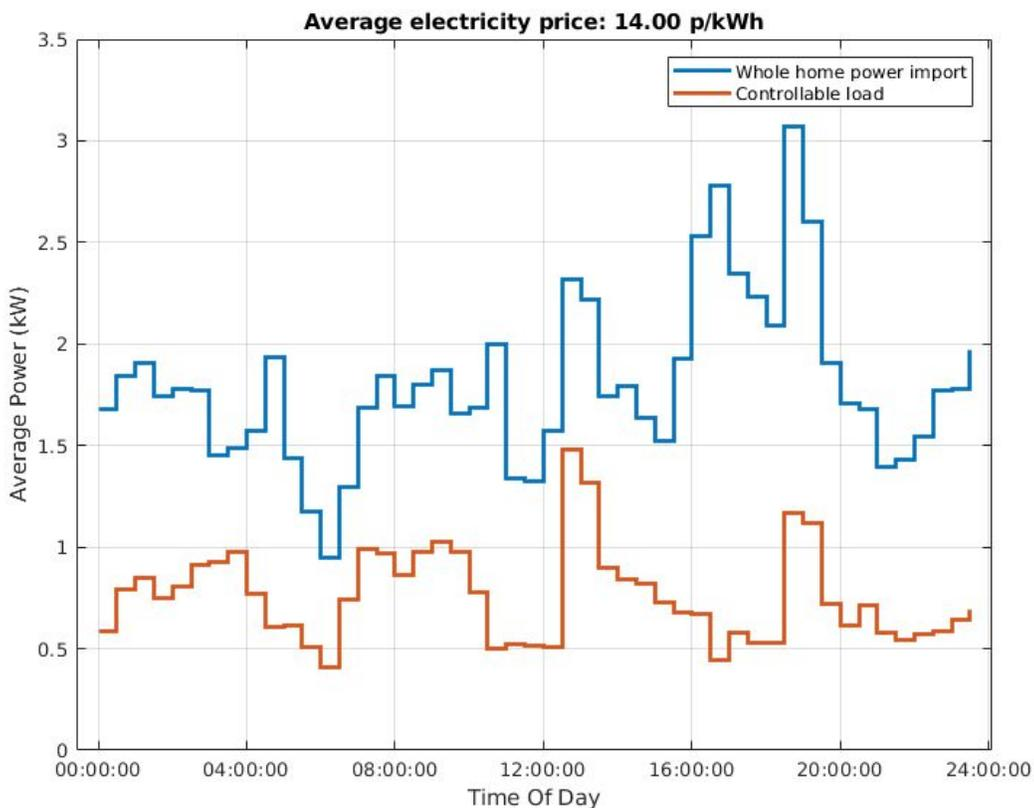
Figure 3.2 - Average load profiles for baseline operation on flat tariff (All homes, 09/12/2019 - 15/12/2019). Controllable load is just the heat pump in this case. Whole home power import = import from (/export to) the grid.
