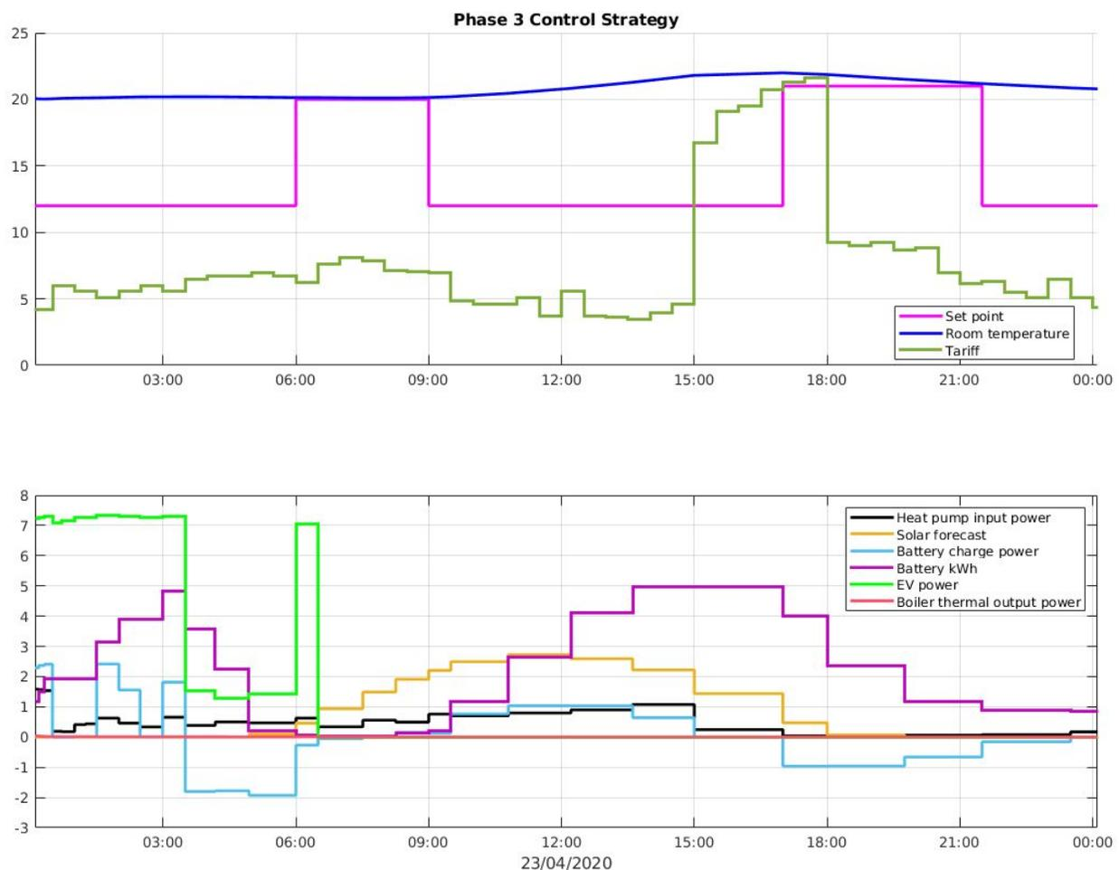
Figure 4.3 - Optimisation output under Phase 3 control (Digital twin of Home 5, 23/04/2020)
