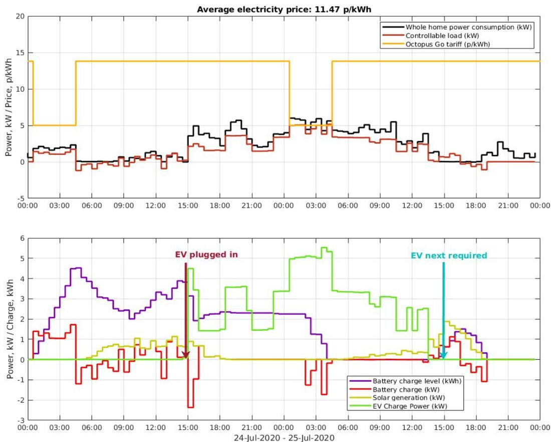
Figure 3.22 - Controlling load during cheap overnight tariff period on Octopus Go tariff (Home 04, 24/07/2020 - 25/07/2020). Here controllable load consists of heat pump, battery and EV power.
