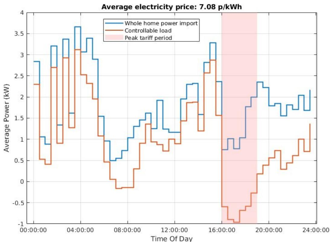
Figure 3.9 - Average load profiles for phase 2 operation on Octopus Agile tariff (All homes, 07/02/2020 - 13/02/2020). Controllable load is the combination of heat pump and battery in this case. Whole home power import = import from (/export to) the grid.
