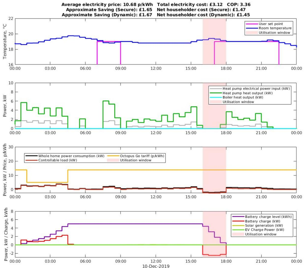
**Figure 9.6 - Full simulation run, 16:00 - 18:00 request utilised on the Octopus Go tariff (Digital twin of Home 2, 10/12/2019)**
