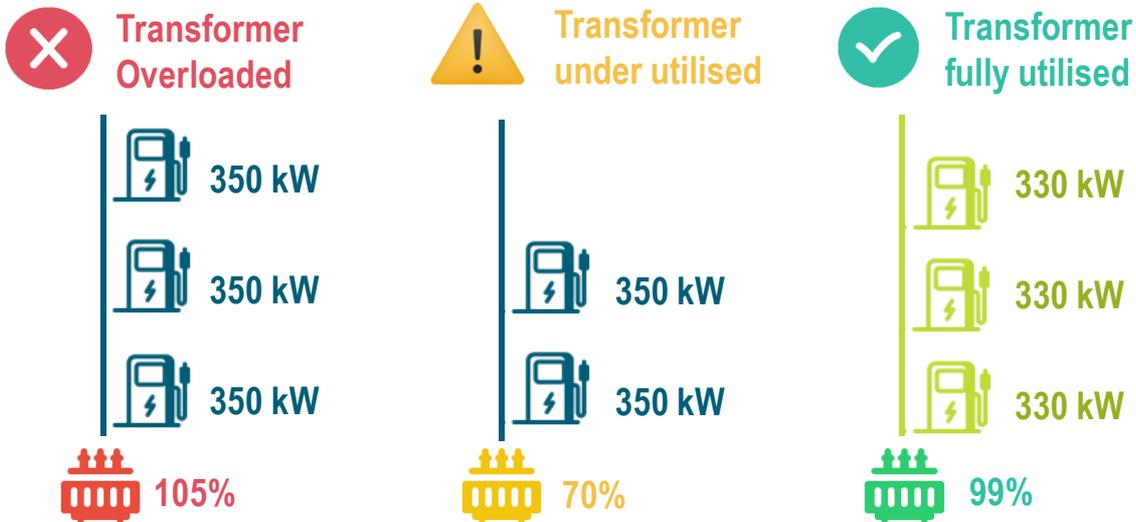
Figure 2-17 Illustration of different EV infrastructure arrangement
