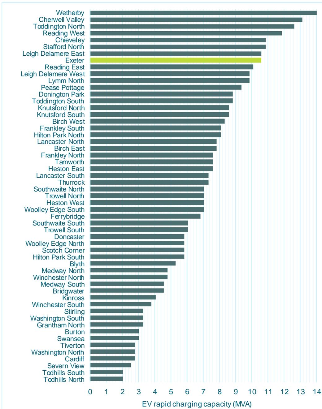
**Figure 3-18 7 MVA average EV rapid charging capacity pro-rated by footfall numbers**
