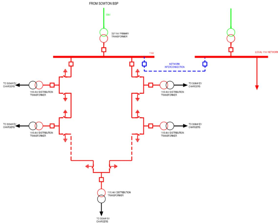
Figure 5-2 Example of network connection by single primary transformer and interconnection to local 11kV network for charging station
