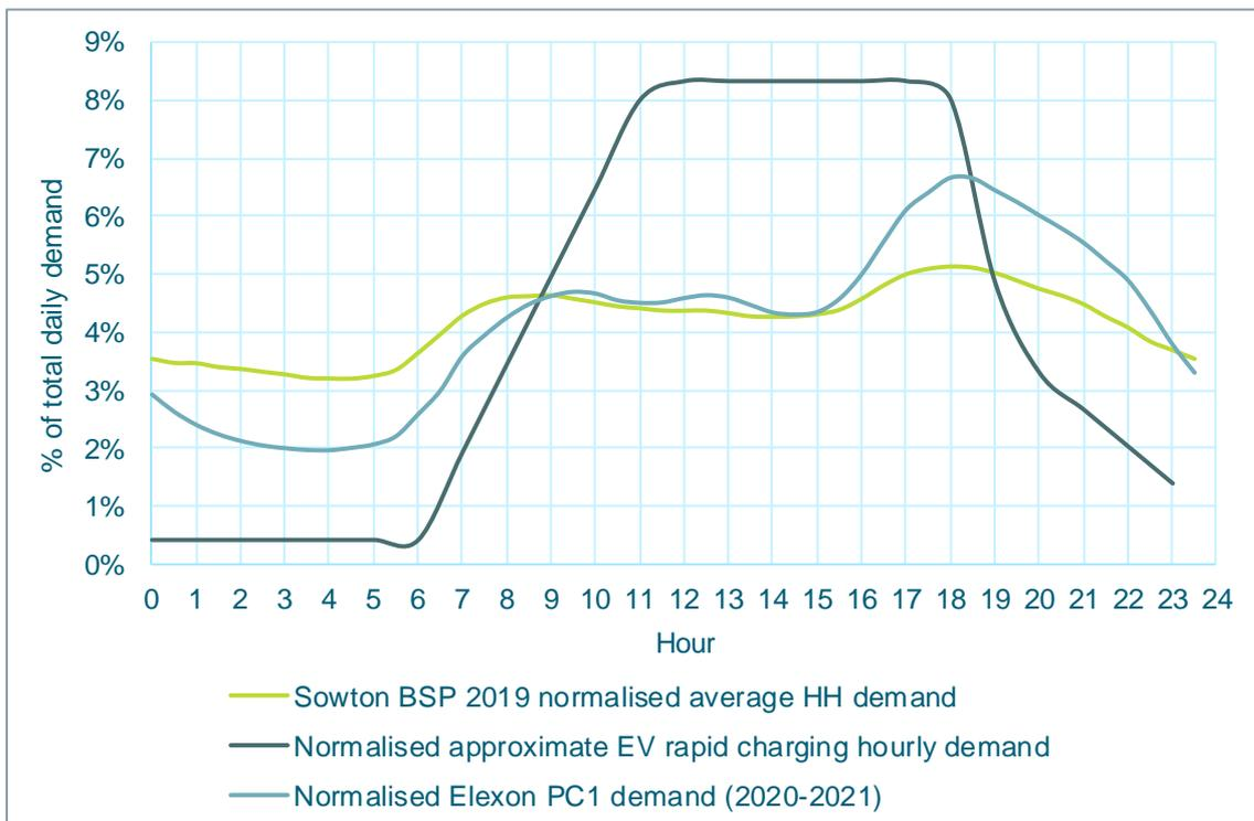
**Figure 3-13 Comparison of normalised approximate EV rapid charging profile with Sowton BSP 2019 average half-hourly demand and Elexon PC1 profile**
