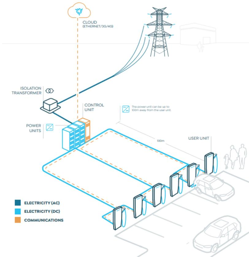
**Figure 2-16 Example of system components for installation of Veefil PK 350kW chargers.**
