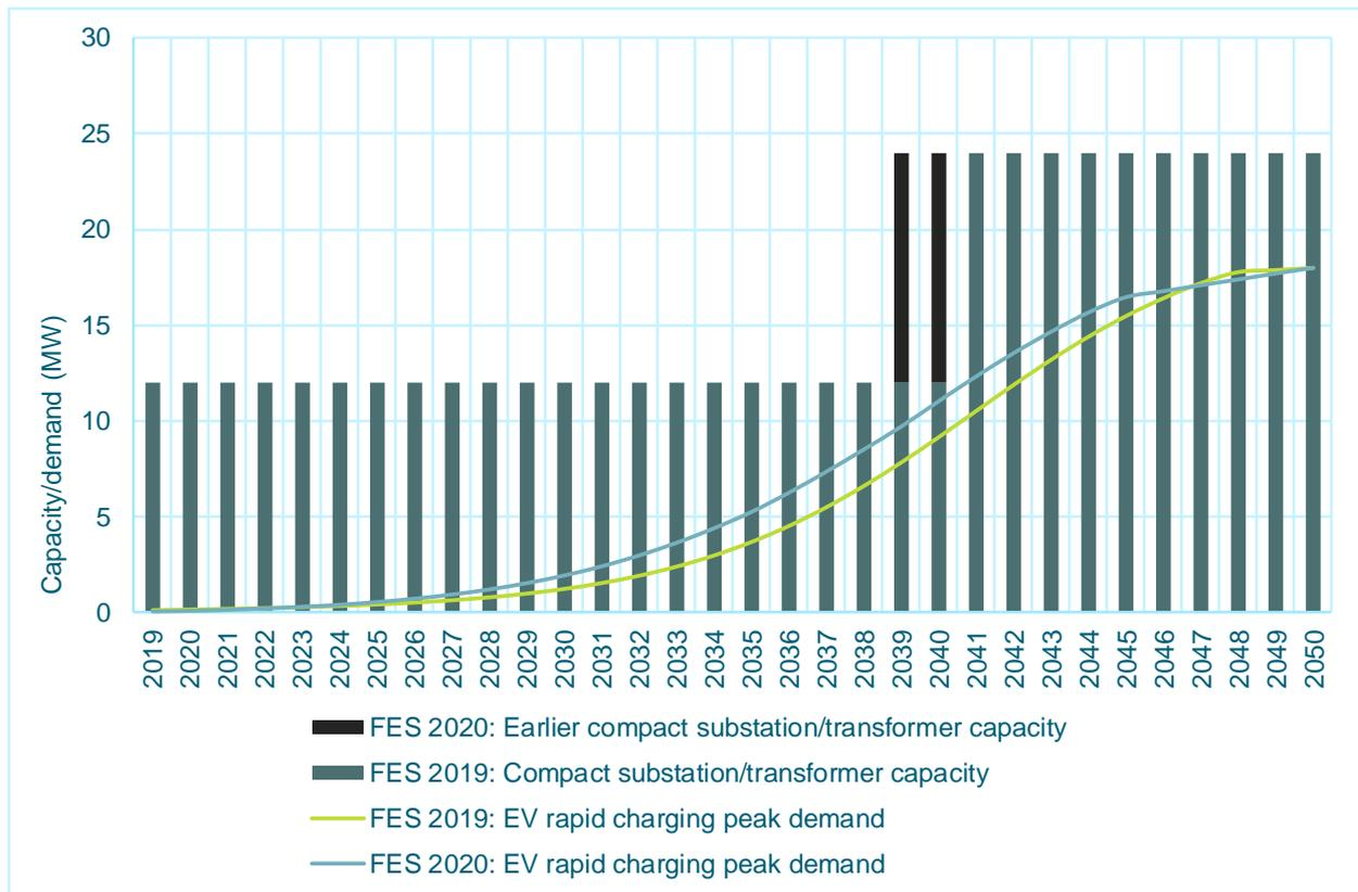
**Figure 3-19 Compact substation/transformer capacity requirement to meet demand calculated using approach 2**
