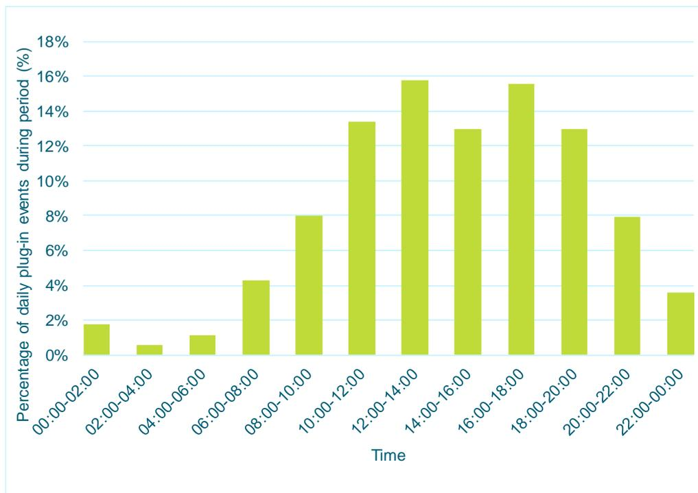
**Figure 2-9 Percentage of chargers within day using rapid chargers according to [17]**
