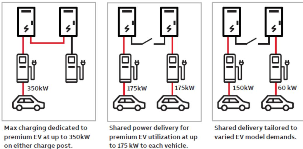
Figure 2-15 Dynamic DC power-sharing capabilities illustrated for ABB Terra HP 350kW charger [31]
