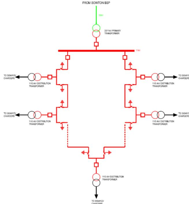
Figure 2-18 Example of network connection diagram for EV charging station
