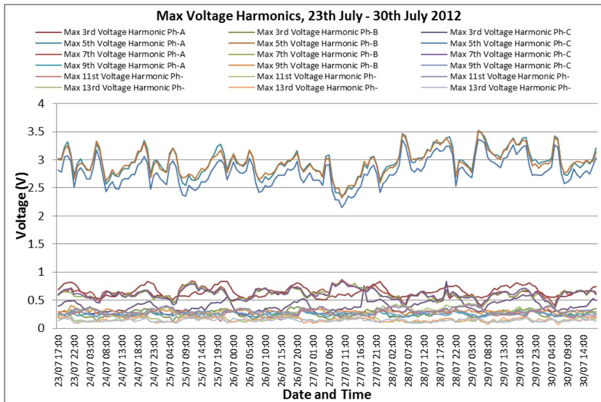
Figure 17 – 3<sup>rd</sup>- 13<sup>th</sup> maximum voltage harmonics
