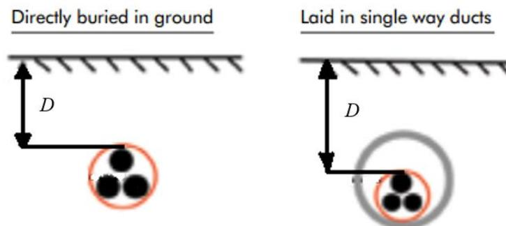
Figure 5.6: Schematic of depth of cover (D)
