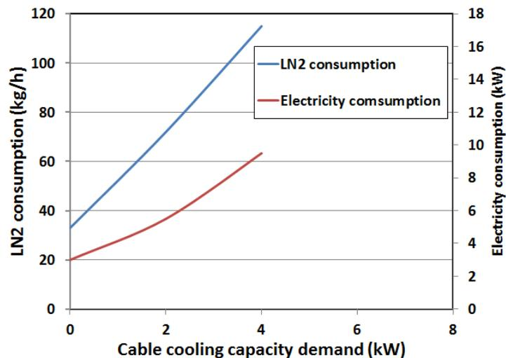
Figure 4.19: Liquid nitrogen (LN2) and electricity consumption of a completed 1 km superconducting cable system [47]
