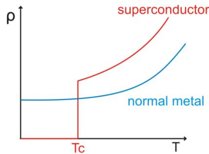
Figure 3.1: Critical temperature ( $T_c$ ) of superconductor compared to normal metal
