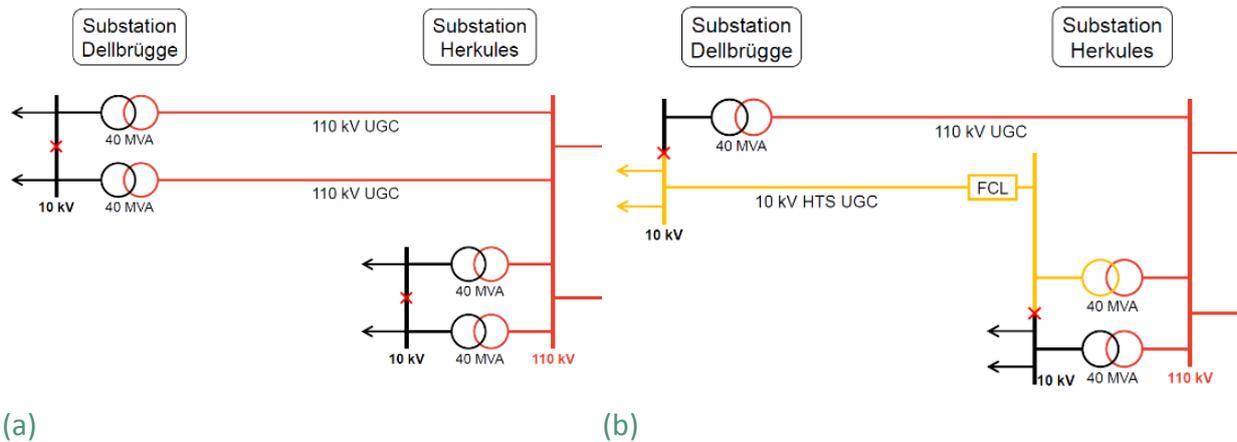
Figure 3.5: AmpaCity grid configuration (a) installation of conventional cable solution, (b) alternative installation of superconducting cable solution [16]
