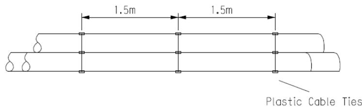
Figure 5.5: 33, 66 and 132 kV cables laid in trefoil configuration and tied at 1.5 m interval
