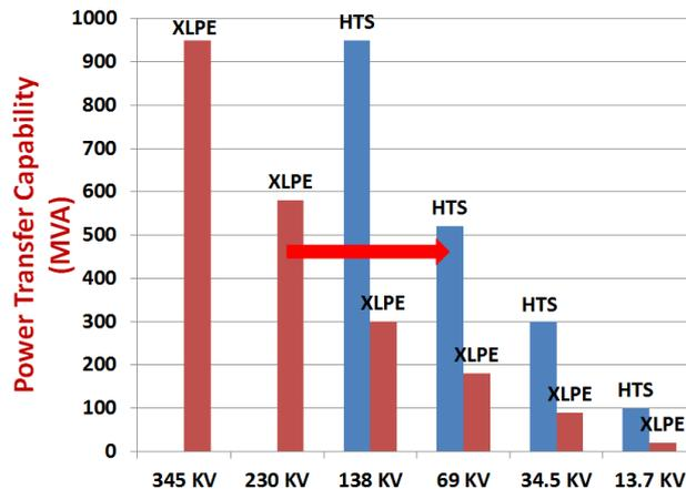
Figure 3.2: The power transmission capacity and voltage level of XLPE cable and superconducting cable. [10]
