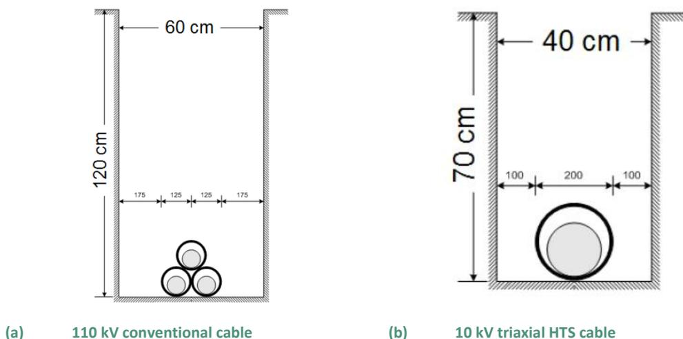
Figure 4.11: Dimensions of the trench for 110 kV conventional cable and 10 kV triaxial HTS cable [16]
