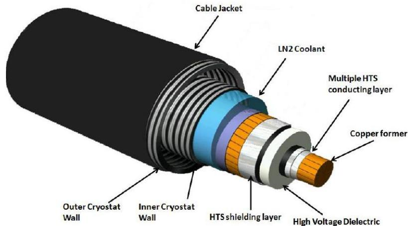
Figure 4.1: Single-phase superconducting cable. [4]
