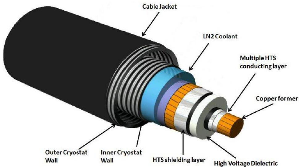
Figure 4.2 : Single-phase superconducting cable
