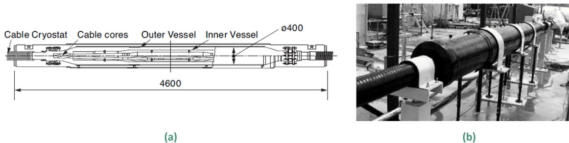
Figure 4.14: (a) Schematic view of "3-in-one" HTS joint. (b) Appearance of "3-in-one" HTS joint. [24]
