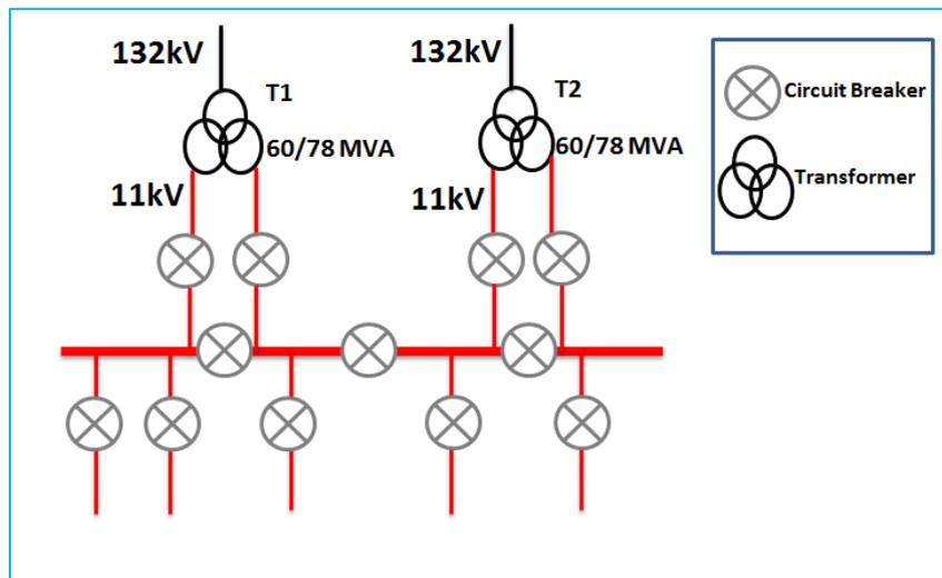
Figure 2.1 - Example 132/11kV substation
