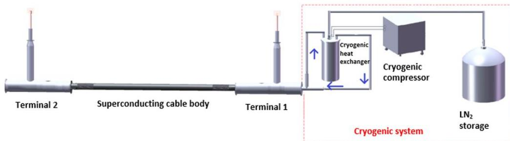
Figure 4.16: Schematic of superconducting cable cryogenic cooling system [32]
