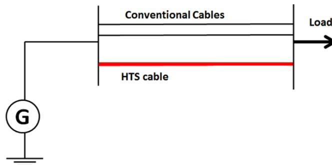
Figure 3.4: Conventional cables and superconducting cables working in parallel
