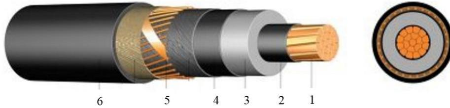
Figure 5.1: Configuration of XLPE/EPR cable
