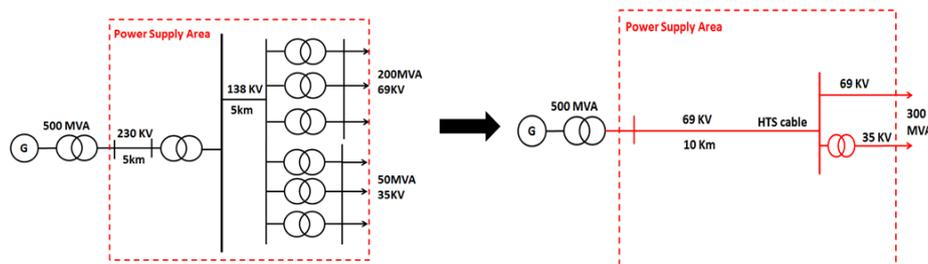
Figure 3.3: The simplified power network replaced by superconducting cable.
