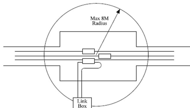
Figure 5.4: Schematic of cross bonding link boxes [39]
