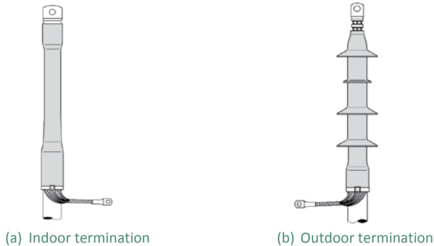
Figure 5.2: Schematic of indoor and outdoor terminations
