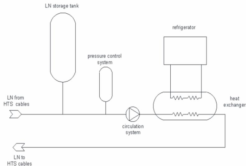
Figure 4.8: Structure of completed cryogenic cooling system.
