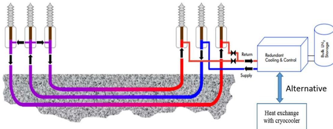
Figure 4.7: The self-circulating cooling system for superconducting cable. [7]
