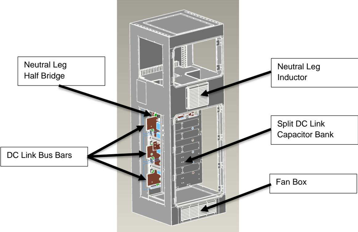
Complete GTI System View with Front Covers Fitted
