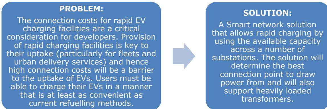
The Project will use an equalisation network to provide an alternative, cost-effective solution for rapid EV charging demands, more flexibly than a traditional AC reinforcement solution. The solution seeks to explore the comparative benefits of a DC network, where power flows can be actively managed, and fault level contained, over a traditional AC network reinforcement.
