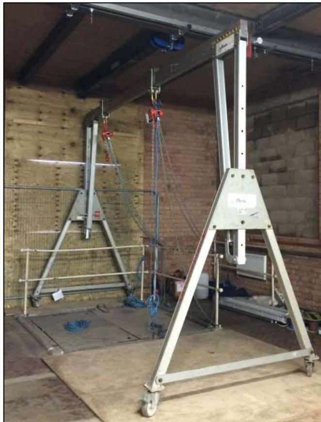
Figure 2-10: Portable lifting frame used to lift the cryostat vessels to the first floor
