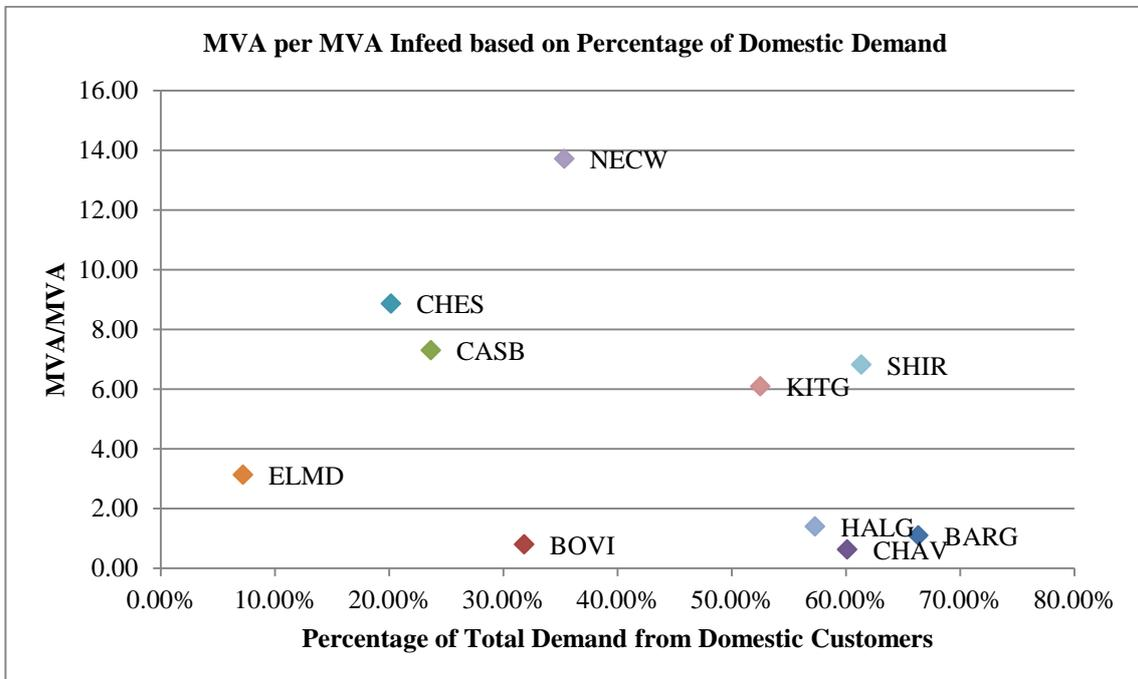
Figure 2-3: MVA per MVA Load Infeed based on % Domestic Demand at each Substation
