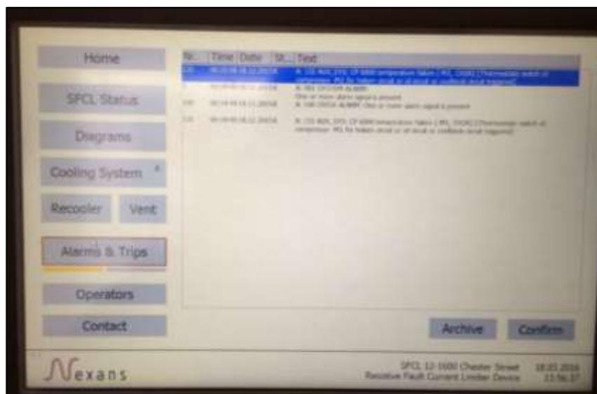
Figure 2-6 - Screenshot from FCL HMI showing cooling system alarms
