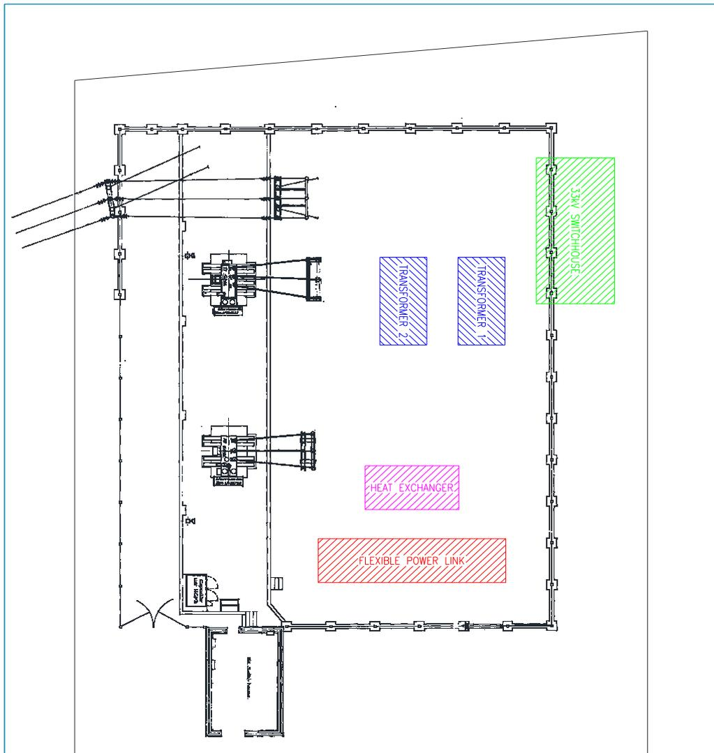
Figure 4-2: Proposed FPL and 33kV Switchhouse Layout at Exebridge
