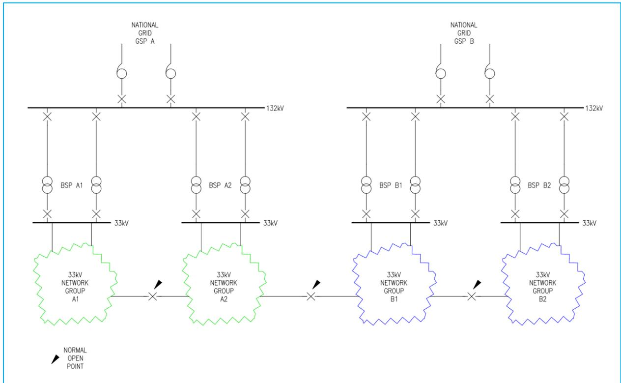
**Figure 1-1: Typical Arrangement of a DNO Network**
