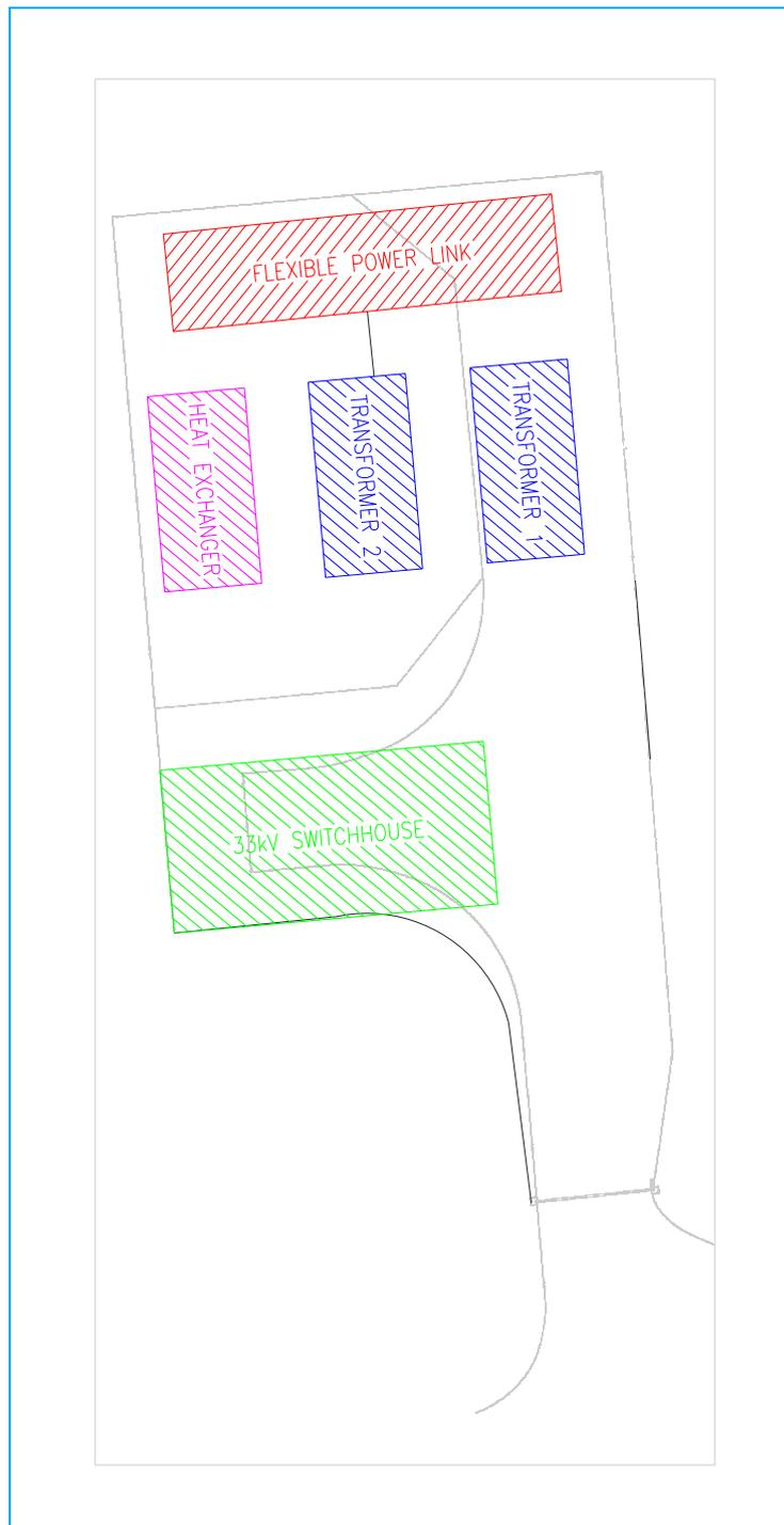
Figure 4-2: Proposed FPL and 33kV Switchhouse Layout at Winslakefoot
