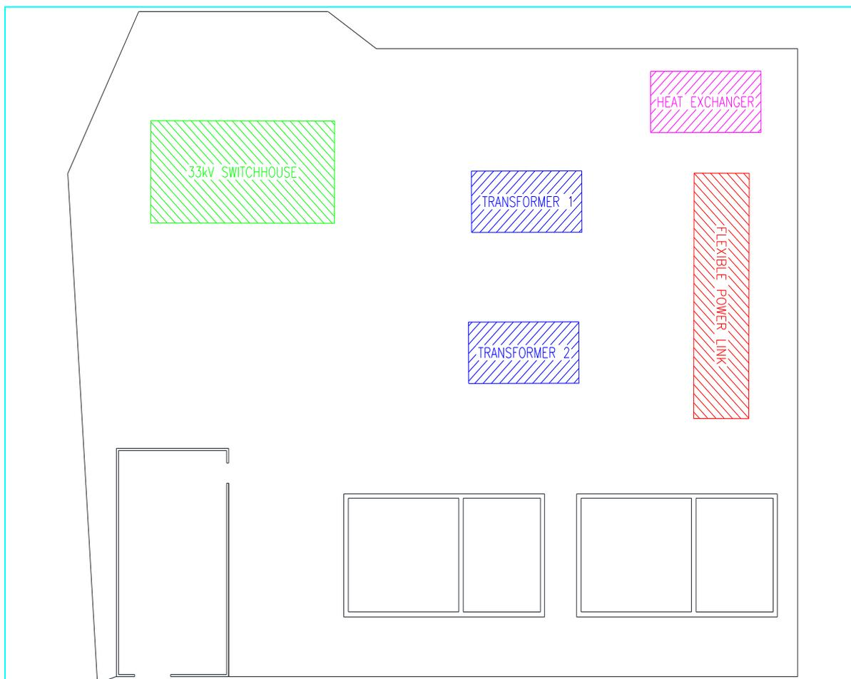
Figure 4-2: Proposed FPL and 33kV Switchhouse Layout at Tiverton Moorhayes
