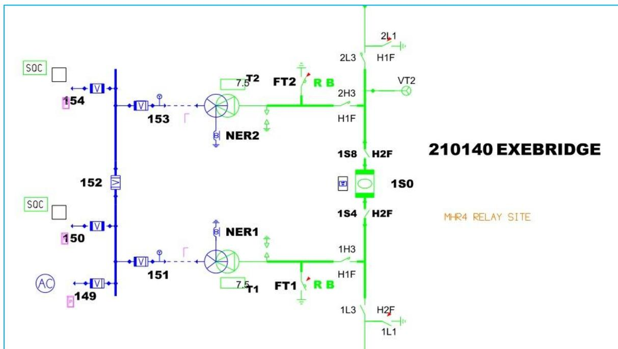
Figure 2-1: Existing Single Line Diagram for Exebridge
