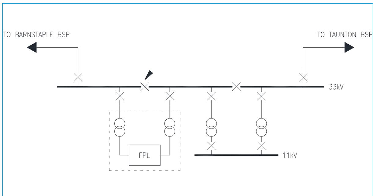
**Figure 4-1: Proposed Exebridge 33/11kV Single Line Diagram Following the FPL Installation**
