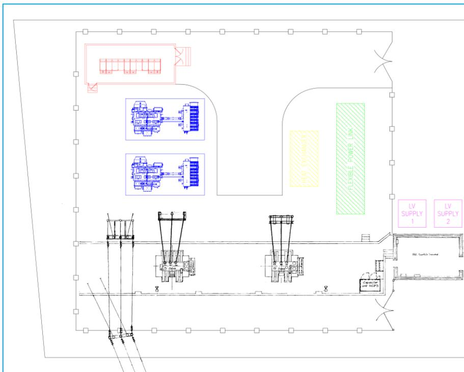
**Figure 6-5: Proposed FPL and Switch House Layout for Exebridge**
