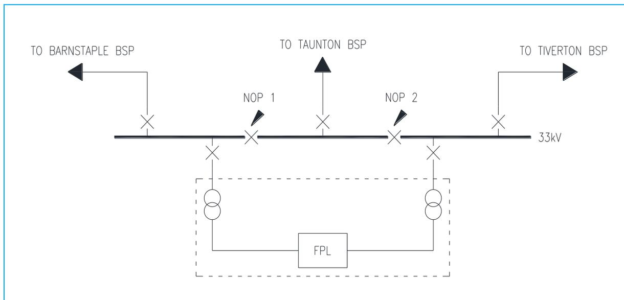
**Figure 4-1: Proposed Quartley Single Line Diagram following the FPL Installation**
