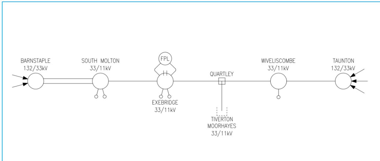
**Figure 6-1: Overview of 33kV Network at Exebridge**
