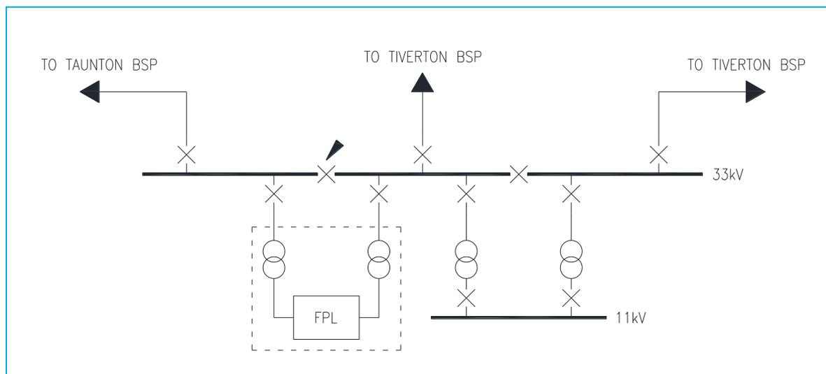
Figure 4-1: Proposed Tiverton Moorhayes Single Line Diagram following the FPL Installation
