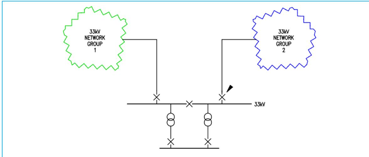
Figure 3-1: Option 1 - Existing Network Arrangement
