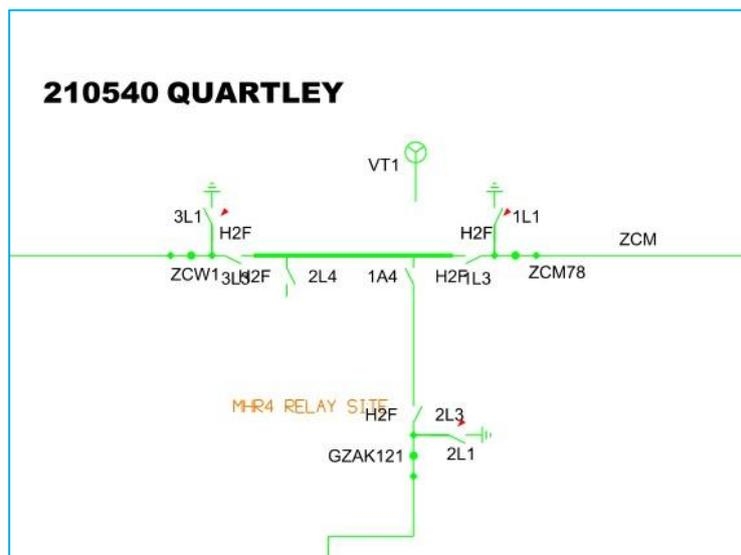
Figure 2-1: Existing Single Line Diagram for Quartley
