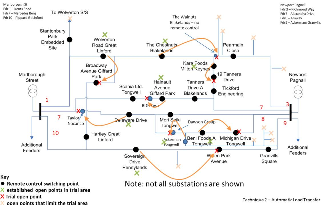
Figure 12: Stylised network diagram showing changes for 17-24 Jun - Configuration 2
