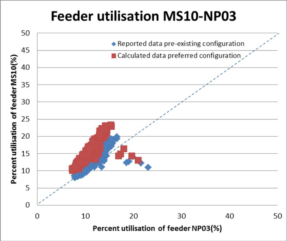
Figure 67 : Measured and estimated feeder utilisation of MS10 and NP03 over week 1
