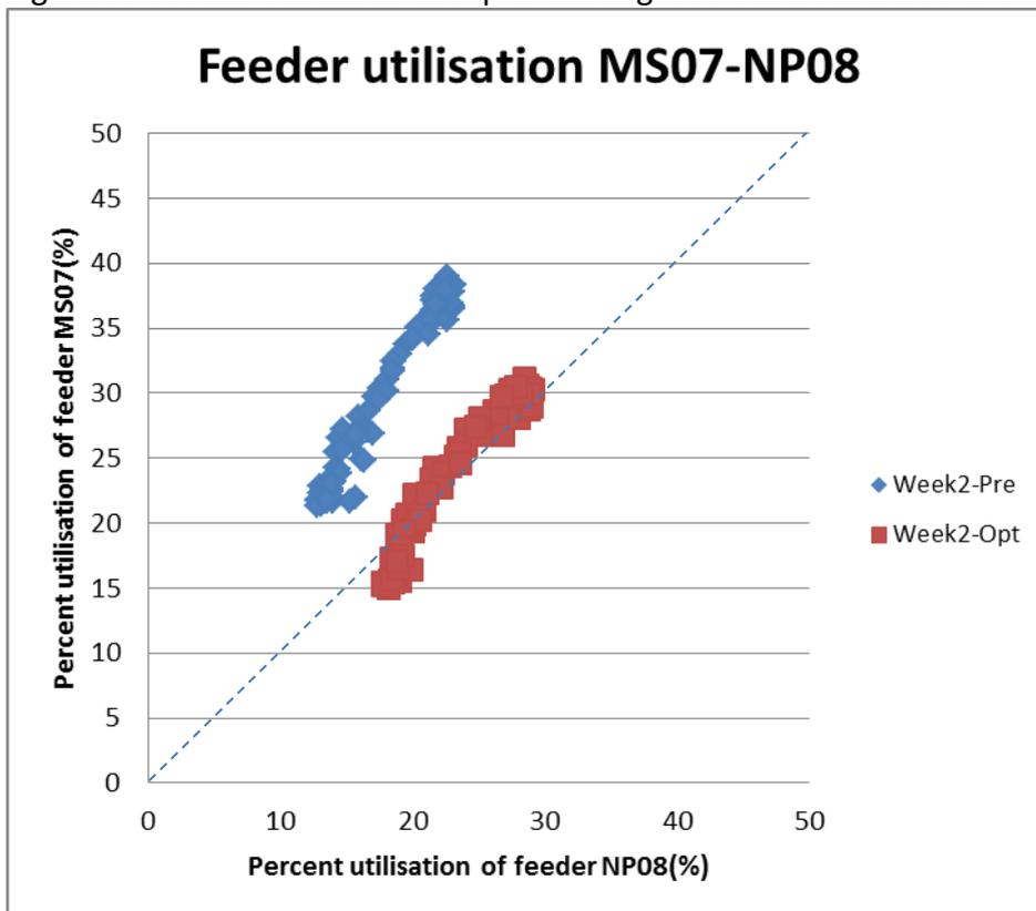
Figure 34 Feeder utilisation with optimised NOP between MS07 and NP08
