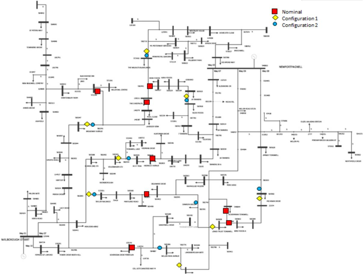
*Cable Trial Network showing location of calculated open points*
