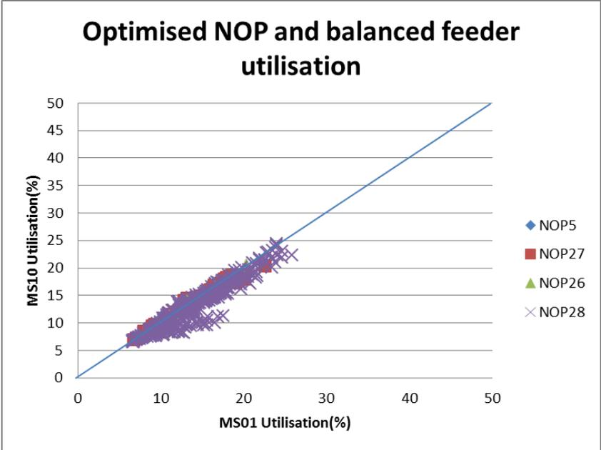
Figure 48: Feeder utilisation with optimised NOP between MS10 and MS01 (No.5 Wolverton Rd)
