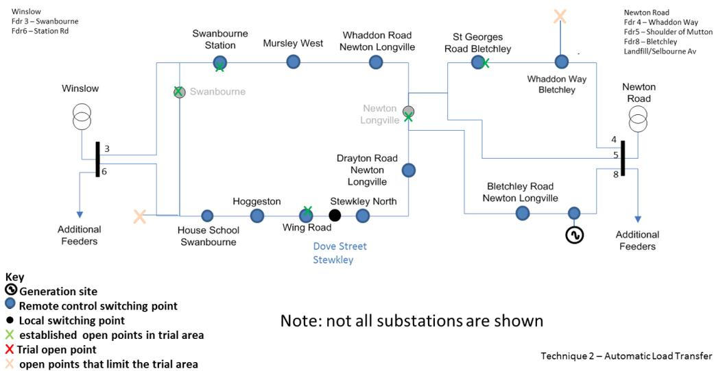
Figure 2: Stylised representation of the ALT overhead trial network
