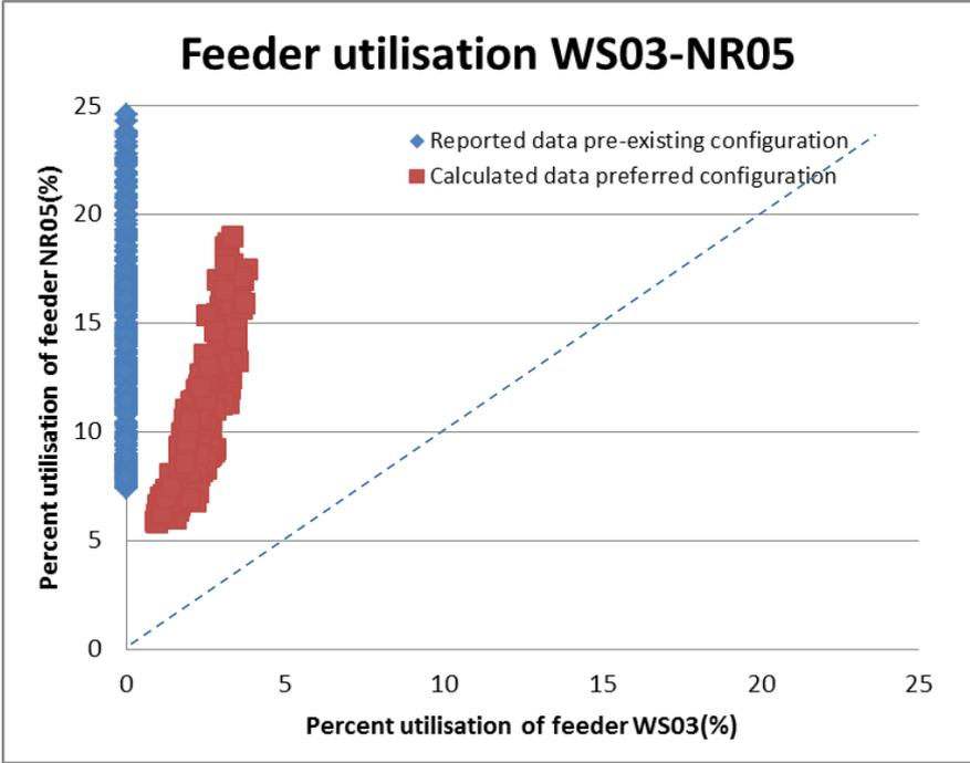
Figure 53: Measured and estimated feeder utilisation of WS03 and NR05 over week 1
