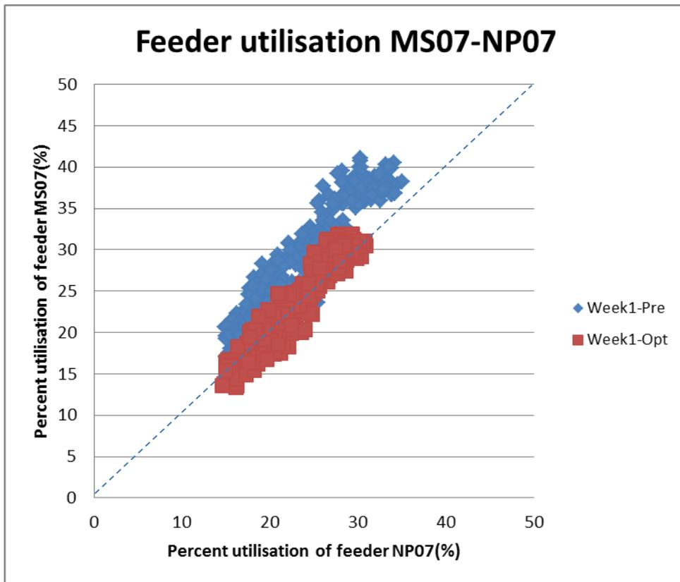
Figure 95 : Feeder utilisation with pre-existing NOP between MS07 and NP07
