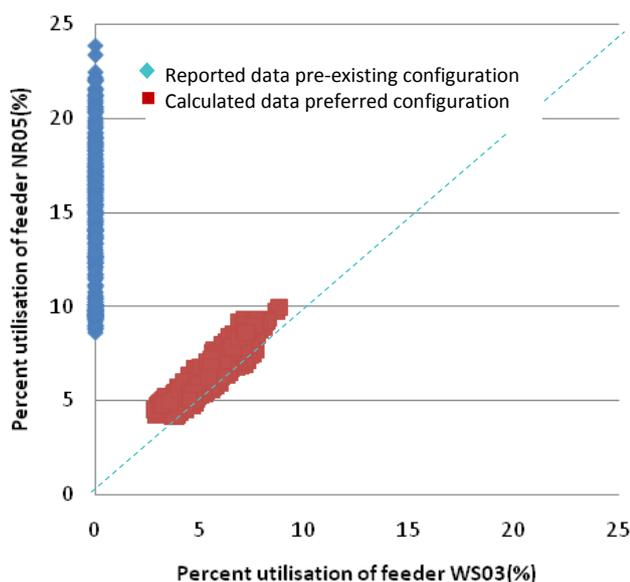
Figure 29: Feeder utilisation for week 1 (WS03/NR05)
