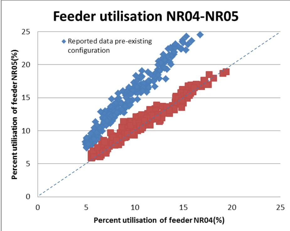
Figure 61 : Measured and estimated feeder utilisation of NR04 and NR05 over week 1
