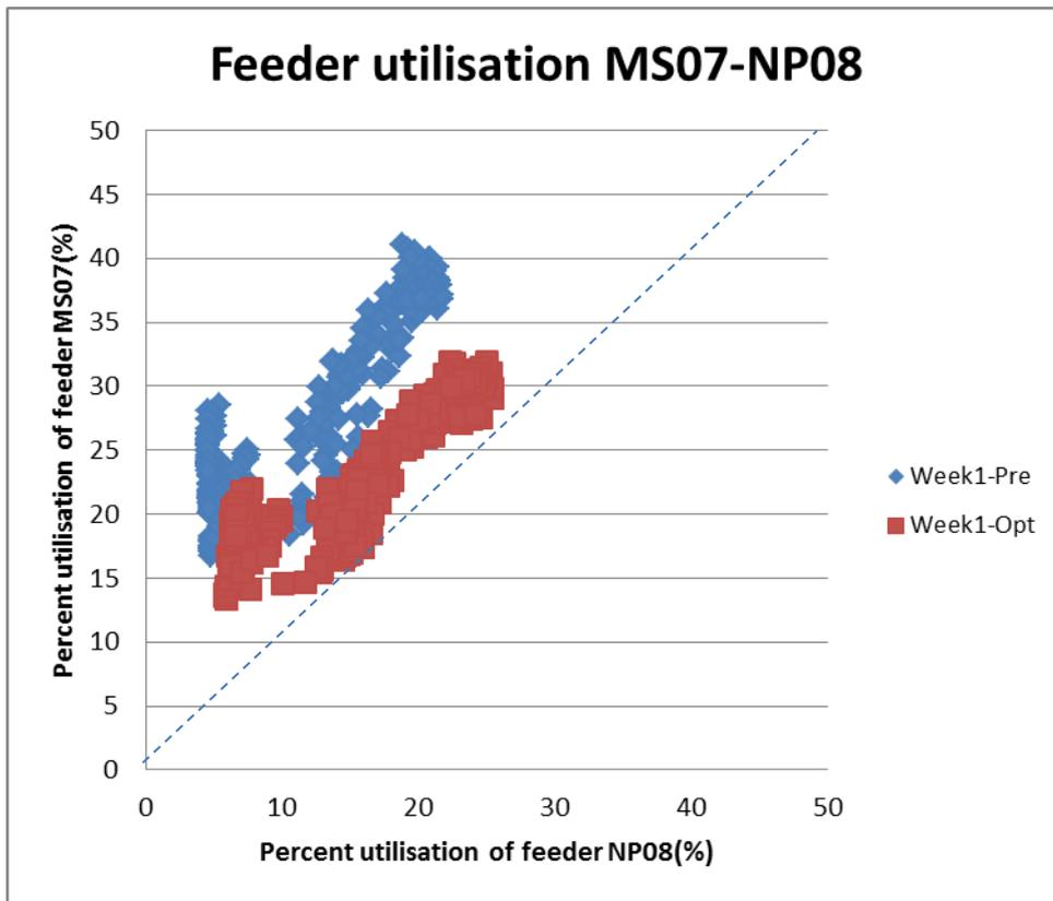
Figure 33 Feeder utilisation with pre-existing NOP between MS07 and NP08
