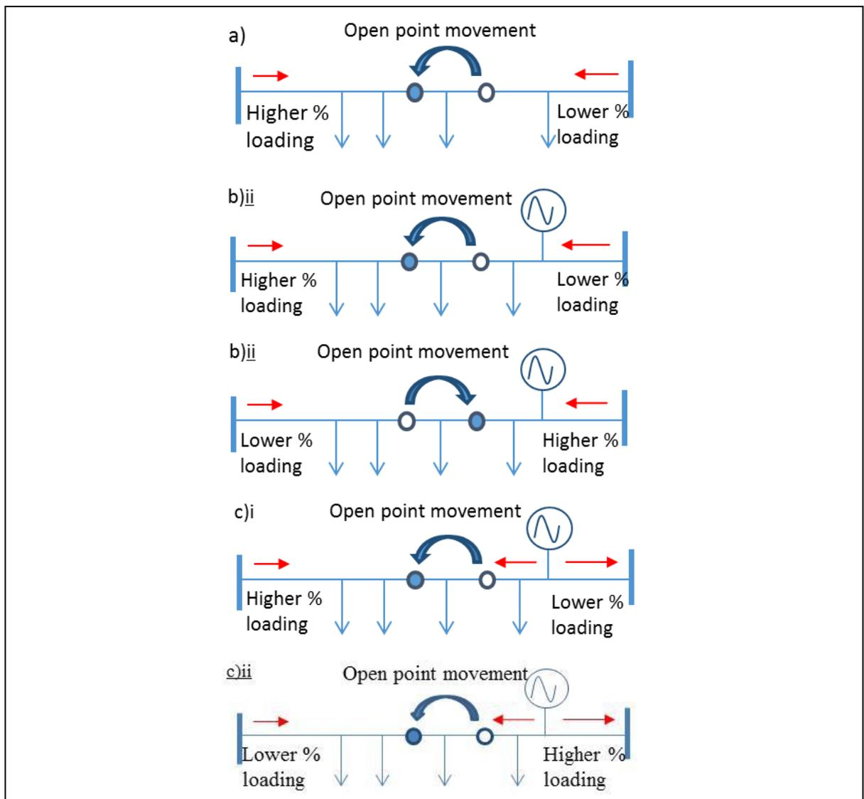
Figure 8 : NOP movement to balance feeder utilisation in the presence of a) load only, b) load and low value generation and c) load and high value generation.
