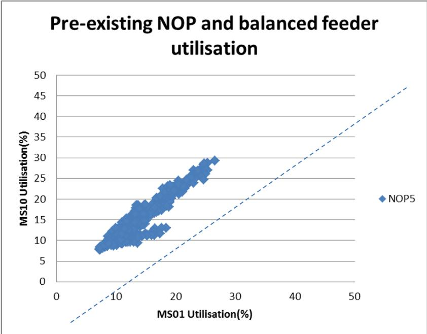
Figure 47: Feeder utilisation with pre-existing NOP between MS10 and MS01 (No.5 Wolverton Rd)
