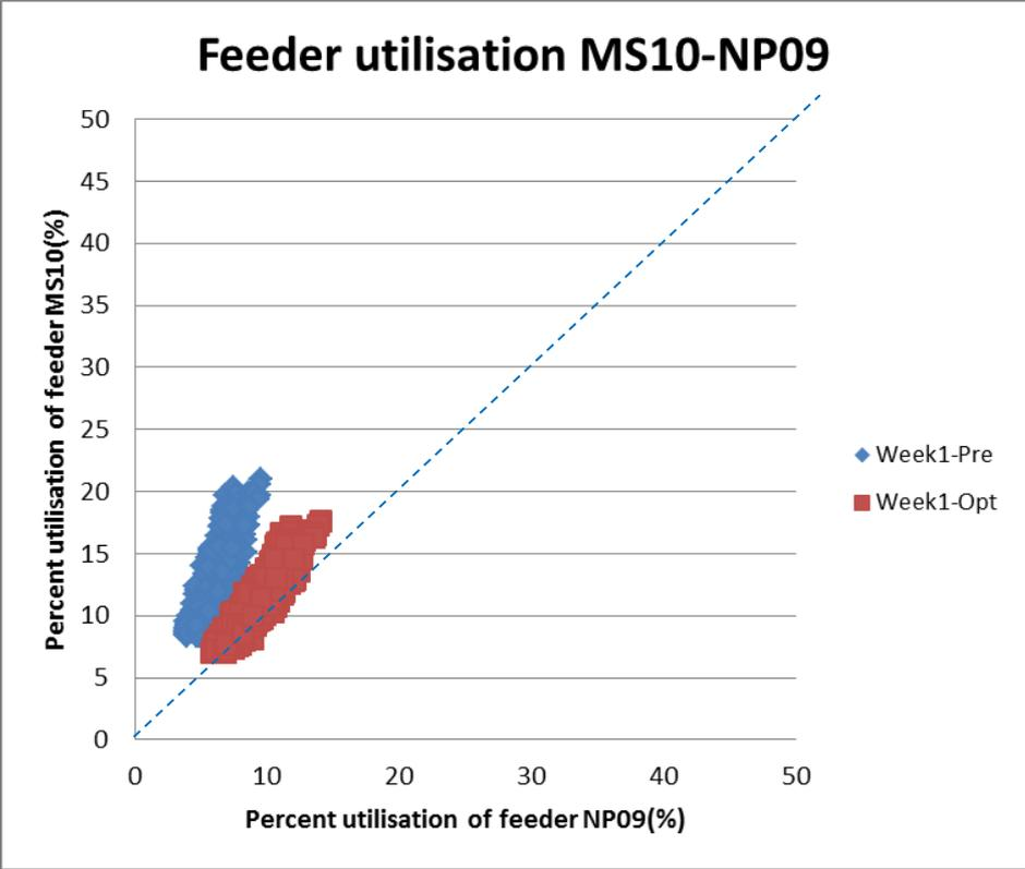
Figure 87 : Feeder utilisation with pre-existing NOP between MS10 and NP09
