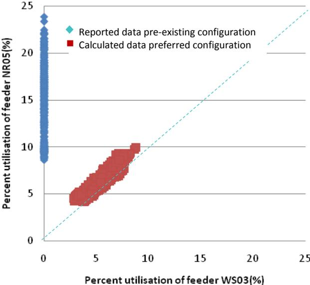
Figure 75: Feeder utilisation for week 1 (WS03/NR05)
