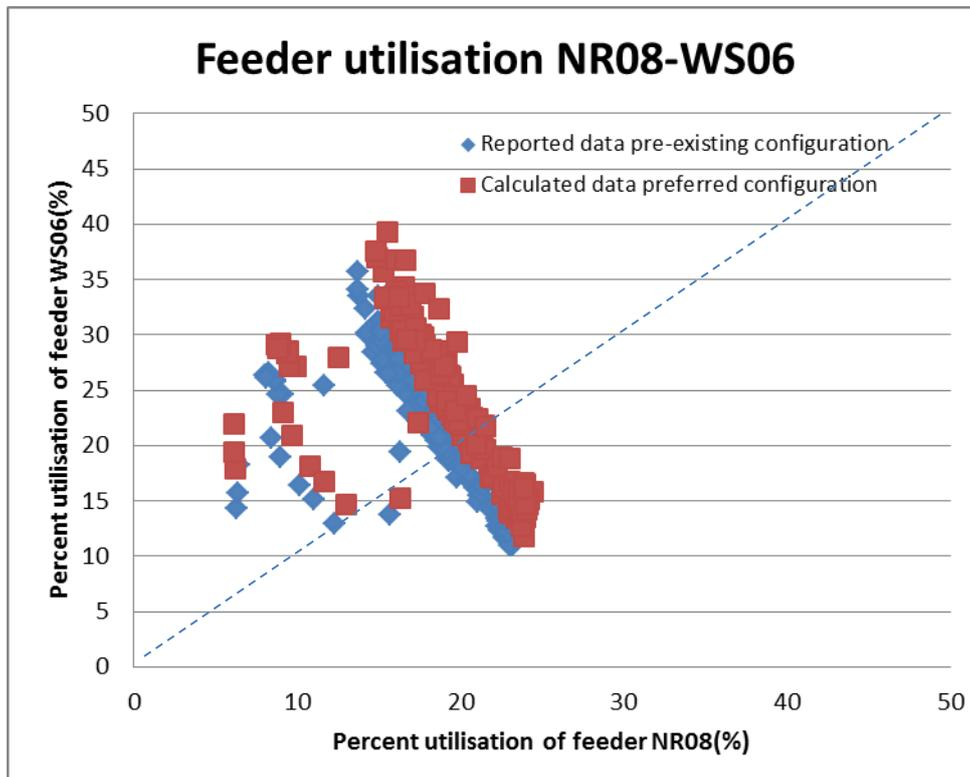
Figure 55: Measured and estimated feeder utilisation of WS06 and NR08 over week 1
