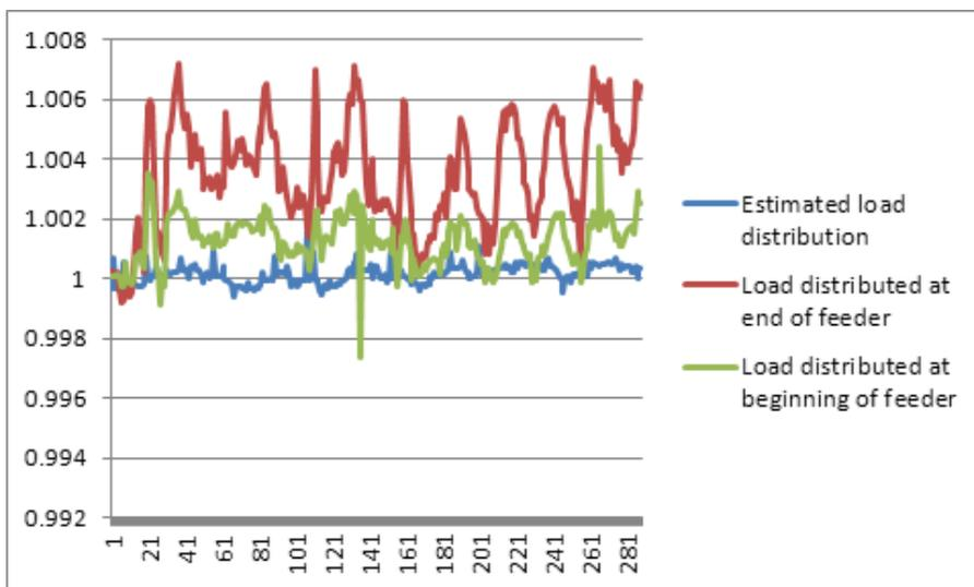
Figure 40 :Cable Network ratio  $(\text{Ref}\#1/\text{Ref}\#4)/(\text{Ref}\#2/\text{Ref}\#3)$  for each half hour slot over trial period
