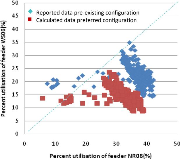
Figure 77: Feeder utilisation for week 1 (NR08/WS06)
