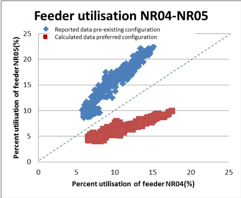
Figure 83 : Measured and estimated feeder utilisation of NR04 and NR05 over week 1
