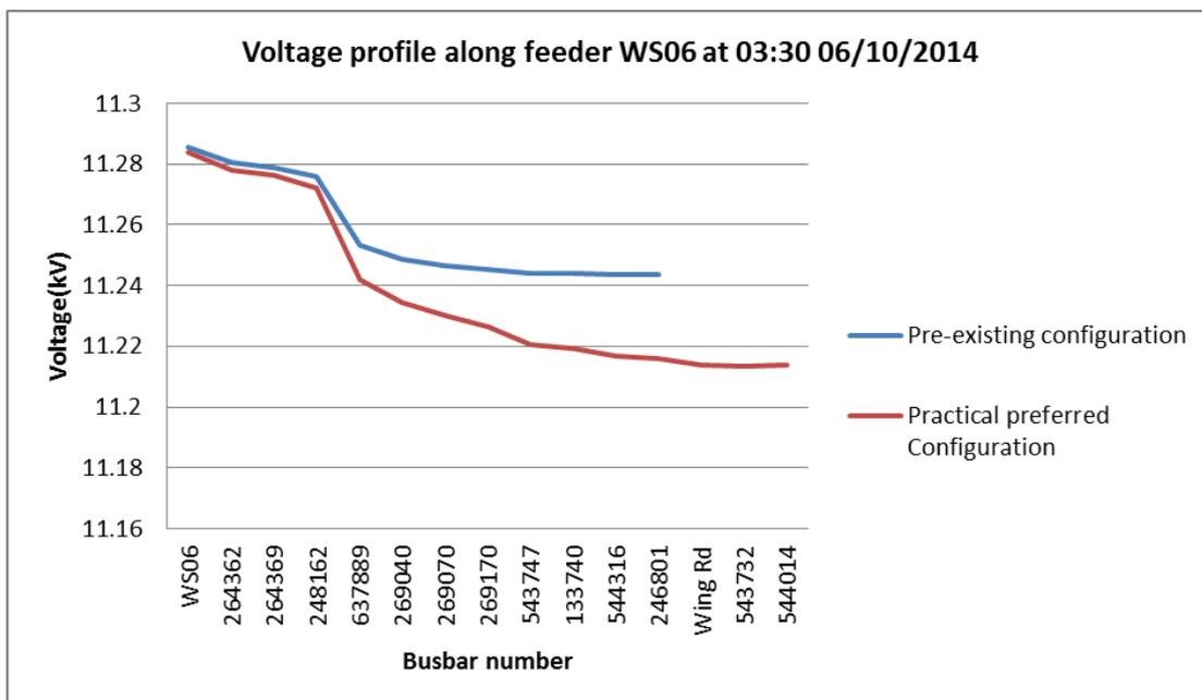
Figure 36 : Voltage profile along Winslow feeder 6 showing changes to voltage as the feeder is re-configured under method 1
