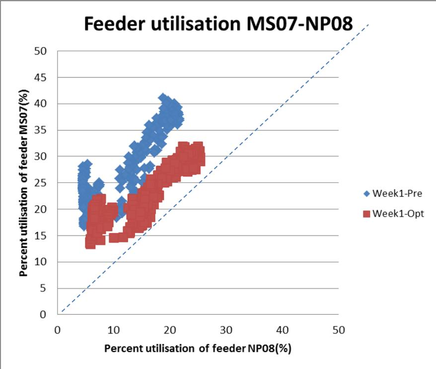
Figure 85 : Feeder utilisation with pre-existing NOP between MS07 and NP08
