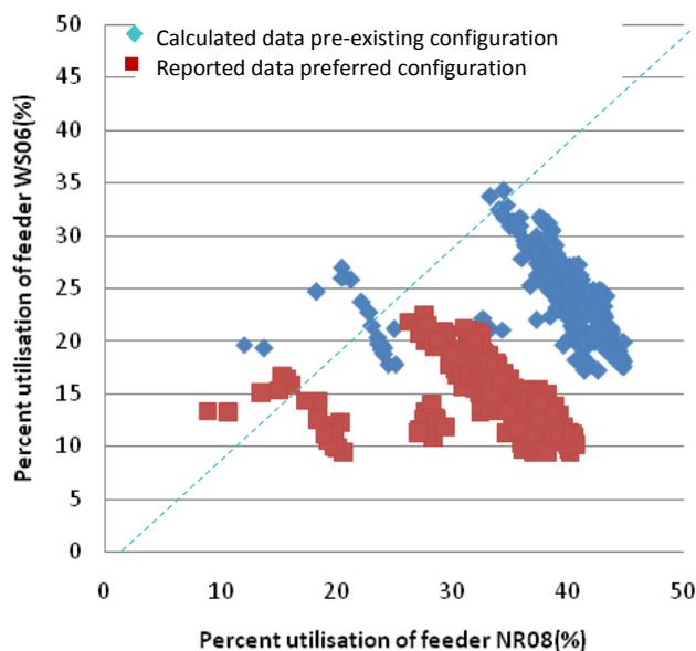
Figure 32: Feeder utilisation for week 2 (NR08/WS06)
