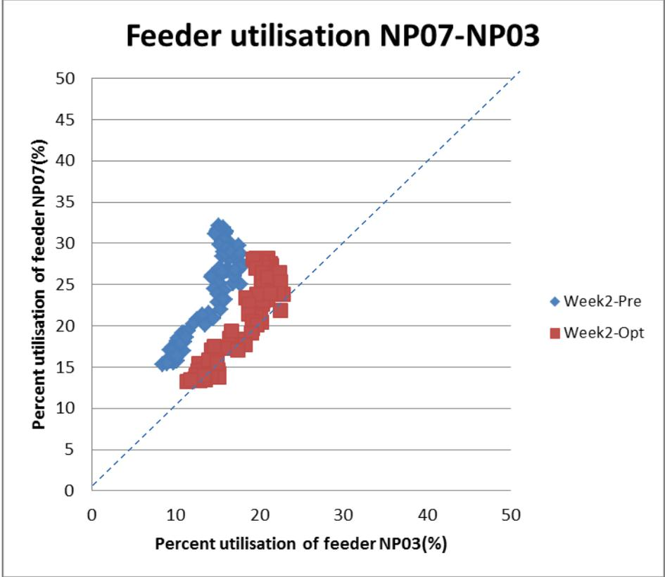
Figure 92 : Feeder customer utilisation with optimised NOP between NP07 and NP03
