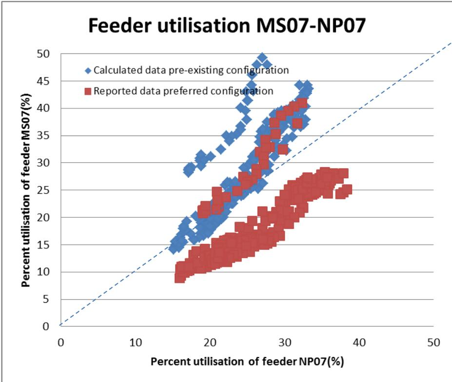
Figure 74 : Measured and estimated feeder utilisation of MS07 and NP07 over week 2
