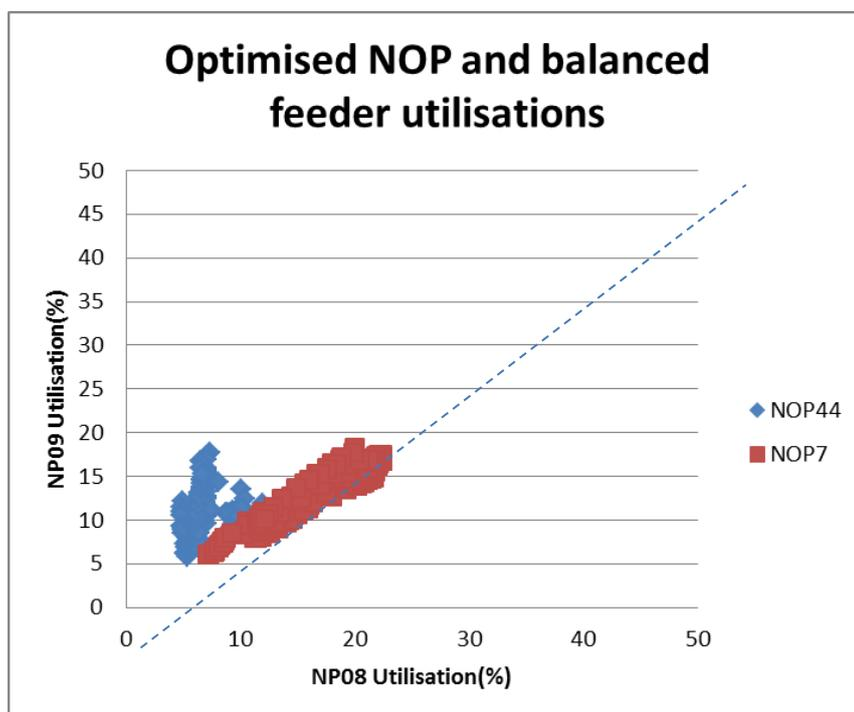
Figure 52: Feeder utilisation with optimised NOP between NP09 and NP08 (No. 7 Ackerman)
