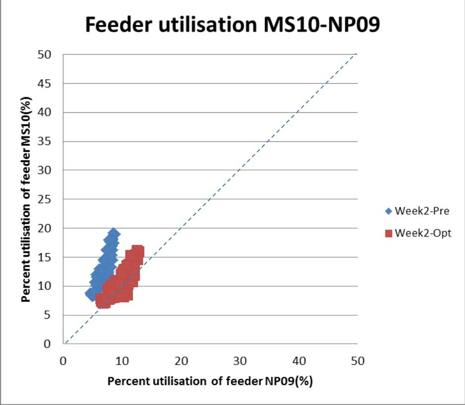
Figure 88 : Feeder utilisation with optimised NOP between MS10 and NP09
