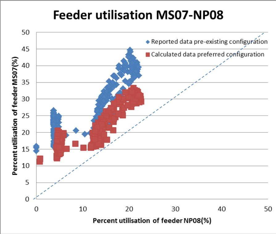
Figure 63: Measured and estimated feeder utilisation of MS07 and NP08 over week 1
