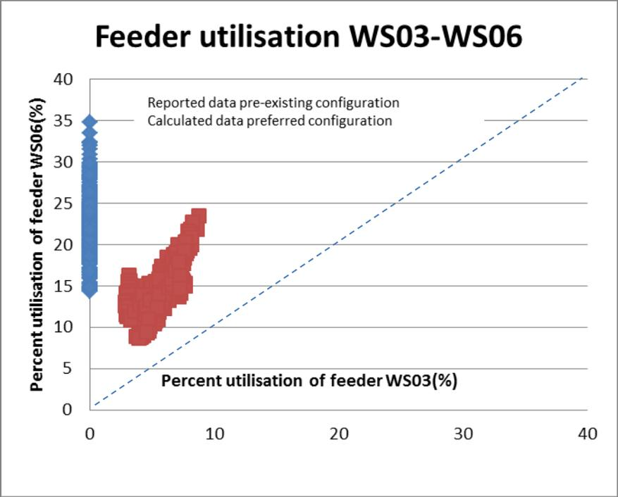
Figure 79 : Measured and estimated feeder utilisation of WS03 and WS06 over week 1
