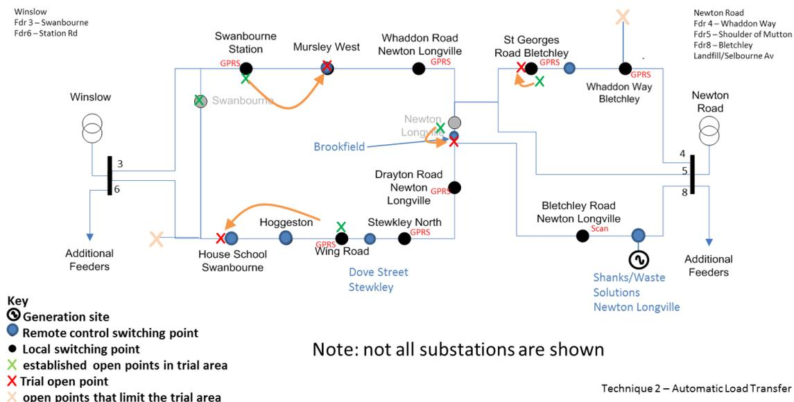
Figure 21: Stylised network diagram showing changes for network test starting 02/06/2015
