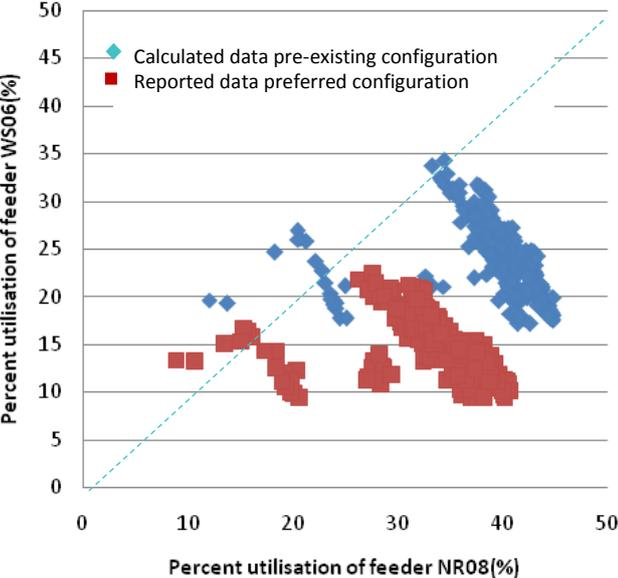
Figure 78: Feeder utilisation for week 2 (NR08/WS06)
