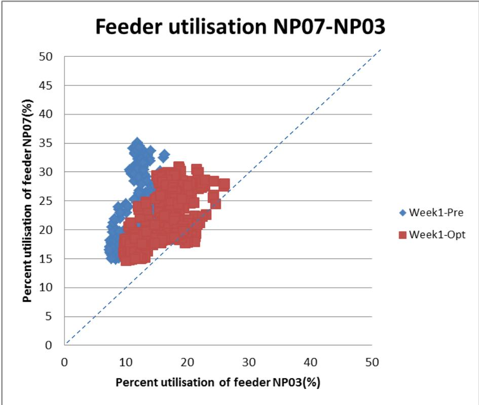
Figure 91 : Feeder utilisation with pre-existing NOP between NP07 and NP03
