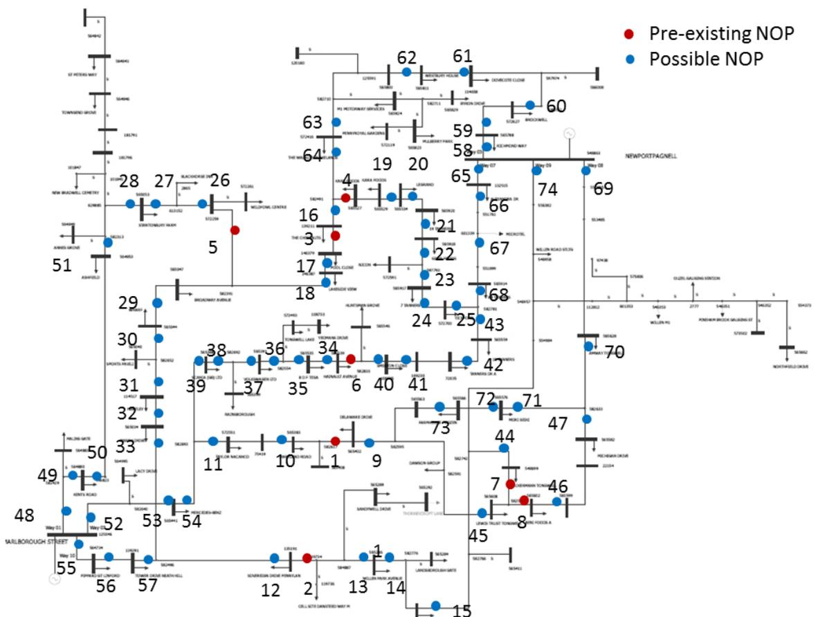
Figure 22: Illustration of possible NOP location for feeder utilisation balance on Cable trial network
