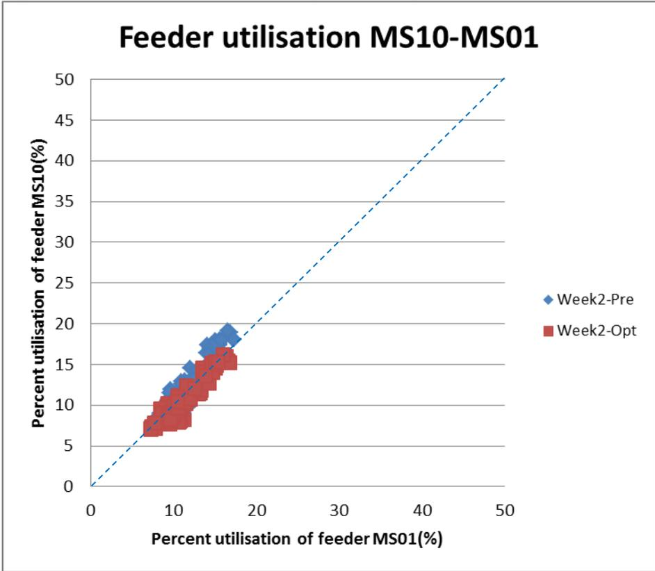
Figure 94 : Feeder customer utilisation with optimised NOP between MS10 and MS01
