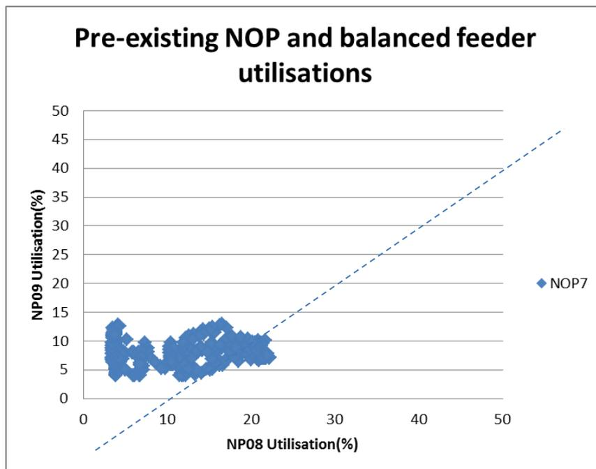
Figure 51: Feeder utilisation with pre-existing NOP between NP09 and NP08 (No. 7 Ackerman)
