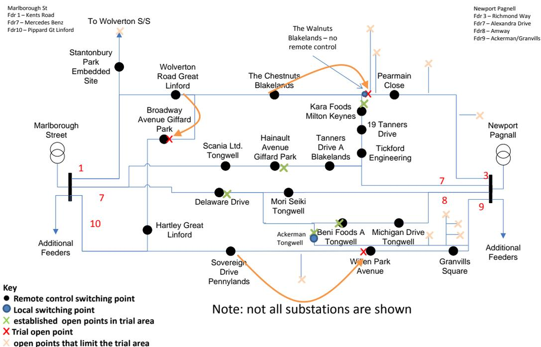
Figure 10 : Stylised network diagram showing changes for 22-29 May – initial test configuration
