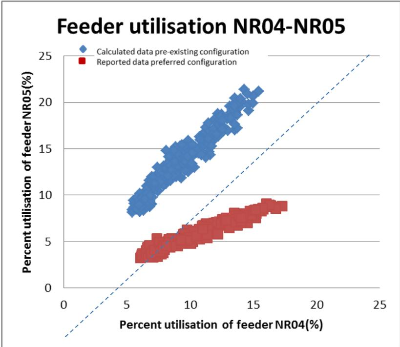
Figure 84 : Measured and estimated feeder utilisation of NR04 and NR05 over week 2
