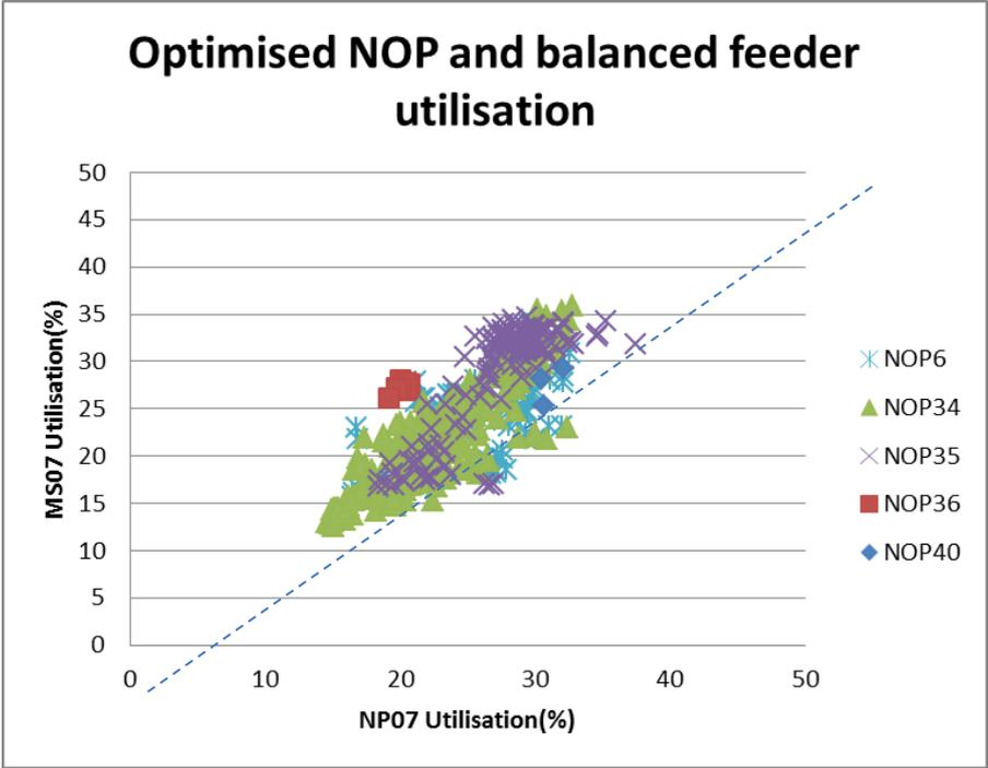
Figure 50 Feeder utilisation with optimised NOP between MS07 and NP07 (No. Hainault)
