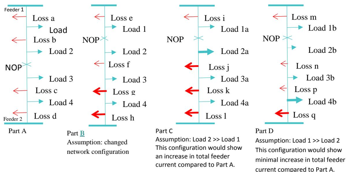
**Figure 43 :** Example showing how results from a poorly conditioned model would be picked up.
