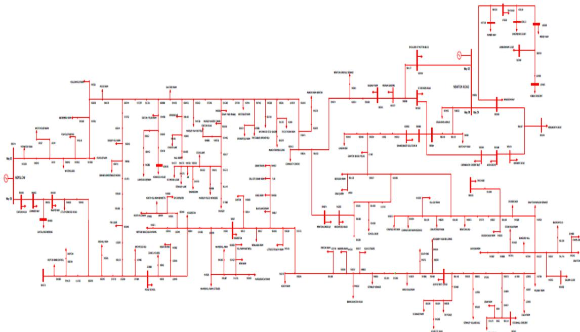
**Figure 7: IPSA model for the Newport Pagnell and Marlborough Street substations**
