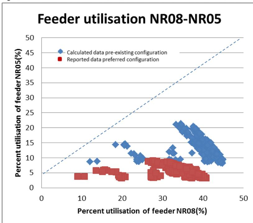
Figure 82 : Measured and estimated feeder utilisation of NR08 and NR05 over week 2
