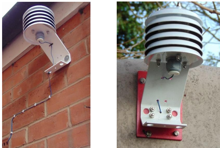
Figure 27: Radiation shield installation
