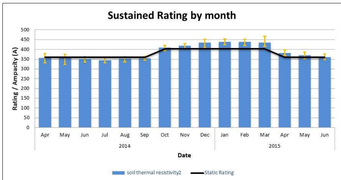
Figure 24 : 33kV Trial Cable Dynamic Asset Rating, averaged by month
