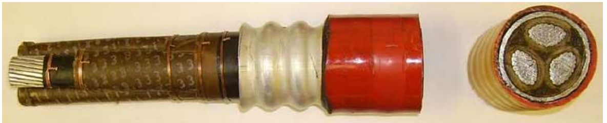
Figure 7: Representative picture of 11kV trial cable
