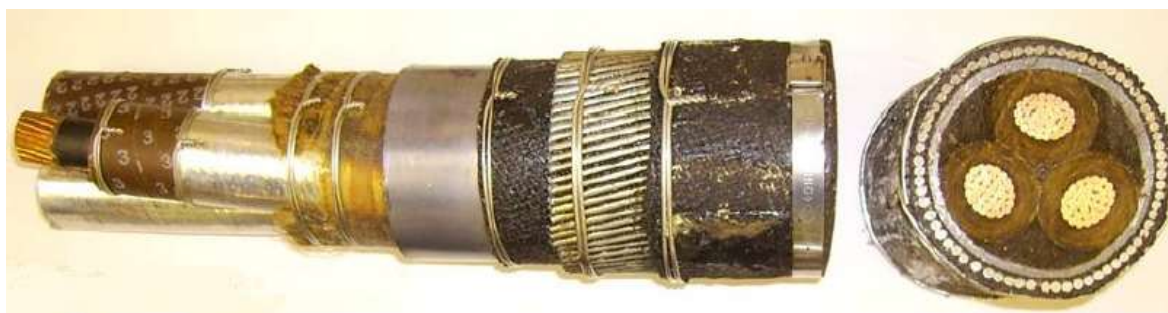
Figure 6: Representative picture of 33kV trial cable
