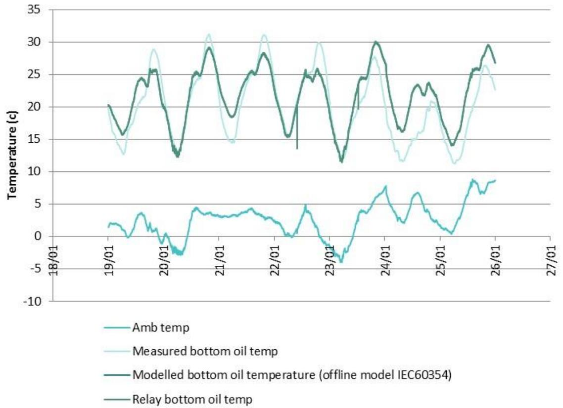
Figure 60 : Bottom-oil temperature modelling results compared to measured and relay values (T2, w/c 19/01/2015).
