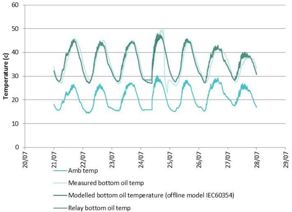
Figure 56 : Bottom-oil temperature modelling results compared to measured and relay values (T2, w/c 21/07/2014).
