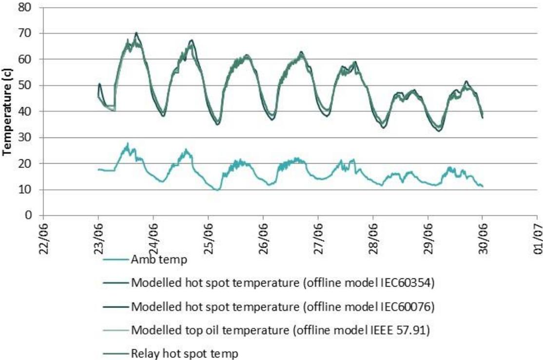
Figure 63 : Hot-spot temperature modelling results with different models compared to relay values (T1, w/c 23/06/2014).
