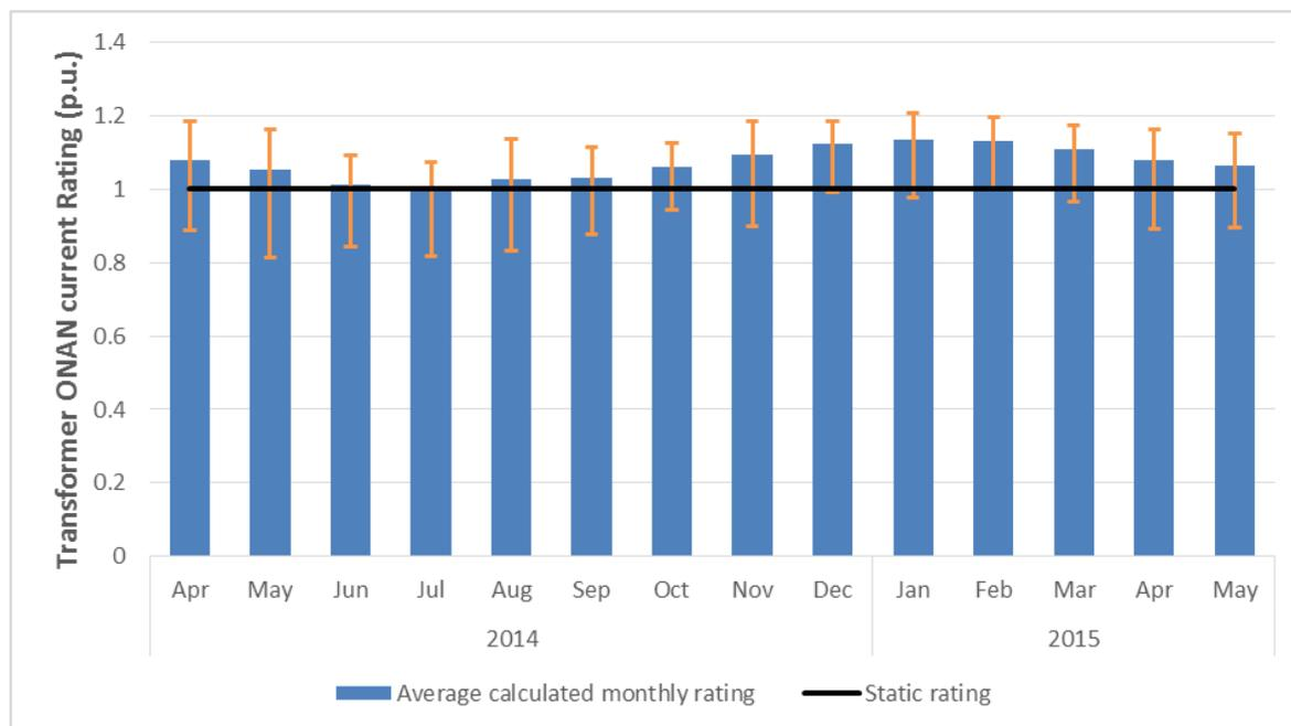
**Figure 20 : Primary transformer T1 monthly dynamic rating limits under ONAN cooling for unit loss-of-life operation (98°C limit)**
