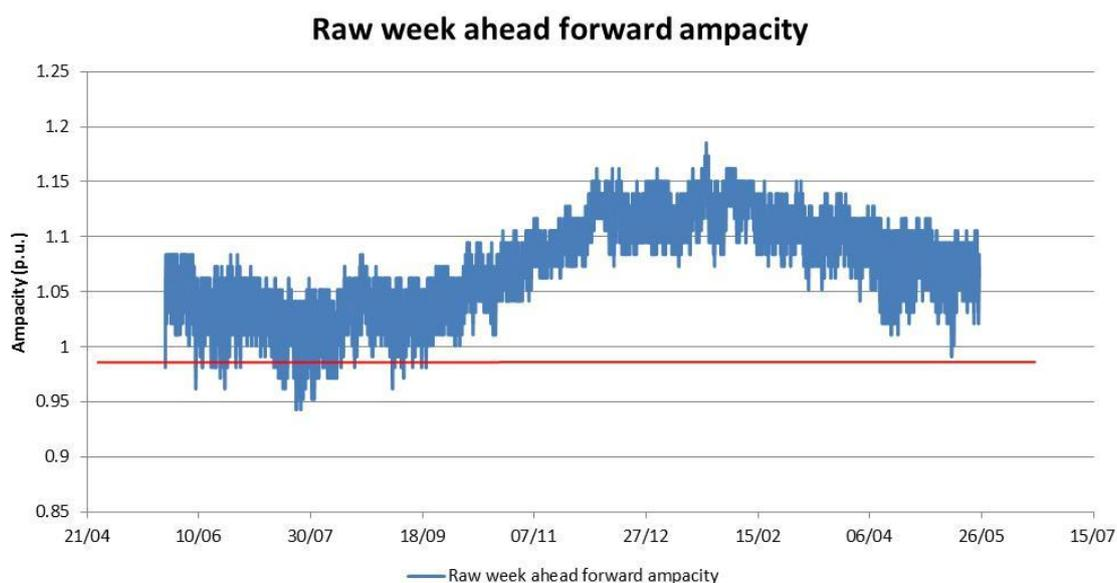
**Figure 26 : Raw week-ahead forward ampacity for unit loss-of-life operation (98°C limit) with ONAN cooling using BBC day-ahead data**
