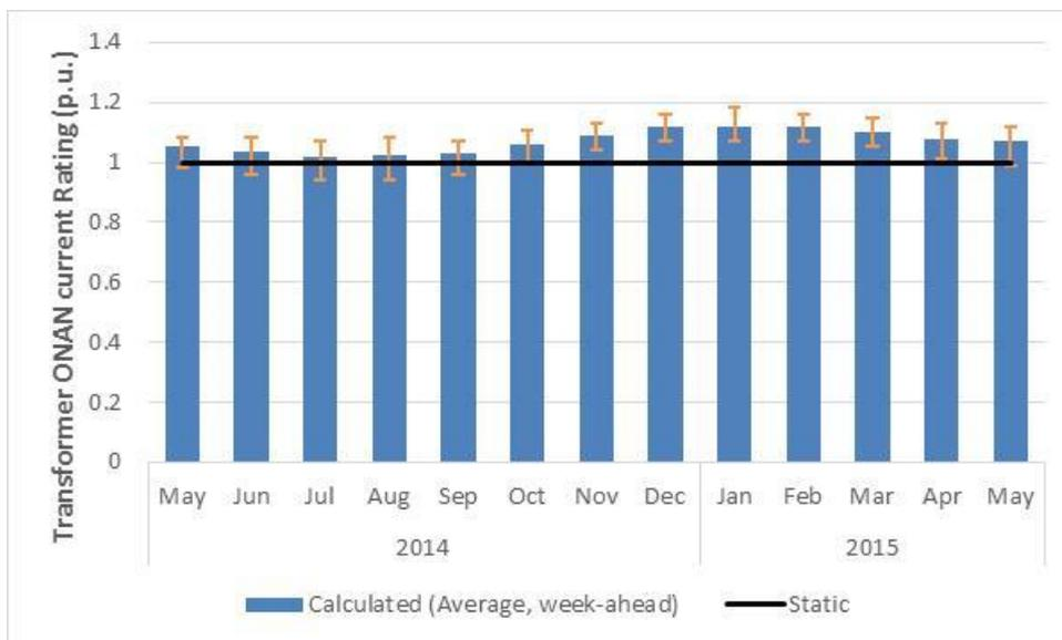
Figure 27 : Raw week ahead forward ampacity as monthly averages with maximum and minimum indicators
