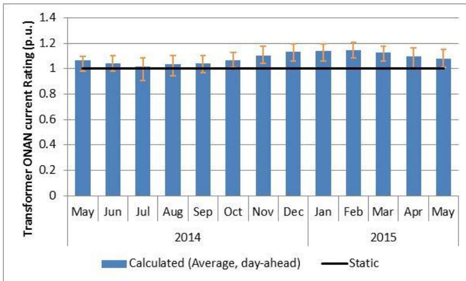
Figure 24 : Raw day ahead forward ampacity as monthly averages with maximum and minimum indicators
