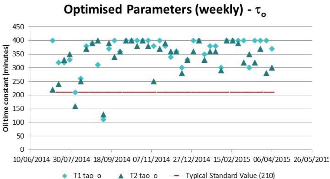
Figure 10: Optimise parameter  $\tau_o$  using weekly data (T1 and T2)
