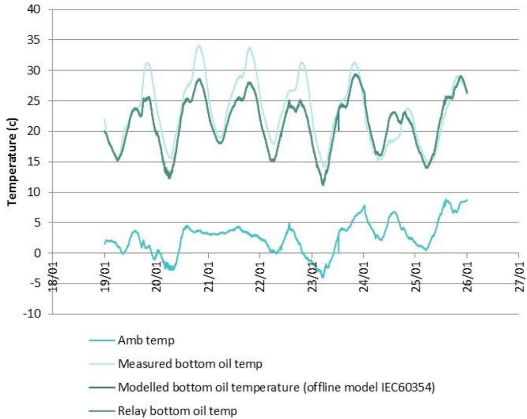
Figure 59 : Bottom-oil temperature modelling results compared to measured and relay values (T1, w/c 19/01/2015).
