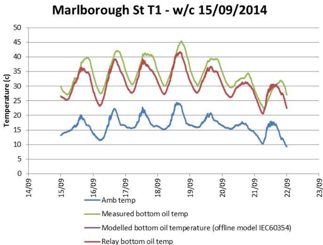
Figure 13: Bottom-oil temperature modelling results compared to measured and relay values (T1, w/c 15/09/2015)
