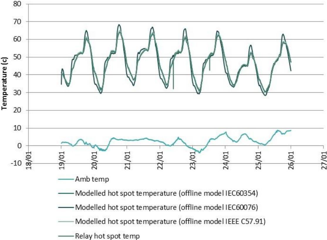
Figure 70 : Hot-spot temperature modelling results with different models compared to relay values (T2, w/c 19/01/2015).
