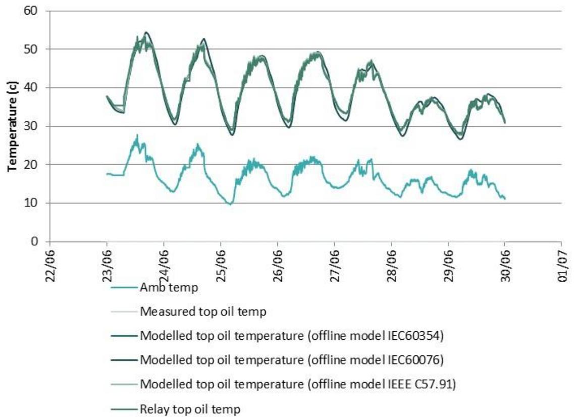
Figure 44 : Top-oil temperature modelling results with different models compared to measured and relay values (T2, w/c 23/06/2014).
