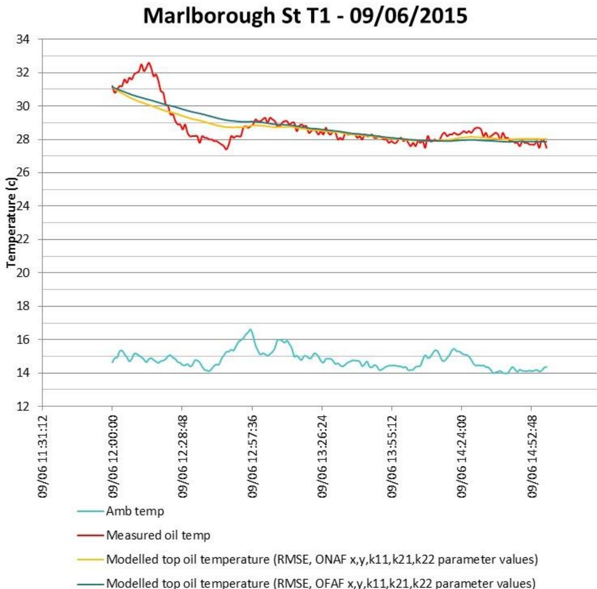
Figure 40: OFAN fitting results using ONAF or OFAF model parameters.
