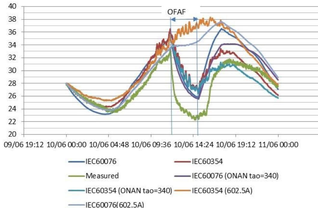
Figure 36: Top-oil temperature comparison, T1, OFAF trial 12.00 – 15.00, 10<sup>th</sup> Jun 2015
