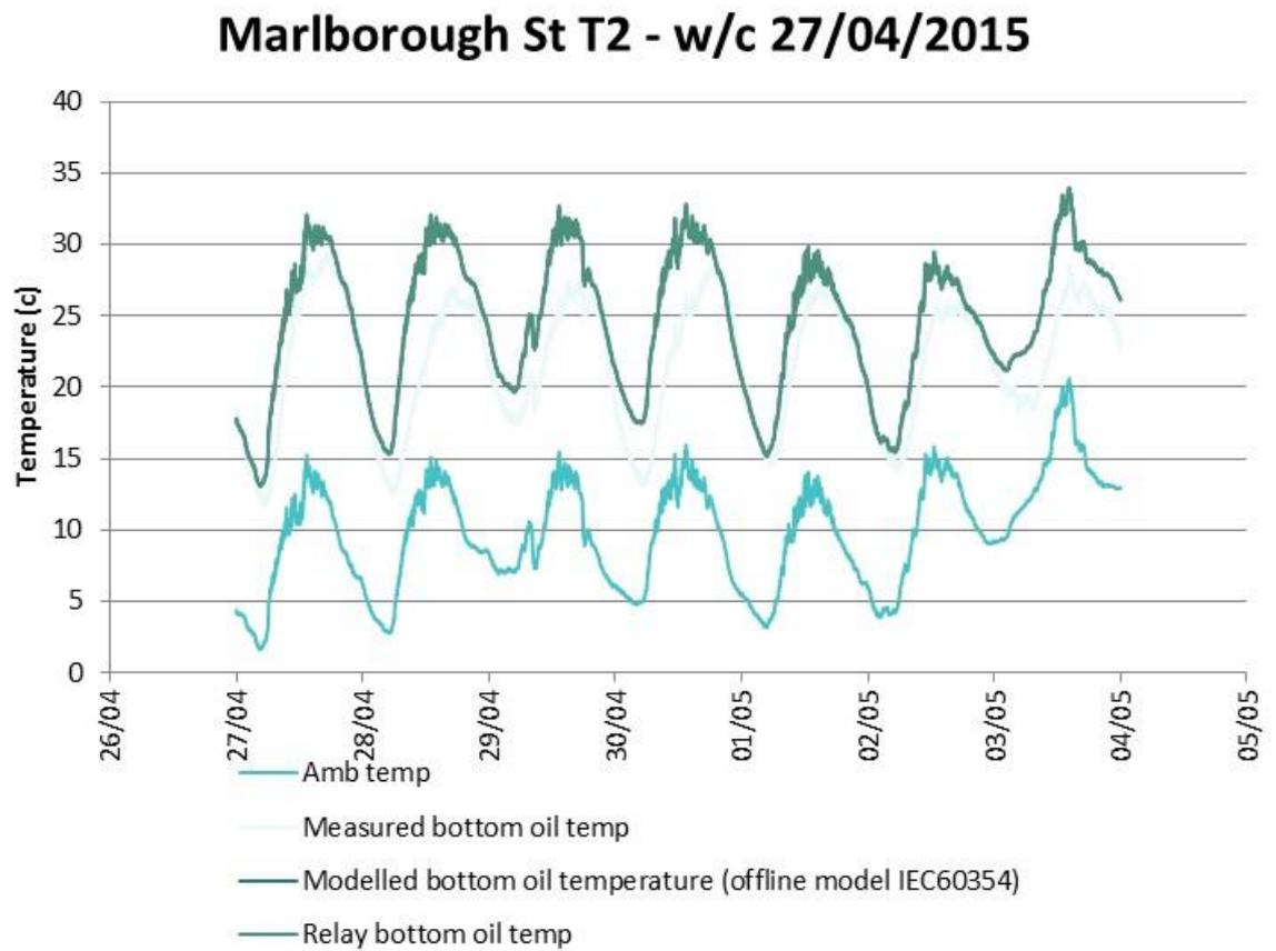
Figure 52 : Bottom-oil temperature modelling results compared to relay values (T2, w/c 27/04/2015).
