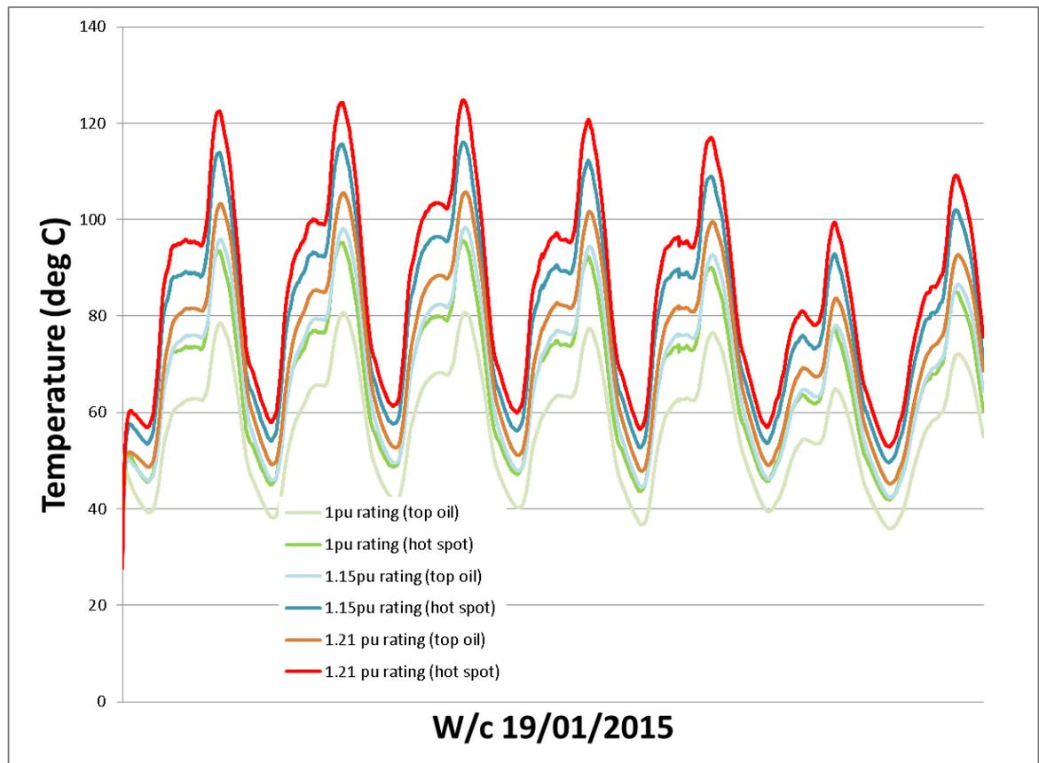
Figure 22 : of hotspot (and top oil) temperatures associated with the modelled load current (peaking at 19MVA equivalent), with the experienced ambient air temperatures)
