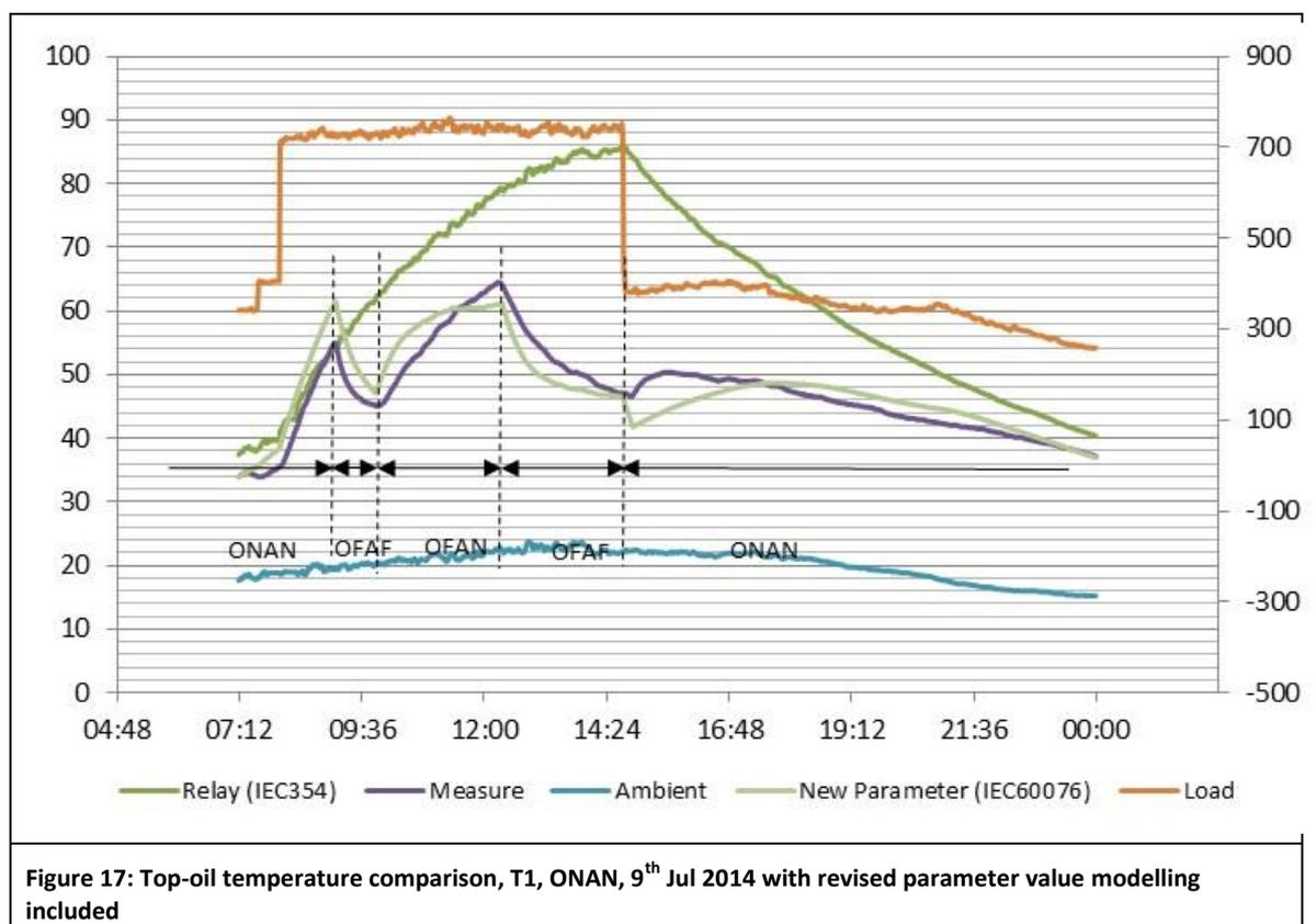
Figure 17: Top-oil temperature comparison, T1, ONAN, 9<sup>th</sup> Jul 2014 with revised parameter value modelling included
