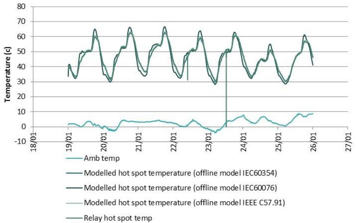
Figure 69 : Hot-spot temperature modelling results with different models compared to relay values (T1, w/c 19/01/2015).
