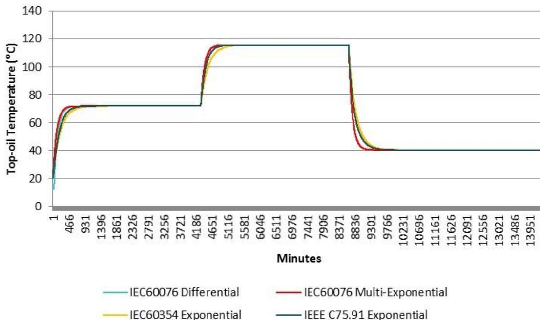
Figure 32: Top oil temperature calculation with different models (long-term step loading)
