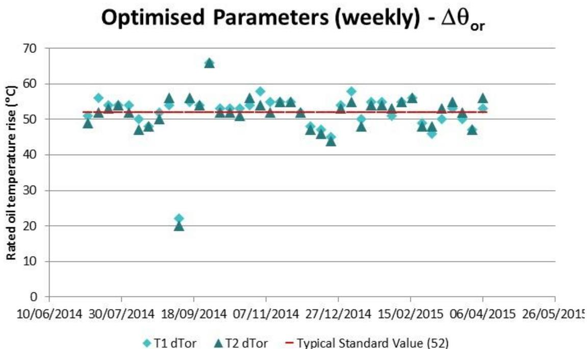
Figure 9: Optimise parameter  $\Delta\theta_{or}$  using weekly data (T1 and T2).
