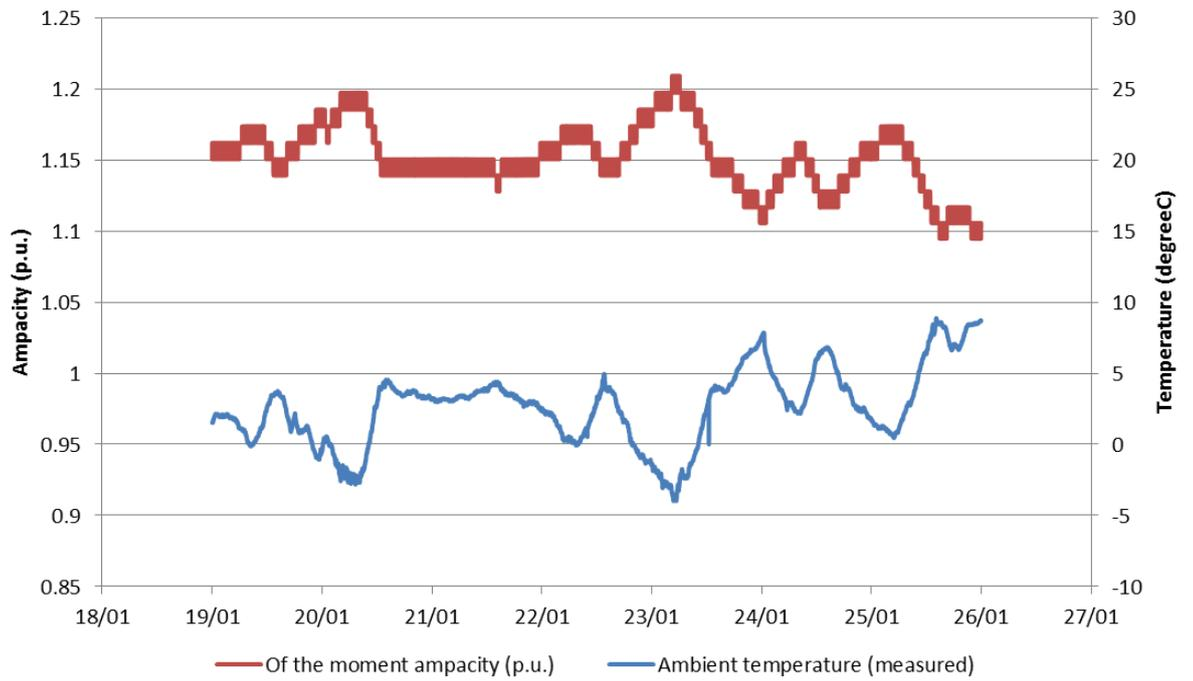
Figure 78: Of-the-moment ampacity (load factor) (ambient temperature w/c 19/01/2015) - Winter.
