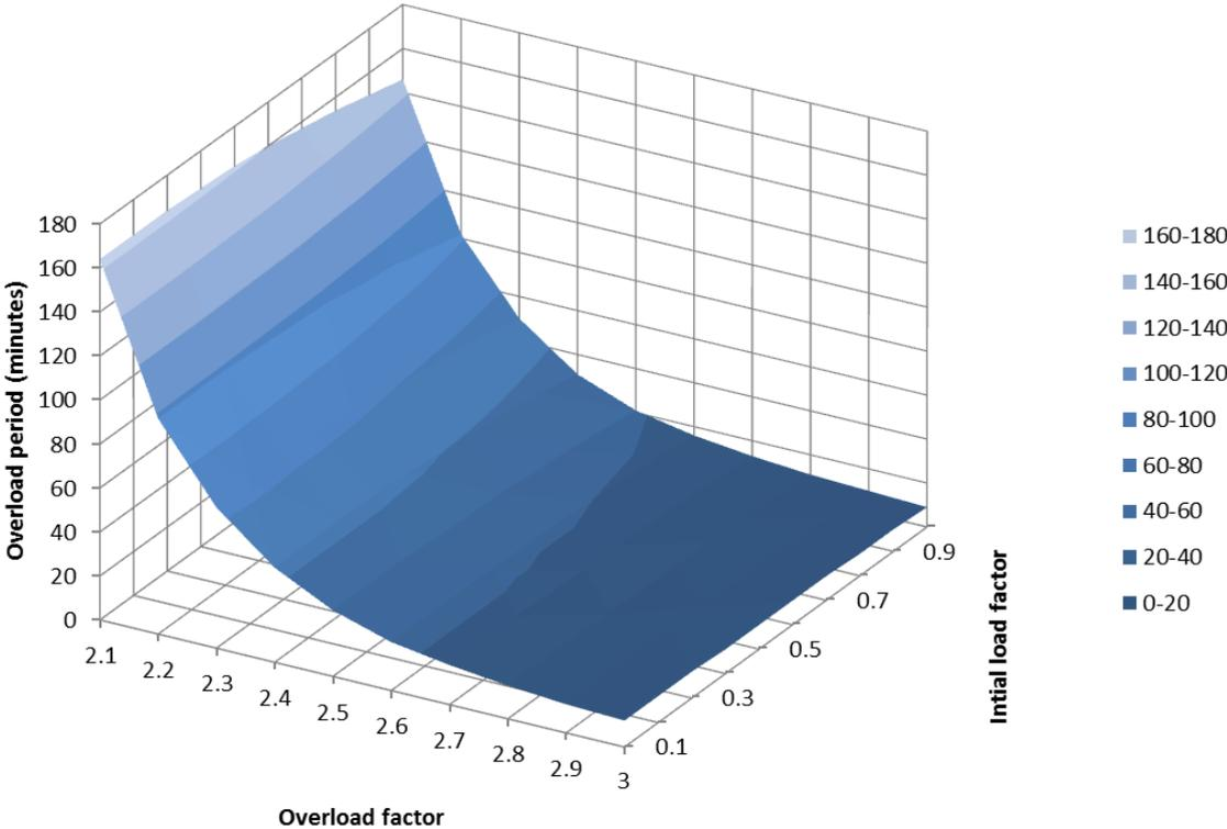
Figure 80: Short-term overload allowable period (pre-emptive OFAF).
