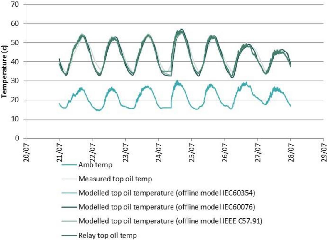
Figure 45 : Top-oil temperature modelling results with different models compared to measured and relay values (T1, w/c 21/07/2014).
