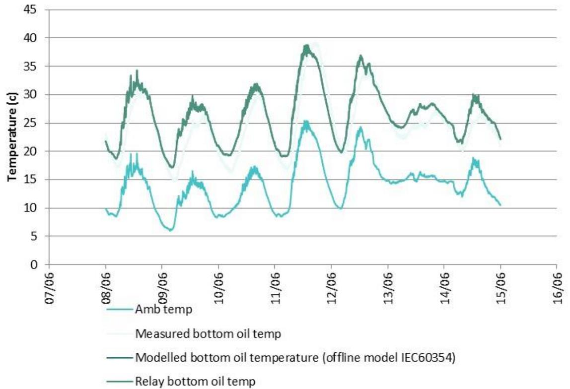
Figure 54 : Bottom-oil temperature modelling results compared to relay values (T2, w/c 08/06/2015).
