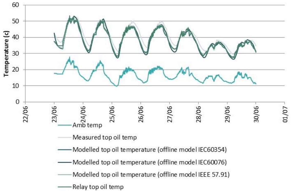
Figure 43 : Top-oil temperature modelling results with different models compared to measured and relay values (T1, w/c 23/06/2014).
