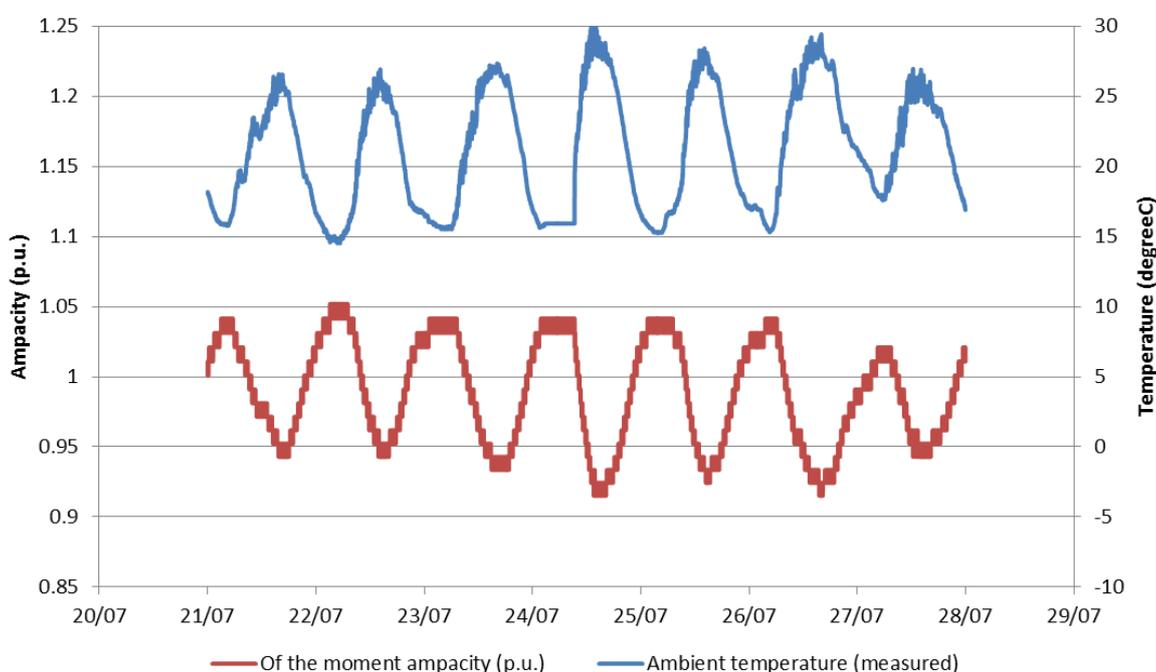
**Figure 19 : Dynamic rating and ambient air temperature for w/c 21/07/2014 – High summer.**
