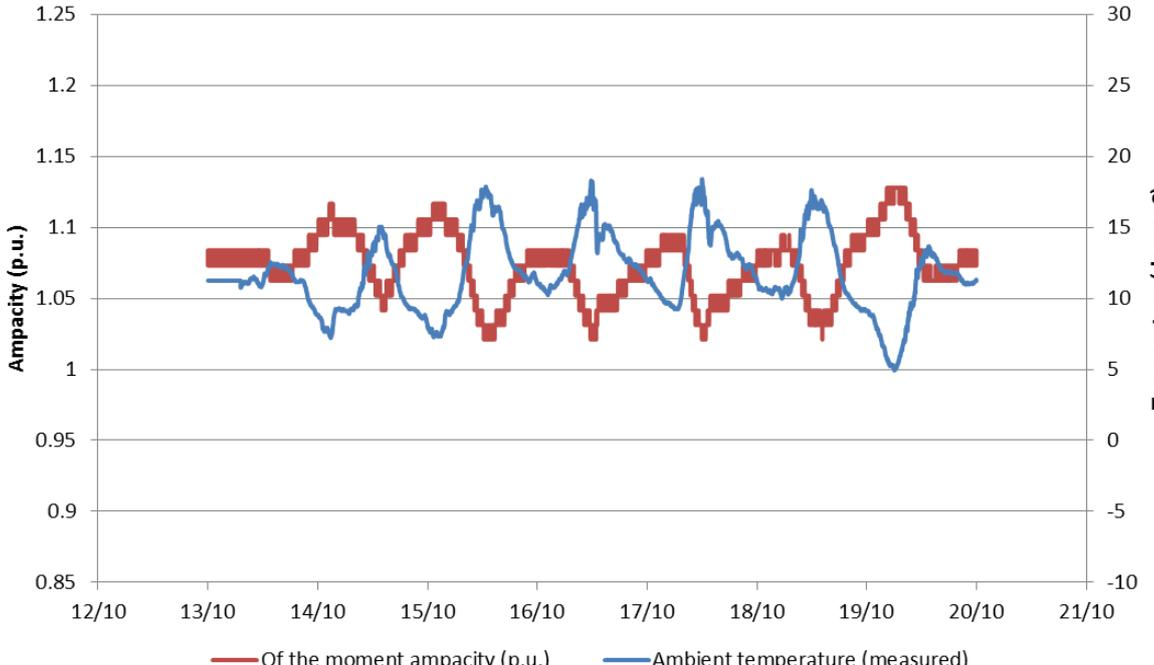
Figure 77: Of-the-moment ampacity (load factor) (ambient temperature w/c 13/10/2014) - Autumn.
