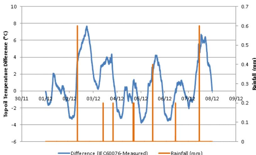
**Figure 73: Comparisons between model-calculated and measured oil temperature values with precipitation (w/c 01/12/2014)**
