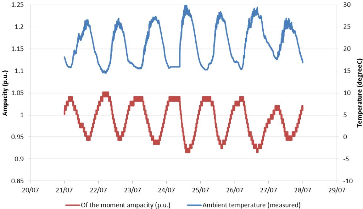
Figure 76: Of-the-moment ampacity (load factor) (ambient temperature w/c 21/07/2014) – High summer.
