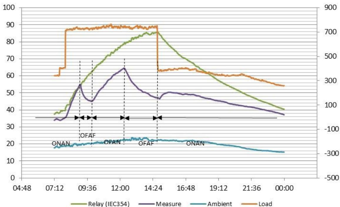
Figure 16: Top-oil temperature comparison, T1, ONAN, 9<sup>th</sup> Jul 2014
