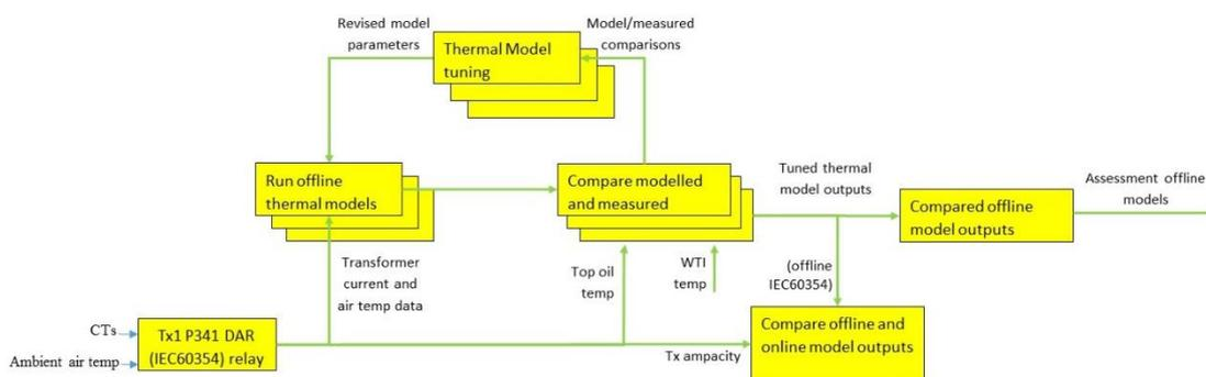
Figure 7: Thermal model validation process
