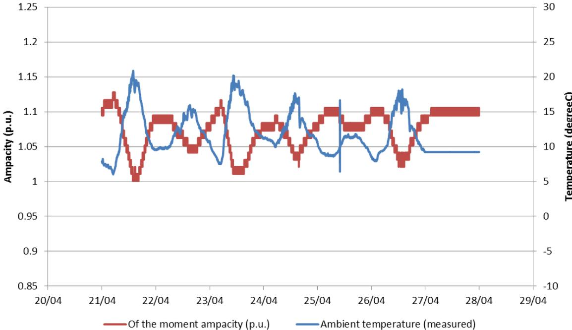
Figure 74: Of-the-moment ampacity (load factor) (ambient temperature w/c 21/04/2014) – Spring.
