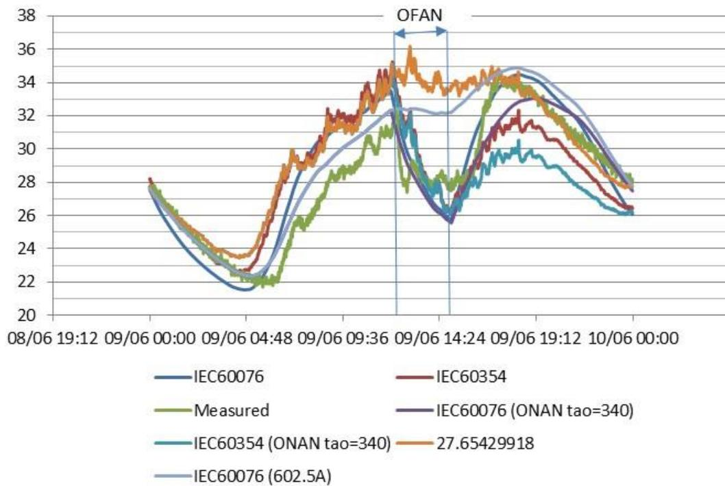
Figure 35: Top-oil temperature comparison, T1, OFAN trial 12.00 – 15.00, 9<sup>th</sup> Jun 2015
