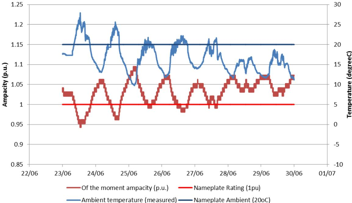
Figure 75: of-the-moment ampacity (load factor) (ambient temperature w/c 23/06/2014) – Summer.
