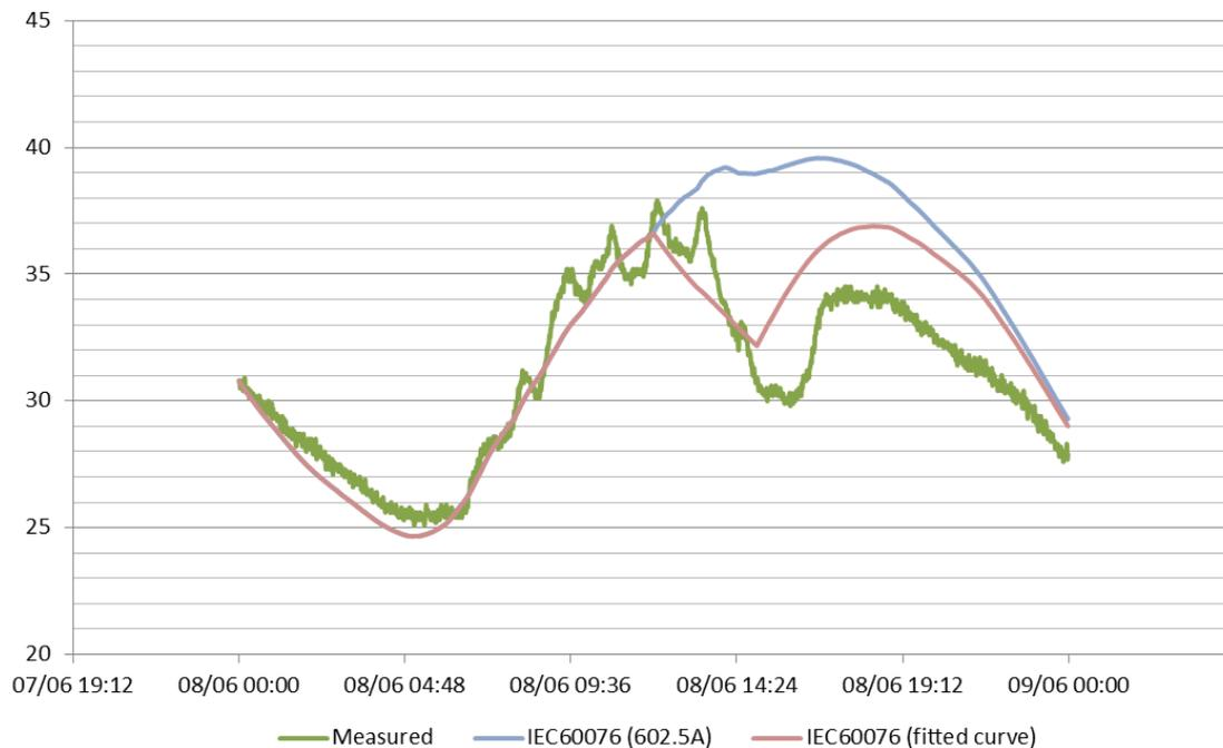
**Figure 37: Top-oil temperature comparison with curve fitting results, T1, ONAF trial 12.00 – 15.00, 8<sup>th</sup> Jun 2015**
