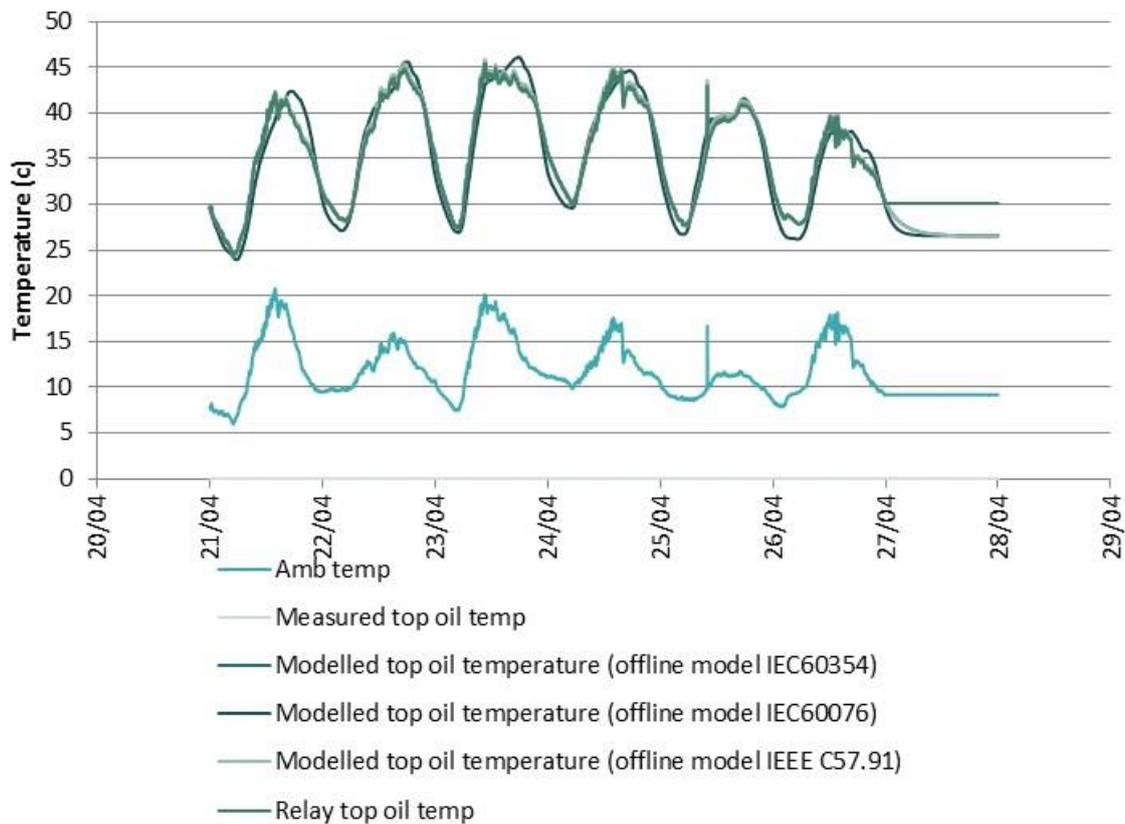
Figure 42 : Top-oil temperature modelling results with different models compared to measured and relay values (T2, w/c 21/04/2014).
