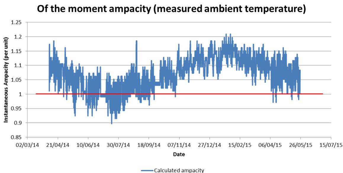
**Figure 18 : Dynamic rating for unit loss-of-life operation (98°C limit) with ONAN cooling over trial period**
