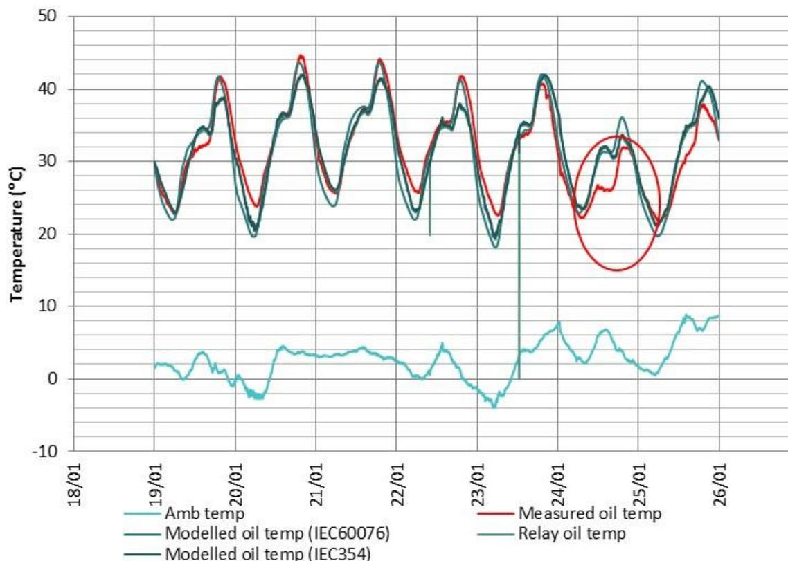
Figure 15: Modelling results with different models compared to measured values (T1, w/c 19/01/2015)
