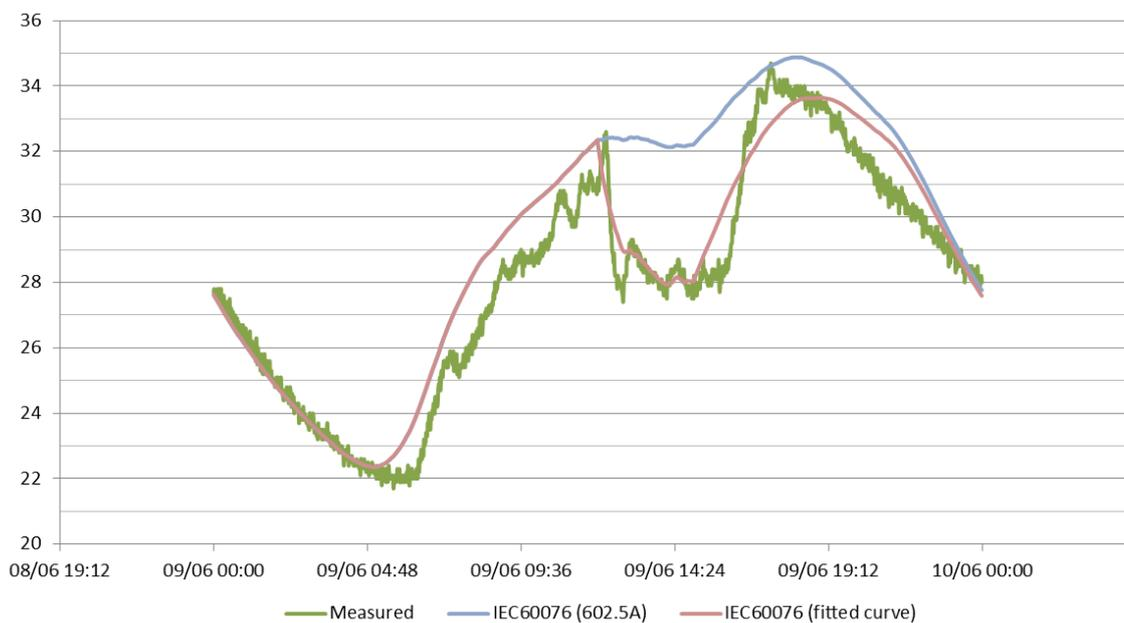
**Figure 38: Top-oil temperature comparison with curve fitting results, T1, OFAN trial 12.00 – 15.00, 9<sup>th</sup> Jun 2015 using ONAF standard constant values**
