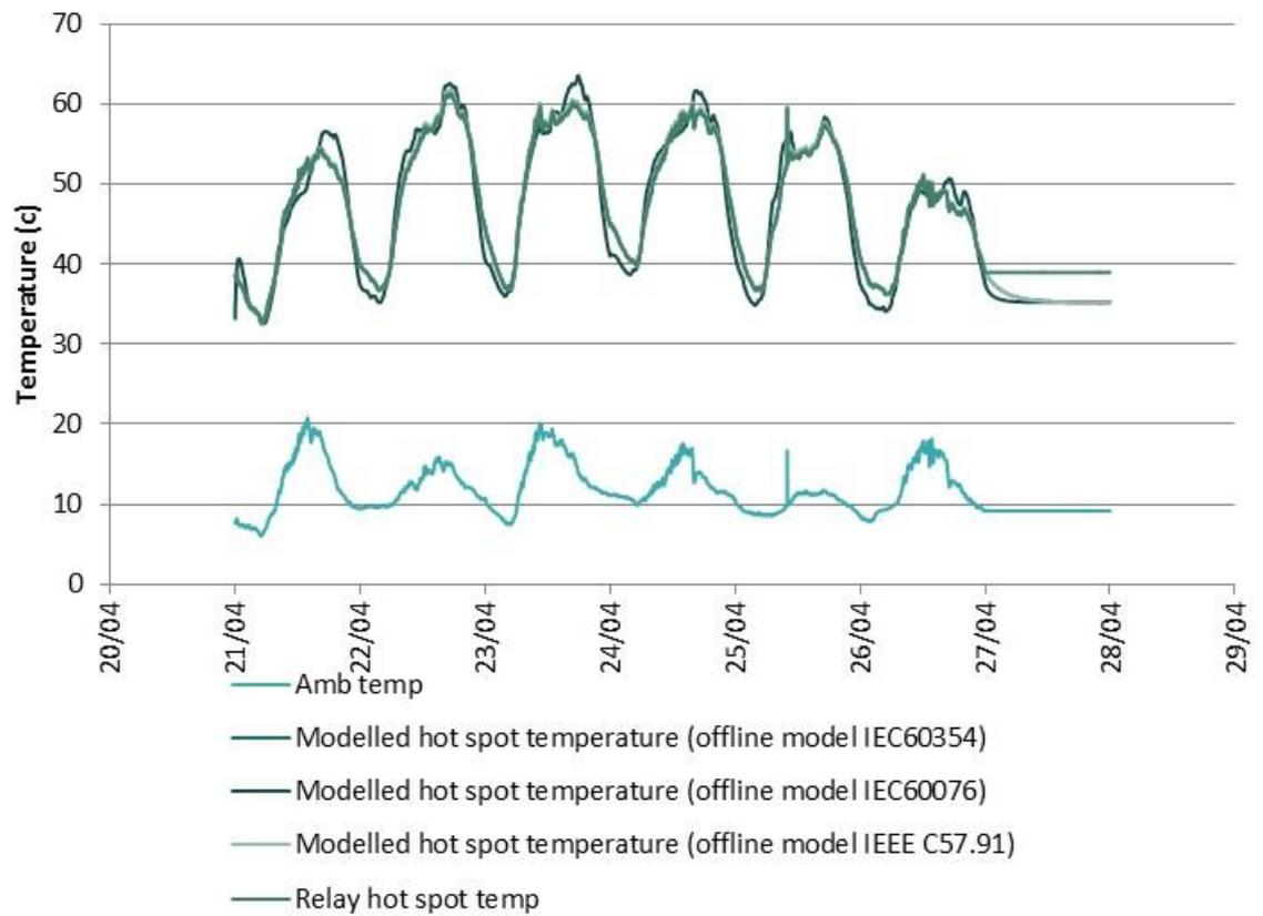
Figure 62 : Hot-spot temperature modelling results with different models compared to relay values (T2, w/c 21/04/2014).
