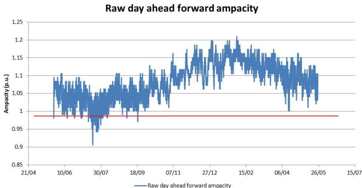
**Figure 23 : Raw day-ahead forward ampacity for unit loss-of-life operation (98°C limit) with ONAN cooling using BBC day-ahead data**
