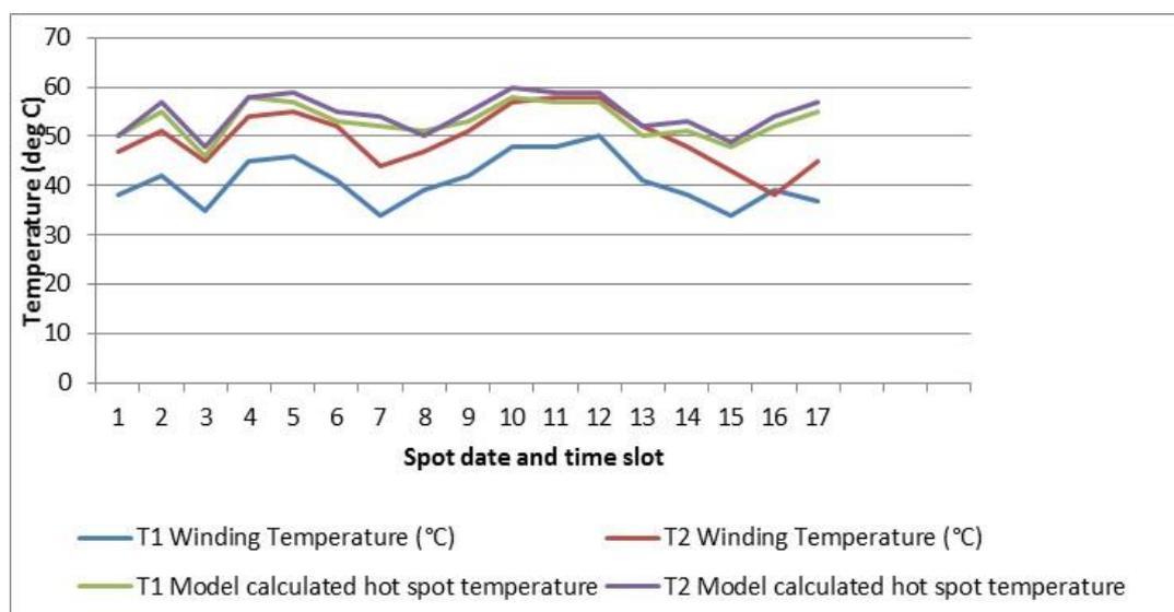
Figure 14: Hot spot temperature modelling results compared to measured WTI values
