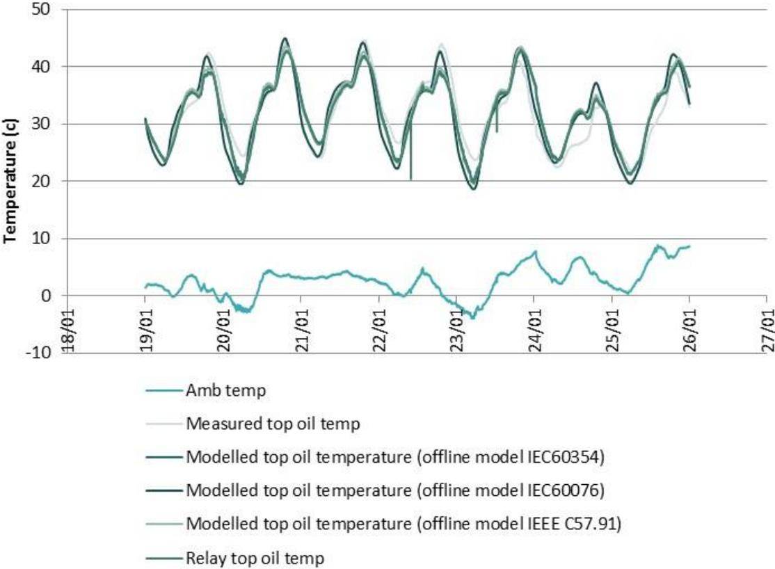
Figure 50 : Top-oil temperature modelling results with different models compared to measured and relay values (T2, w/c 19/01/2015).
