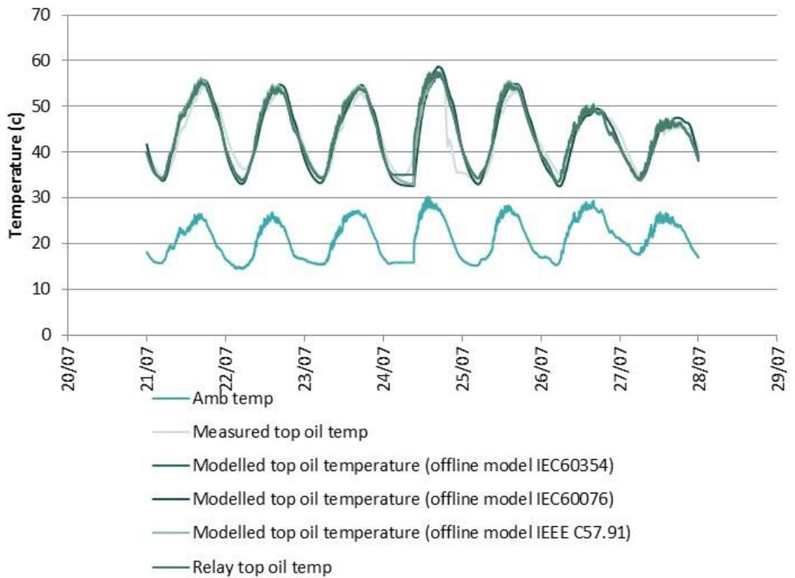
Figure 46 : Top-oil temperature modelling results with different models compared to measured and relay values (T2, w/c 21/07/2014).
