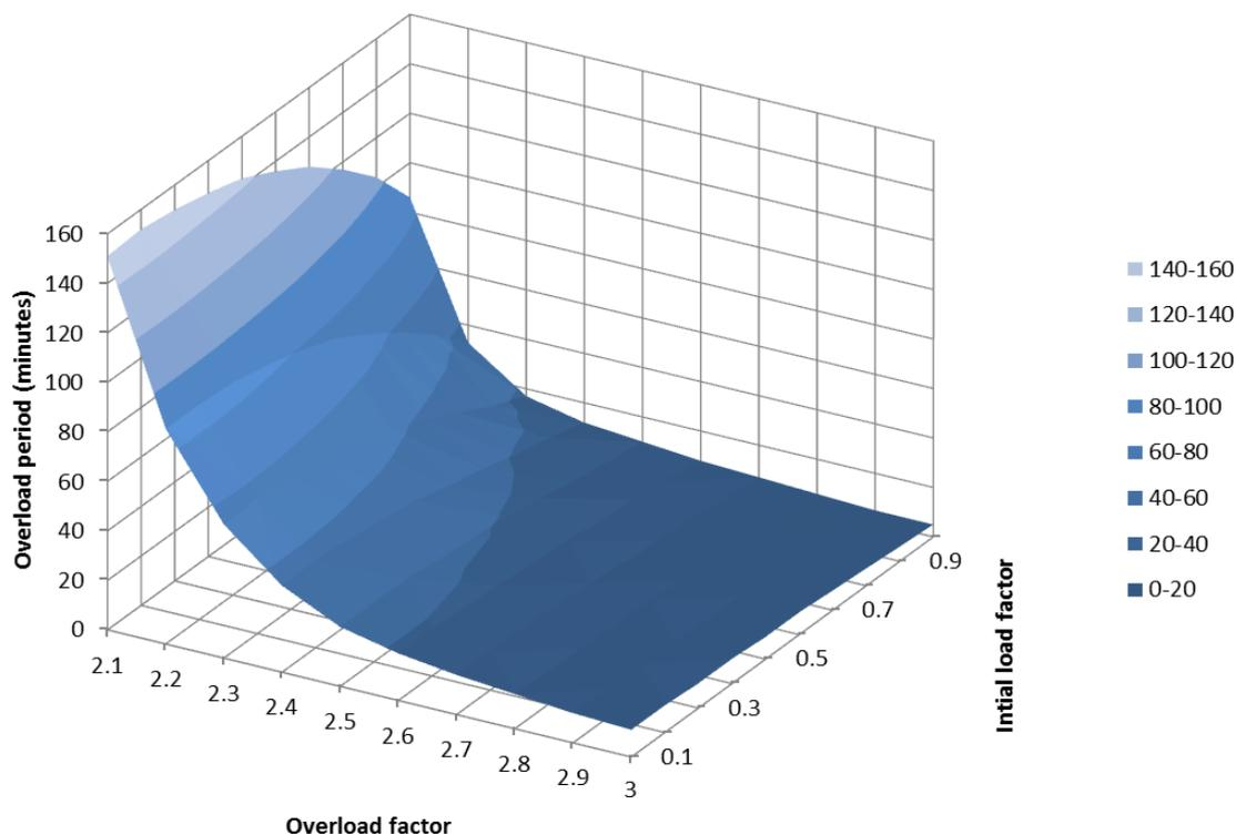
Figure 79: Short-term overload allowable period (OFAF).
