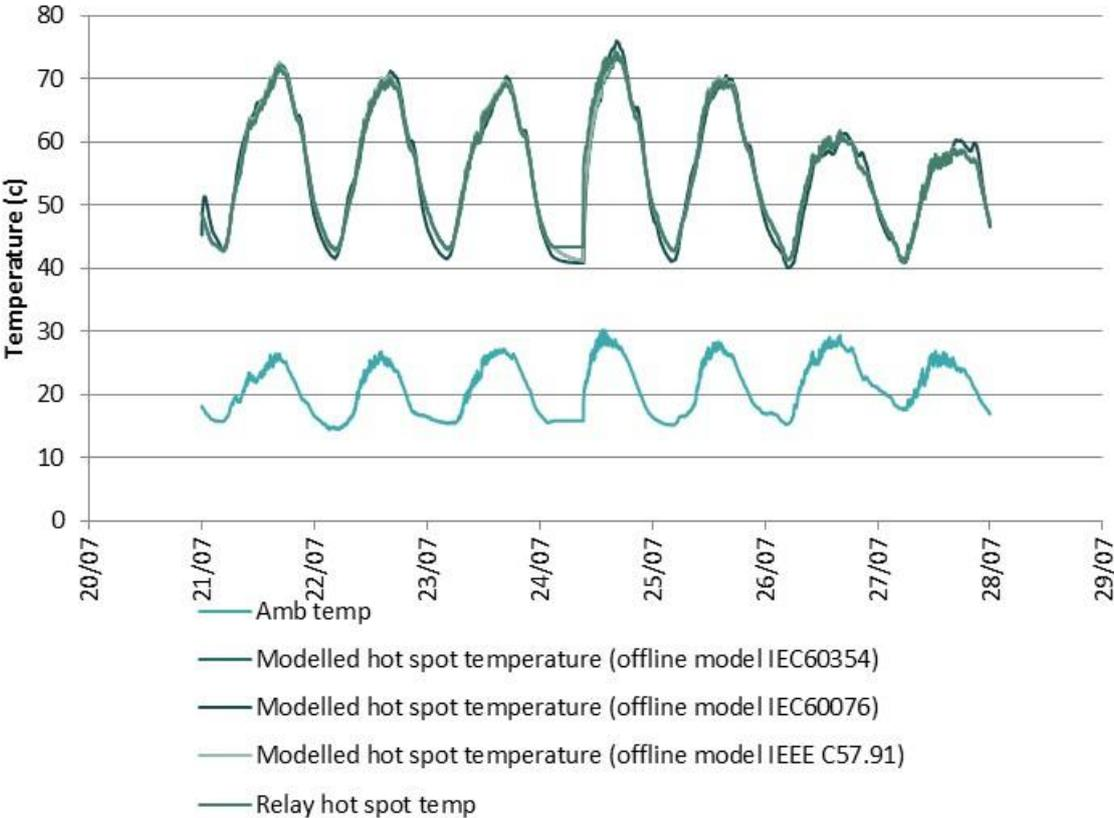
Figure 66 : Hot-spot temperature modelling results with different models compared to relay values (T2, w/c 21/07/2014).
