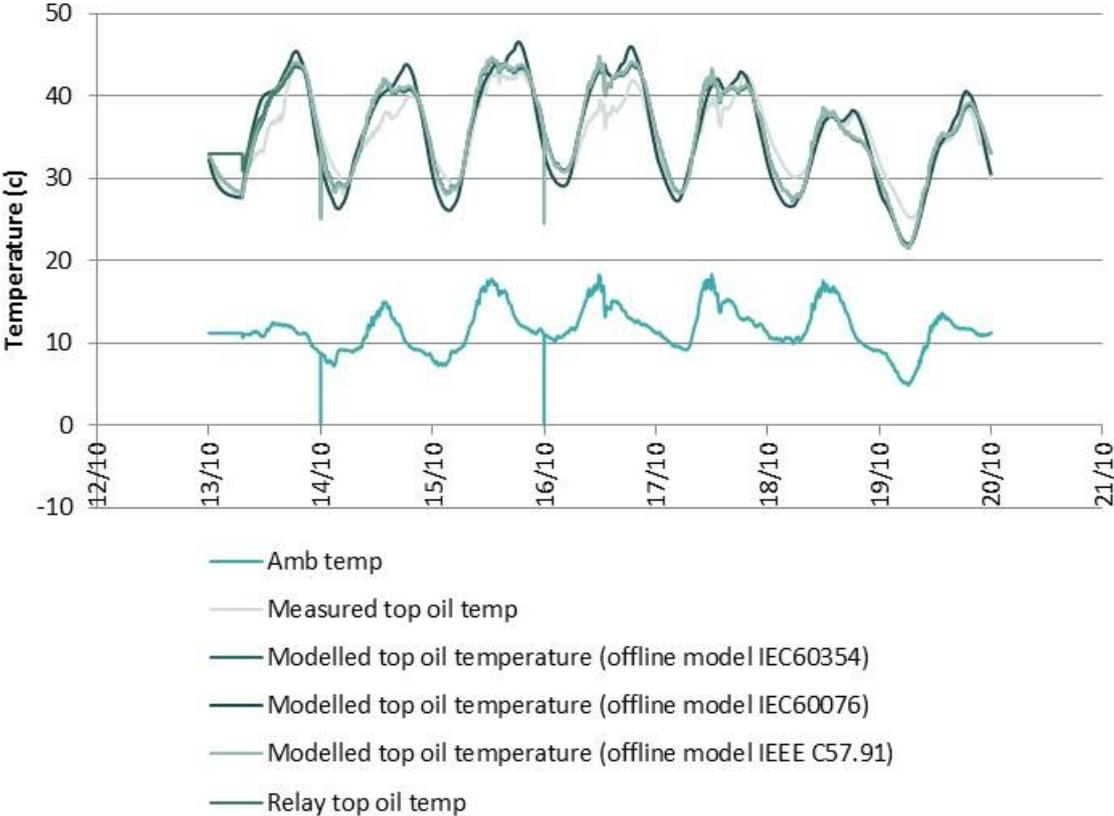
Figure 48 : Top-oil temperature modelling results with different models compared to measured and relay values (T2, w/c 13/10/2014)
