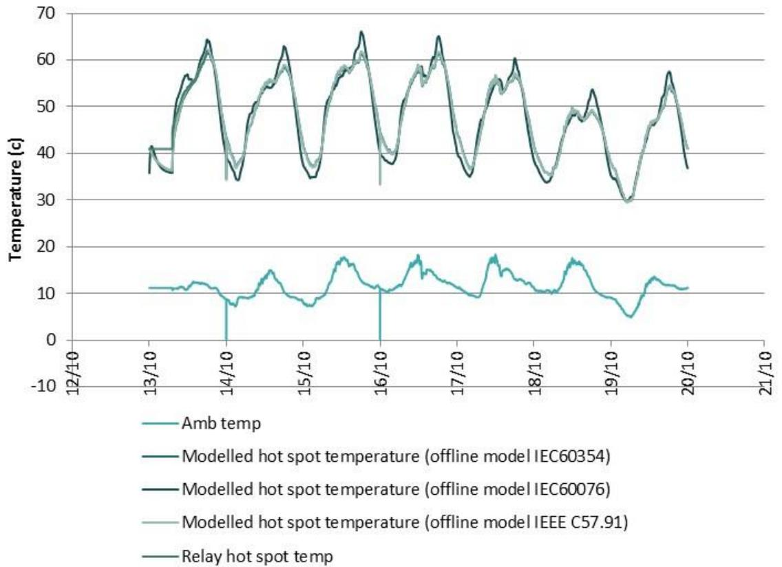
Figure 68 : Hot-spot temperature modelling results with different models compared to relay values (T2, w/c 13/10/2014).
