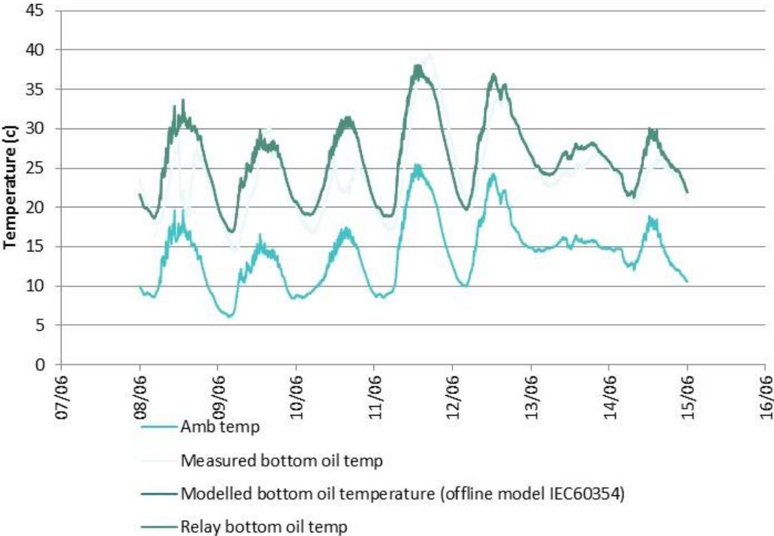
Figure 53 : Bottom-oil temperature modelling results compared to measured and relay values (T1, w/c 08/06/2015).
