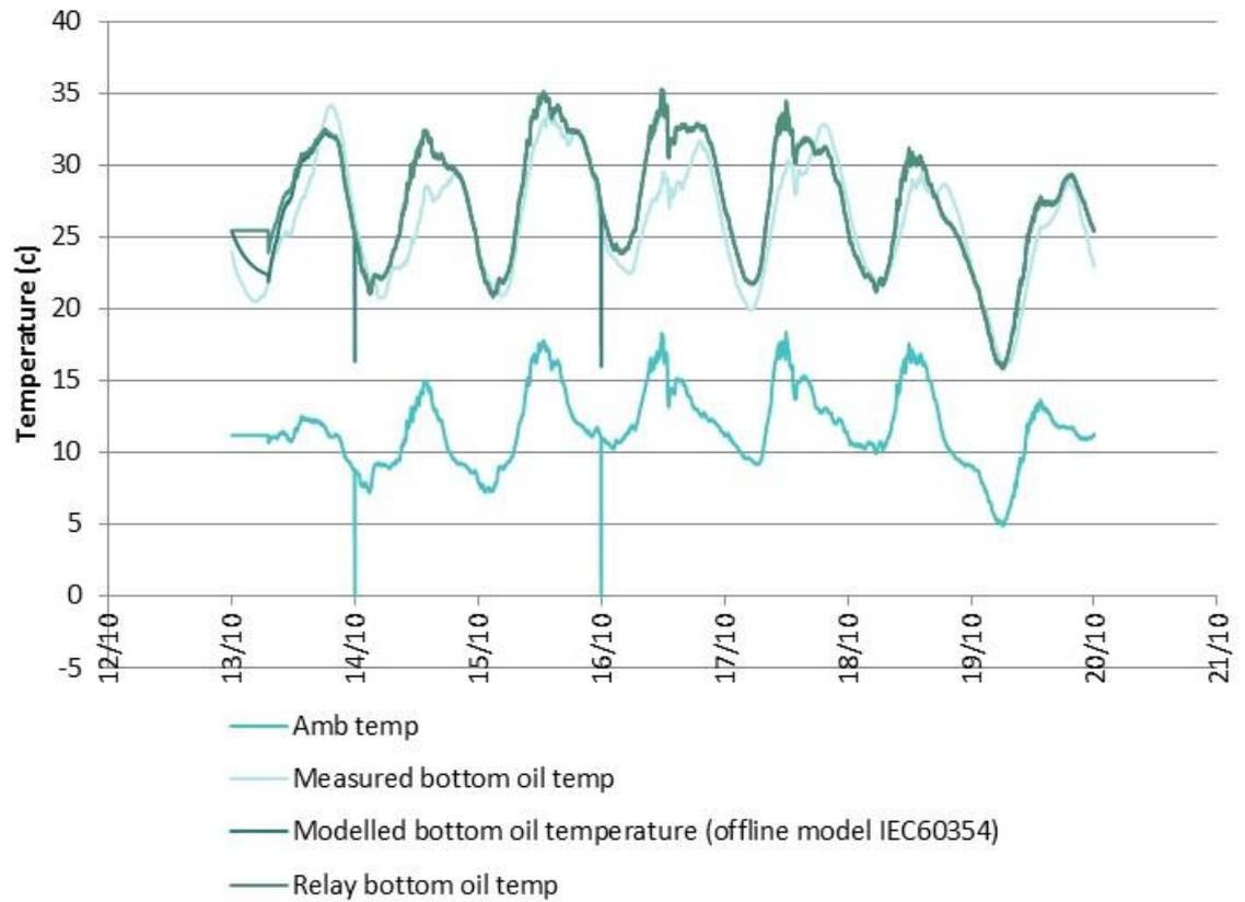
Figure 58 : Bottom-oil temperature modelling results compared to measured and relay values (T2, w/c 13/10/2014).
