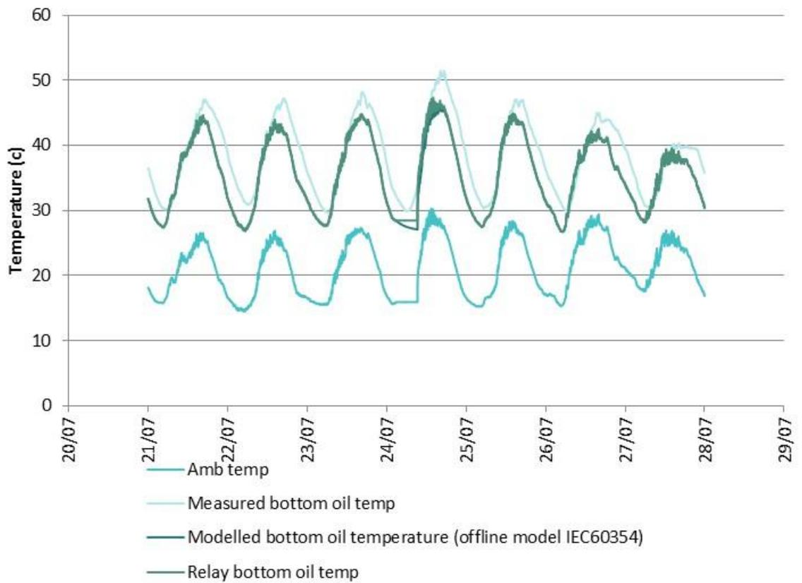
Figure 55 : Bottom-oil temperature modelling results compared to measured and relay values (T1, w/c 21/07/2014).
