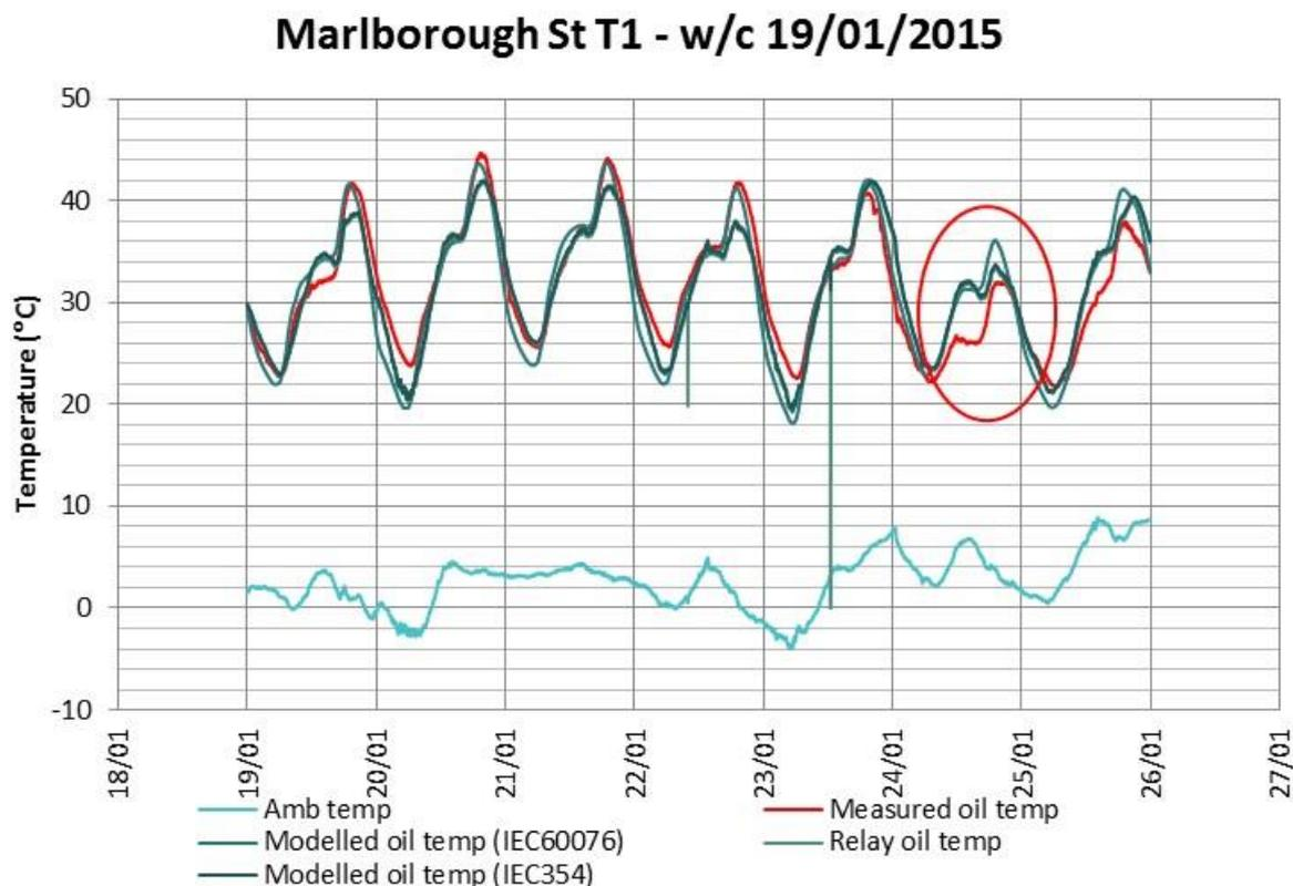
Figure 71 : Modelling results with different models compared to measured values (T1, w/c 19/01/2015).
