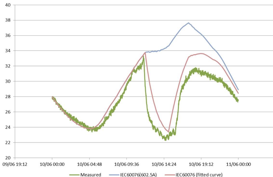
Figure 39: Top-oil temperature comparison with curve fitting results, T1, OFAF trial 12.00 – 15.00, 10<sup>th</sup> Jun 2015
