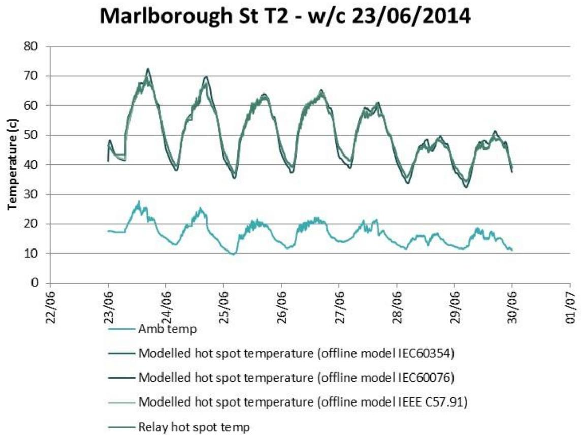
Figure 64 : Hot-spot temperature modelling results with different models compared to relay values (T2, w/c 23/06/2014).
