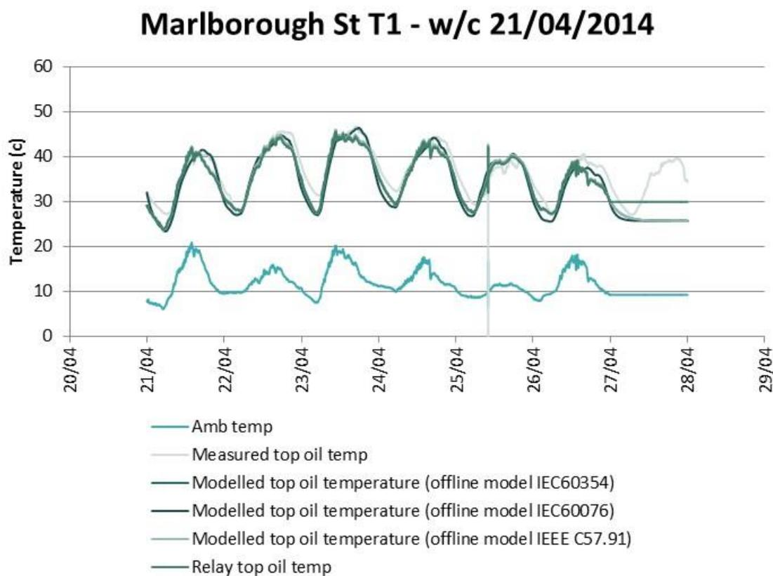
**Figure 41 : Top-oil temperature modelling results with different models compared to measured and relay values (T1, w/c 21/04/2014).**
