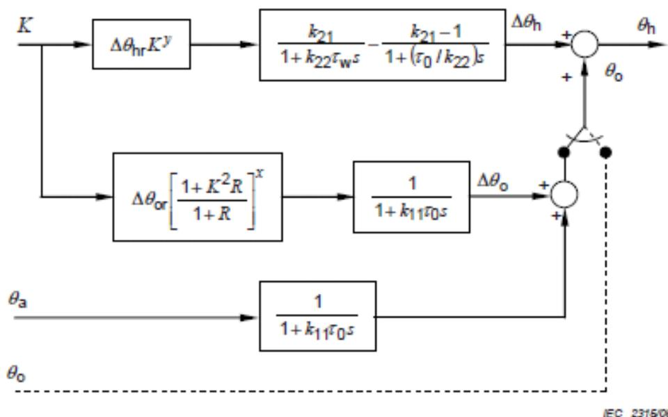
Figure 1: Outline of the IEC 60076 calculation of hot-spot temperature [2]
