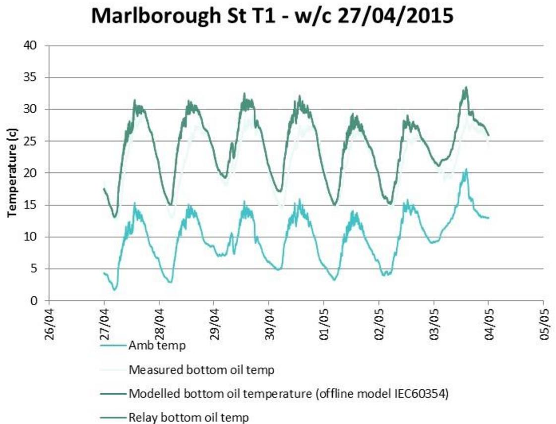
Figure 51 : Bottom-oil temperature modelling results compared to relay values (T1, w/c 27/04/2015).
