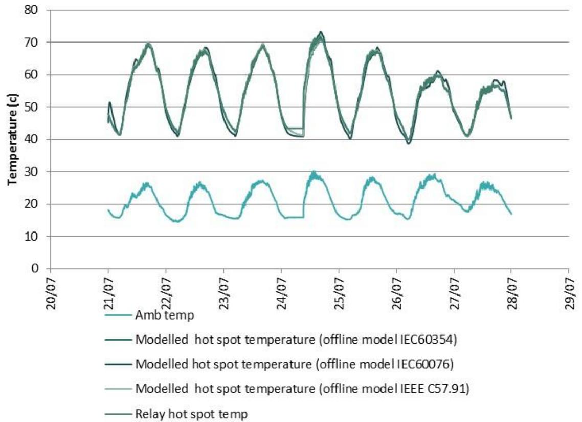
Figure 65 : Hot-spot temperature modelling results with different models compared to relay values (T1, w/c 21/07/2014).
