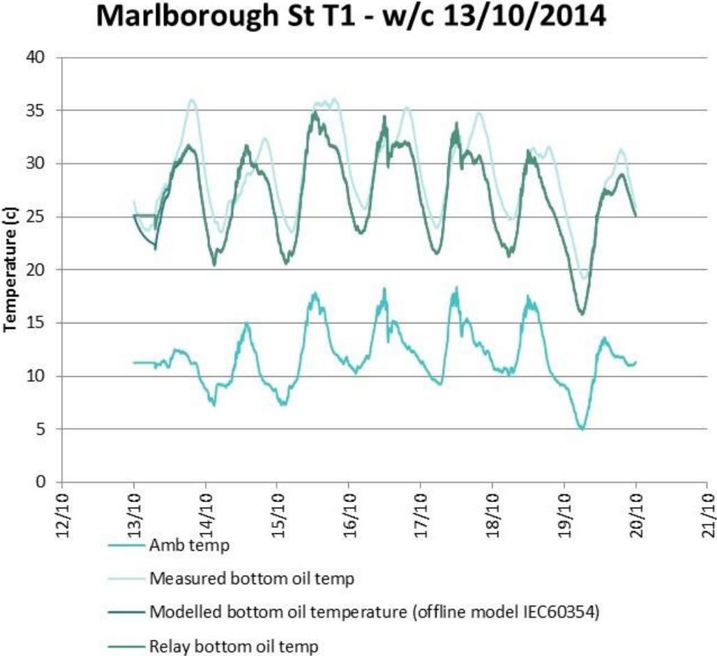
Figure 57 : Bottom-oil temperature modelling results compared to measured and relay values (T1, w/c 13/10/2014).
