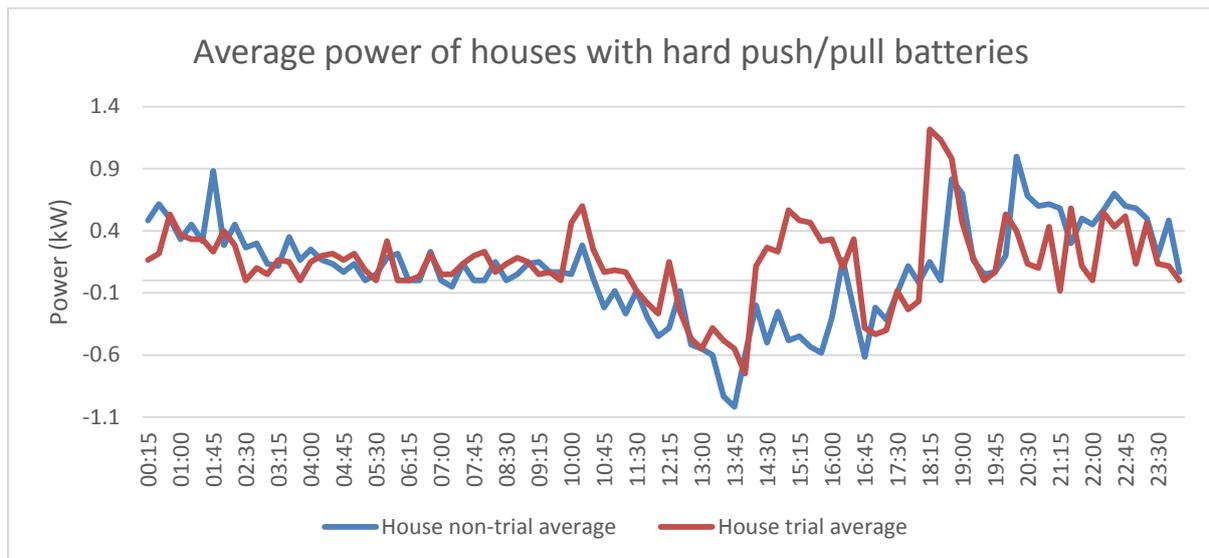
Figure 17 Houses demand comparison with hard push/pull batteries
