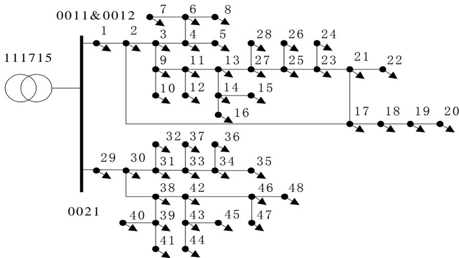
Figure 4 Network configuration of Illminster Avenue substation
