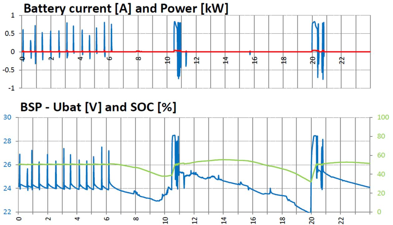
Figure 12 Household battery input power, voltage and SOC in period 1 with low PV export
