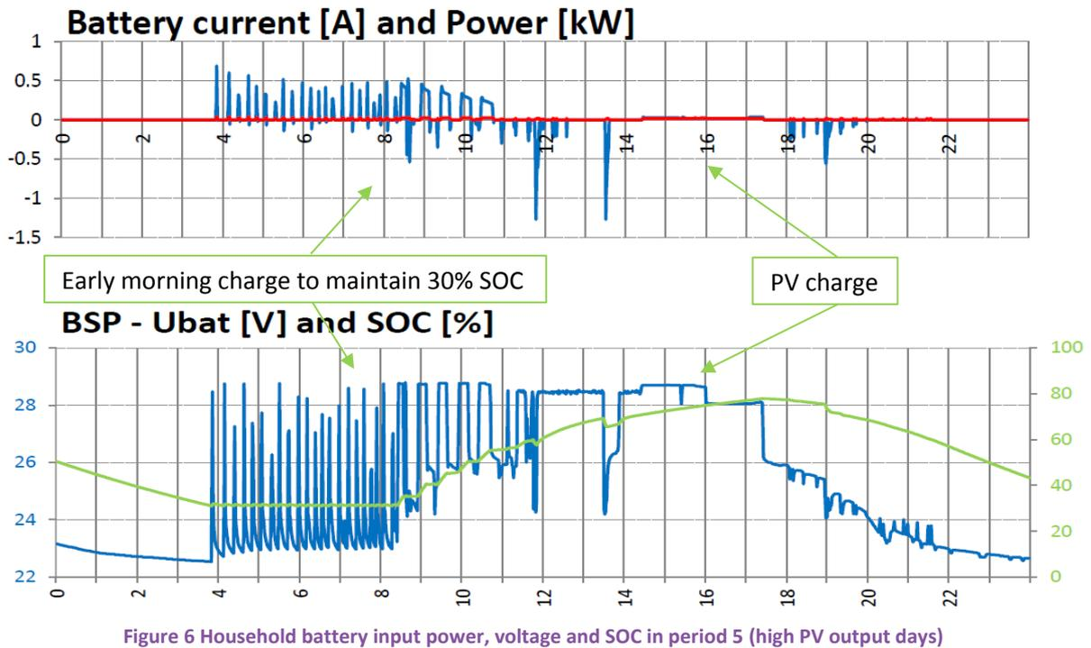
Figure 6 Household battery input power, voltage and SOC in period 5 (high PV output days)
