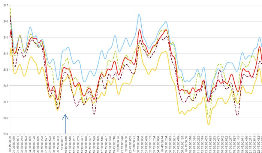
Figure 26 Example of voltage profiles of substation and two houses
