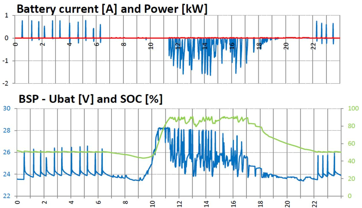
Figure 11 Household battery input power, voltage and SOC in period 1 with high PV export
