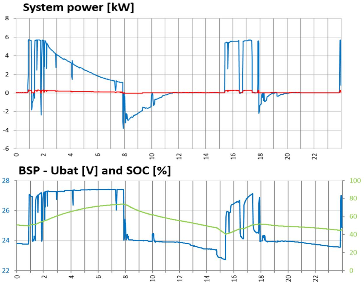
Figure 20 School battery input power, voltage and SOC
