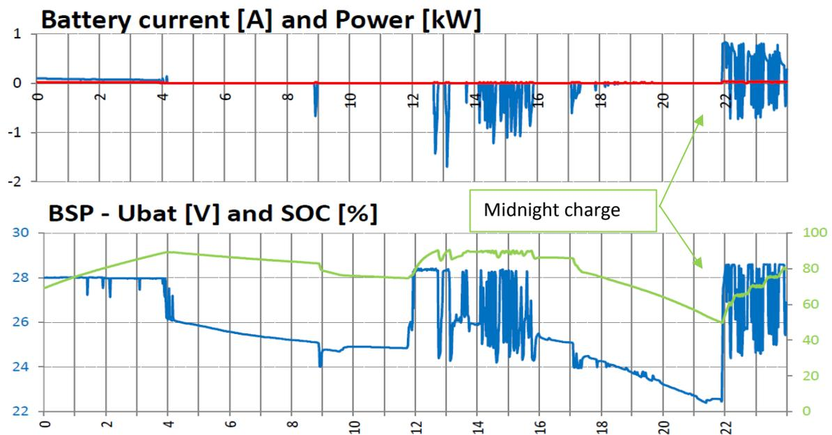
Figure 5 Household battery input power, voltage and SOC in period 4
