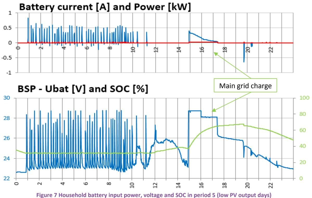
Figure 7 Household battery input power, voltage and SOC in period 5 (low PV output days)
