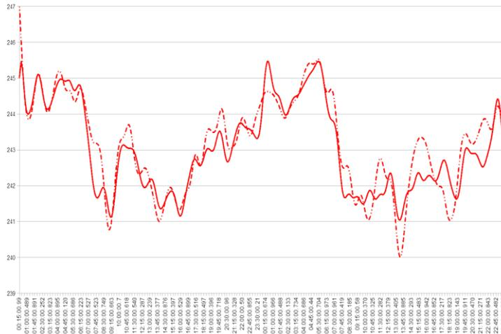
**Figure 27 Voltage profiles of one phase of substation and connected house**
