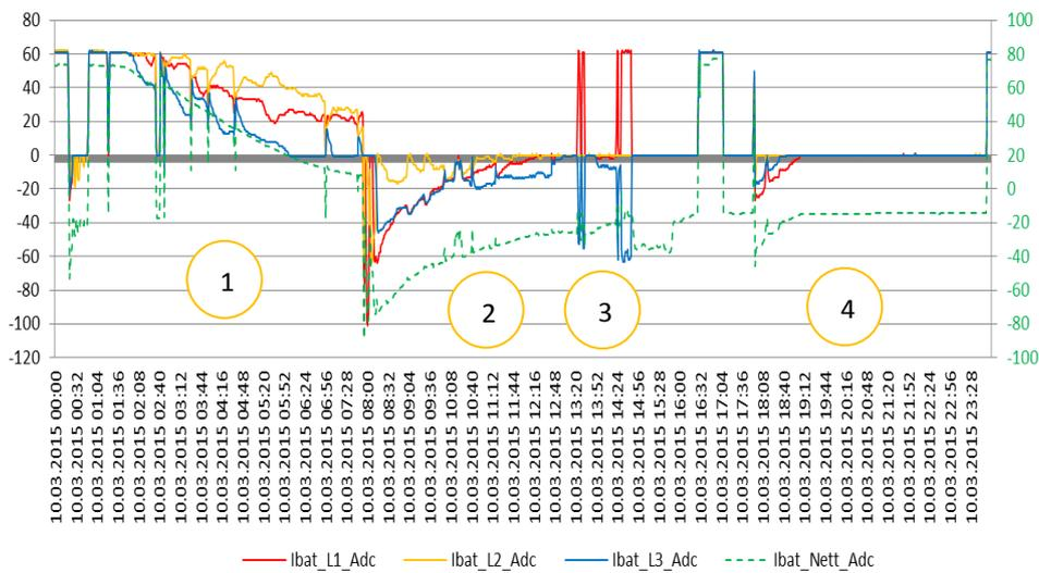
**Figure 21 School battery three phase charging/discharging current**
