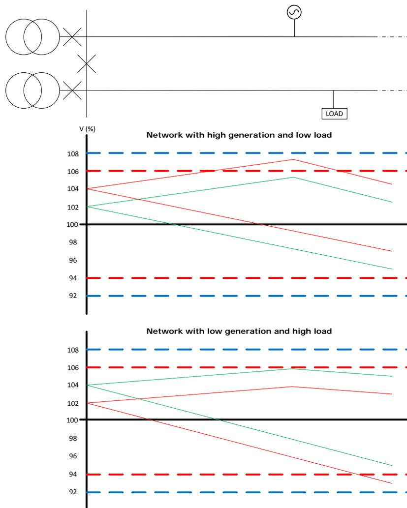
Figure 1 - Graphs of voltage along a line
