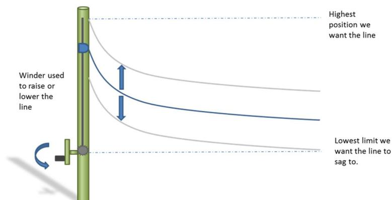
When a load of washing is hung on the line, the weight pulls the line down increasing the risk of the washing dragging on the floor. Winding up at the pole then allows the washing to be lifted.
