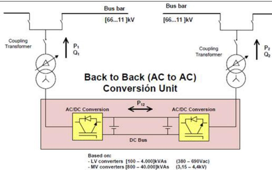
**Figure 4 - Flexible Power Link Schematic (Indicative)**
