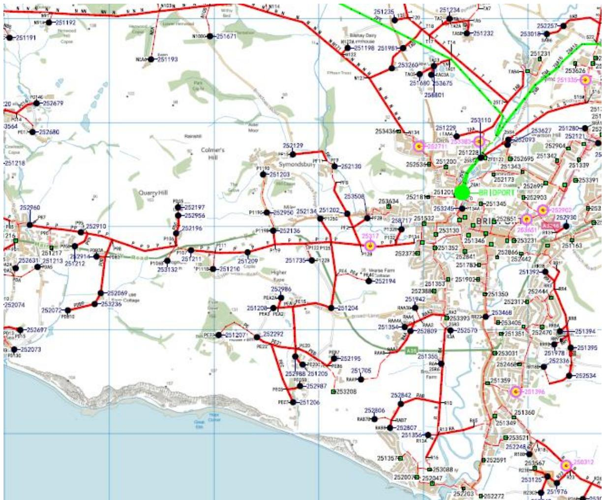
To ensure maximum flexibility in the network, some of the branching circuits connect with other circuits via some form of switch. Usually that switch is off (open) meaning no power can flow between the circuits. However in some circumstances such as faults on the network or maintenance, we may want to join circuits up to change the way power flows. This is done by turning switches on (closed) and connecting the circuits up.
