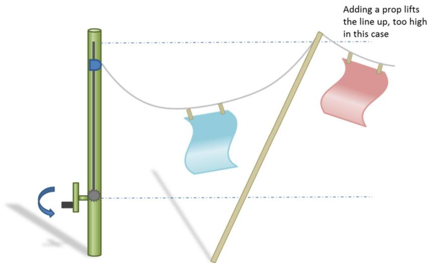
Now imagine the length of this prop can change of its own accord, or even be taken away. Trying to manage the height of the line from the winder alone without full visibility of the line becomes very complex. One solution to this would be to limit the size of the props on the line and cap how many can be used.
