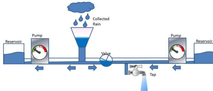
On some areas of our network, joining two circuits up can have a similar problem. Where two circuits meet the voltage on one side of the switch may be considerably higher than on the other. Closing the switch and joining the circuits can cause some instability in the network and in some causes result in network protection devices turning the power off for safety reasons.
