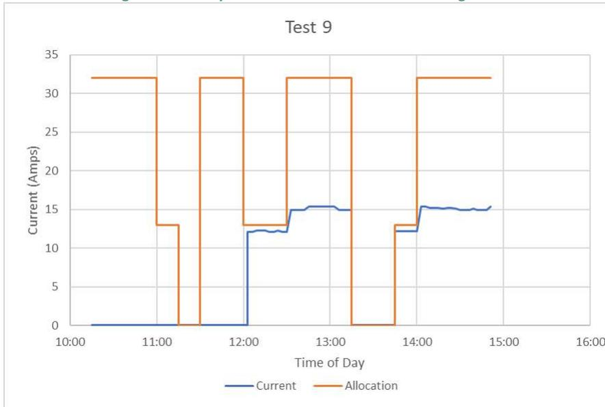
The vehicle was plugged in at 10:15. Charging was paused until 12:00 as expected. The demand limit was followed – for example only charging at 13A from 12:00 until 12:30 and pausing between 13:15 and 14:15.
