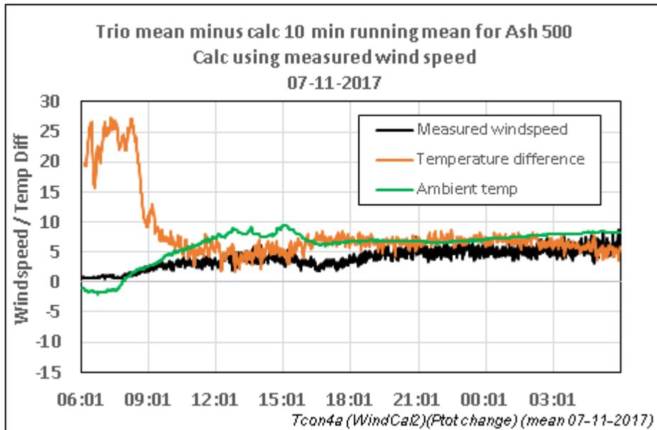
**Figure 13** Trio means minus calculated conductor temperatures (orange) for Ash 500, measured windspeeds (black) and ambient temperatures at line height (green) 7th Nov 2017
