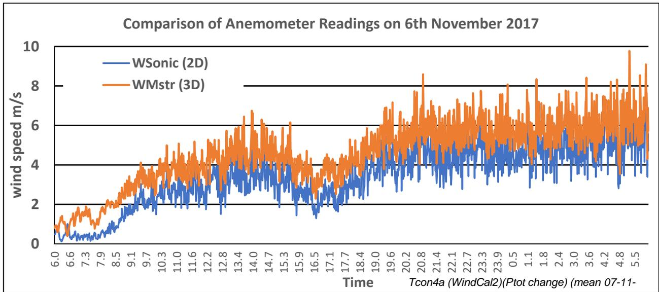
**Figure 16** Discrepancy between the two anemometer readings
