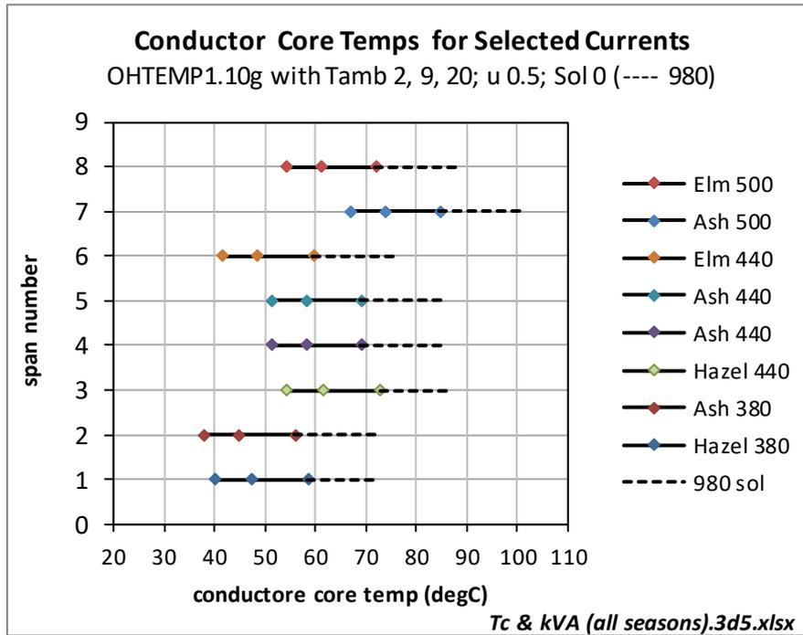
**Figure 18** Rig design values of Tcon from OHRAT
