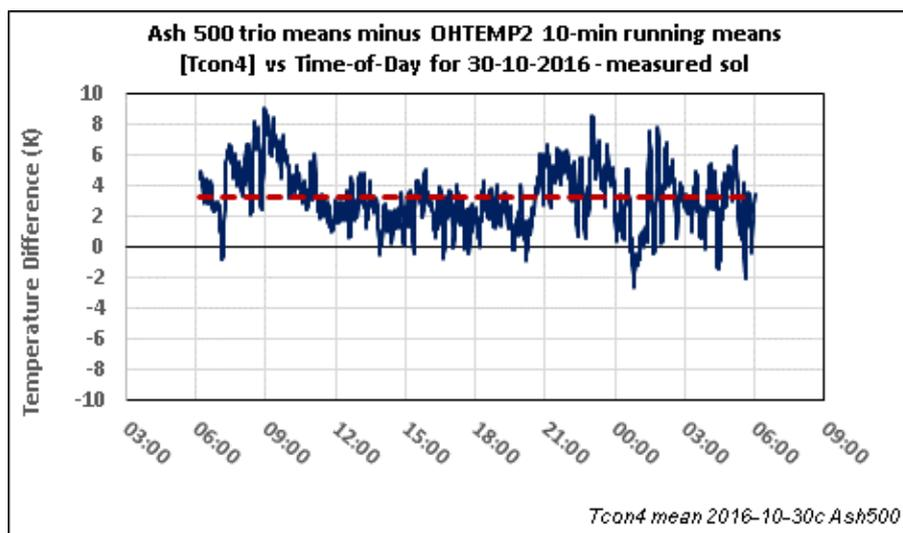
**Figure 12** : 1-minute temperature difference (trio means minus calculated 10-minute running means) for the hottest conductor (Ash500) on a "high-temperature day" (29-30 October 2016)
