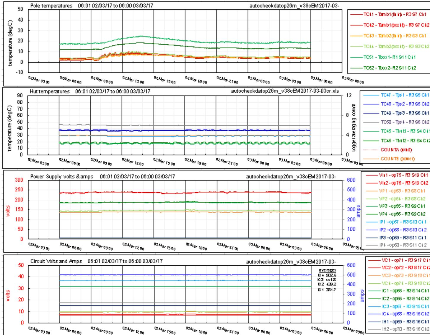
Figure AI.5 "conplot2a" sheet (conductor amps + portacabin temperatures)
