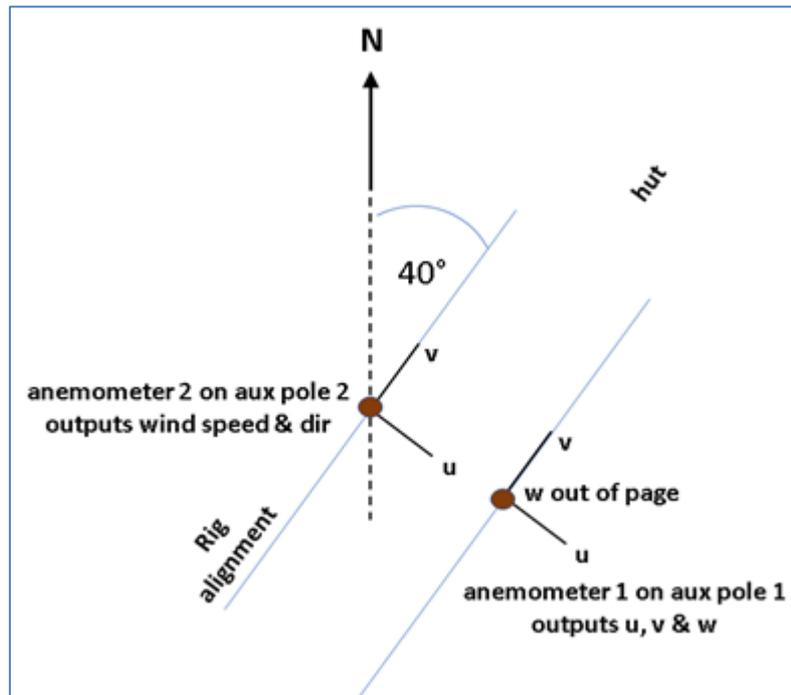
**Figure 5** Diagram of overhead line & anemometer alignments
