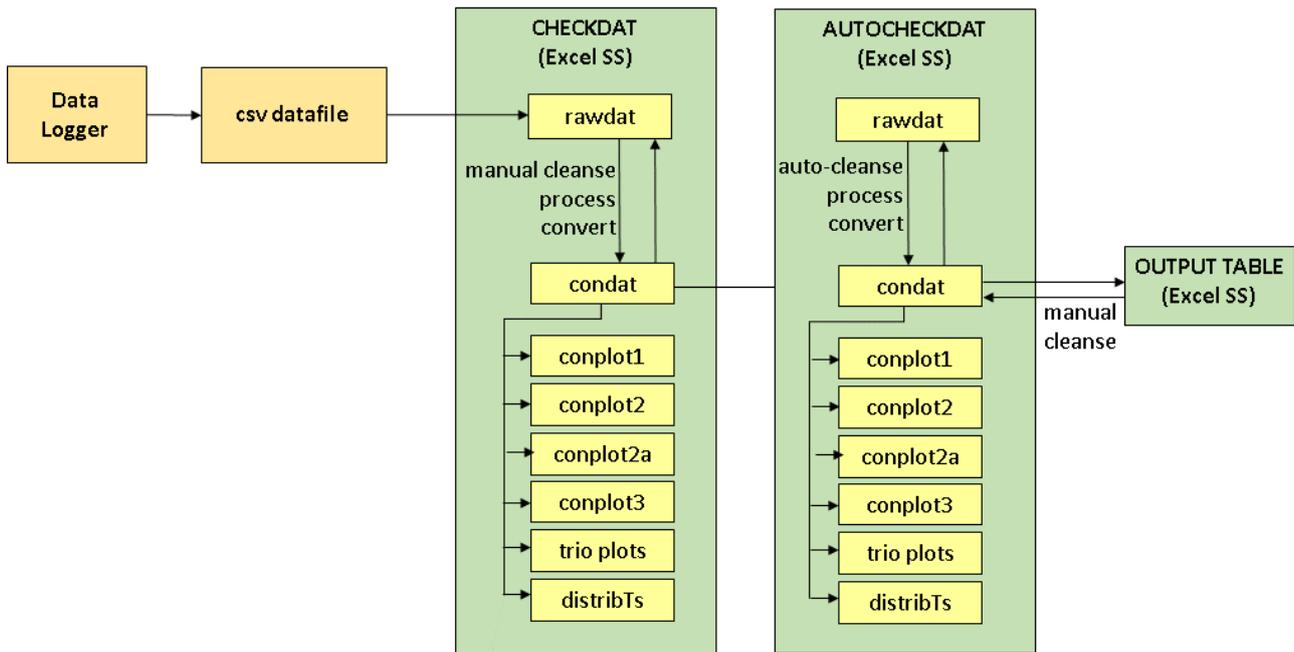
**Figure 10** Flowchart of data handling process to produce cleansed daily datafiles
