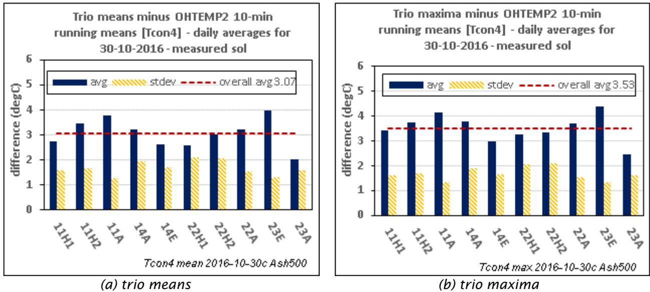
**Figure 11** Difference between measured conductor temperatures and values calculated using OHTEMP2 (CIGRÉ 2014 equations) for a "high-temperature day" (29-30 October 2016)
