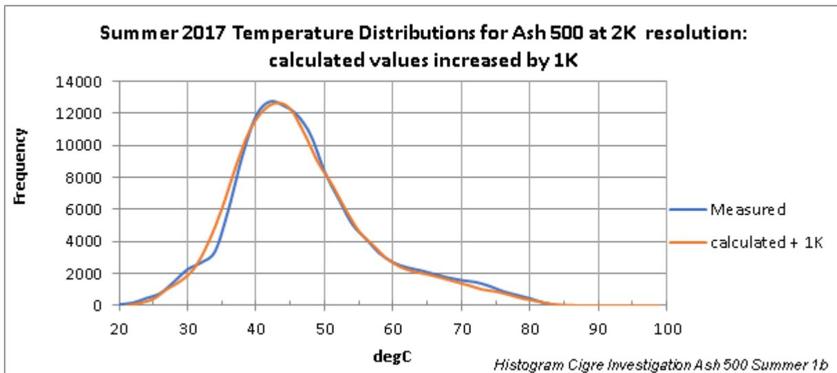
**Figure 15** Same data as Figure 14 but with calculated values increased by 1K
