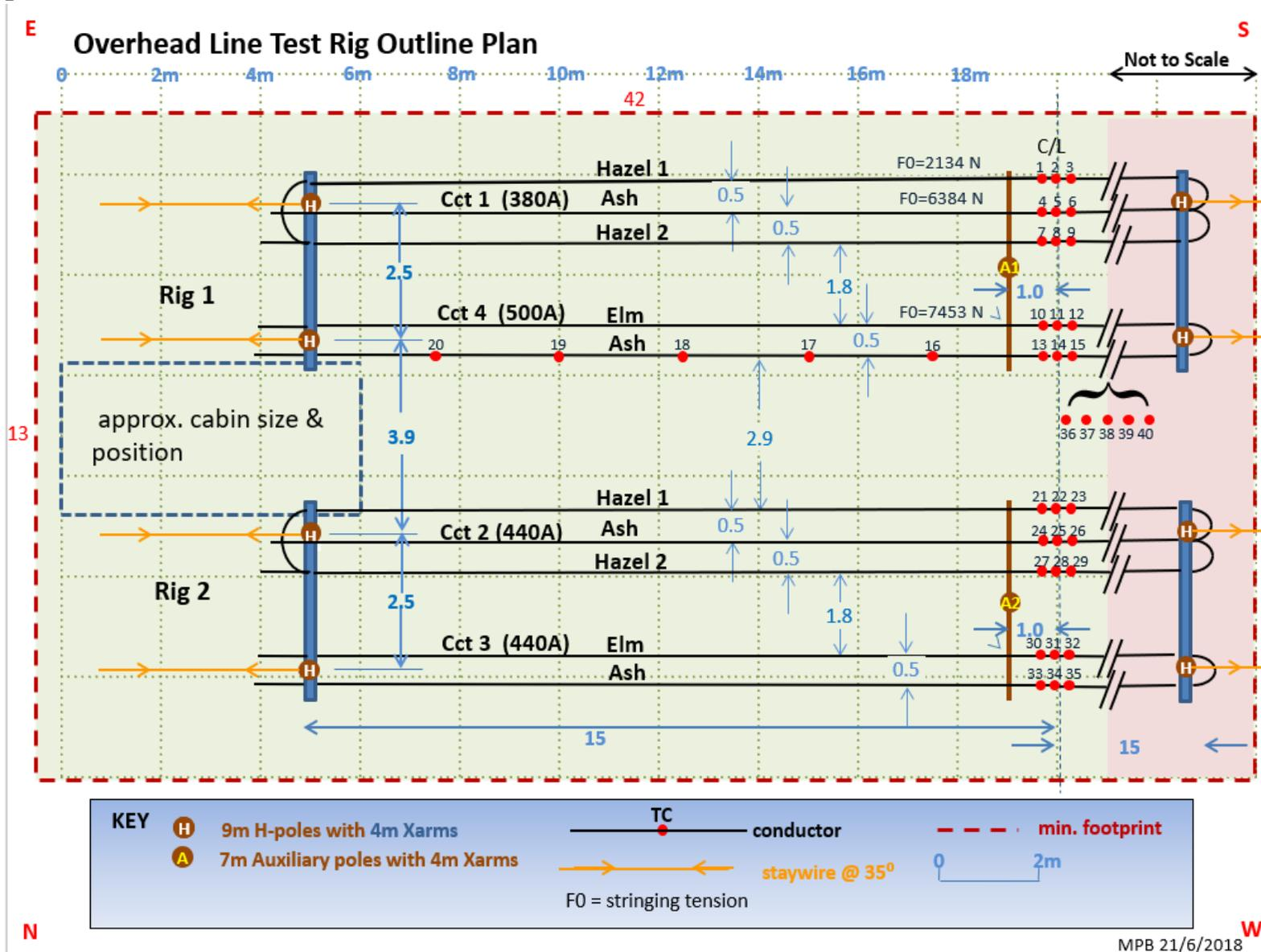
Figure 3 Overhead line test rig plan
