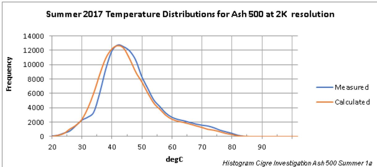
**Figure 14** Frequency Distributions of Measured and Calculated Conductor Temperatures for the 2017 Summer (3 months) for Ash 500
