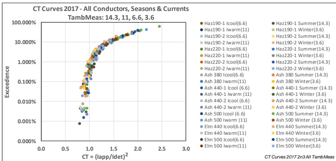
**Figure 30 CT data for all 10 conductor-current combinations. Curves omitted for clarity**
