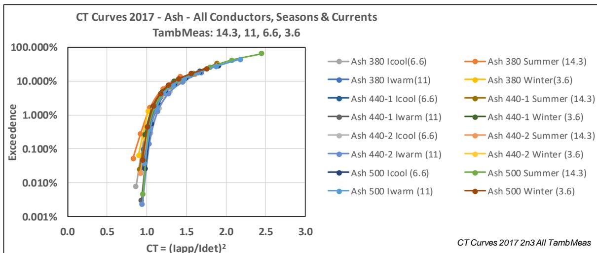
**Figure 29 All the Ash data on single CT plot using measured Tamb as design values**
