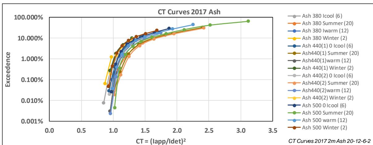
**Figure 23** CT curves for the four Ash conductors based on the provisional design  $T_{amb}$  values given in Table 8 (i.e. Summer 20, Inter warm 12, Inter cool 6, Winter 2)
