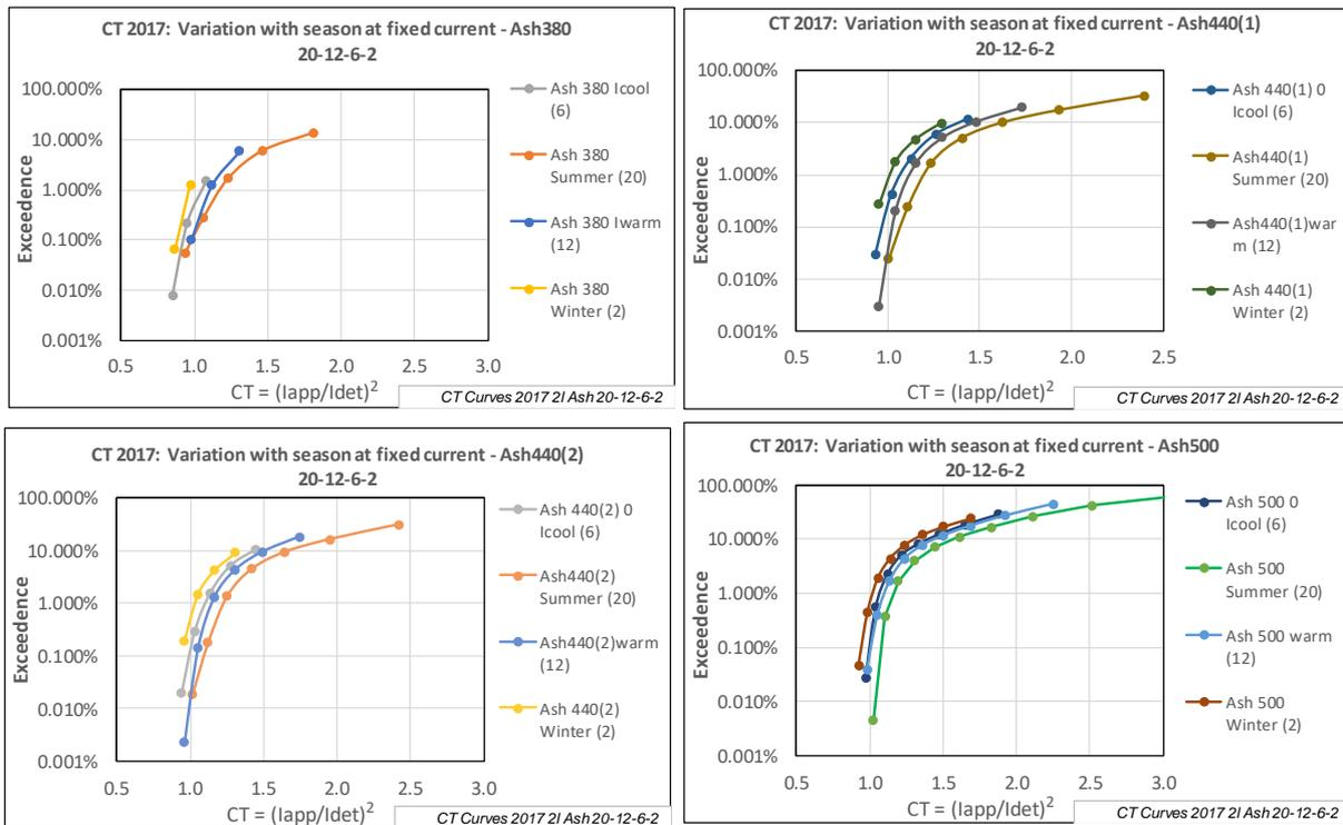
Figure 25 Same data as Figure 23 but with separate plot for each current. The four curves in each plot correspond to the four seasons. (Based on provisional design Tamb: 20-12-6-2)
