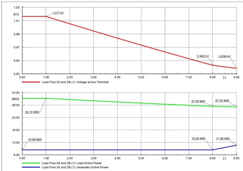
Figure 6-16 – Transformer tap changed from -4 to 4 by CLASS vs ANM reaction
