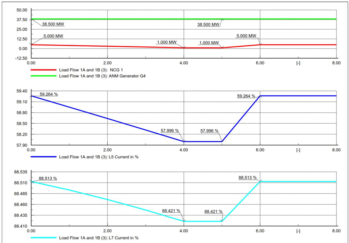
Figure 6-5 - W1: Non-curtailable generator 1 decrement and L6 out of service
