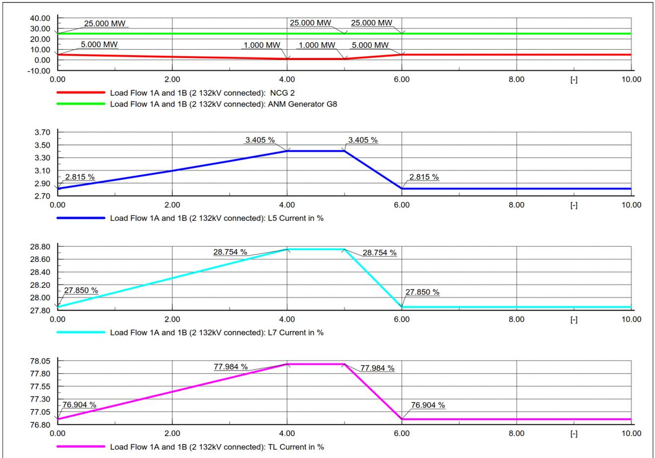
Figure 6-13 - W1: Non-curtailable generator 2 decrement and L1 out of service
