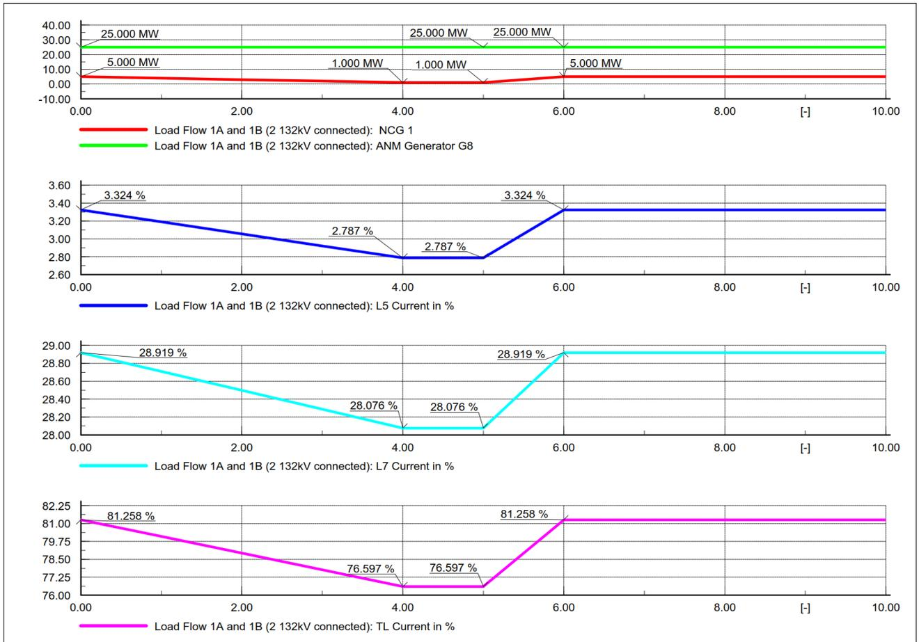
Figure 6-9 - W1: Non-curtailable generator 1 decrement and all cables in service
