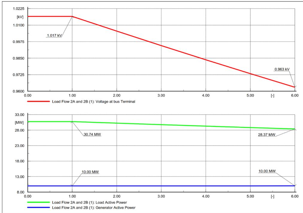
Figure 6-15 – Transformer tap changed from -4 to 1 by CLASS with no ANM reaction
