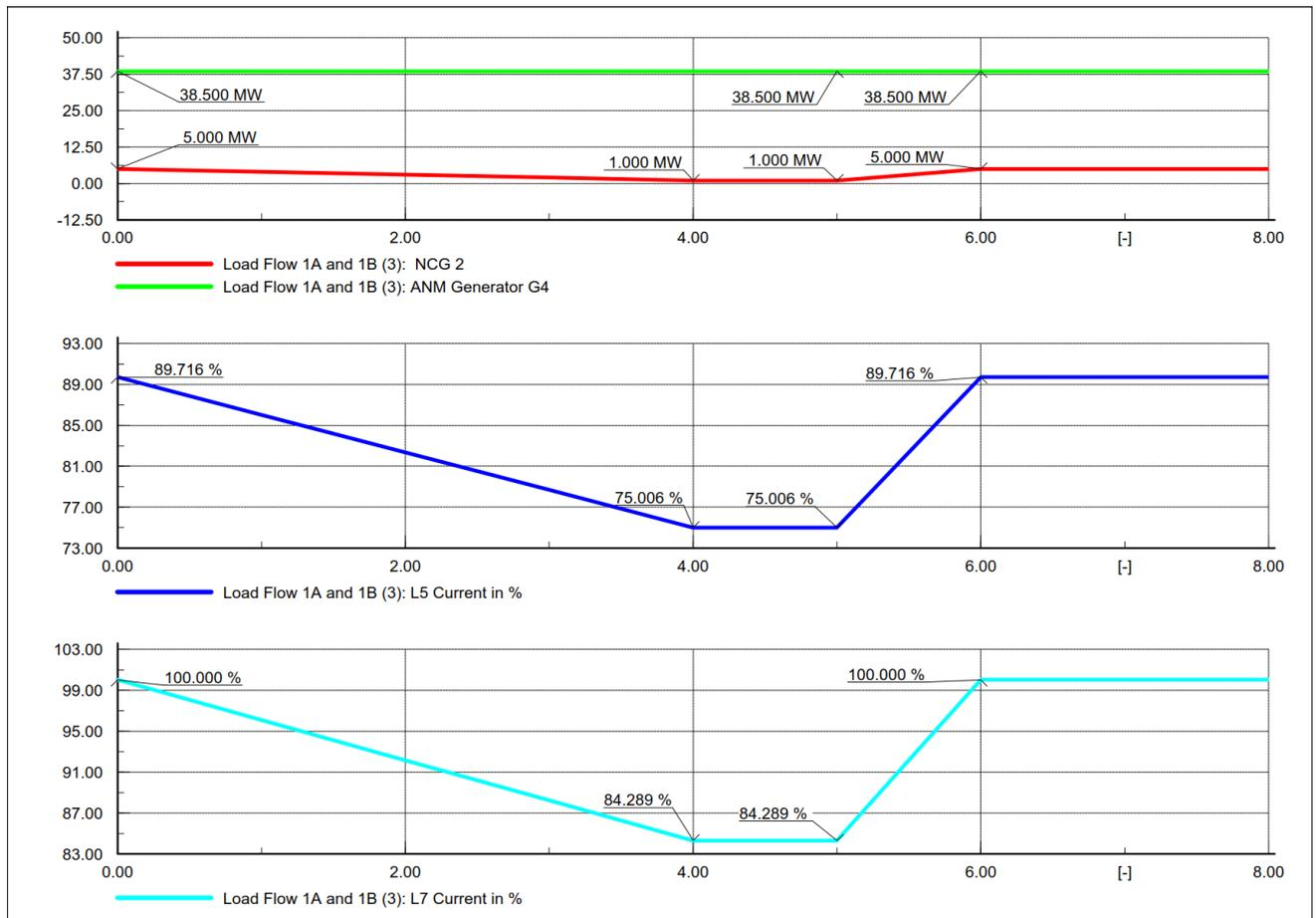
Figure 6-7 - W1: Non-curtailable generator 2 decrement and L1 out of service
