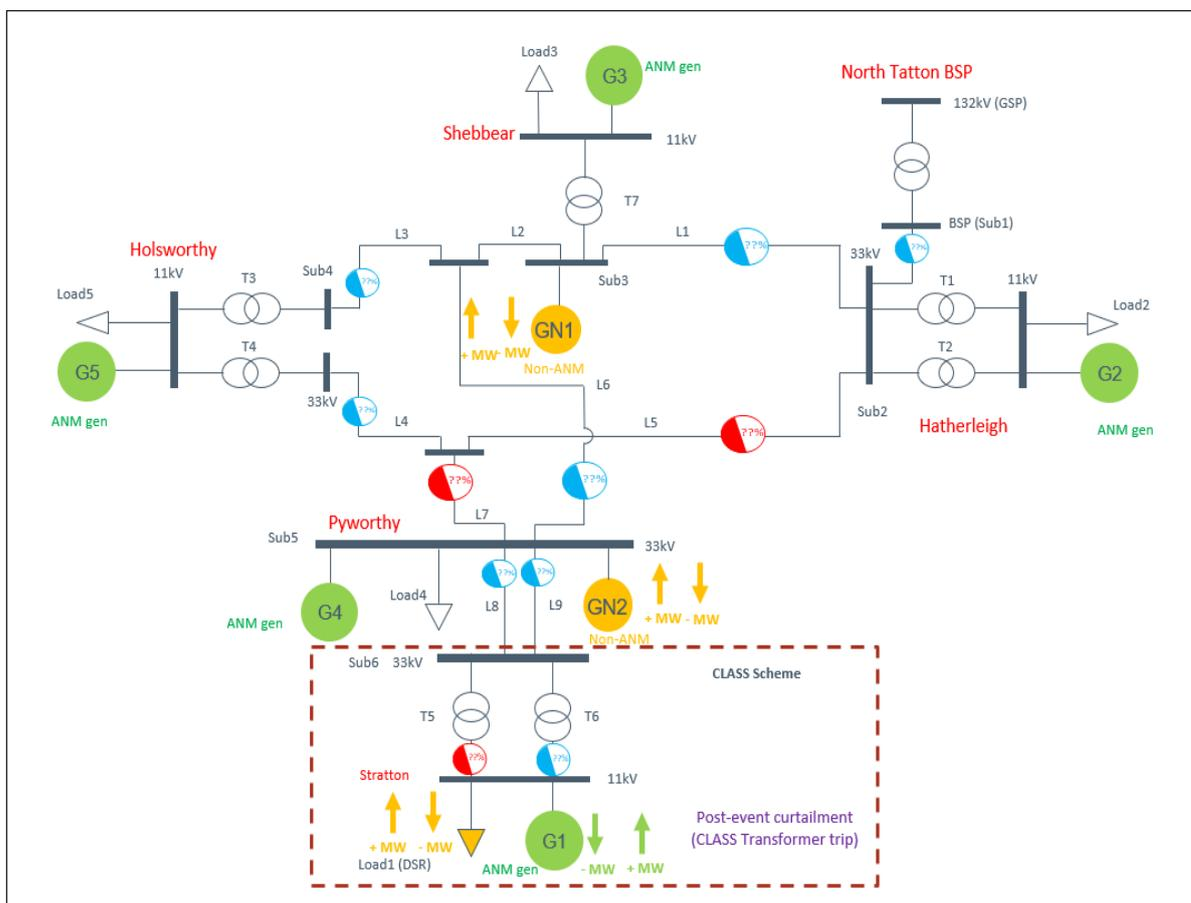
Figure 6-1 – Schematic layout of the test network model
