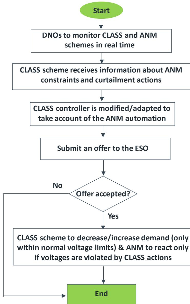
Figure 5-5 - Z2 solution flow chart
