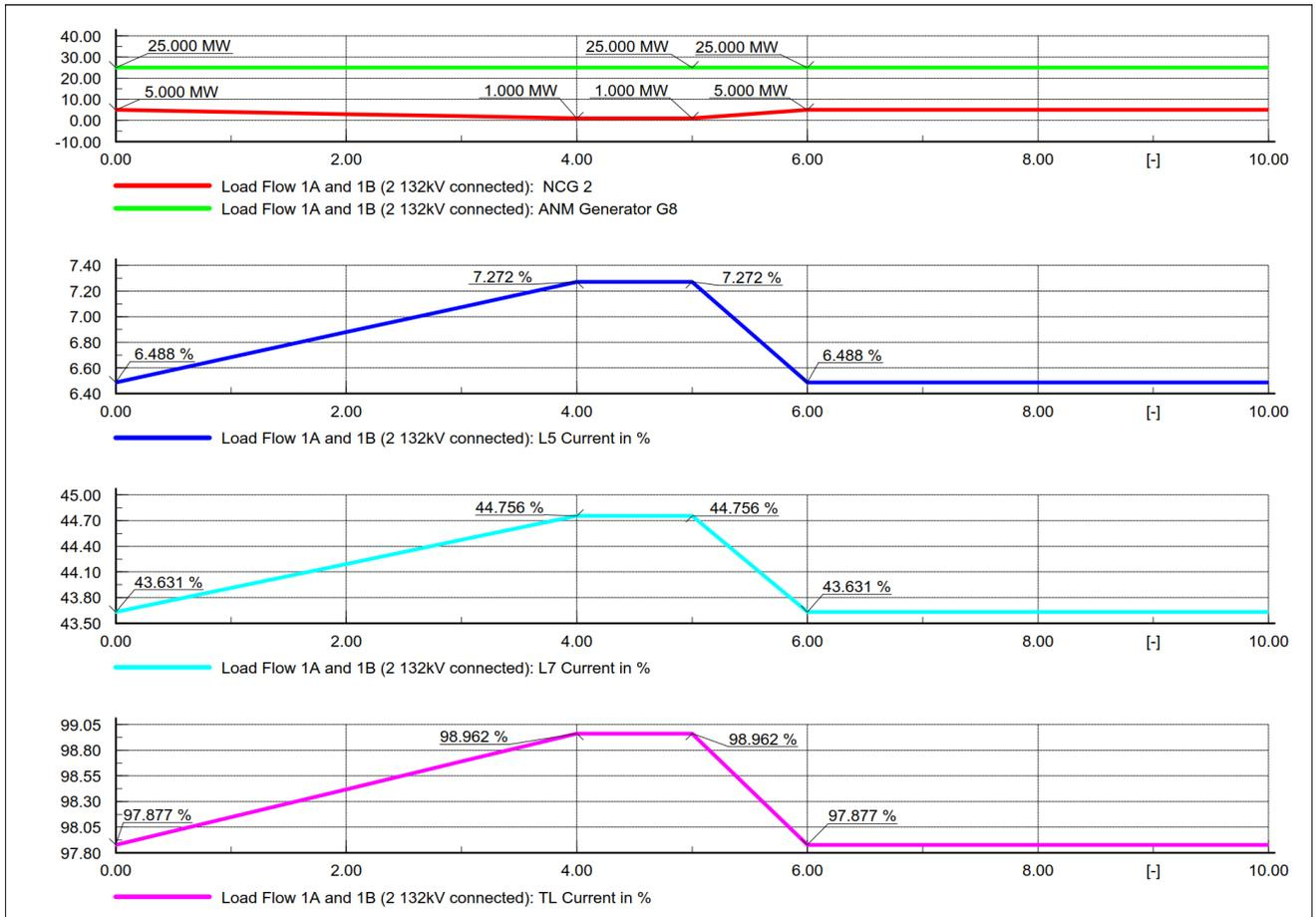
Figure 6-14 - W1: Non-curtailable generator 2 decrement and L6 out of service
