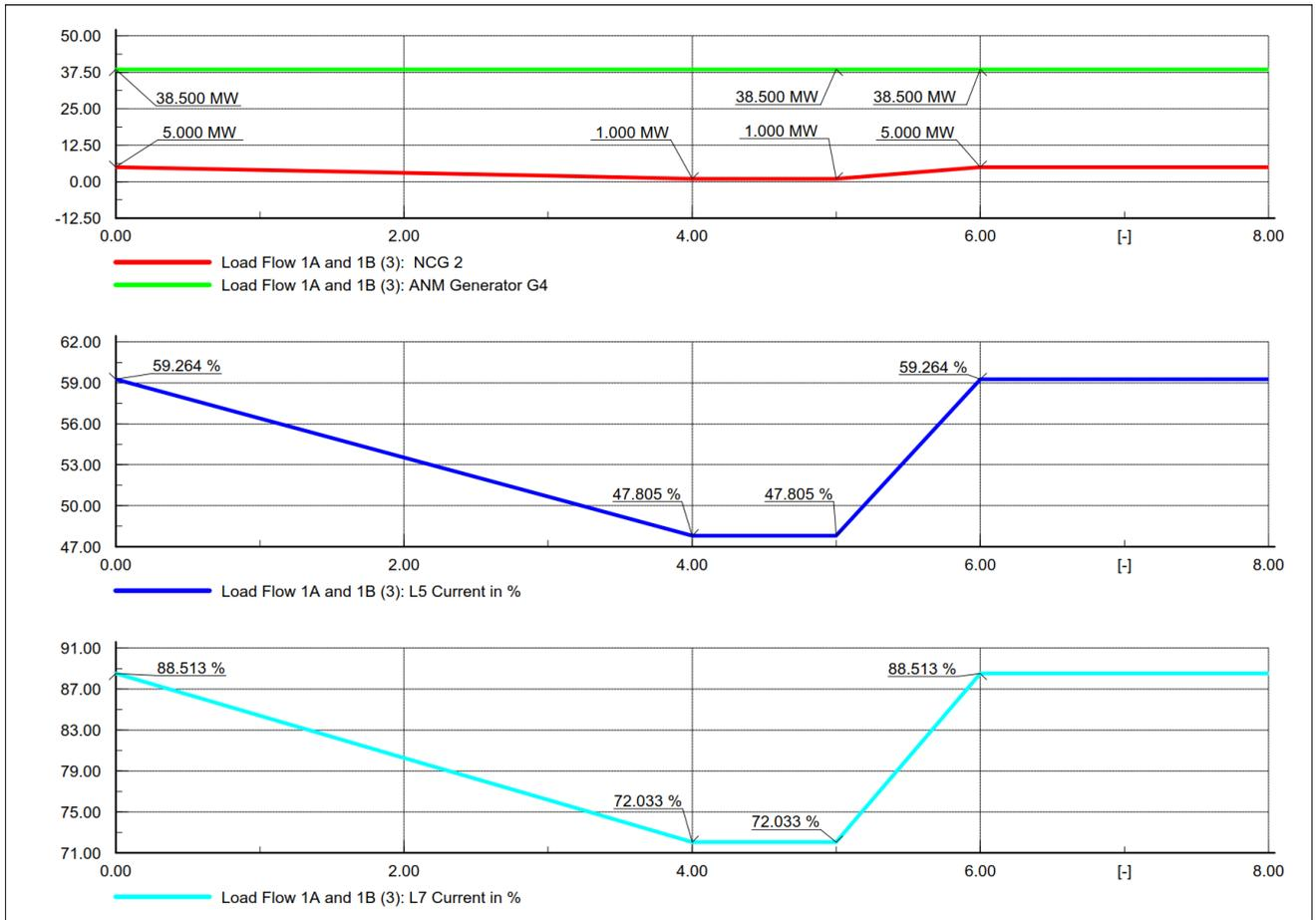
Figure 6-8 - W1: Non-curtailable generator 2 decrement and L6 out of service
