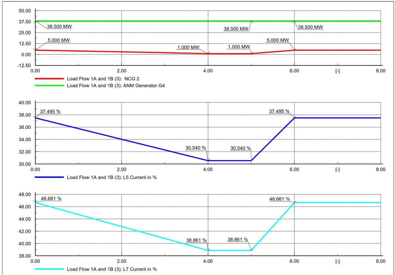
Figure 6-6 - Non-curtailable generator 2 decrement and all cables in service
