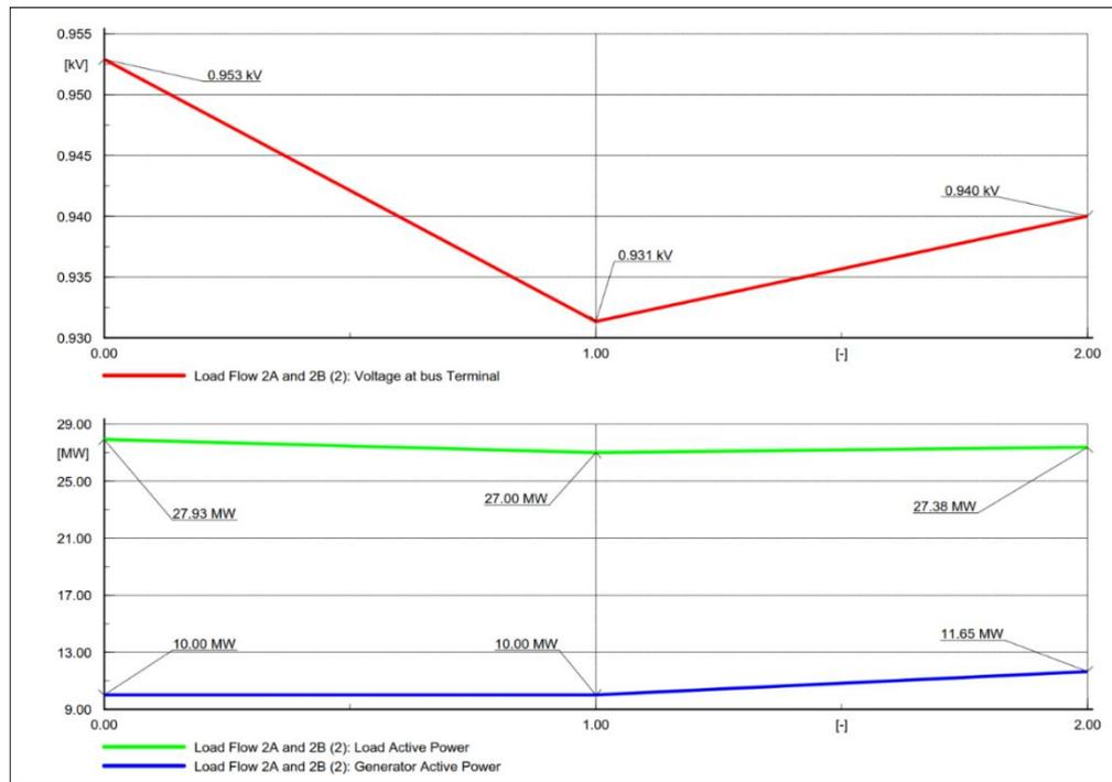
Figure 6-18 - Transformer (T6) taken out of service, initial tap position of 2 with ANM reaction
