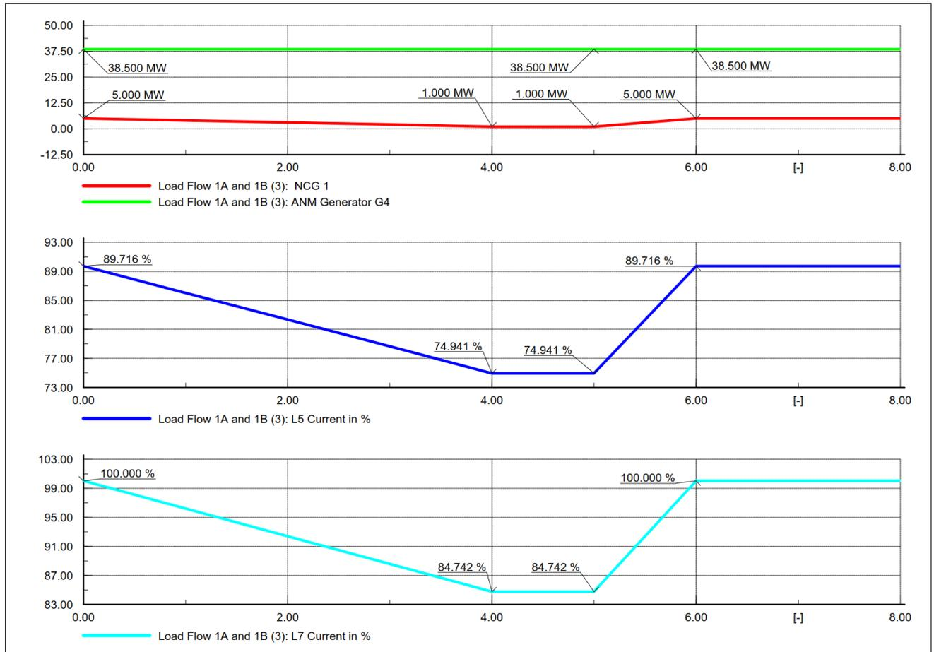
Figure 6-4 - W1: Non-curtailable generator 1 decrement and L1 out of service
