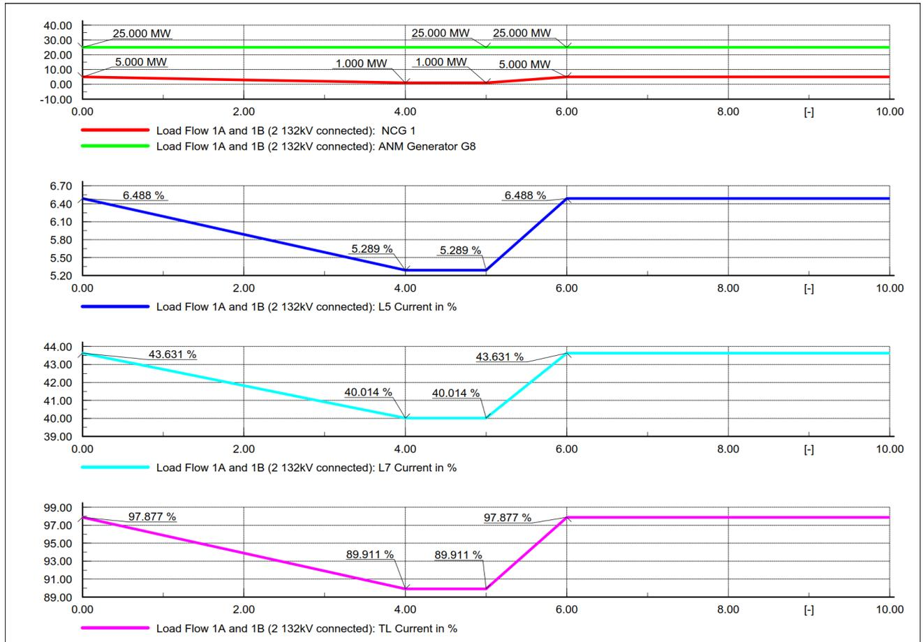
Figure 6-11 - W1: Non-curtailable generator 1 decrement and L6 out of service
