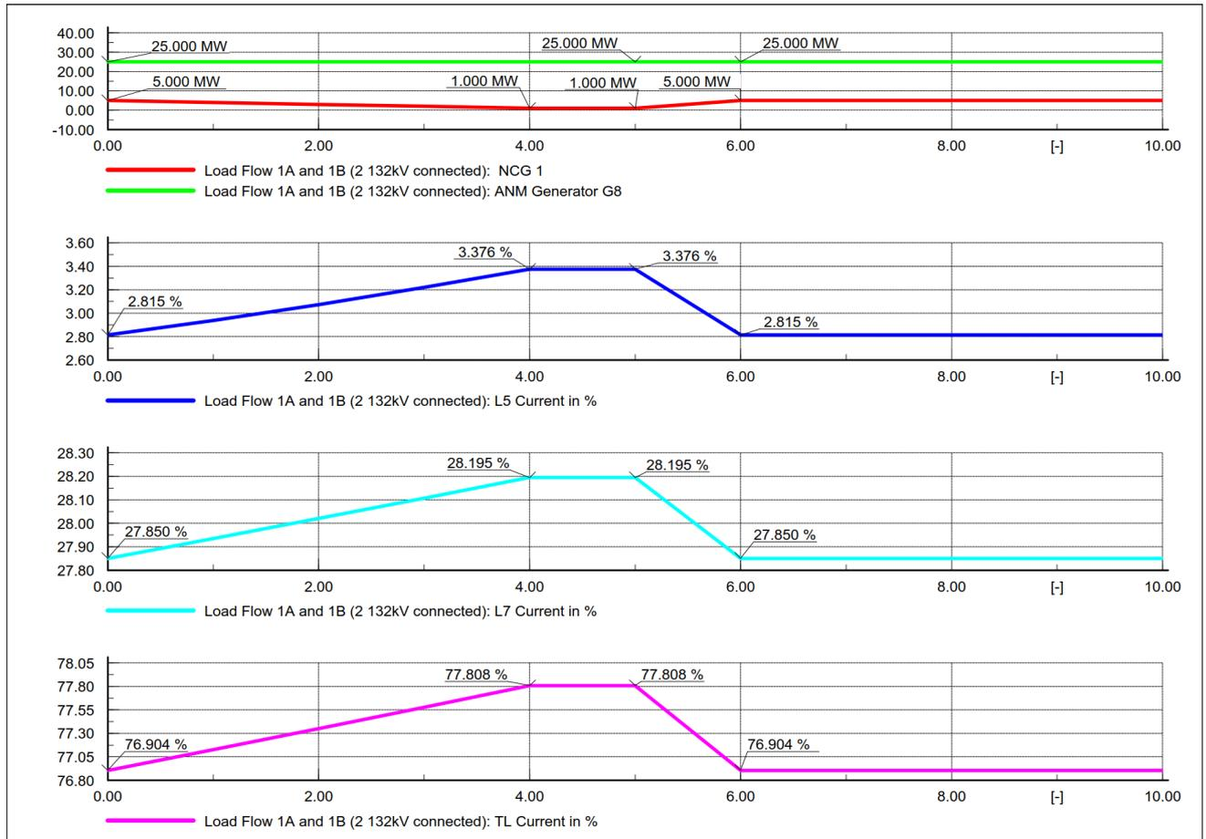
Figure 6-10 - W1: Non-curtailable generator 1 decrement and L1 out of service
