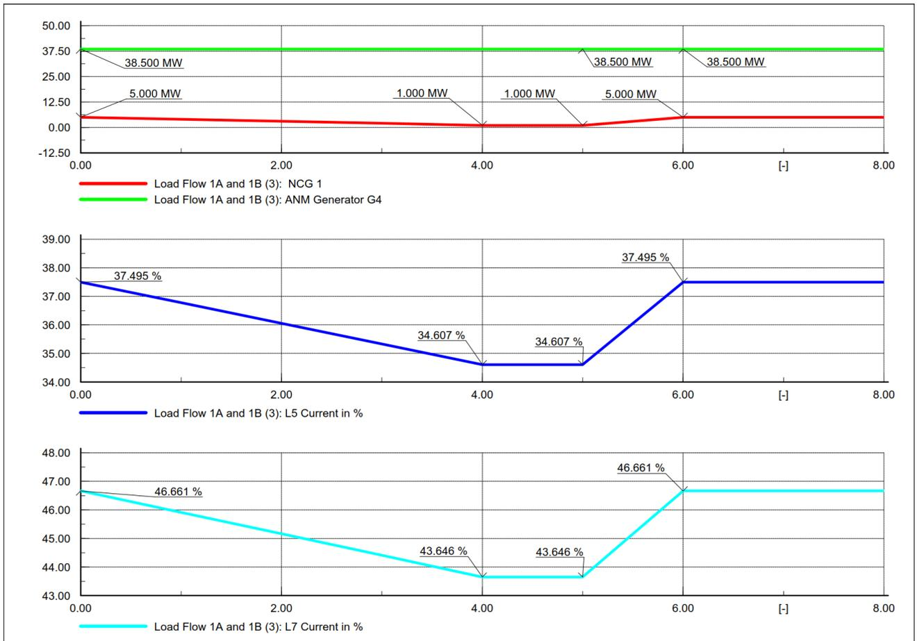
Figure 6-3 - W1: Non-curtable generator 1 decrement and all cables in service
