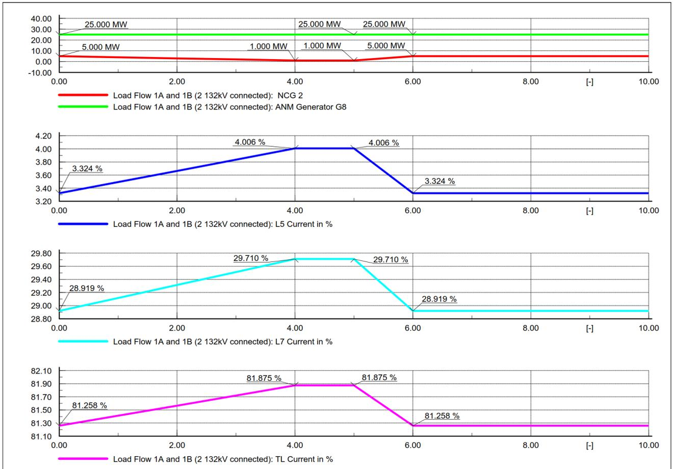
Figure 6-12 - W1: Non-curtailable generator 2 decrement and all cables in service
