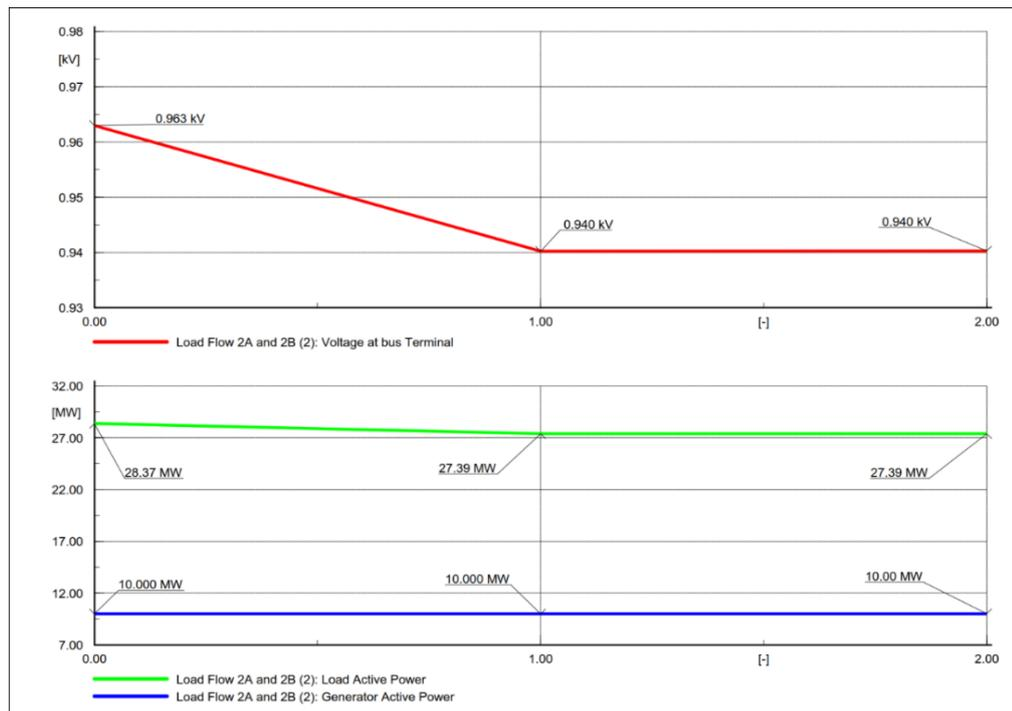
Figure 6-17 – Transformer (T6) taken out of service, initial tap position of 1 with no ANM reaction
