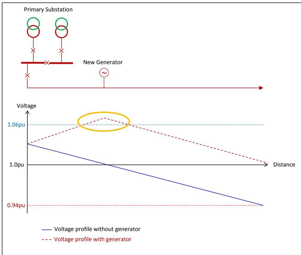
Figure 1-1 - Impact on voltage from new generation connection
