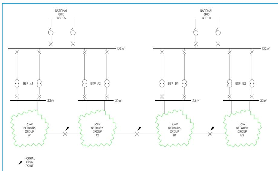
Figure 1-3: Typical Arrangement of a DNO Network
