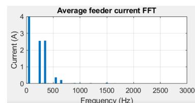
*Figure 1: Feeder current harmonic components without AF operation.*
