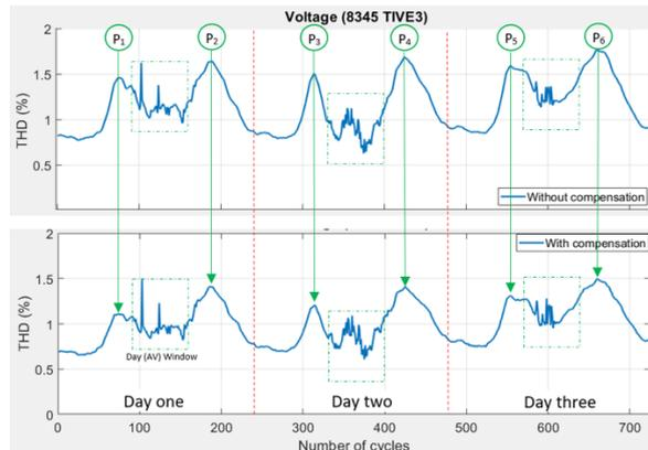
Figure 7: Voltage THD at the BSP without and with AF operation.
