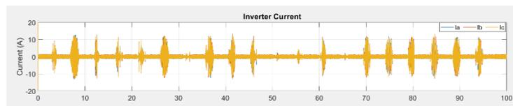
Figure 3: Inverter current, without AF functionality operating (i.e. fundamental PV power conversion only).
