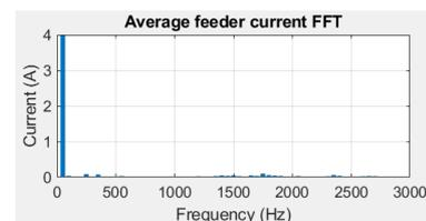
*Figure 2: Feeder current harmonic components with AF operation.*
