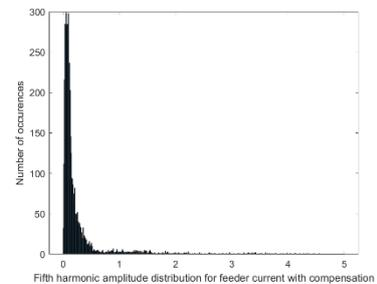
Figure 6: Frequency distribution of 5<sup>th</sup> harmonic current magnitude with AF operation.
