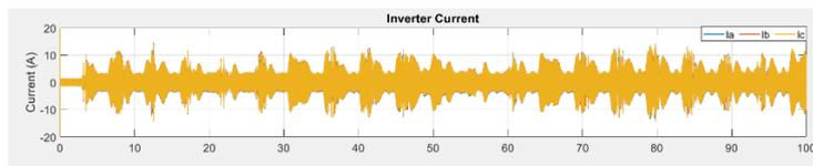
Figure 4: Inverter current with AF operation (i.e. simultaneous fundamental power conversion and harmonic injection).
