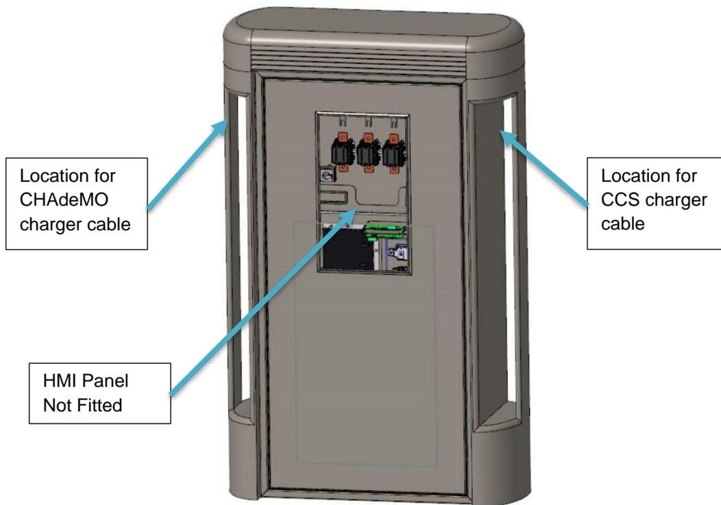
The charger enclosure will be fixed down to the preinstalled base (not shown at present) using M10 stainless steel bolts or similar.
