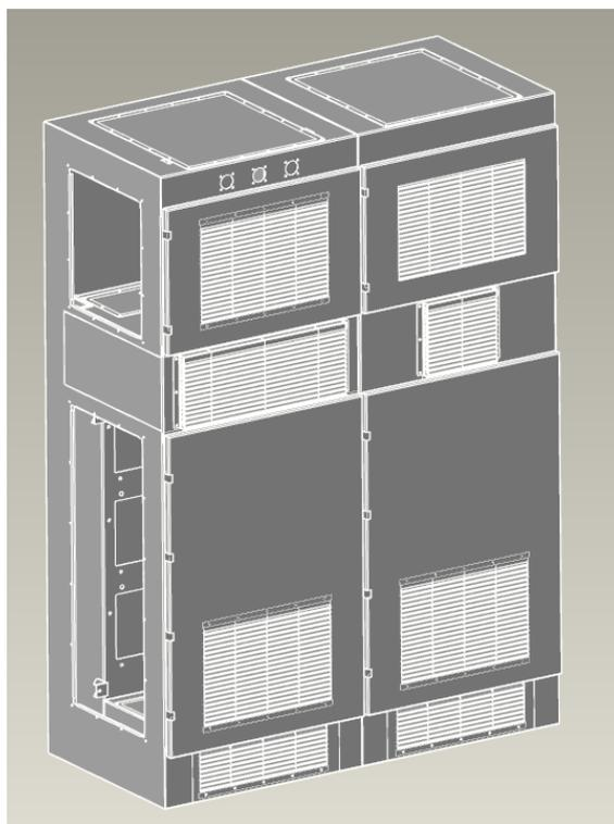
The view in Figure 8 will have blanking-off panel fitted to each end to ensure safety from live parts, and to protect the internal equipment from dust, moisture, and vermin.
