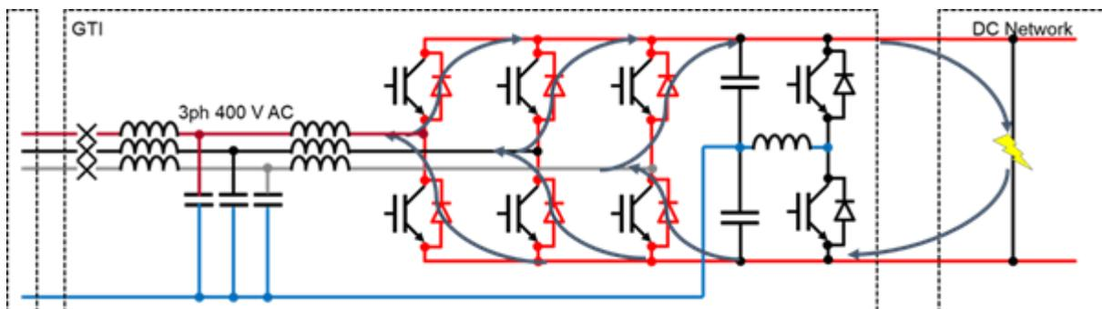
In the Soft Open Point (SOP) back-to-back converters, the DC bus is internal to these devices, very short and protected by the mechanical structure of the device. The risk of a DC fault is low so therefore no DC protection scheme was required and a circuit breaker on the input AC side can
