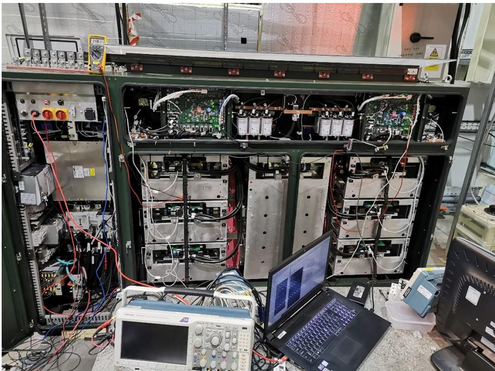
GTI is a connection of both projects. Power modules are from 2T and they are placed in 3T cubicle. As a result, we have 250KVA converter designed as an indoor device.
