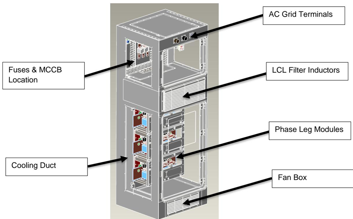
The view in Figure 6 shows the enclosure with the front cover fitted. The sides of the enclosure are open for the DC link bus bar (and other signal power wiring) to connect through to the other enclosures. The bolted together combined enclosure ends top and bottom openings will be closed off with external covers to protect against live terminals.
