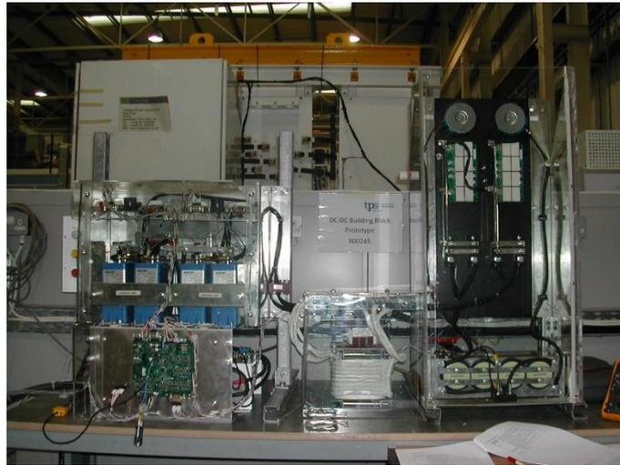
Figure 18: Resonant DC-DC Converter 2020 (utilising FUN-LV GTI)
