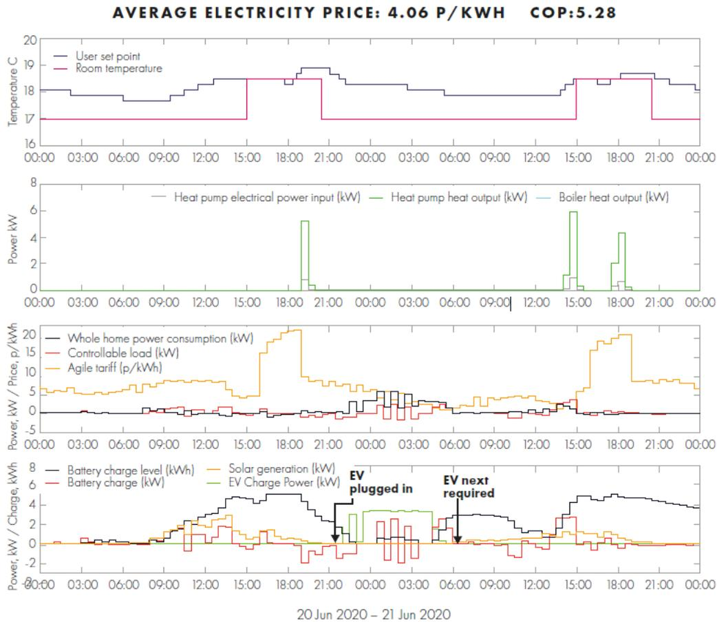
Figure 10: Fully coordinated control on the Octopus Agile tariff (Home 01, 20/06/2020 - 21/06/2020)
