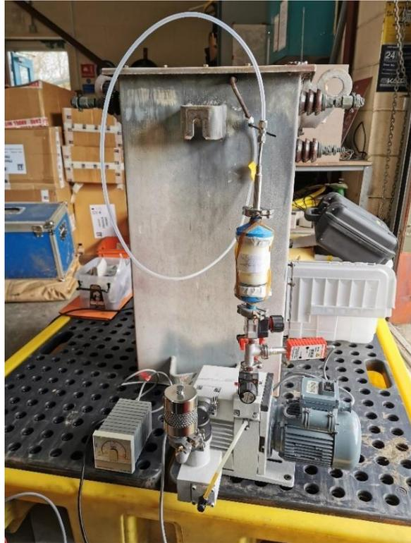
Fig.8 Experimental setup using a test transformer with ~50 ppm PCB contamination.
