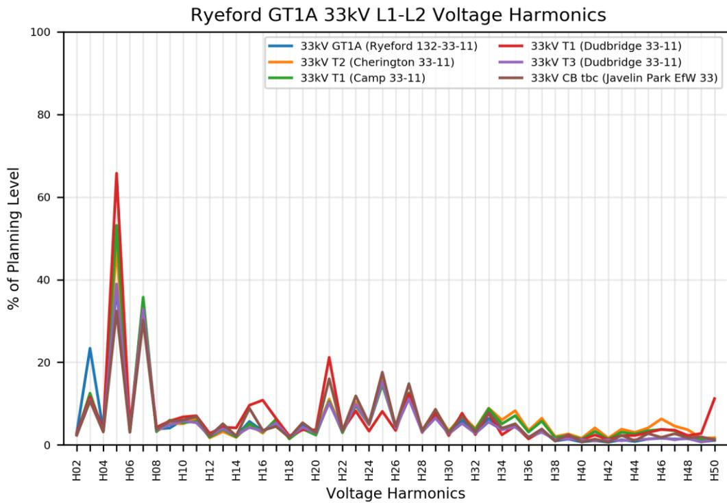
Figure 2-2: 95<sup>th</sup> percentile aggregate voltage harmonic values for the Ryeford (GT1A) 33 kV sites calculated using all available data
