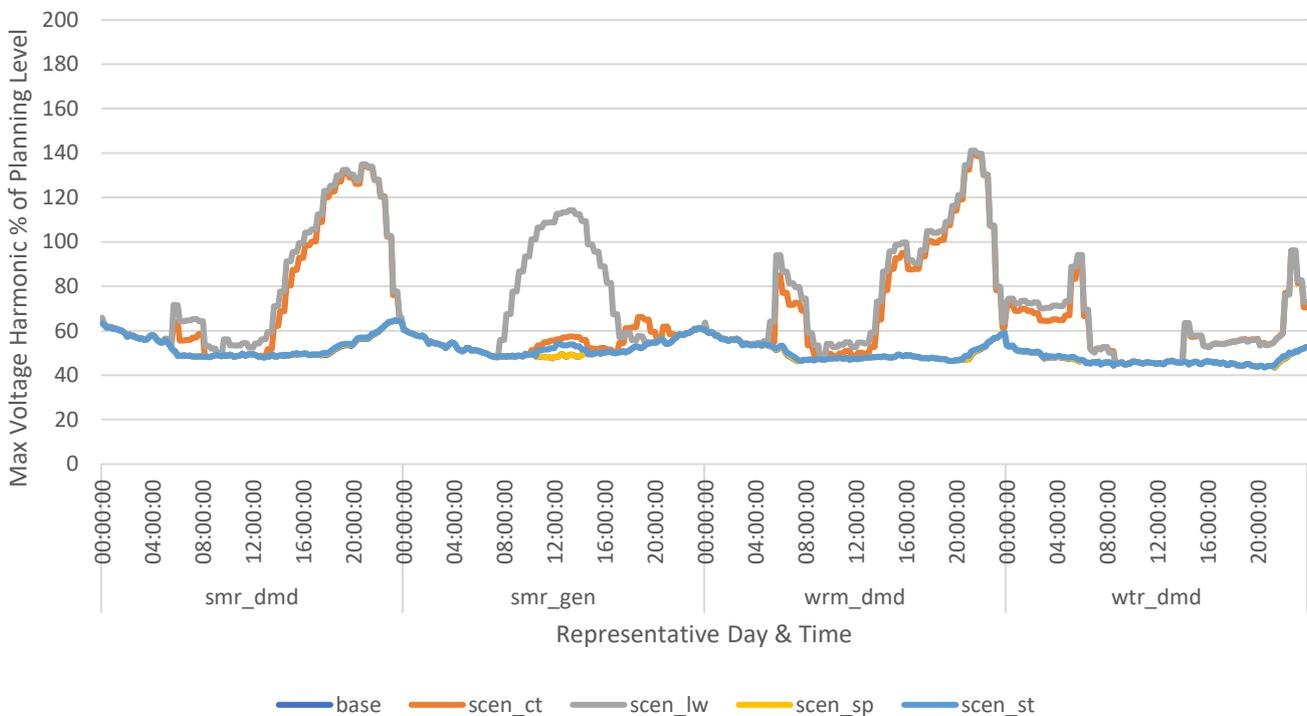
Figure 2-7: Estimated maximum harmonic voltages for the 2030 scenarios in the Meaford C 33 kV network
