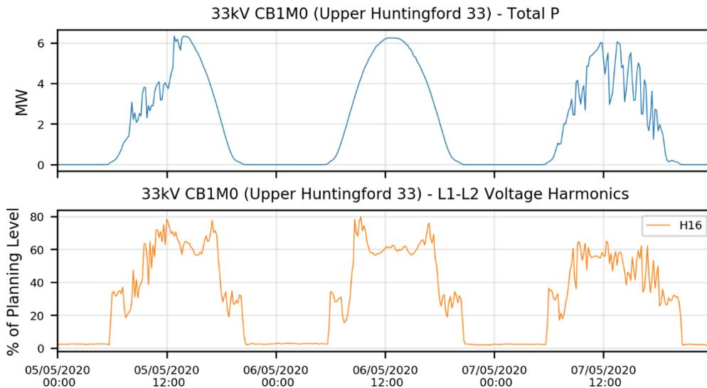
Figure 2-4: Power output and the 16<sup>th</sup> harmonic voltage at Upper Huntingford solar over 3 sunny days
