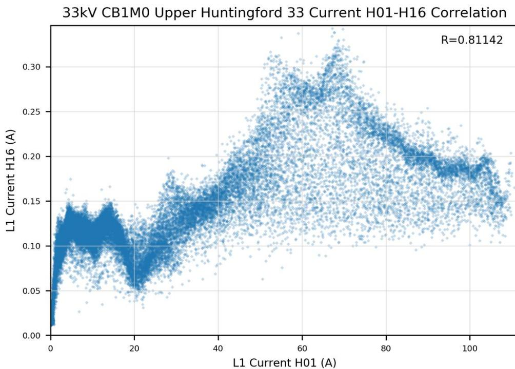
Figure 2-5: Scatter plot of fundamental current vs. 16<sup>th</sup> harmonic current for Upper Huntingford solar farm using approximately a year of data gathered at 10 minute intervals
