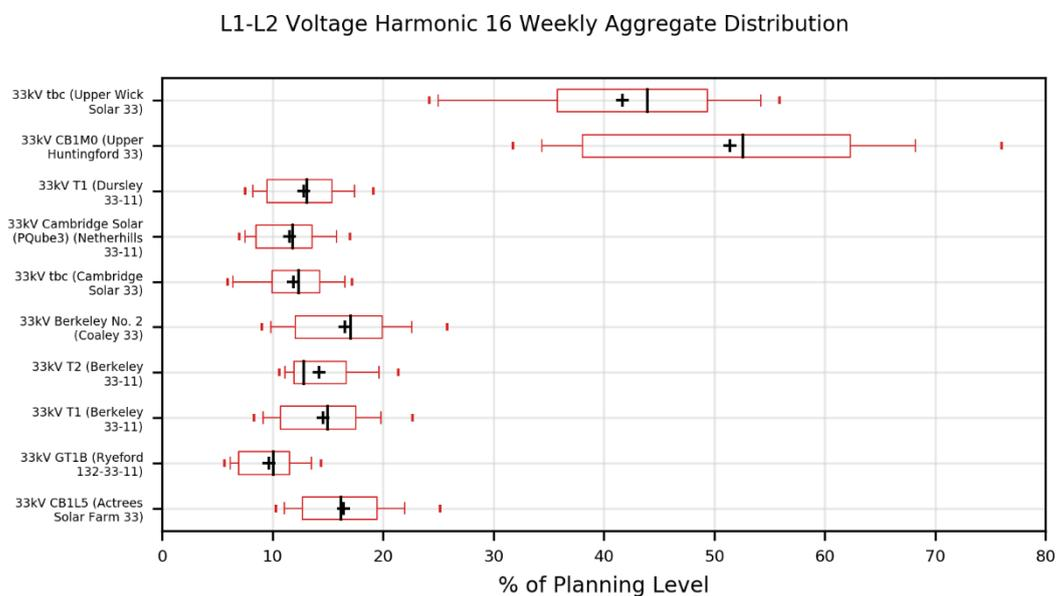
Figure 2-6: Box plot showing the distribution of 16<sup>th</sup> harmonic voltage weekly aggregates for the Ryeford (GT1B) 33 kV sites
