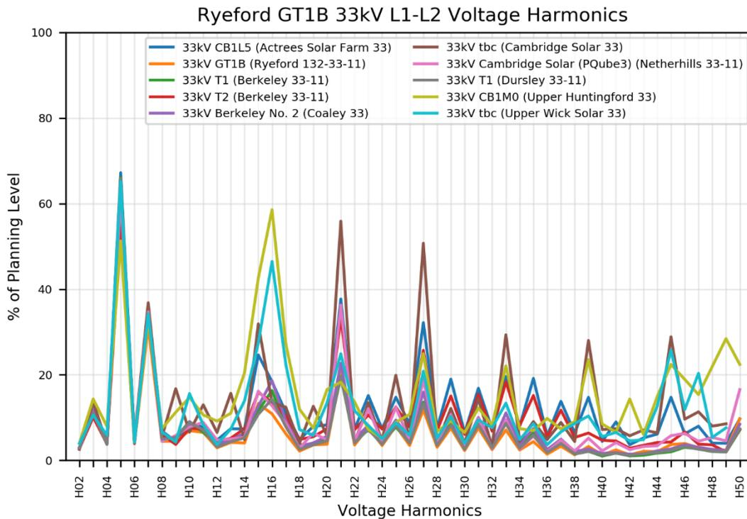
Figure 2-3: 95<sup>th</sup> percentile aggregate voltage harmonic values for the Ryeford (GT1B) 33 kV sites calculated using all available data
