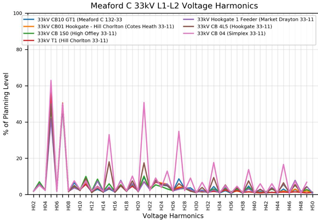
Figure 2-1: 95<sup>th</sup> percentile aggregate voltage harmonic values for the Meaford C 33 kV sites calculated using all available data
