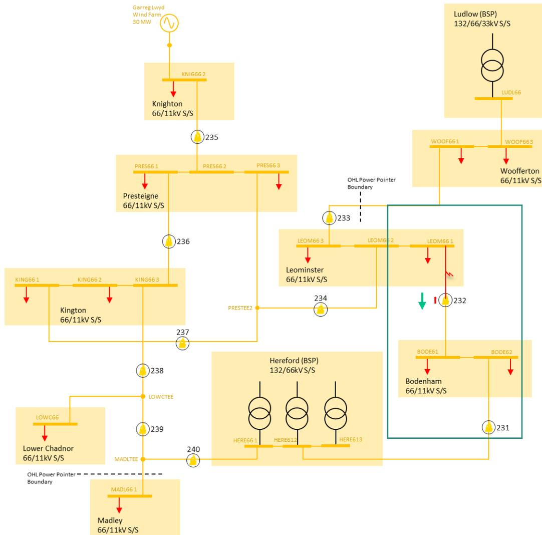
**Figure 2-2 – Directional fault passage indication on the Hereford 66kV network**
