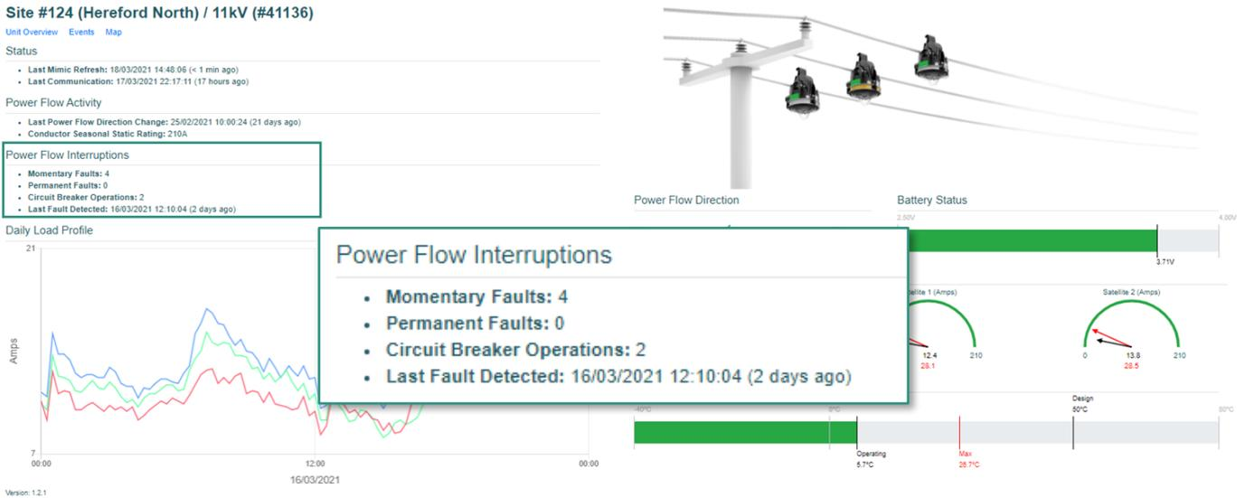
**Figure 2-1 – Power Flow Interruptions presented on the Smart Navigator 2.0 dashboard**
