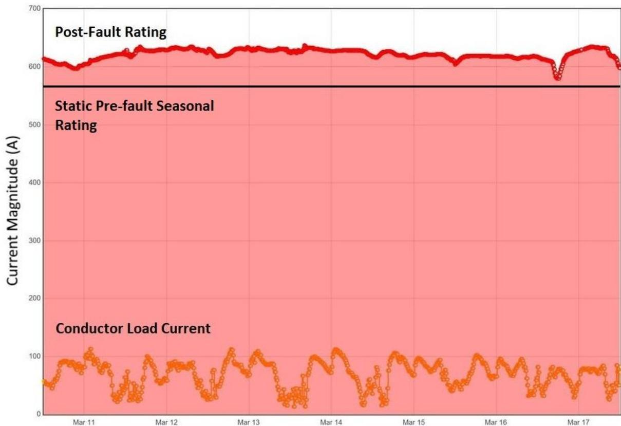
**Figure 2-3 – Post-fault rating determined at trial site #241 (132kV K-Line)**
