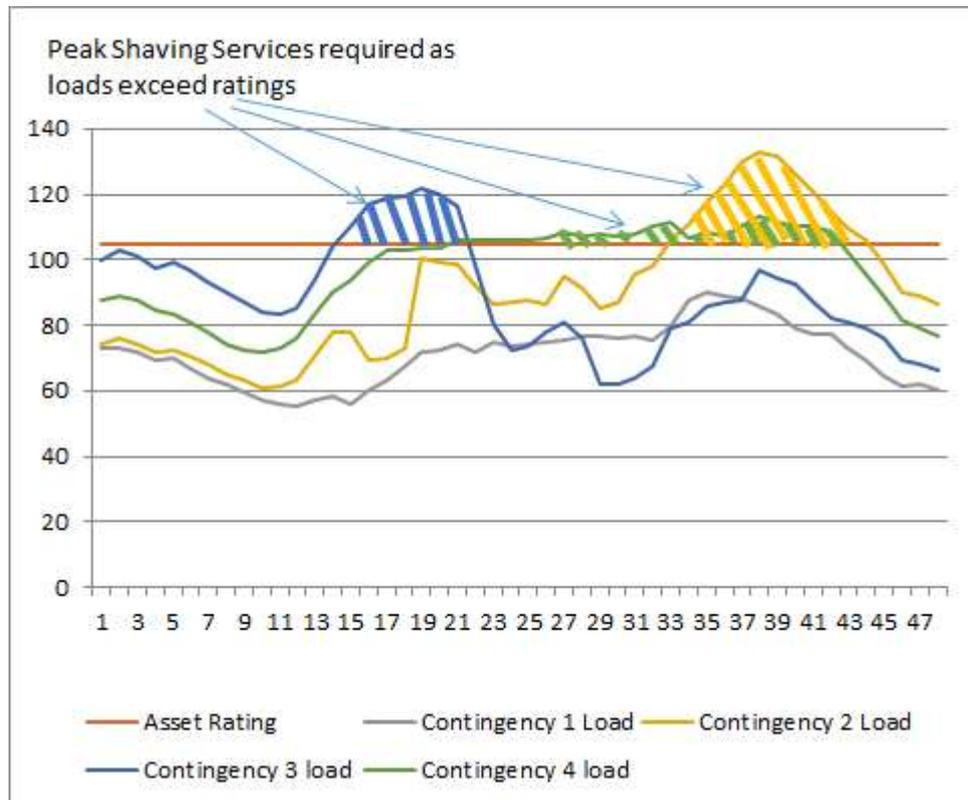
Different contingencies reflect different network configurations, and this means that the flexibility service that is required to resolve issues under one contingency scenario might make the issues under a different contingency scenario worse.
