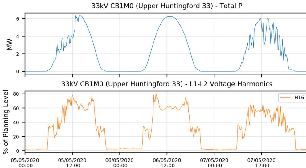
Figure 5-45: Time series plot of power and voltage harmonic H16 at Upper Huntingford solar for three sunny days in May 2020
