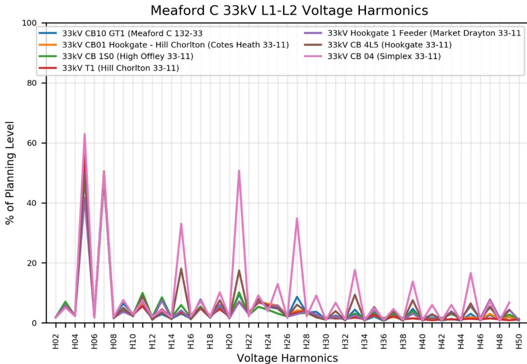
Figure 5-44: Overall voltage harmonic aggregates for Meaford C 33 kV sites
