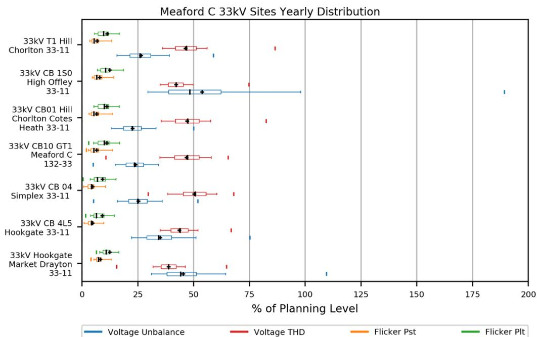
Figure 5-57: Box plot showing distribution of all non-harmonic PQ measurements for Meaford C 33 kV sites
