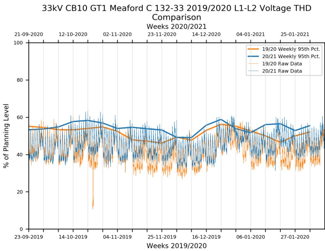
Figure 5-55: Year-on-year comparison of voltage THD for Meaford C 33 kV substation (GT1)
