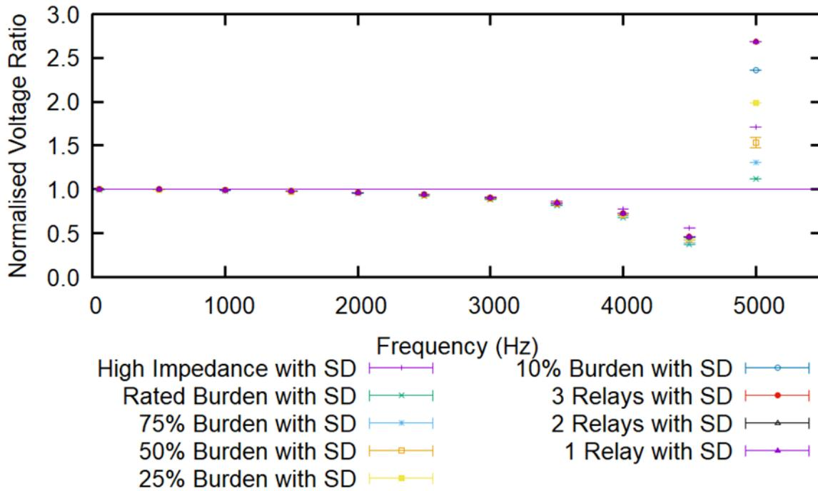
Figure 5-6: Ratio of secondary to primary voltage for phase 3 on VT #2, for various frequencies and burdens. The horizontal line shows the nominal ratio.
