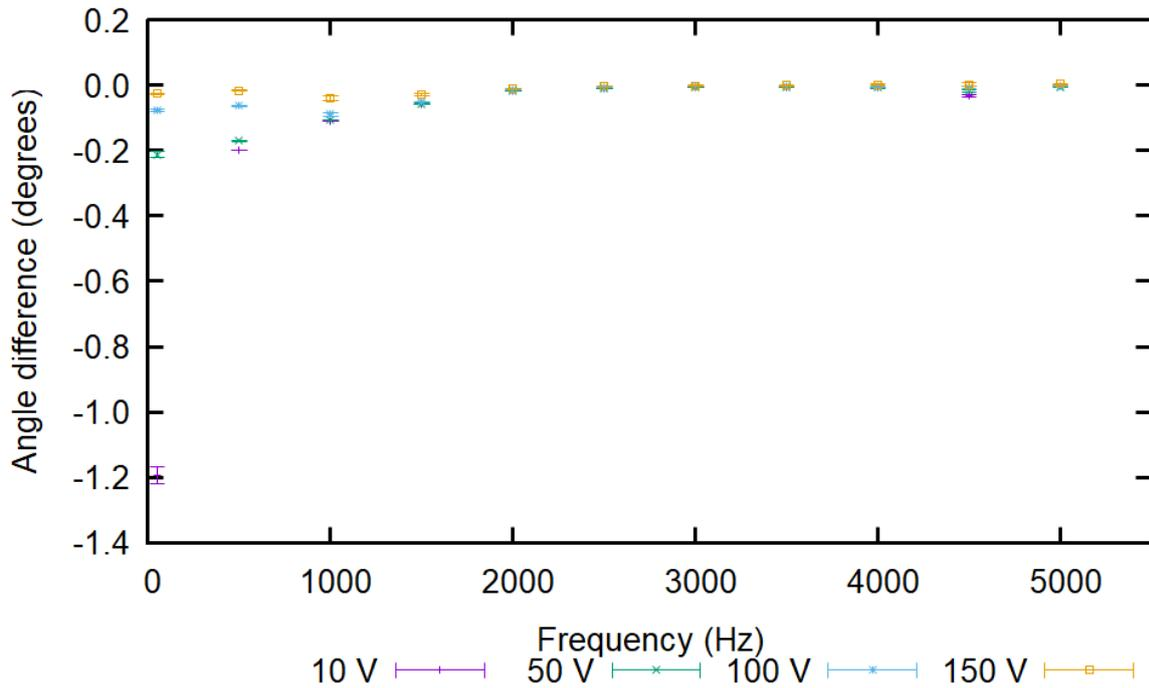
Figure 5-13: Comparison of phase angle difference between secondary and primary voltage for phase 3 of VT #2 to 200V, for various applied primary voltages.
