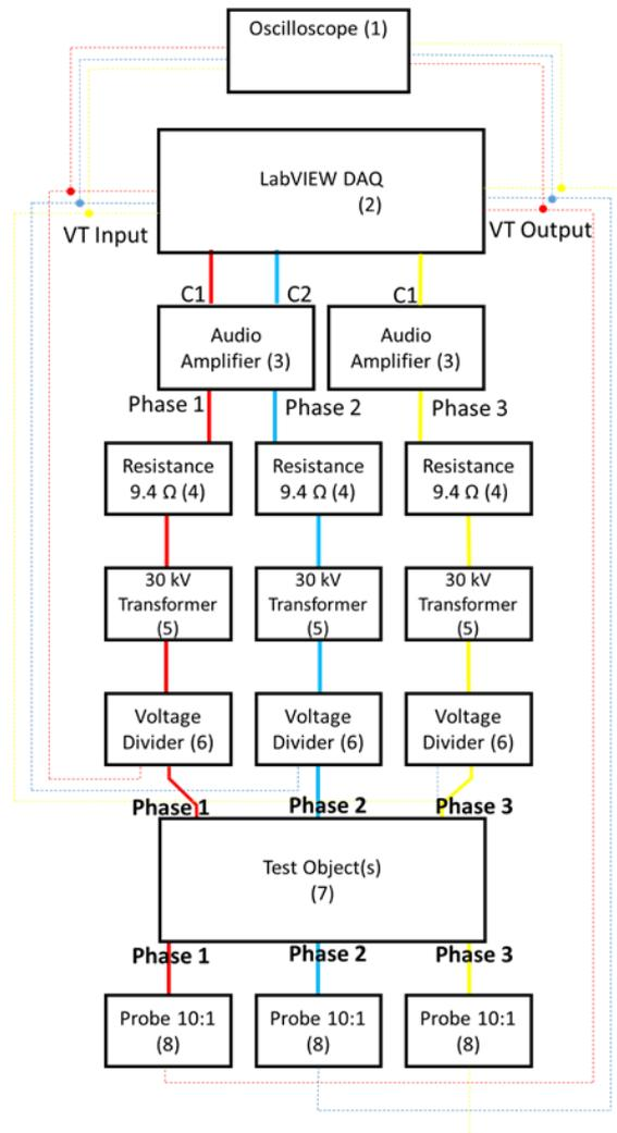
Figure 5-1: Test circuit used for VT testing at The University of Manchester
