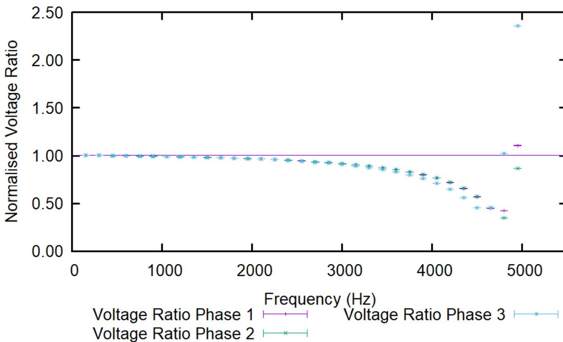
Figure 5-11: Ratio of secondary to primary voltage for VT #2, for various triplen frequencies.
