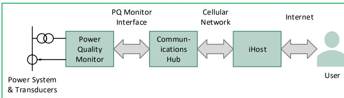
Figure 5-23: Summary of overall architecture for PNPQA PQ monitoring and communication.
