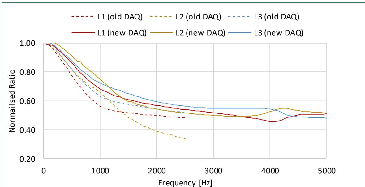
Figure 5-2: Magnitude frequency response of the 11 kV 3-ph VT
