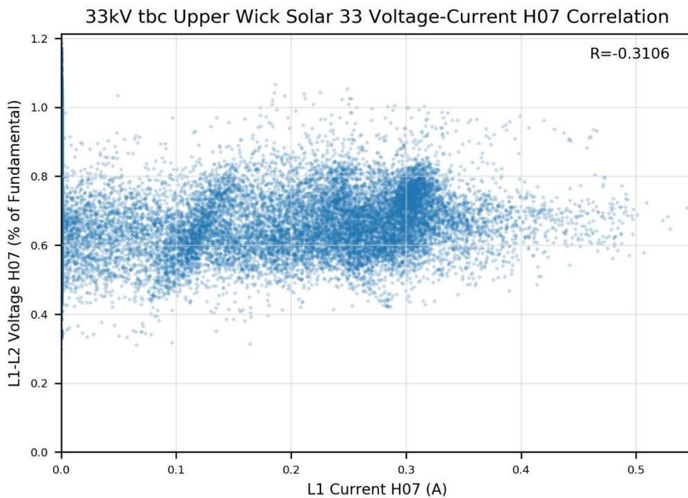
Figure 5-47: Scatter plot of harmonic current H07 vs. harmonic voltage H07 for Upper Wick Solar
