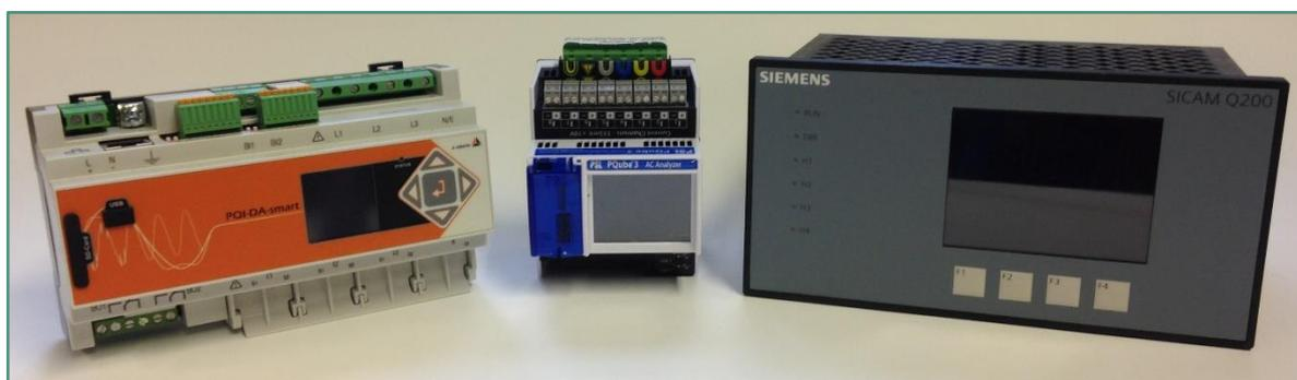
Figure 5-24: The three PQ monitors being used for the project, from left to right: the a-eberle PQI-DA smart, the PSL PQube3, and the Siemens SICAM Q200
