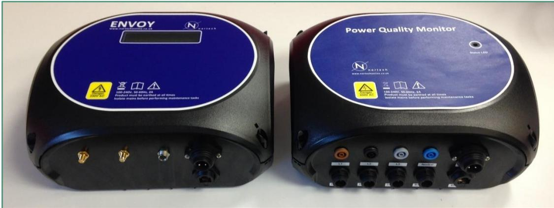
Figure 5-38: Envoy communications hub and prototype PQ monitor enclosure
