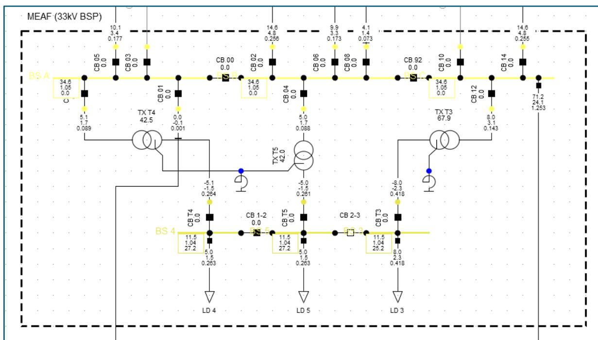
Figure 5-35: A section of the power system model for the Meaford C trial area, showing Meaford C BSP 33 kV elements
