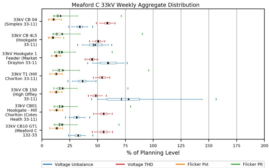
Figure 5-53: Range of non-harmonic PQ measurand weekly aggregates for Meaford C 33 kV sites
