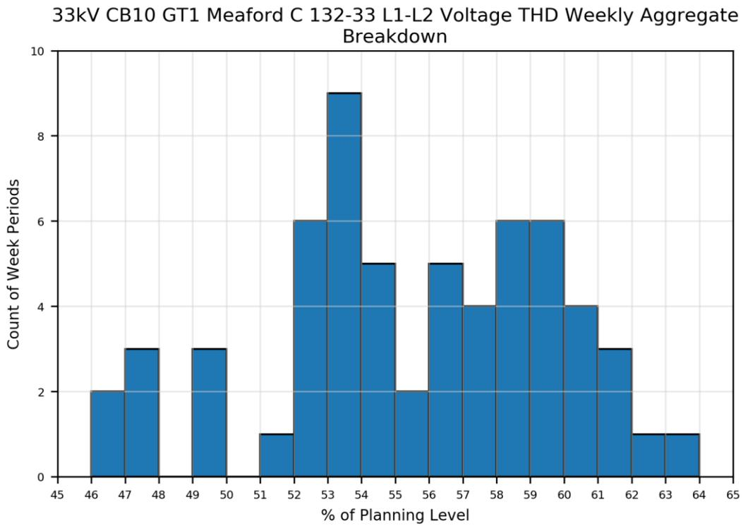
Figure 5-51: Histogram of weekly aggregate values for voltage THD (L1-L2) at Meaford C 33 kV BSP
