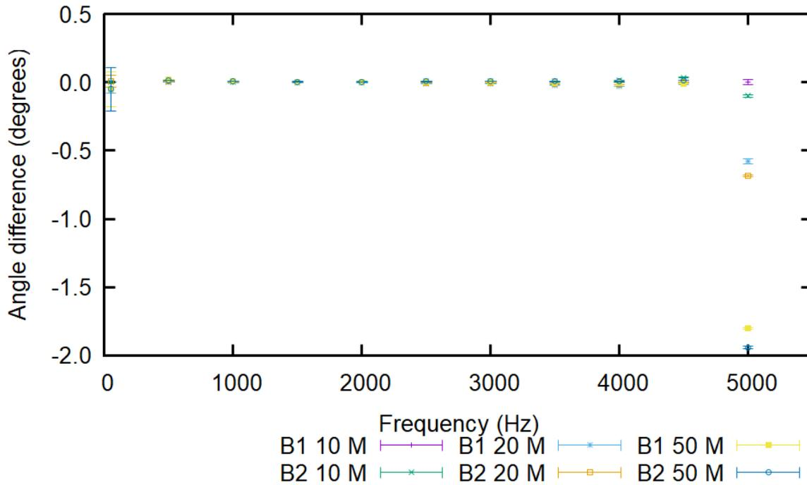
Figure 5-15: Comparison of phase angle difference between secondary and primary voltage for phase 2 of VT #2 to B1 10M, for various secondary wiring configurations and frequencies.
