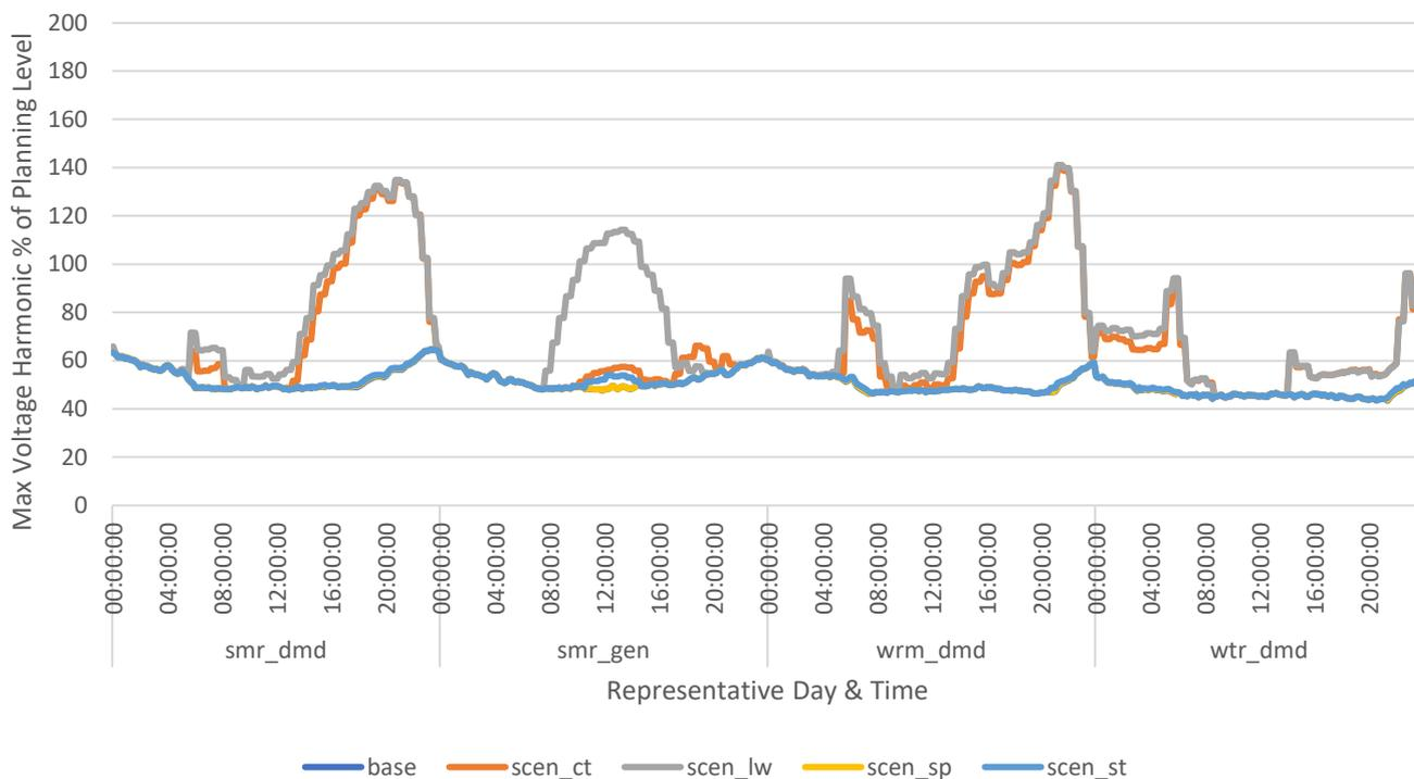
Figure 5-36: Estimated maximum harmonic voltages for the 2030 scenarios in the Meaford C 33 kV network
