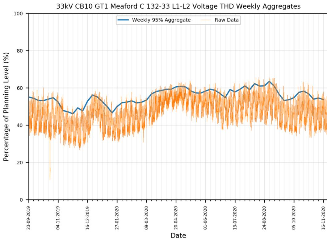
Figure 5-50: Time series plot of voltage THD (L1-L2) for Meaford C 33 kV BSP showing raw data (10 minute resolution) and weekly 95<sup>th</sup> percentile aggregates
