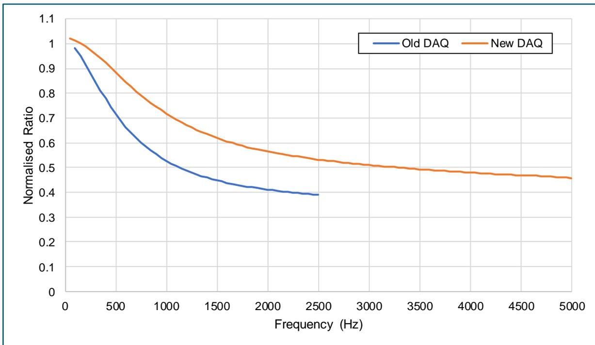
Figure 5-3: Magnitude frequency response of the 33 kV 1-ph VT #1
