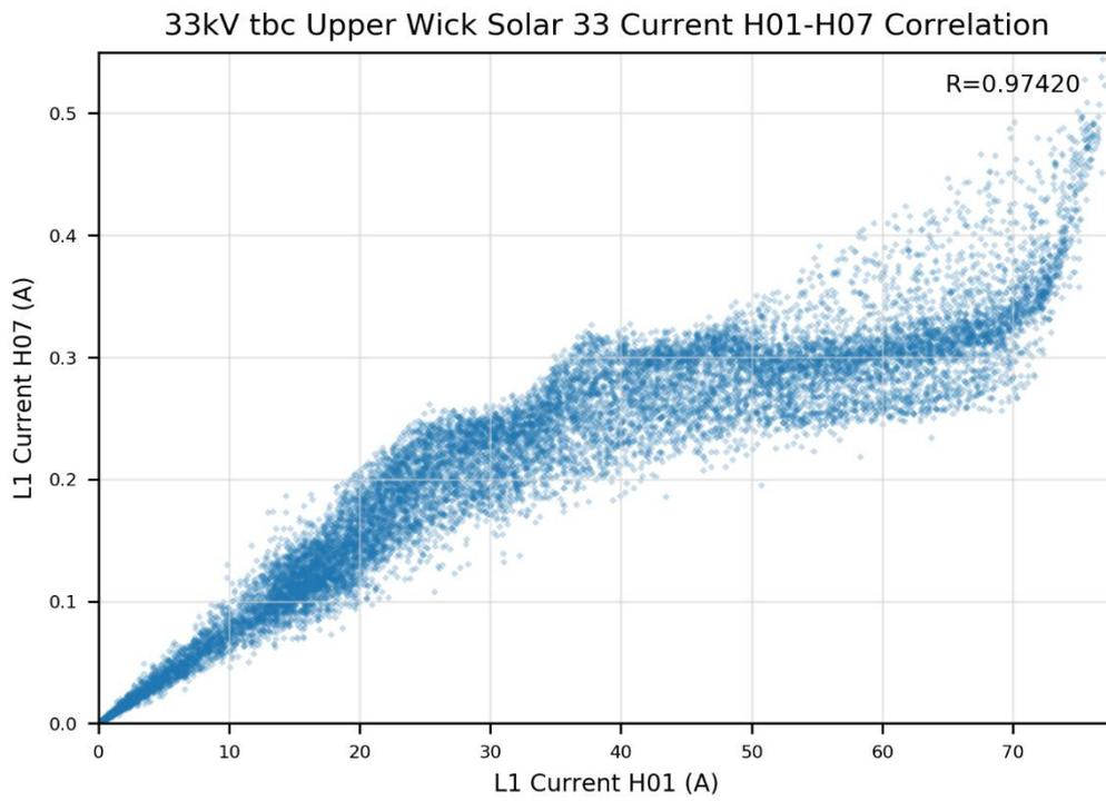
Figure 5-46: Scatter plot of fundamental current (H01) vs. harmonic current H07 for Upper Wick Solar
