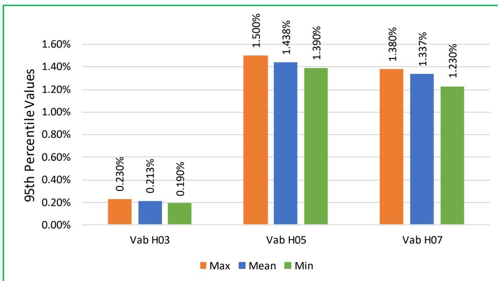
Figure 5-22: Summary of effect on harmonic summary statistics by changing the start date and time of a standard week-long monitoring window (Vab, based on 10 minute interval data).
