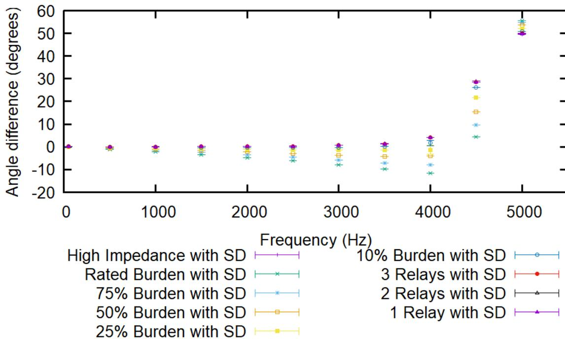
Figure 5-7: Phase angle separation between secondary and primary windings for phase 3 on VT#2 for various frequencies and burdens.
