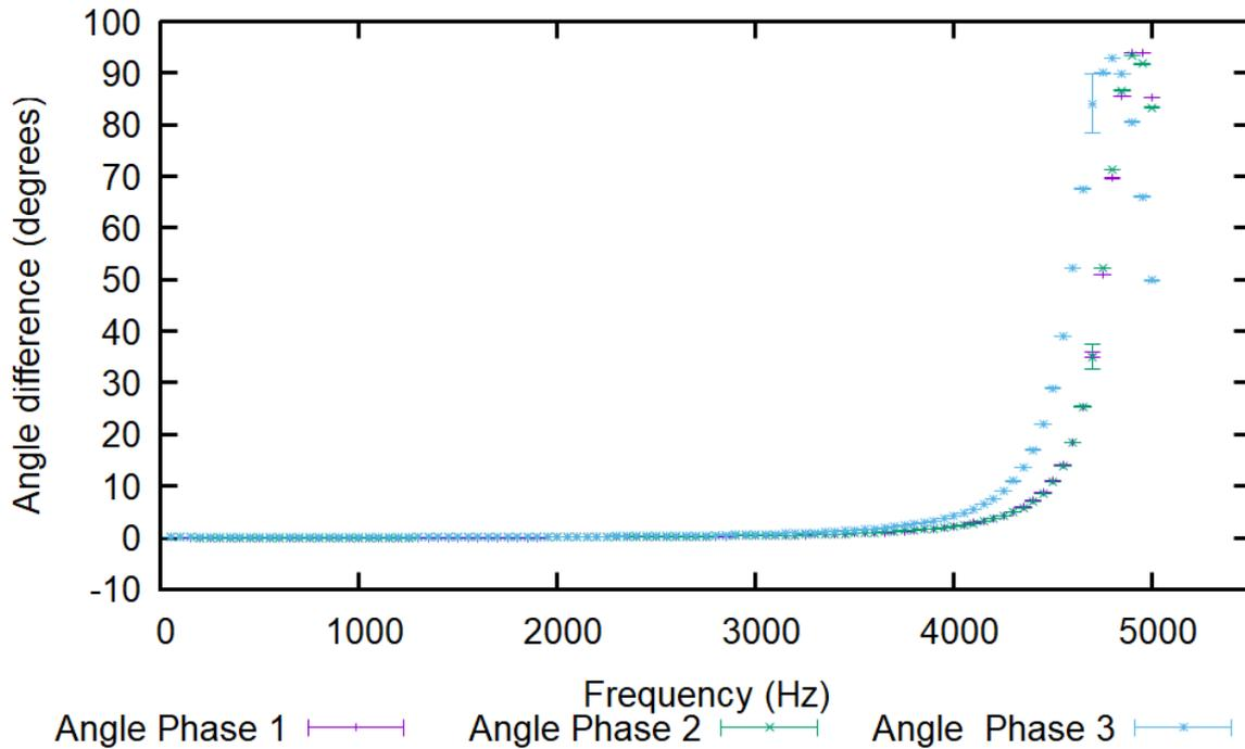
Figure 5-9: Phase angle separation between secondary and primary windings for all phases on VT #2 for various frequencies.
