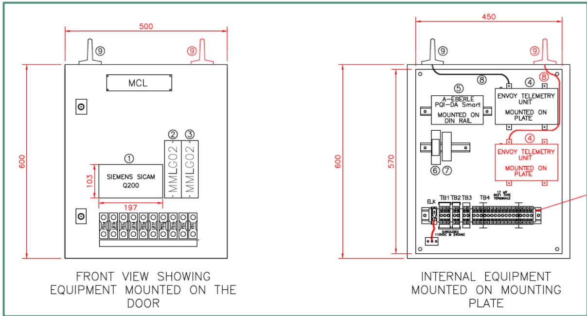
Figure 5-41: Example general arrangement drawing for PQ panel
