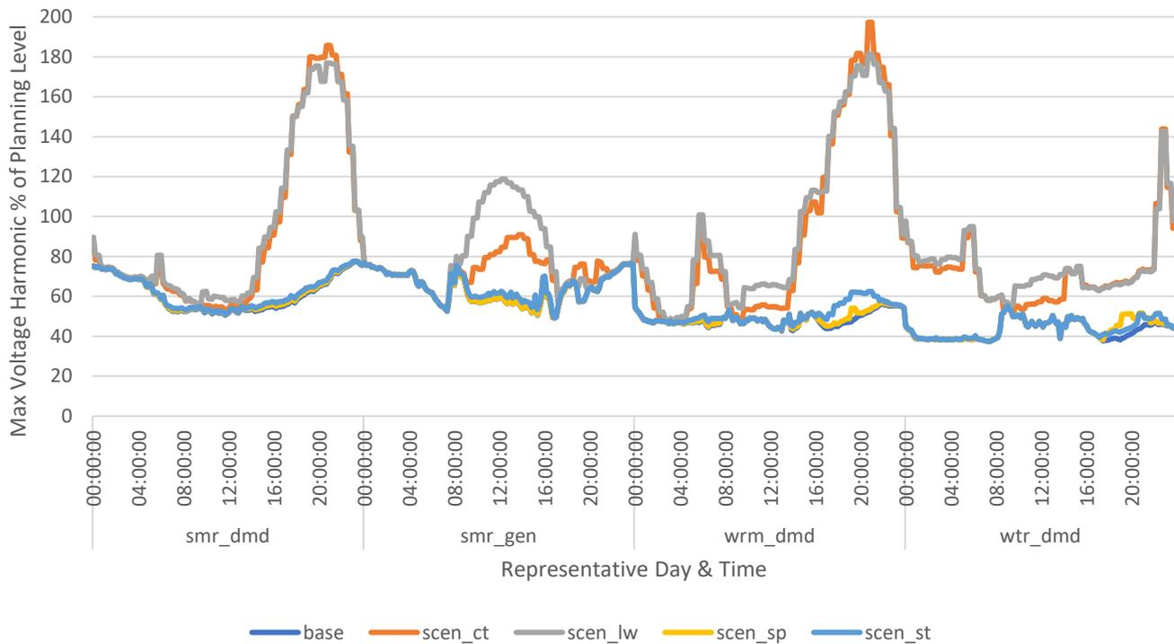
Figure 5-37: Estimated maximum harmonic voltages for the 2030 scenarios in the Ryeford 33 kV network
