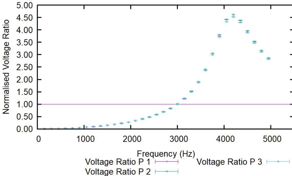
Figure 5-10: Ratio of secondary to primary voltage for VT #4, for various triplen frequencies.
