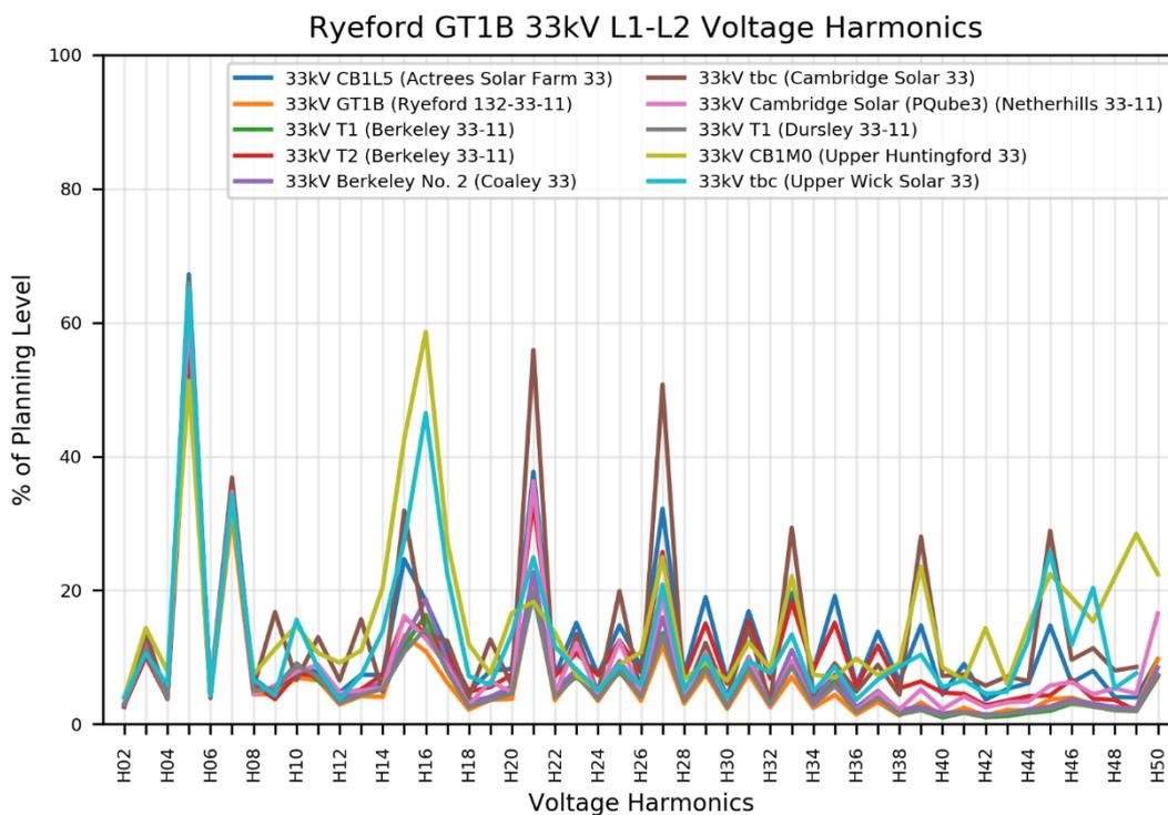
Figure 5-43: Overall voltage harmonic aggregates (95<sup>th</sup> percentile values) for Ryeford 33 kV GT1B group sites
