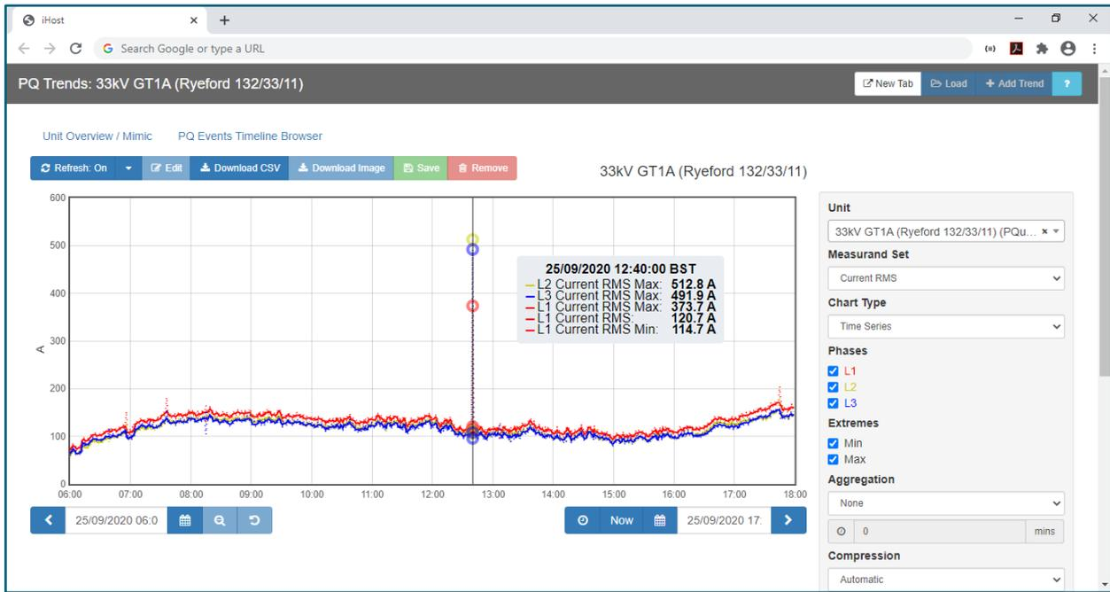
Figure 5-33: Updated PQ Trends with min and max data displayed for RMS current, including a current spike likely due to fault activity
