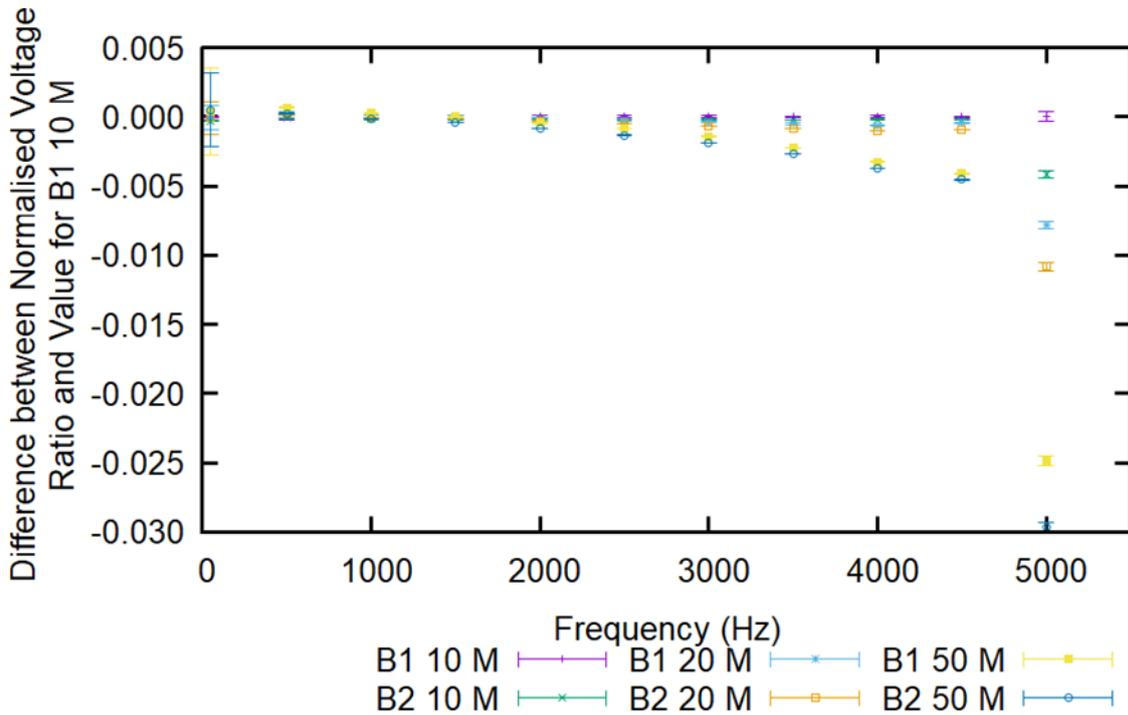
Figure 5-14: Comparison of ratio of secondary to primary voltage for phase 2 of VT #2 to B1 10M, for secondary wiring configurations and frequencies.
