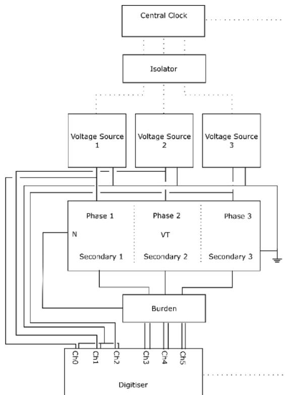
Figure 5-5: 3-phase VT test setup, with solid lines showing voltage connections and dotted lines showing timing signals
