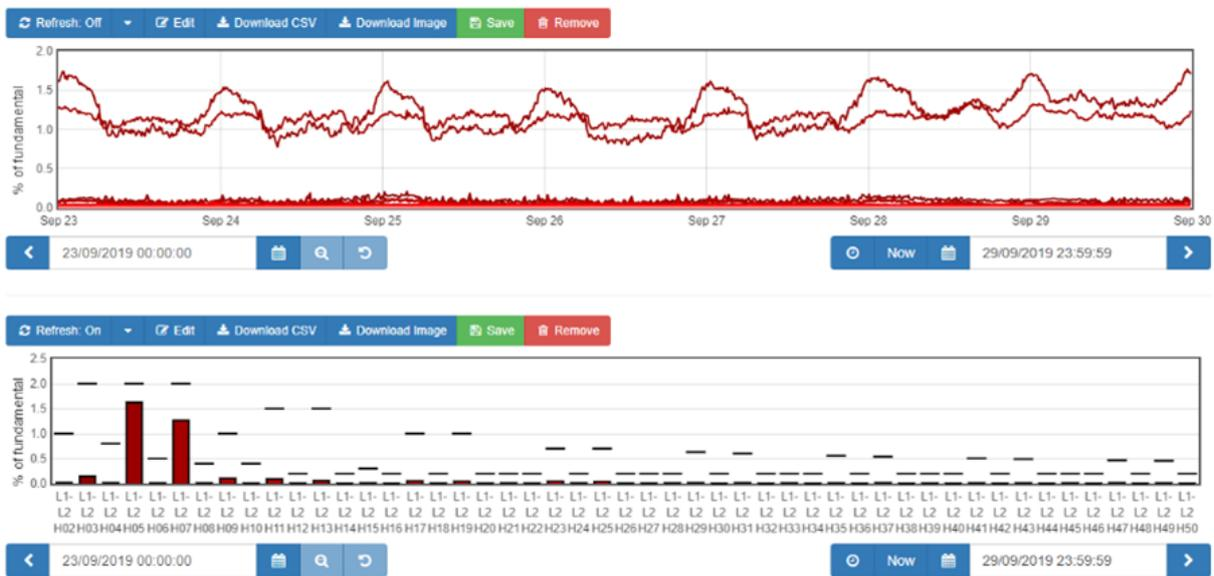
Figure 5-25: Example PQ Trend showing a week of harmonic data as time-series and bar plots
