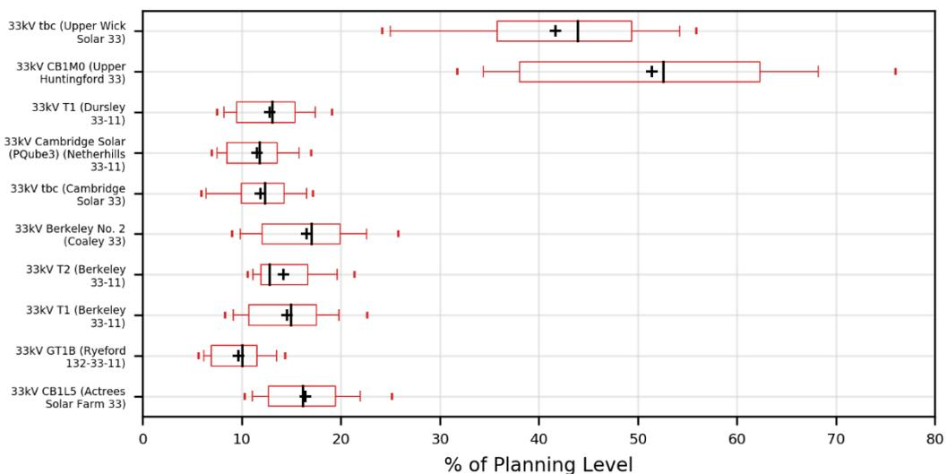
Figure 5-54: Box plot showing the distribution of 16<sup>th</sup> voltage harmonic weekly aggregates for the Ryeford 33 kV GT1B sites
