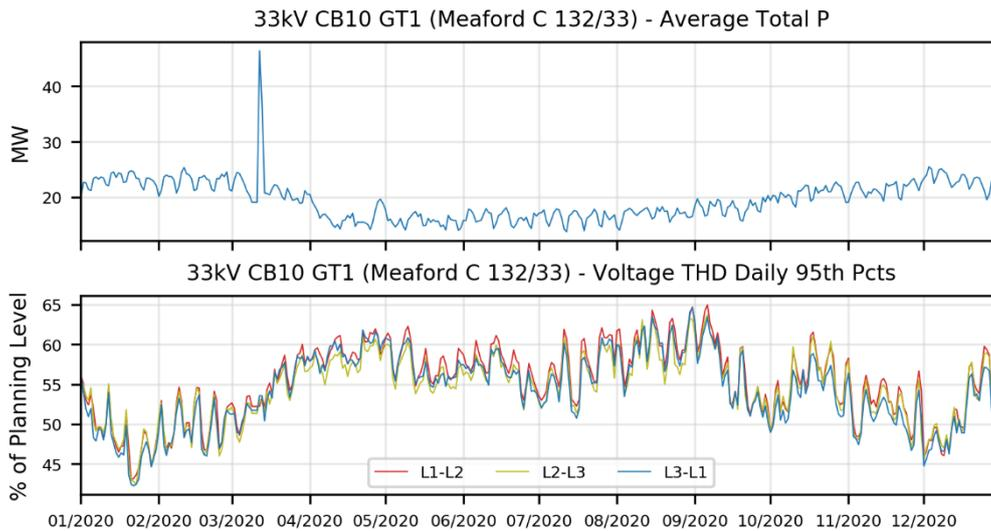
Figure 5-56: Daily average power and 95<sup>th</sup> percentile voltage THD values at Meaford C 33 kV BSP during 2020
