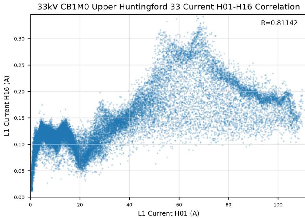
Figure 5-48: Scatter plot of fundamental current (H01) vs. harmonic current H16 for Upper Huntingford solar
