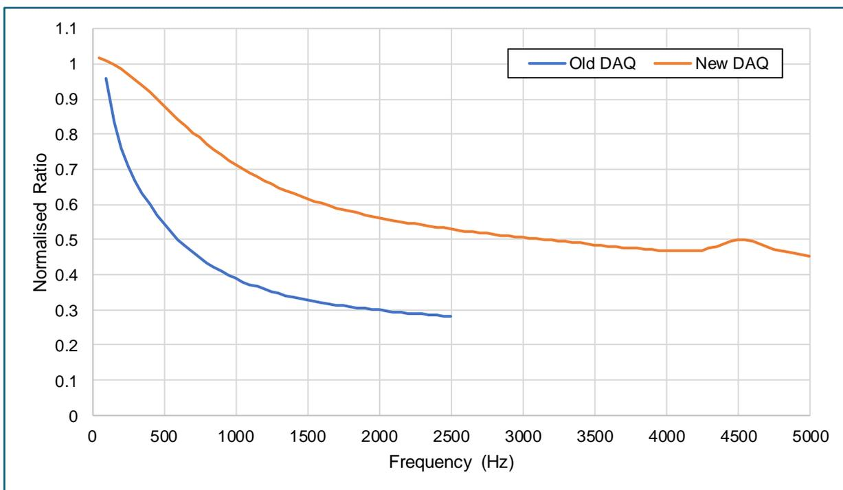
Figure 5-4: Magnitude frequency response of the 33 kV 1-ph VT #2
