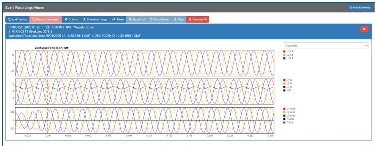
Figure 5-28: Event Recordings Viewer displaying a voltage and current waveform data
