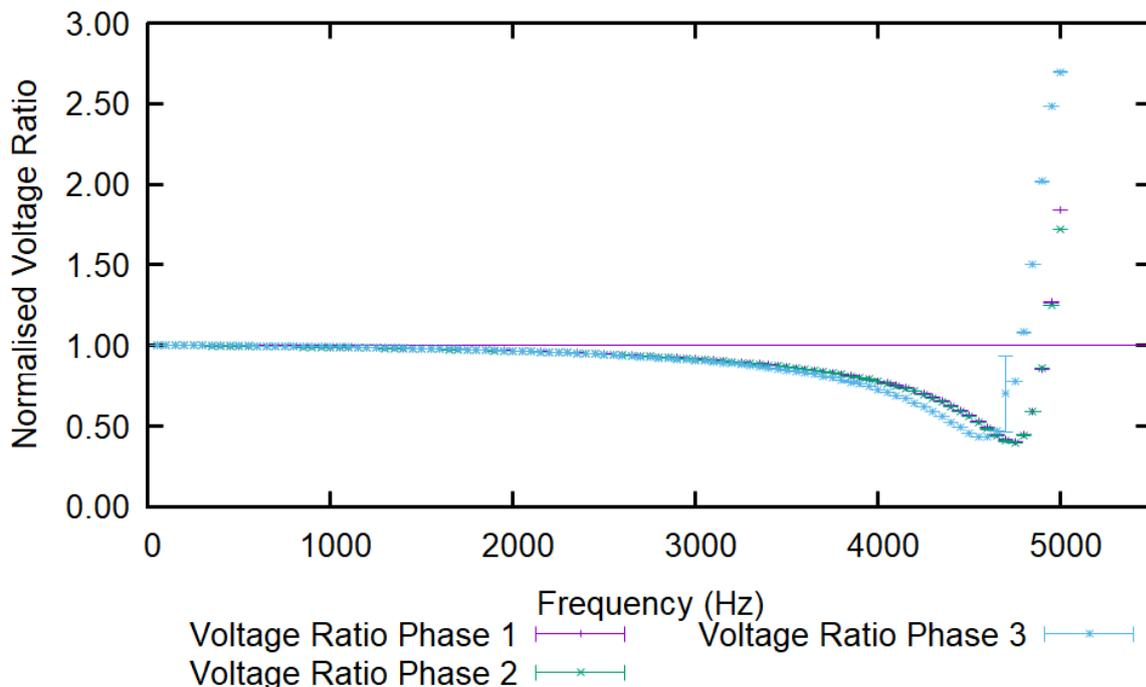
Figure 5-8: Ratio of secondary to primary voltage on VT #2 for various frequencies and all phases. The horizontal line shows the nominal ratio.
