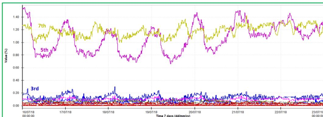
Figure 5-20: Harmonic profiles for an example week (10 minute samples, displayed in Pronto).
