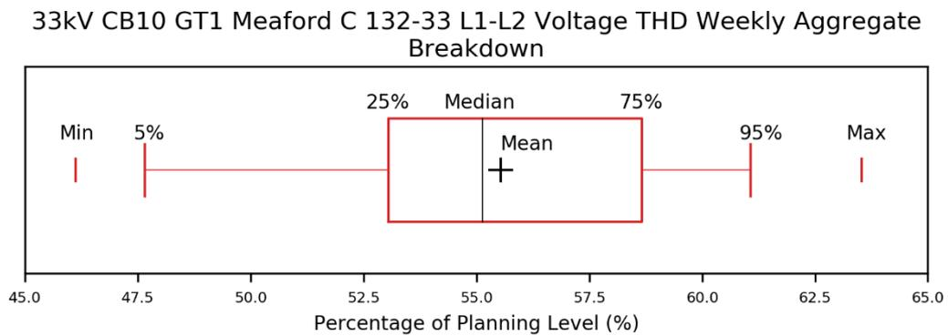
Figure 5-52: Annotated box plot showing distribution of weekly aggregate voltage THD values (L1-L2) at Meaford C 33 kV BSP
