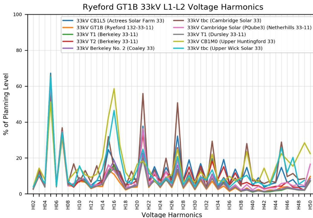
Figure 5-58: Overall voltage harmonic aggregates (95th percentile) for Ryeford 33 kV GT1B group sites
