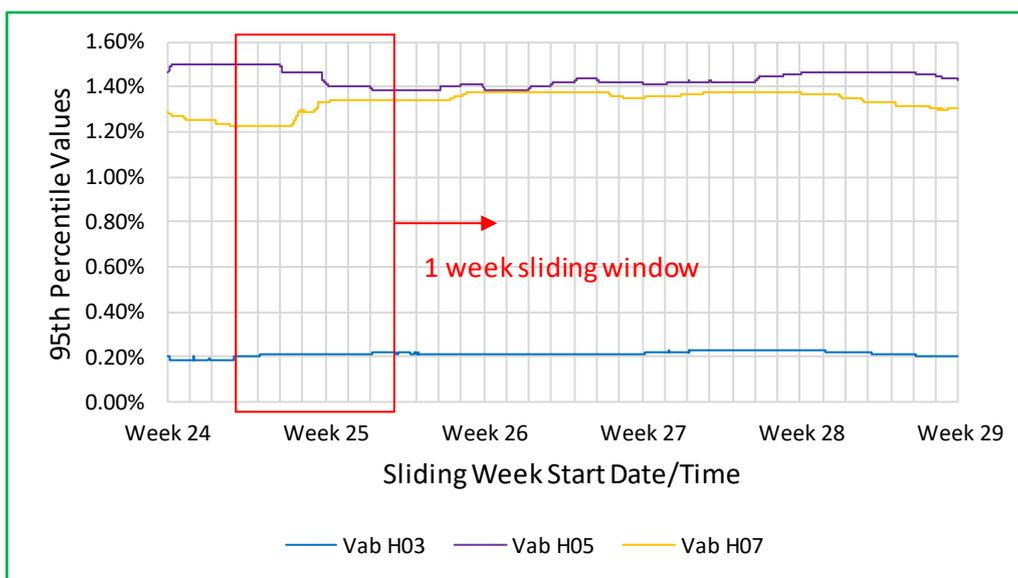
Figure 5-21: Effect on voltage harmonic summary statistics (95th percentile values) by changing the start date and time of a standard week-long monitoring window (Vab, based on 10 minute interval data).
