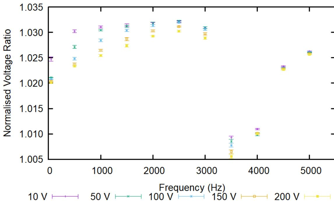
Figure 5-12: Ratio of secondary to primary voltage phase 1 of VT #1, for various primary voltages and frequencies.
