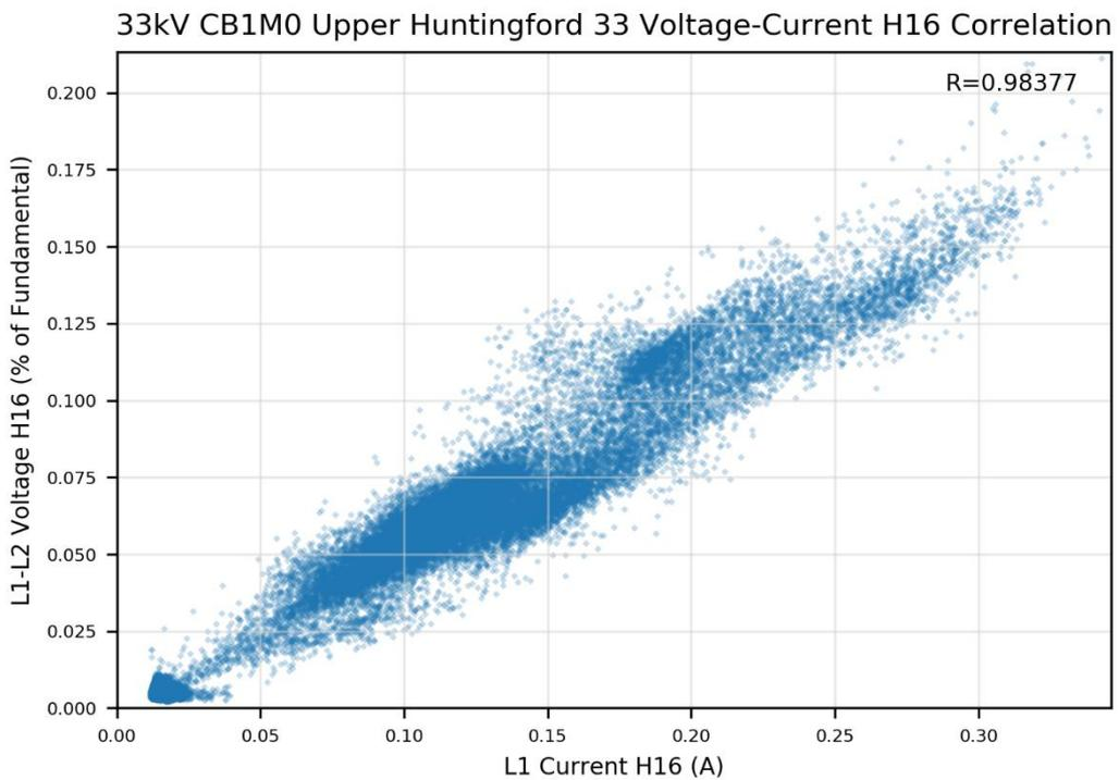
Figure 5-49: Scatter plot of harmonic current H16 vs. harmonic voltage H16 for Upper Huntingford solar
