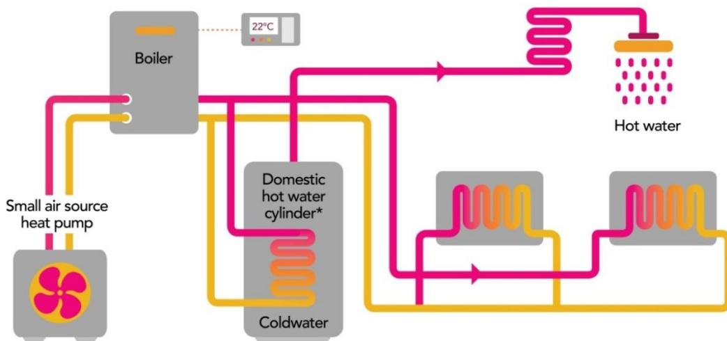
Figure 6: Configuration of a Hybrid Heating System
