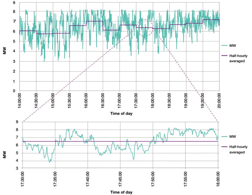
This half-hourly average data is used extensively to design the network. This raises the question as to what recording frequency of monitoring will be needed in the future to determine actual peaks and the length that these peaks persist. This needs to be considered along with the coincident peaks of other generation and demands to determine what granularity of averaging is desirable.
