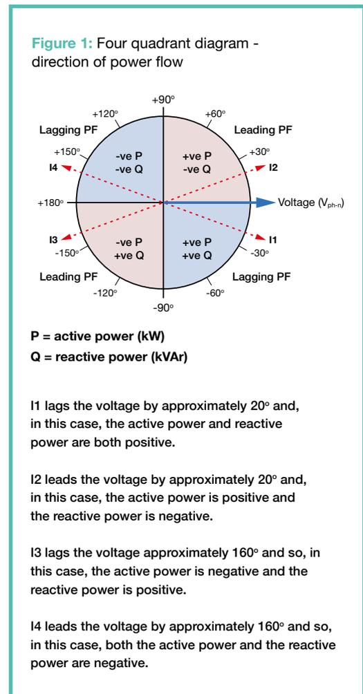
All of these methods of determining power are utilised to some extent on the network. Amps and dummy volts are only used where no voltage is available, as it introduces an error where the voltage is not operating at nominal voltage. Operating above nominal voltage is common at most substation busbars, to account for voltage drop at the extremities of the network.
