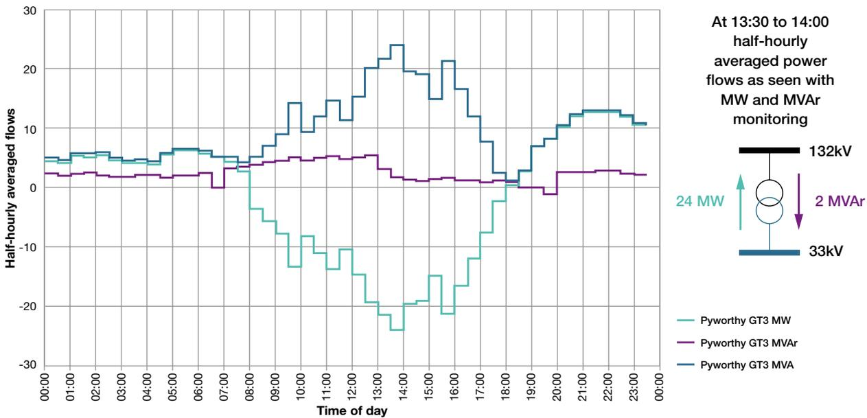
Figure 4 shows the same transformer on the same day, but with full directional MW and MVAR metering.
