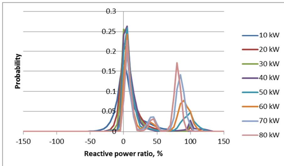
Figure 38 Probability distribution of reactive power for LV feeders
