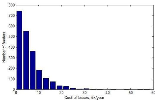
Figure 60 Histogram of number of HV feeders versus annual cost of feeder losses
