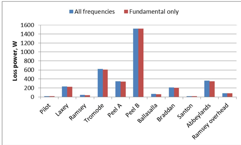
Figure 40 LV feeder cable losses calculated from measurement data using RMS current amplitude and fundamental current amplitude
