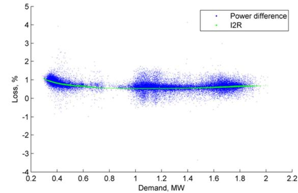
Figure 88 Aug 2018 Loss, % vs demand (Amway Tongwell HV feeder)
