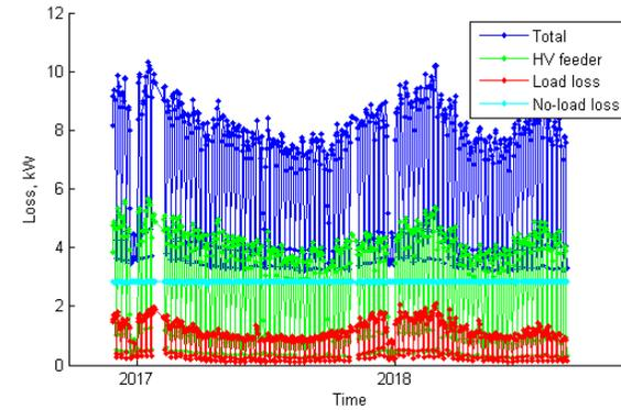
Figure 86 Long term mean daily ( $I^2R$ ) loss (Amway Tongwell HV feeder)
