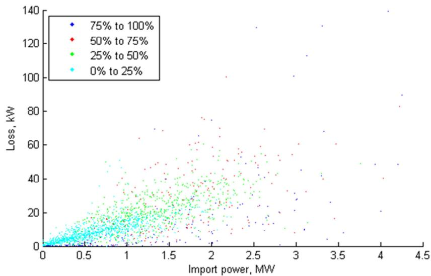
Figure 56 Loss vs. network import power coloured for proportion of losses due to HV cable load losses
