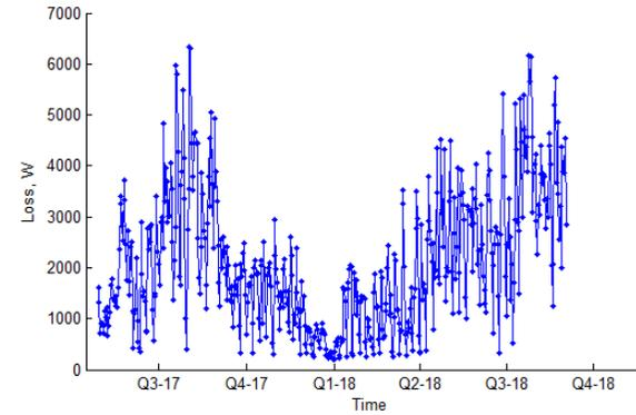
Figure 130 Long term mean daily ( $I^2R$ ) loss (Peel B I&C LV feeder)
