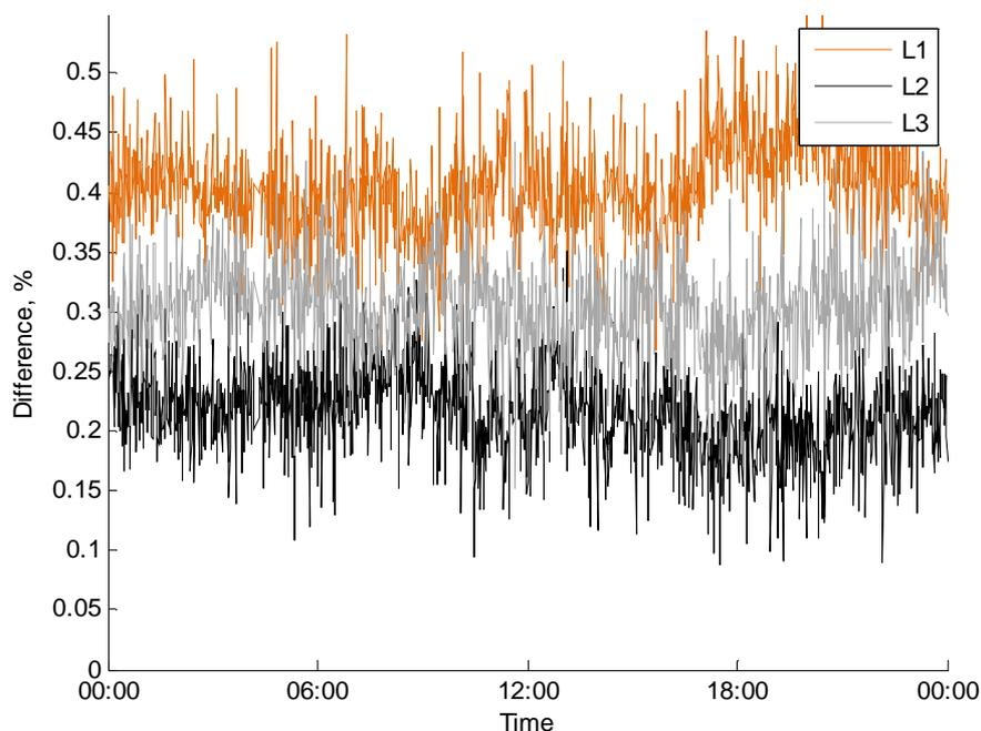
Figure 11 Difference between calculated and measured Distribution Substation voltage on Woodlands feeder, 28<sup>th</sup> March 2016
