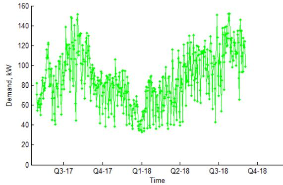
Figure 129 Long term mean daily feeder demand (Peel B I&C LV feeder)
