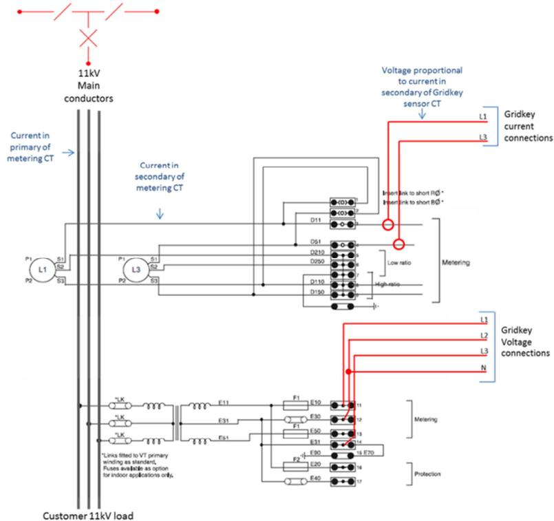
**Figure 4 Schematic of monitoring at HV customer connections**
