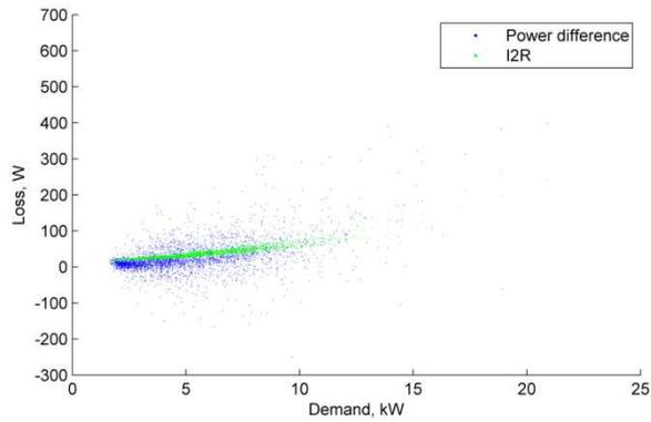
Figure 143 Aug 2018 Loss, kW vs demand, 10 min. av. (Santon OH LV feeder)
