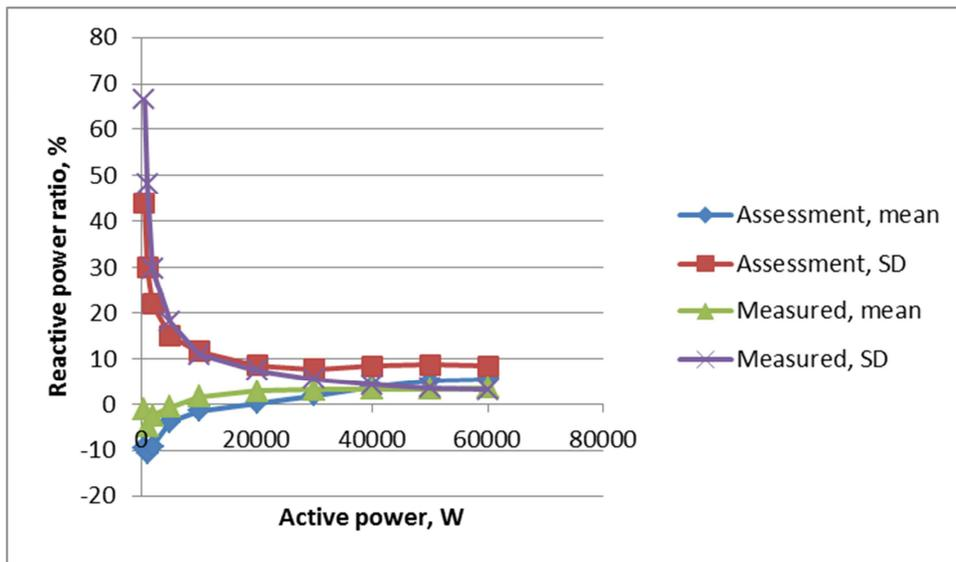
Figure 174 Mean and standard deviation of reactive power for domestic feeders at Milton Keynes trial distribution substations, from measured data and from loss assessment method
