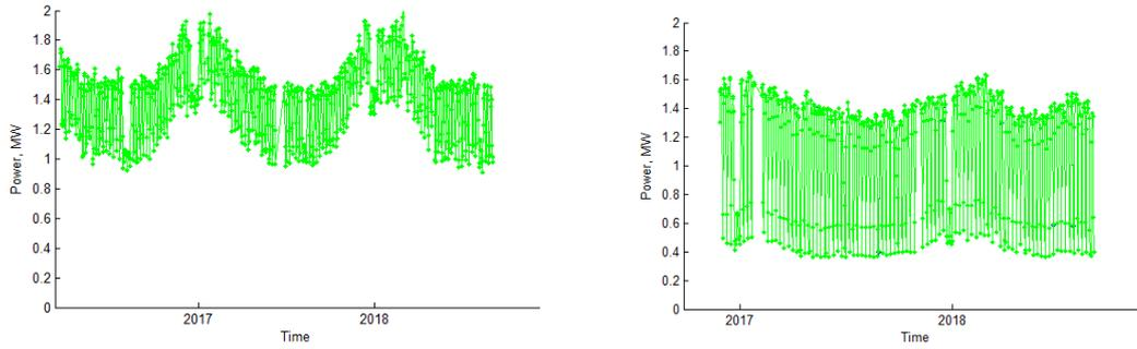
Figure 50 Sample monitored LV feeder loss vs load plot, 1 minute loss/load points using  $I^2R$  calculation method
