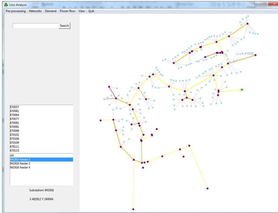
**Figure 25 LV loss assessment software Python interface showing unbalances for substation 941916 feeder 1 (ratio of mean zero sequence current to mean positive sequence current, red indicates ratios near 1)**
