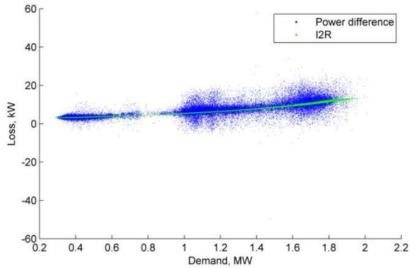
Figure 87 Aug 2018 Loss, kW vs demand (Amway Tongwell HV feeder)
