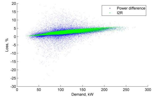
Figure 132 Aug 2018 Loss, % vs demand, 1 min. av. (Peel B I&C LV feeder)
