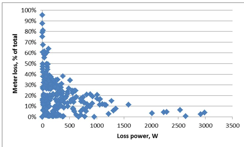
Figure 64 Metering loss as a proportion of the total loss power for LV feeders in Milton Keynes trial.
