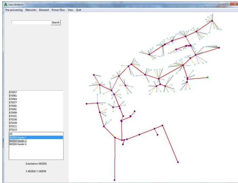
Figure 23 LV loss assessment software Python interface showing losses for substation 941916 feeder 1 (colour scale with highest losses in red, lowest losses in pale yellow)
