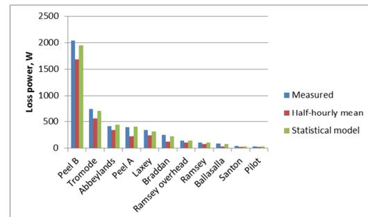
Figure 42 Loss results comparison for monitored LV feeders
