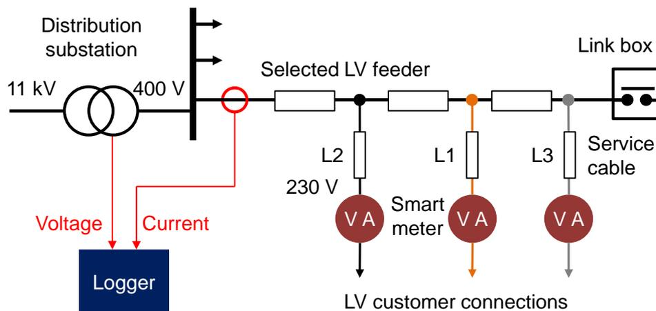
Figure 7 Schematic of LV feeder monitoring
