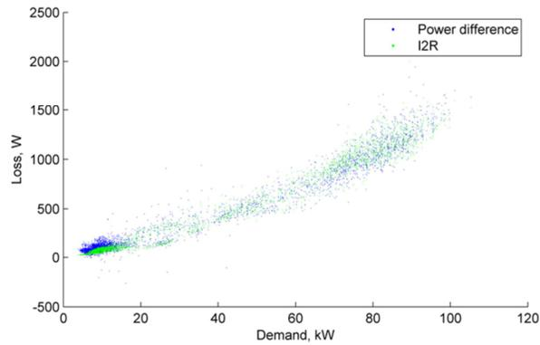
Figure 139 Jan 2018 Loss, kW vs demand, 10 min. av. (Braddan I&C LV feeder)
