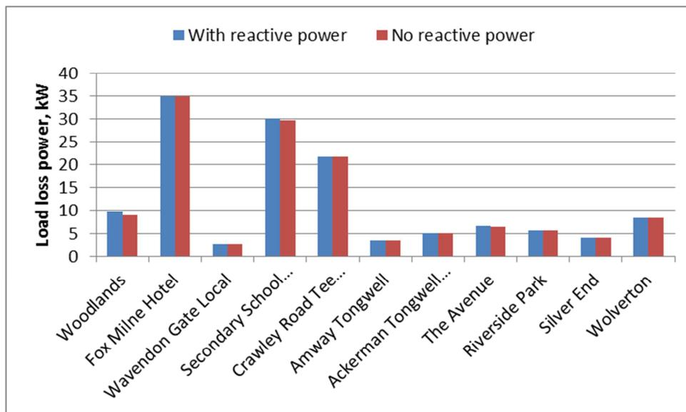
Figure 39 HV feeder mains losses calculated with and without reactive power
