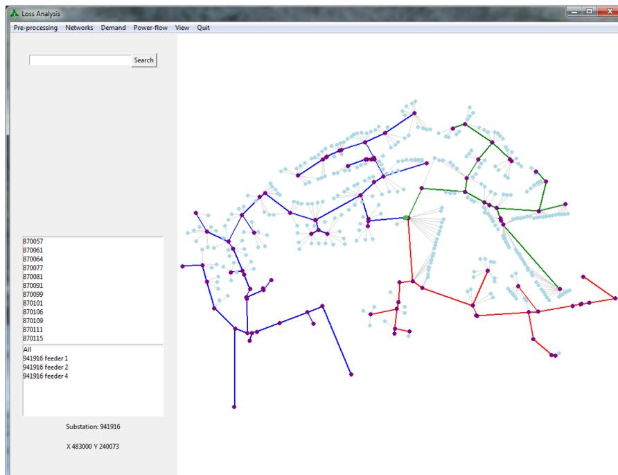
Figure 22 LV loss assessment software Python interface showing LV feeders for substation 941916s
