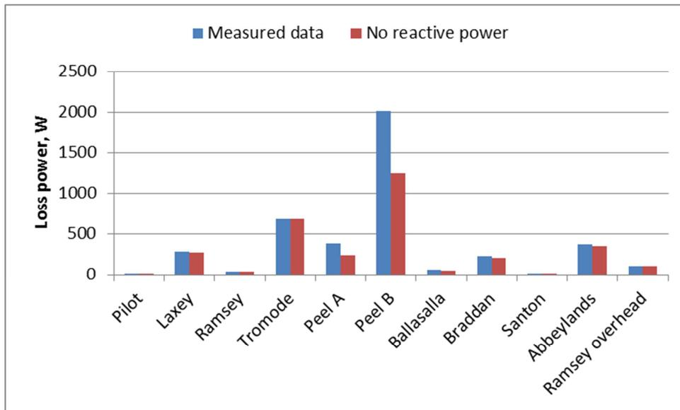
Figure 37 LV feeder mains losses calculated with and without reactive power
