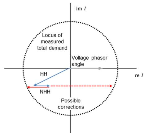
Figure 156 Corrections applied to non-half-hourly demand where the amplitude of the primary substation current due to half-hourly demand is less than the measured current at the primary, with half-hourly demand as generation.
