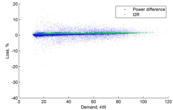
Figure 116 Jan 2018 Loss, % vs demand, 1 min. av. (Laxey Dom. LV feeder)
