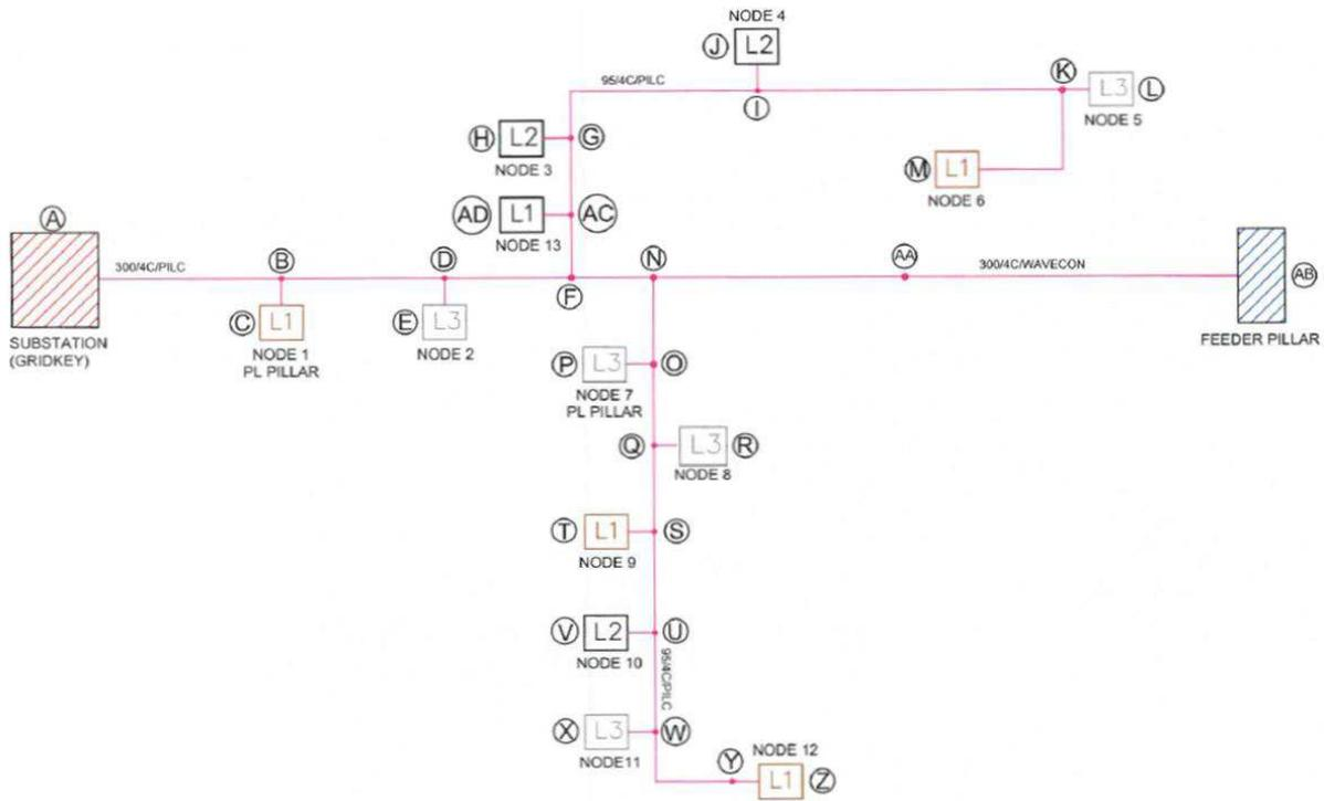
Figure 9 Pilot LV feeder
