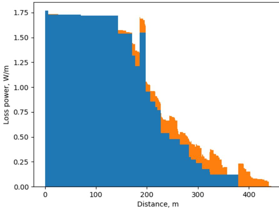
Figure 168 Example plot showing variation of losses with distance from substation for 941916 feeder 4
