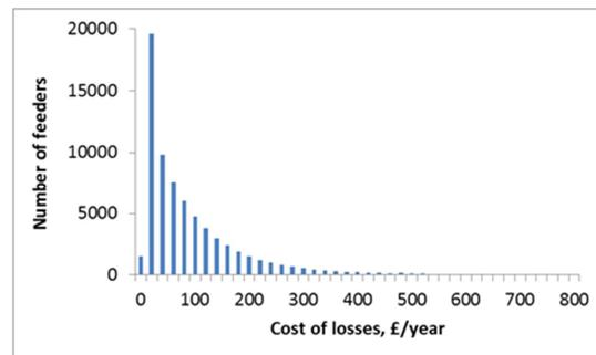
Figure 61 Histogram of number of LV feeders versus annual cost of feeder losses, curtailed at £600/year representing 99% of all losses
