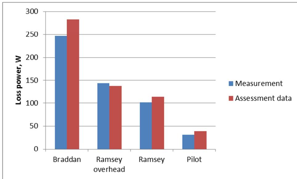
Figure 171 Mean loss power for LV trials feeders with demand and network approximations
