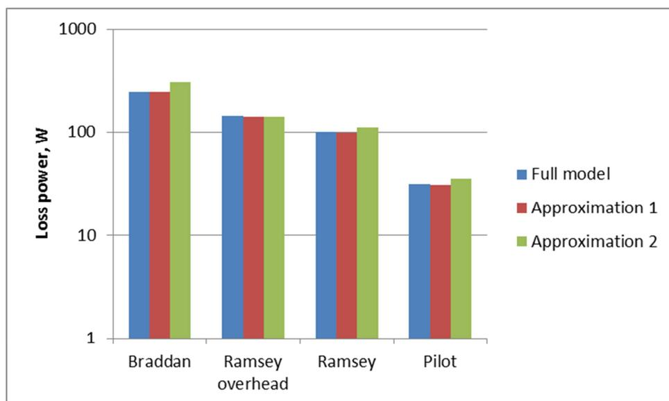
Figure 169 Impact of service cable approximations on LV trials feeders
