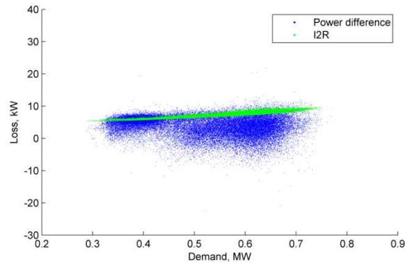
Figure 91 Aug 2018 Loss, kW vs demand (Ackerman Tongwell Aldrich Drive Tee HV feeder)
