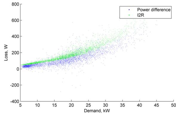
Figure 151 Jan 2018 Loss, kW vs demand, 10 min. av. (Ramsey OH LV feeder)
