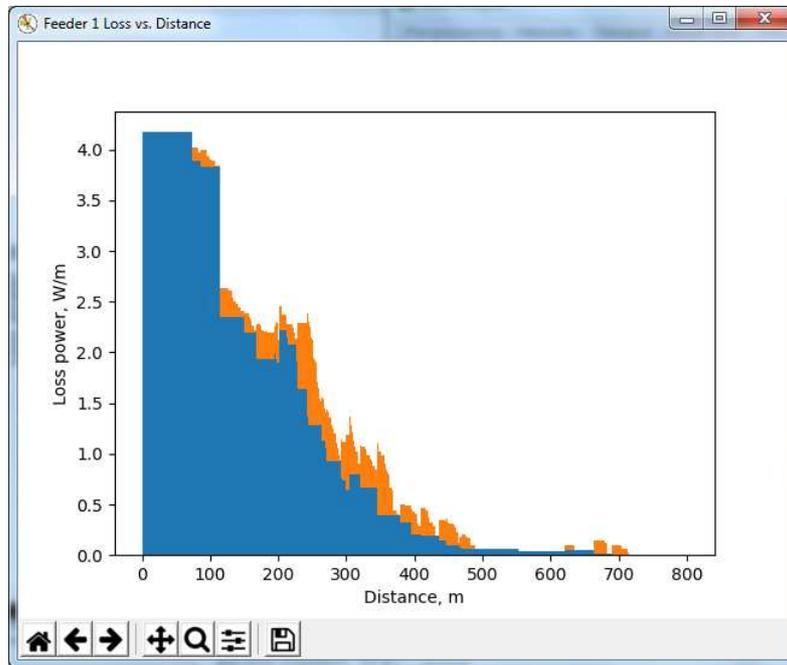
Figure 57 LV loss assessment software output showing cable loss power per unit length vs distance for feeder 1 (mains cable losses in blue, service cable losses in orange)
