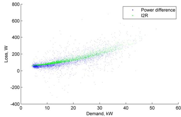
Figure 119 Aug 2018 Loss, kW vs demand, 10 min. av. (Ramsey Dom. LV feeder)
