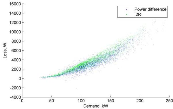
Figure 131 Aug 2018 Loss, kW vs demand, 10 min. av. (Peel B I&C LV feeder)
