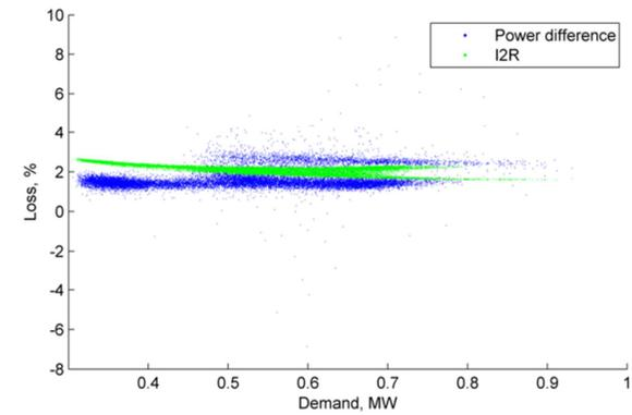
Figure 108 Aug 2017 Loss, % vs demand (Wolverton HV feeder)
