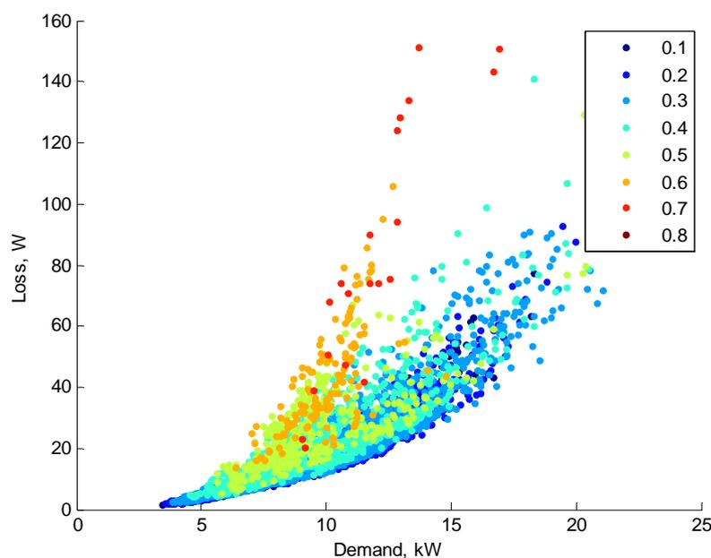
Figure 165 Loss vs. demand with colour indicating unbalance factor
