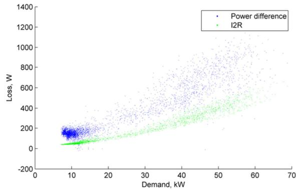
Figure 135 Jan 2018 Loss, kW vs demand, 10 min. av. (Ballasalla I&C LV feeder)
