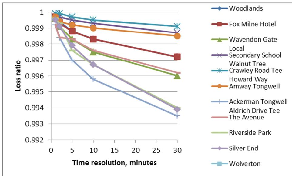
Figure 154 Impact of measurement time resolution for HV feeders
