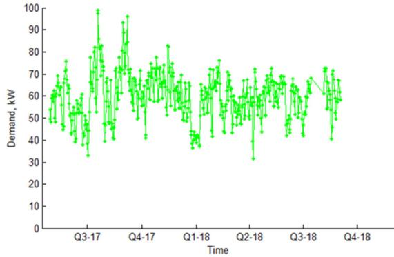
Figure 125 Long term mean daily feeder demand (Peel A I&C LV feeder)
