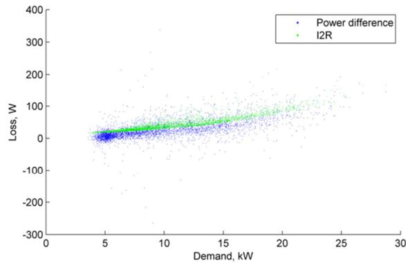
Figure 111 Jan 2018 Loss, kW vs demand, 10 min. av. (Dom. Pilot LV feeder)
