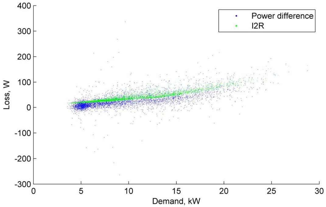
Figure 63 Loss vs demand per 1-minute sample for LV Pilot feeder with 10-minute averaging of the loss results
