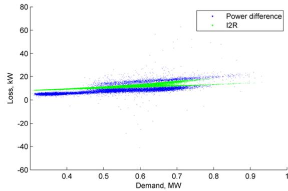
Figure 107 Aug 2017 Loss, kW vs demand (Wolverton HV feeder)
