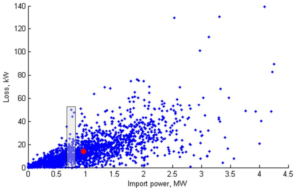
Figure 51 Loss vs. network import power for HV feeders showing mean feeder loss-load point in red
