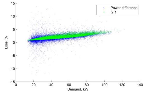
Figure 124 Jan 2018 Loss, % vs demand, 1 min. av. (Tromode Dom. LV feeder)
