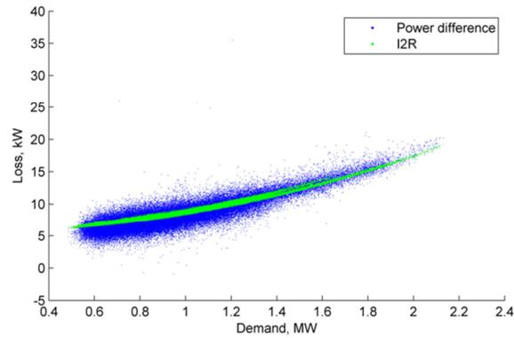
Figure 75 Mar 2018 Loss, kW vs demand (Wavendon Gate Local HV feeder)
