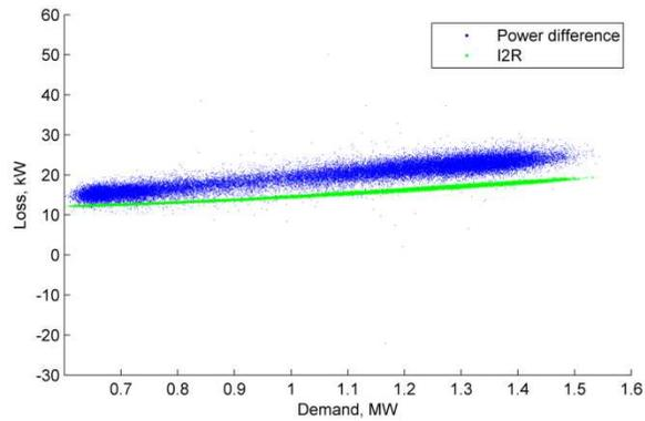
Figure 99 Aug 2018 Loss, kW vs demand (Riverside Park HV feeder)
