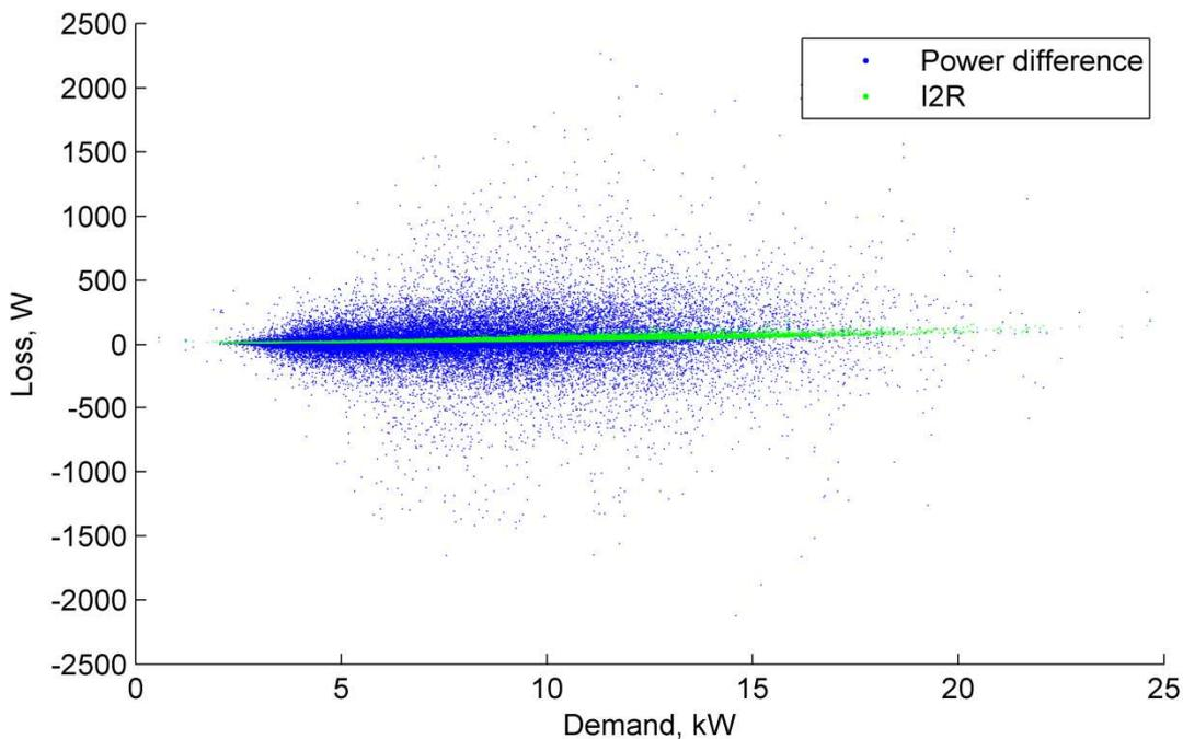
Figure 17 Loss vs demand for 1 minute samples on Pilot LV feeder
