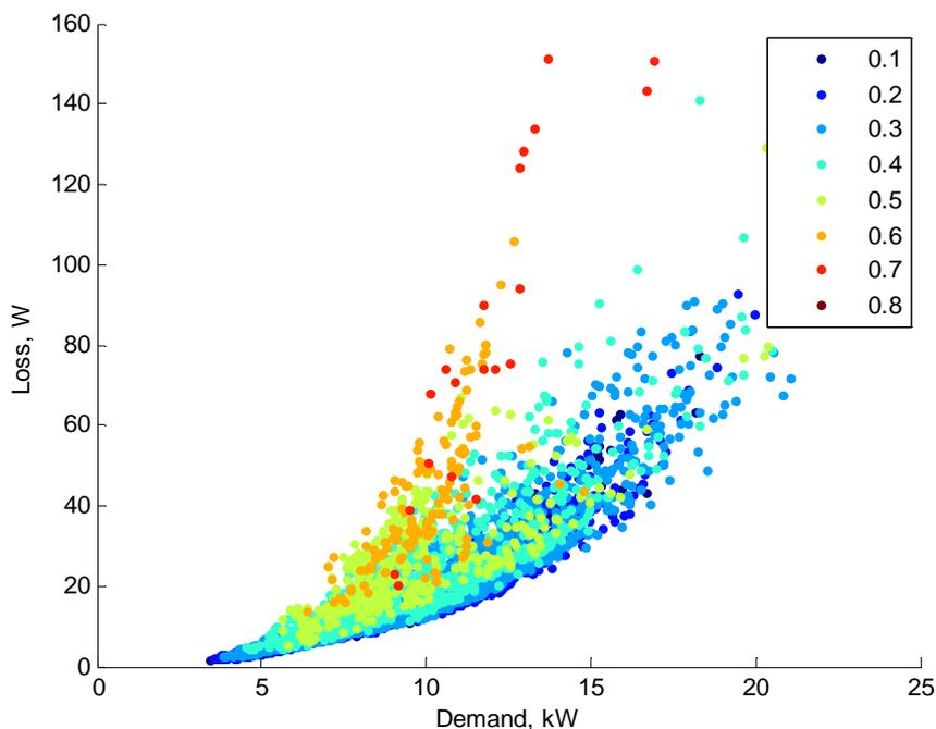
Figure 35 Loss vs. demand with colour indicating unbalance factor
