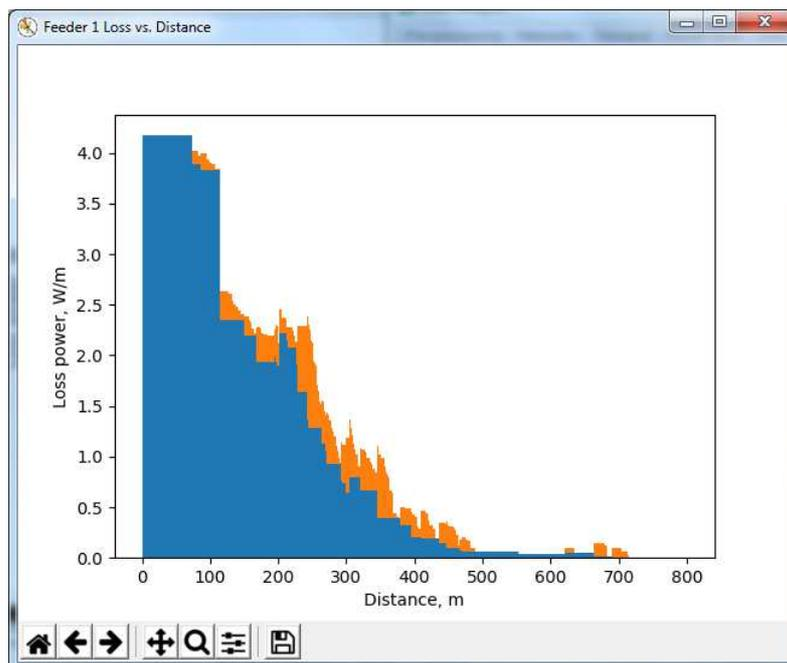
Figure 26 LV loss assessment software output showing cable loss power per unit length vs distance for feeder 1 (mains cable losses in blue, service cable losses in orange)
