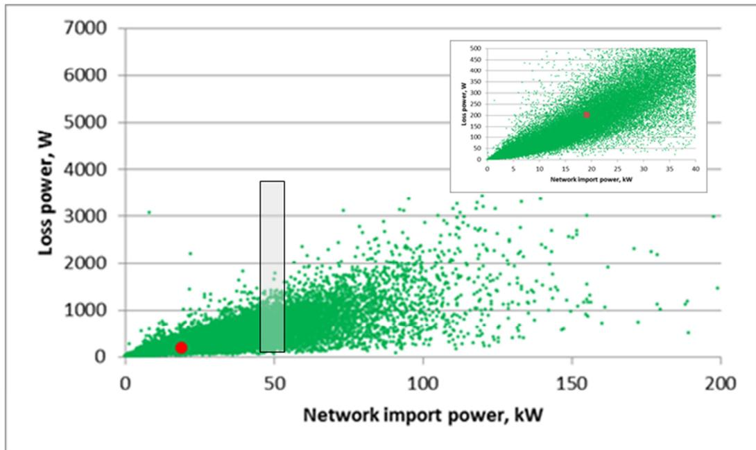
Figure 52 Loss vs. network import power for HV feeders showing mean feeder loss-load point and an indicative trend line
