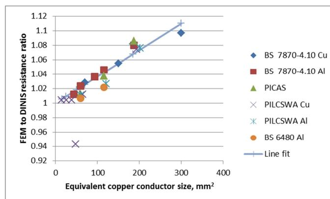
Figure 153 AC resistance scaling for underground cables.
