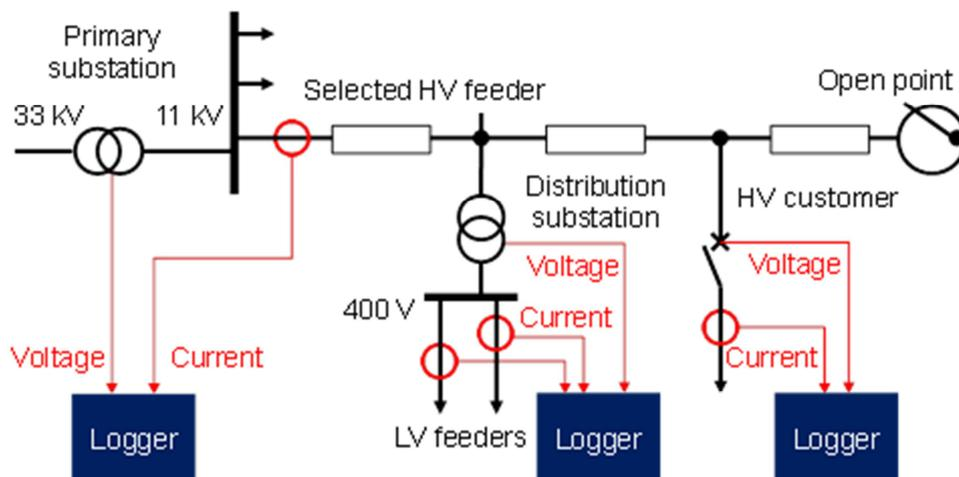
Figure 1 Schematic of HV feeder monitoring
