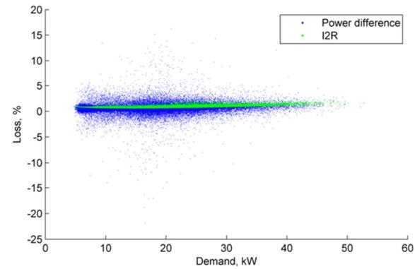
Figure 152 Jan 2018 Loss, % vs demand, 1 min. av. (Ramsey OH LV feeder)
