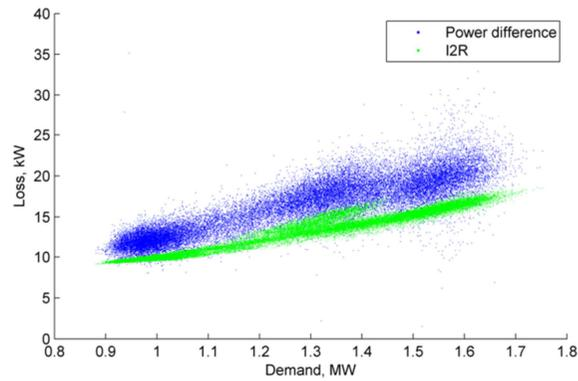
Figure 95 Sep 2017 Loss, kW vs demand (The Avenue HV feeder)
