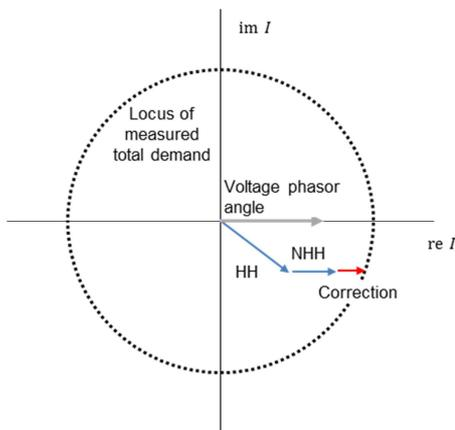
Figure 155 Corrections applied to non-half-hourly demand where the amplitude of the primary substation current due to half-hourly demand is less than the measured current at the primary, and with half-hourly, with non-half-hourly demand as loads.
