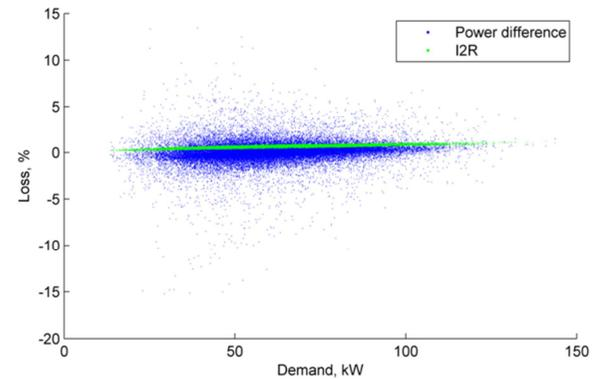
Figure 128 Jan 2018 Loss, % vs demand, 1 min. av. (Peel A I&C LV feeder)
