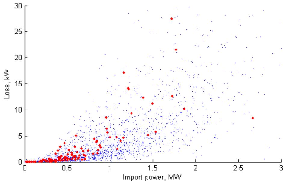
Figure 55 Line loss vs. network import power coloured for voltage (blue: 11 kV, red 6.6 kV)
