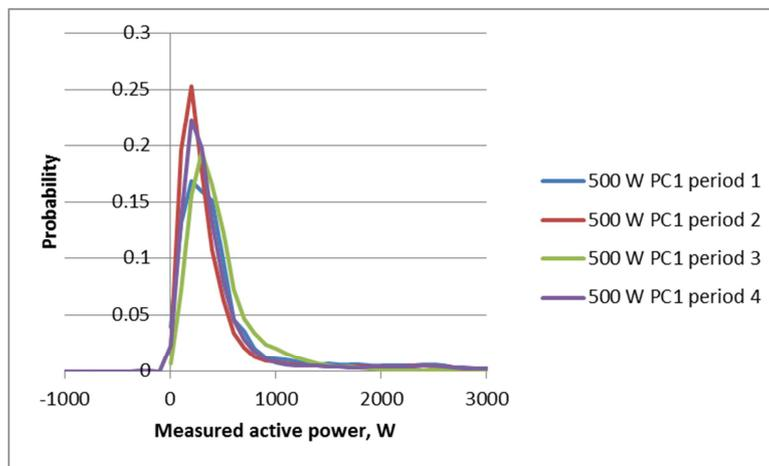
Figure 161 Probability distribution of measured 1-minute power for profile class 1, predicted demand power 500 W, and for periods 1 to 4
