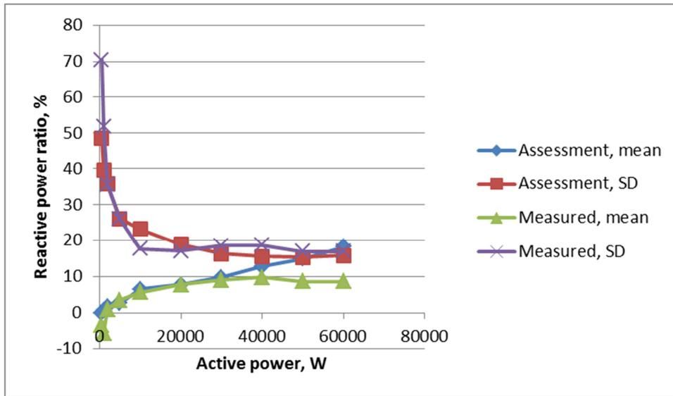
Figure 173 Mean and standard deviation of reactive power for all feeders at Milton Keynes trial distribution substations, from measured data and from loss assessment method
