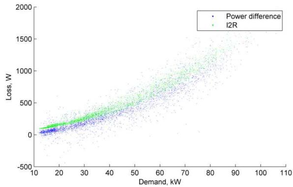
Figure 115 Jan 2018 Loss, kW vs demand, 10 min. av. (Laxey Dom. LV feeder)
