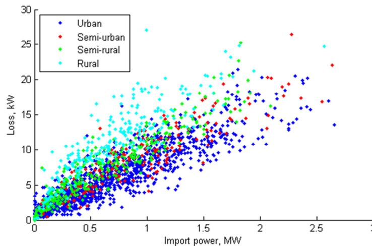
Figure 54 Transformer no-load loss vs. import power
