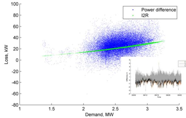
Figure 83 Aug 2018 Loss, kW vs demand (Crawley Road Tee Howard Way HV feeder)
