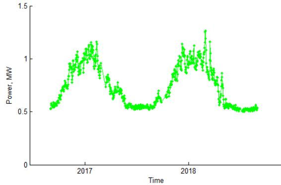
Figure 73 Long term mean daily feeder demand (Wavendon Gate Local HV feeder)
