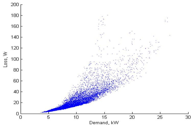
Figure 49 Sample monitored LV feeder loss vs load plot, 1 minute loss/load points using I<sup>2</sup>R calculation method
