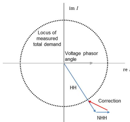
Figure 157 Corrections applied to non-half-hourly demand where the amplitude of the primary substation current due to half-hourly demand is greater than the measured current at the primary.
