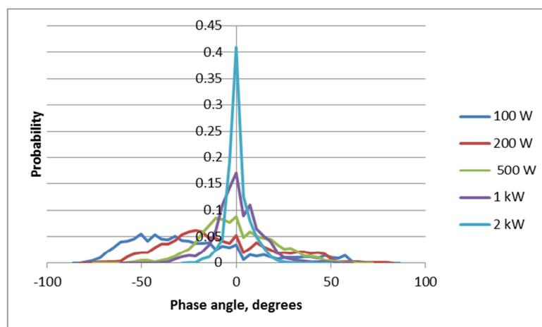
Figure 162 Probability distribution of measured 1-minute reactive power phase angle for profile class 1
