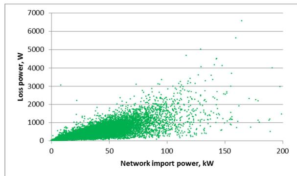
Figure 46 Filtered LV feeder loss assessment results, loss power vs. demand
