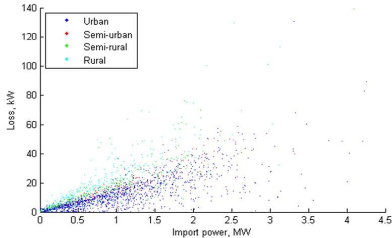
Figure 53 Loss vs. network import power coloured for feeder type
