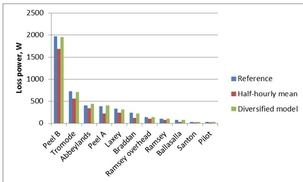
Figure 170 Mean loss power for LV trials feeders with demand model and measurement
