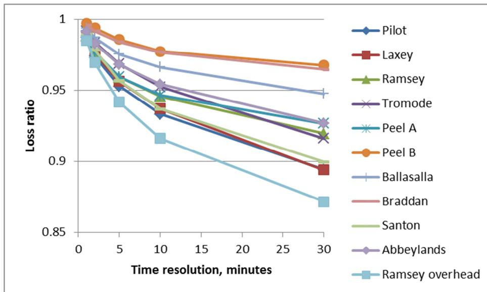
Figure 160 Impact of measurement time resolution for LV feeders
