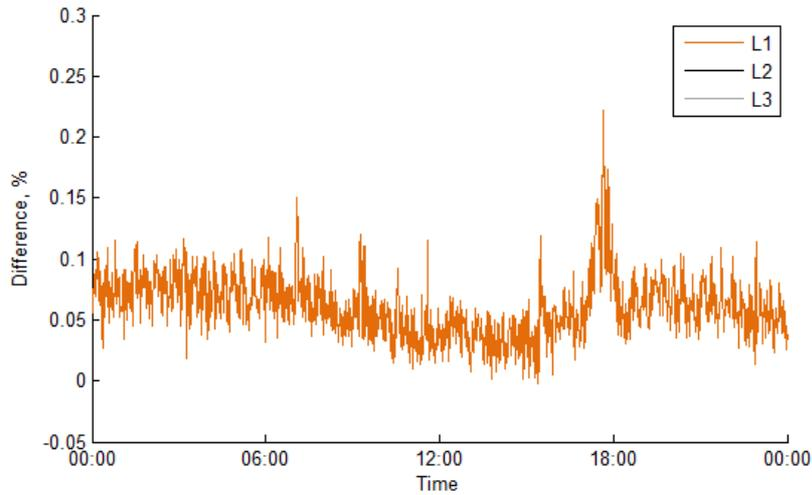
Figure 13 Difference between calculated and measured substation voltages for a load on phases L1
