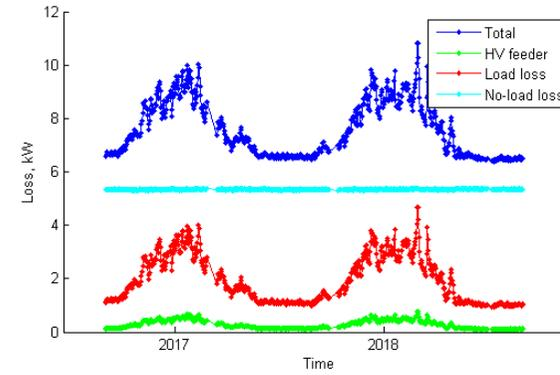
Figure 74 Long term mean daily ( $I^2R$ ) loss (Wavendon Gate Local HV feeder)
