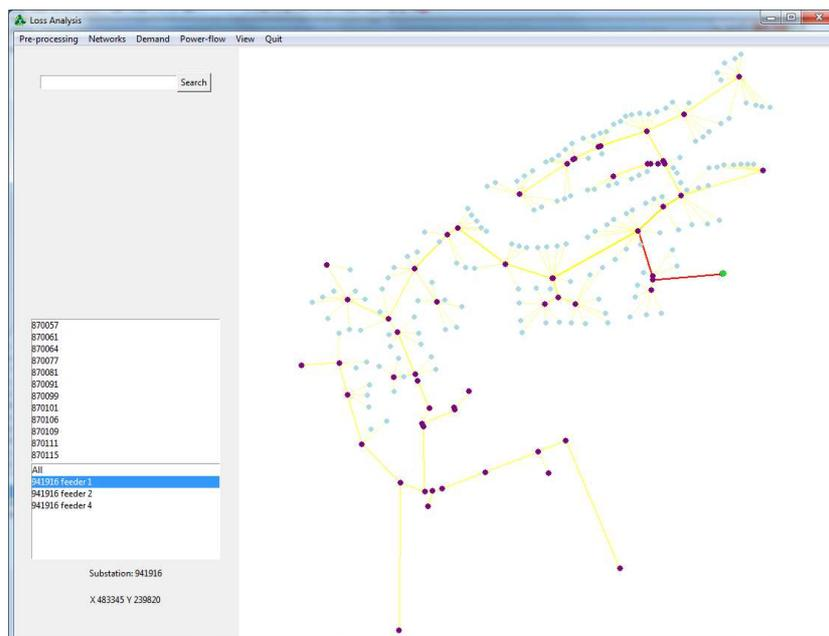
Figure 24 LV loss assessment software Python interface showing phase allocations for substation 941916 feeder 1 (L1 to L3 use standard colouring, three-phase shown in red)
