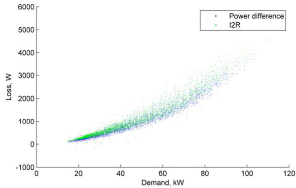
Figure 123 Jan 2018 Loss, kW vs demand, 10 min. av. (Tromode Dom. LV feeder)
