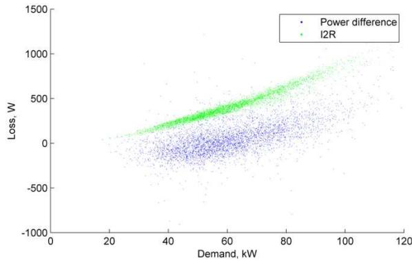
Figure 127 Jan 2018 2017 Loss, kW vs demand, 10 min. av. (Peel A I&C LV feeder)
