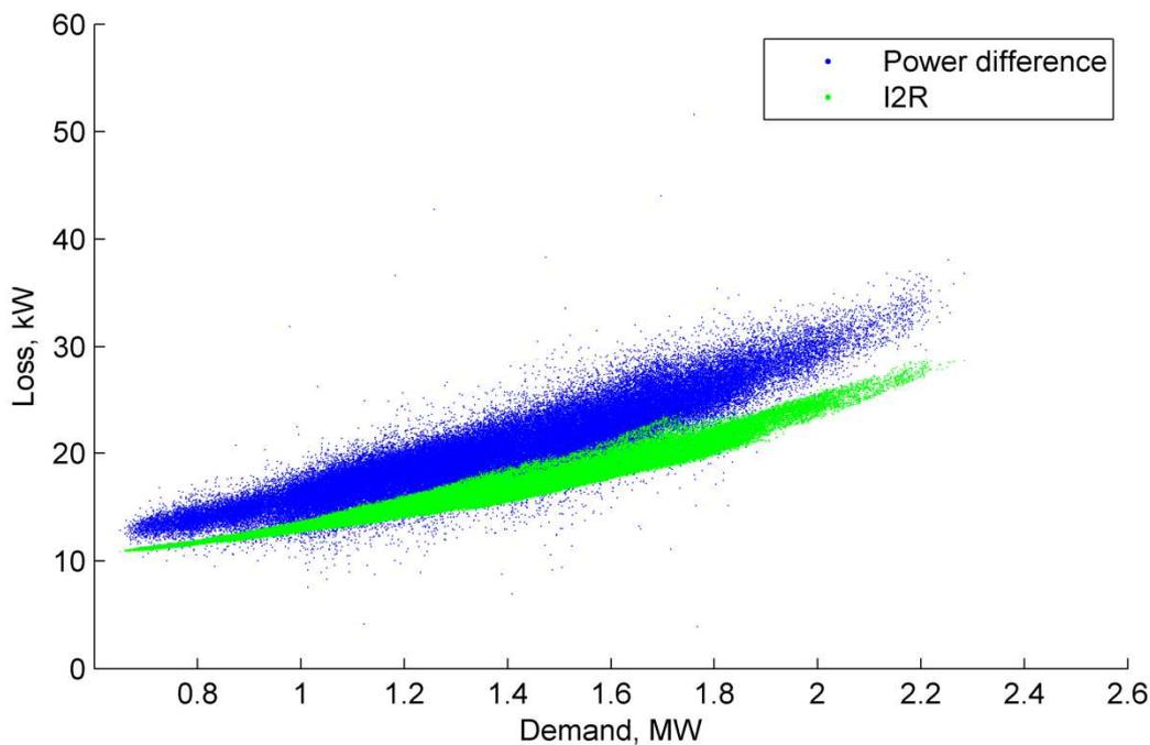
Figure 16 Loss vs demand for 1-minute samples on Woodlands HV feeder
