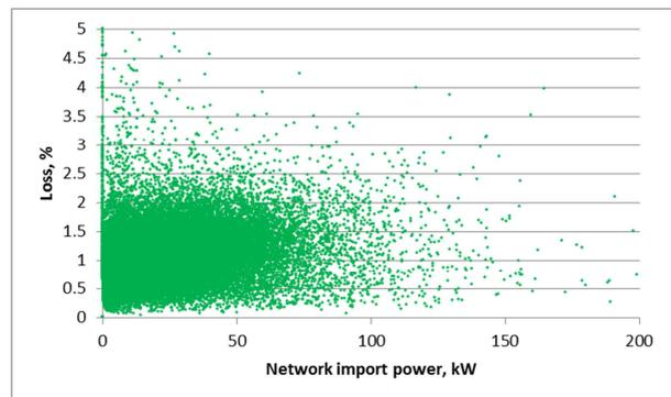
Figure 47 Filtered LV feeder loss assessment results, loss percentage vs. demand
