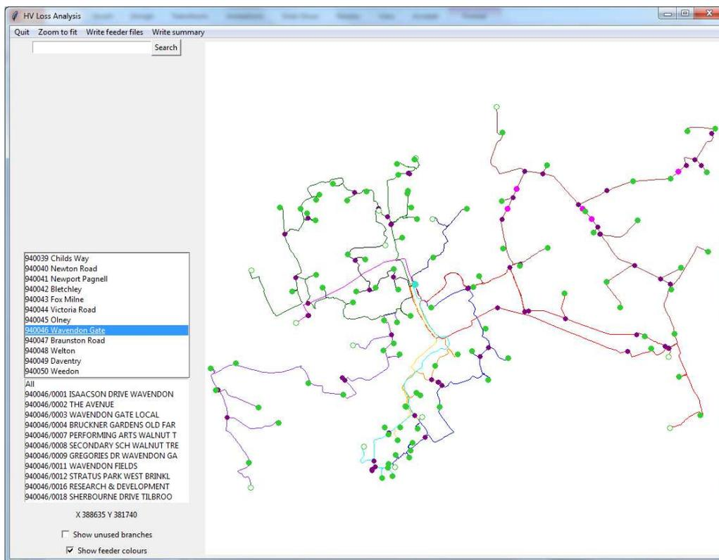
Figure 20 HV loss assessment software Python interface showing feeders for a single primary substation
