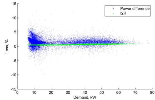
Figure 136 Jan 2018 Loss, % vs demand, 1 min. av. (Ballasalla I&C LV feeder)
