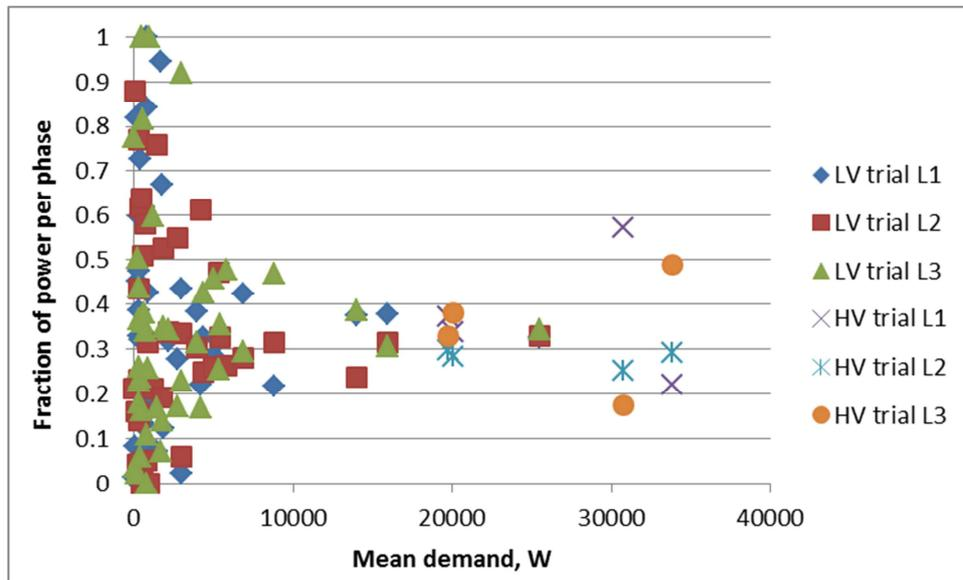
Figure 163 Mean unbalance of three-phase meters
