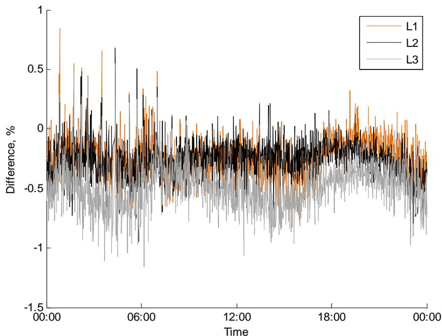
Figure 10 Difference between calculated and measured substation current, 28<sup>th</sup> March 2016
