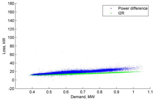
Figure 103 Jul/Aug 2017 Loss, kW vs demand (Silver End HV feeder)
