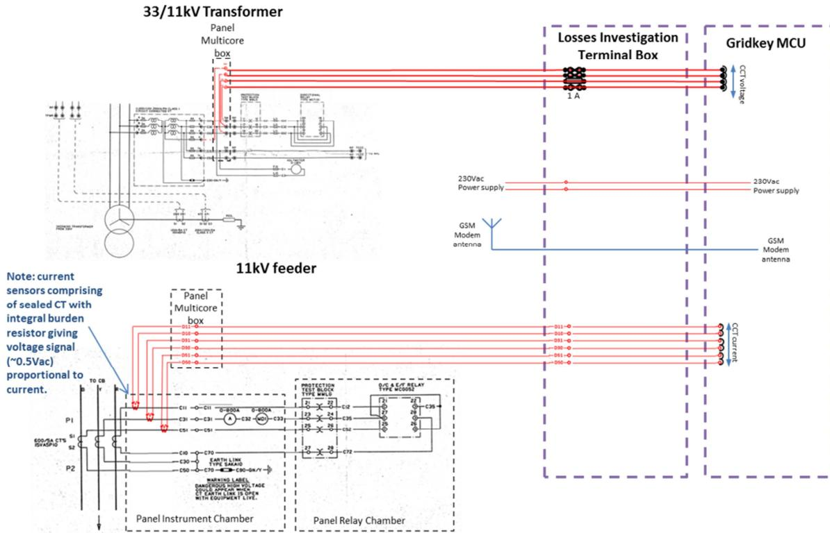
Figure 2 Schematic of monitoring at 11kV primary feeder
