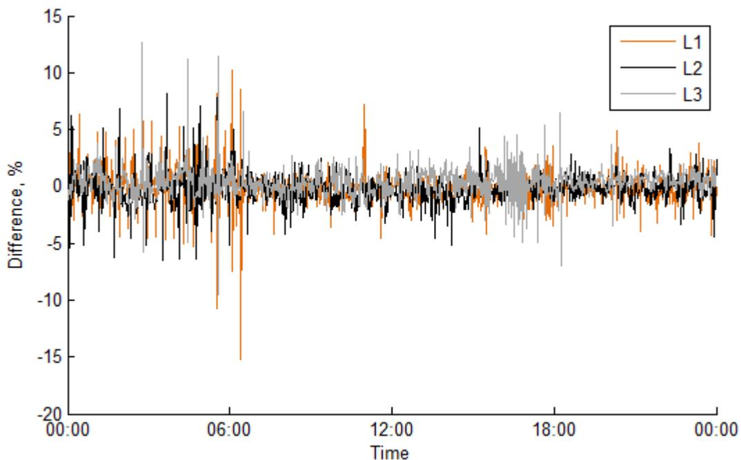
Figure 12 Difference between calculated and measured substation current phases L1, L2 and L3
