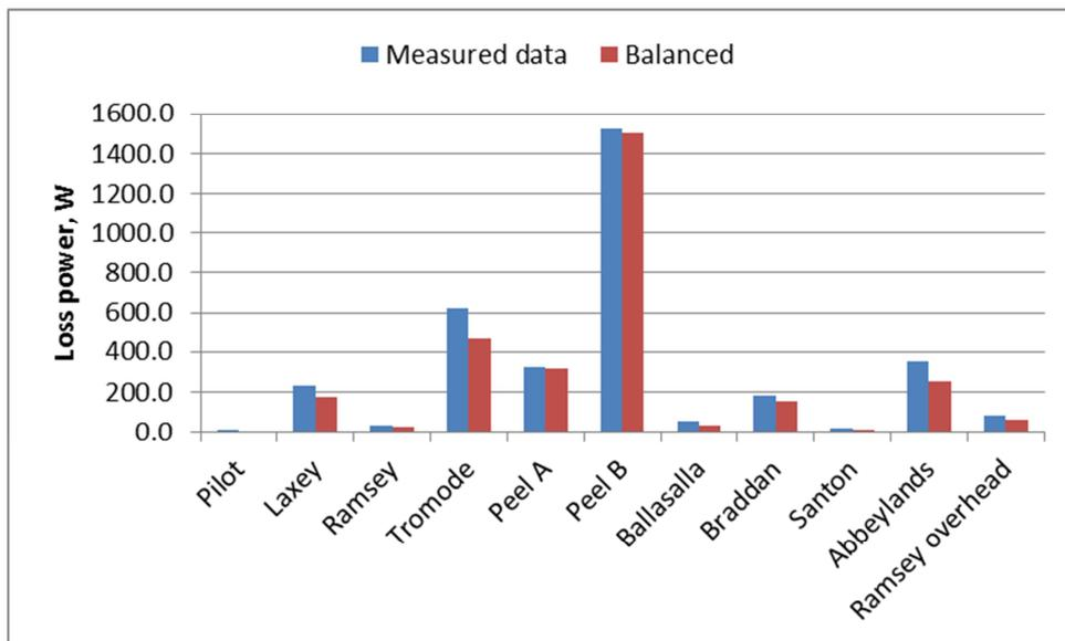
Figure 36 LV feeder mains losses calculated from measurement data and with balanced demand data
