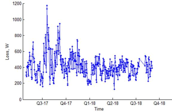
Figure 126 Long term mean daily ( $I^2R$ ) loss (Peel A I&C LV feeder)
