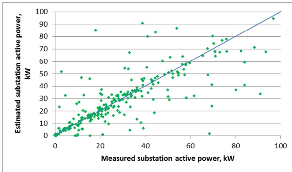
Figure 172 Mean demand from loss assessment and measurement for HV trials feeders
