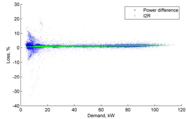
Figure 140 Jan 2018 Loss, % vs demand, 1 min. av. (Braddan I&C LV feeder)
