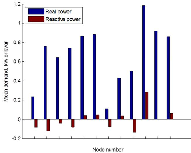
**Figure 15 Mean demand for meter connections on Pilot LV feeder**
