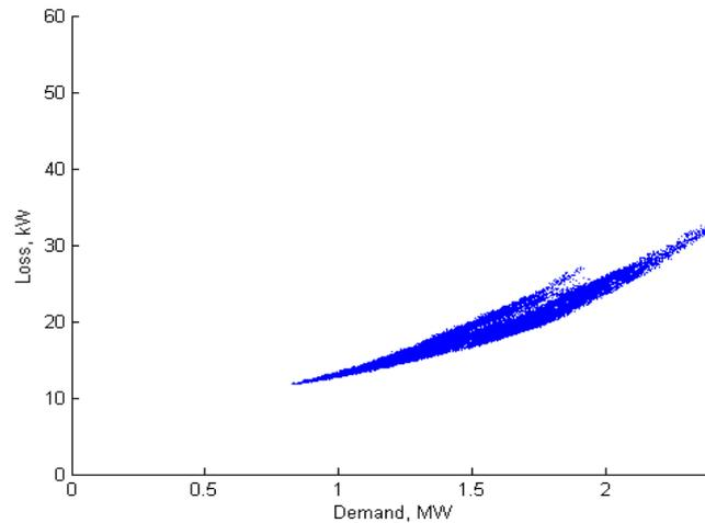
Figure 48 Sample monitored HV feeder loss vs load plot, 1 minute loss/load points using I<sup>2</sup>R calculation method
