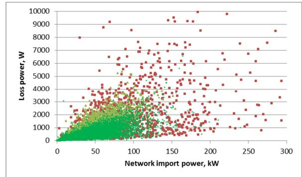
Figure 45 LV feeder loss assessment results, with potentially unreliable results highlighted
