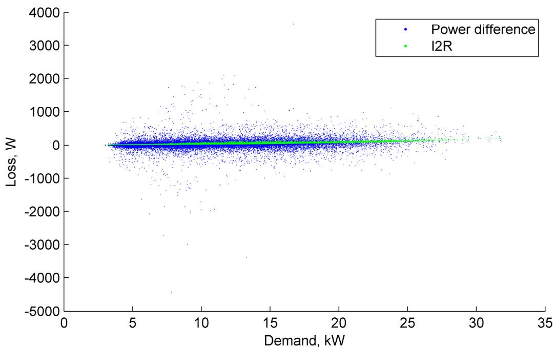
Figure 62 Loss vs demand per 1-minute sample for LV Pilot feeder
