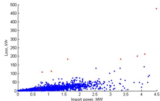
Figure 43 HV feeder loss assessment results, with potentially unreliable results highlighted
