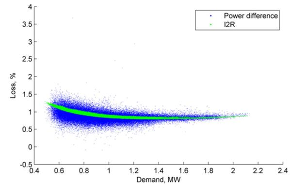
Figure 76 Mar 2018 Loss, % vs demand (Wavendon Gate Local HV feeder)
