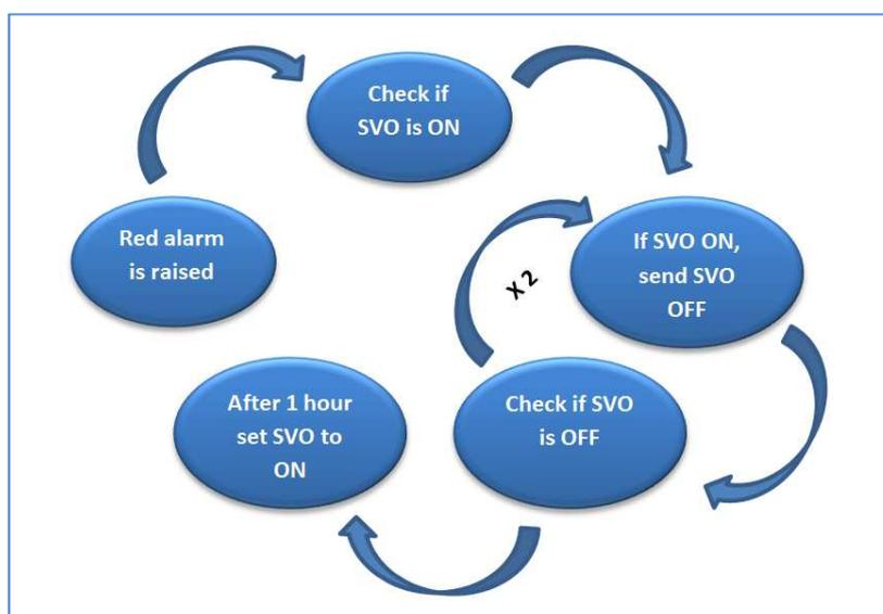
Figure 2-1 Updated Automatic Restoration Procedure
