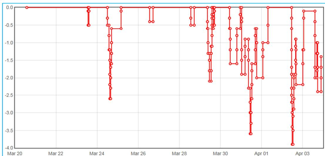
Figure 2-3: Reactive power (MVar) absorption by the FPL on Barnstaple side over a two week period
