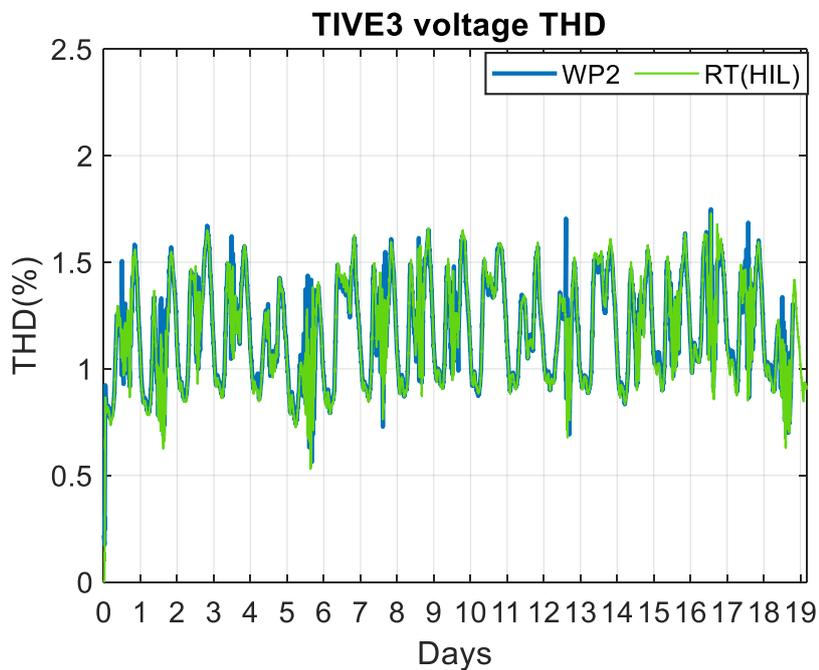
Figure 43: THD at TIVE3 busbar for WP2, and for HIL (with compensation).
