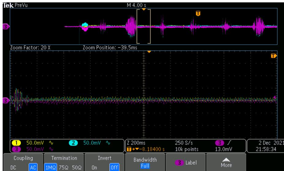
Figure 38: Inverter current from the oscilloscope when AF operation is not active – the zoomed in window in the second plot shows small current during the night.
