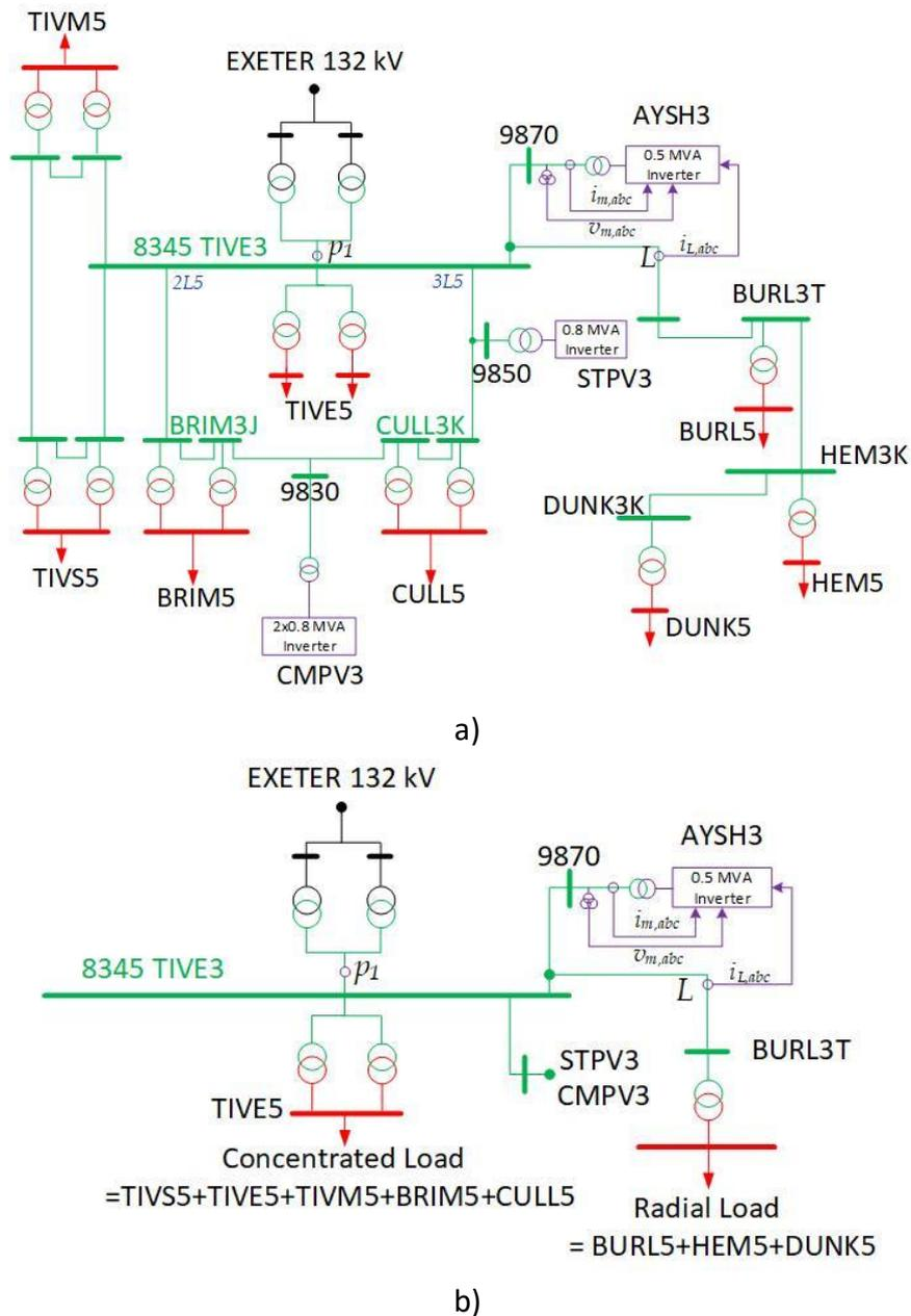
Figure 29: Comparison between a) the complete network model and b) the simplified network model network for HIL analysis.
