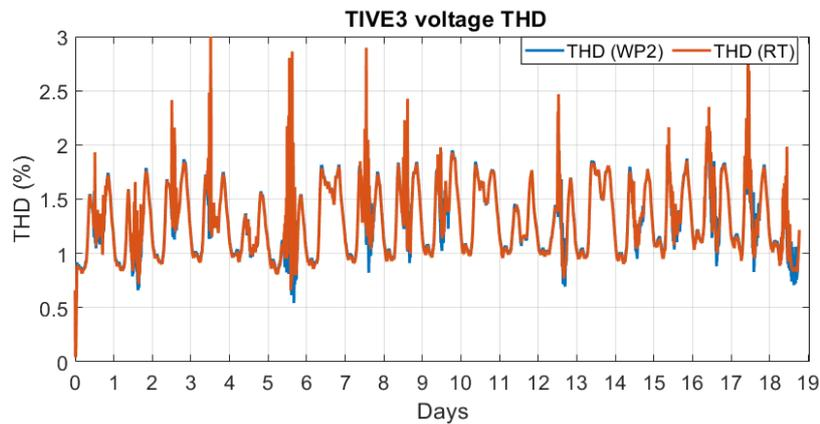
Figure 27: Voltage THD at TIVE3 for the entire observation period after correction of the PQ data.
