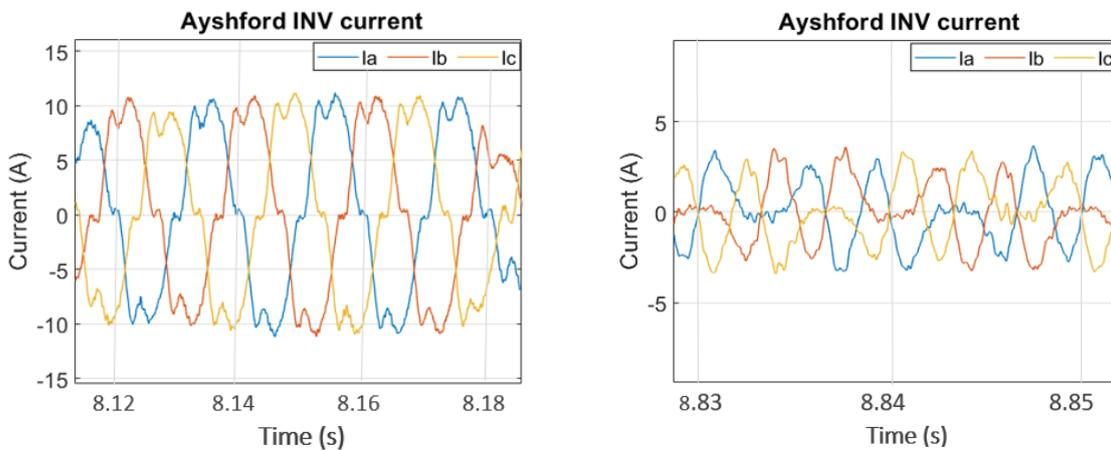
Figure 45: Ayshford inverter current with compensation (SIL).
