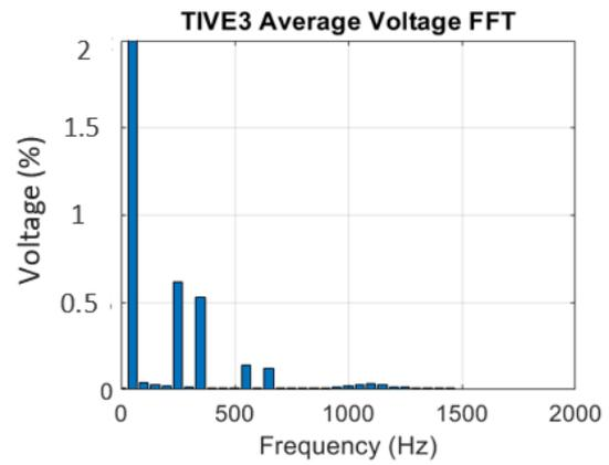
Figure 47: Voltage FFT with and without harmonic mitigation (SIL).
