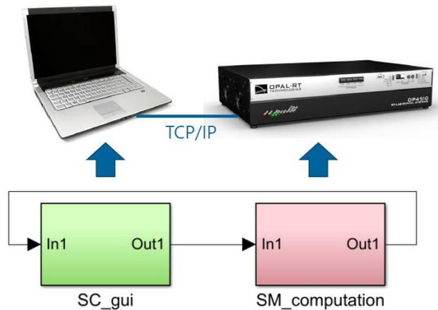
Figure 3: Overview of the model configuration for real-time execution (stock image from OPAL-RT).
