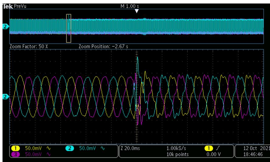
Figure 33: Current waveform at the inverter terminals (recorded from the oscilloscope).
