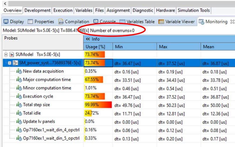
Figure 4: RT-LAB interface used to communicate with the inverter.
