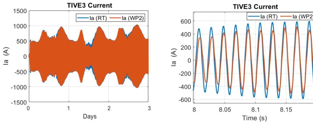
Figure 23: Fundamental current at TIVE3 showing a significant error due to time shift. Original and zoomed in version.
