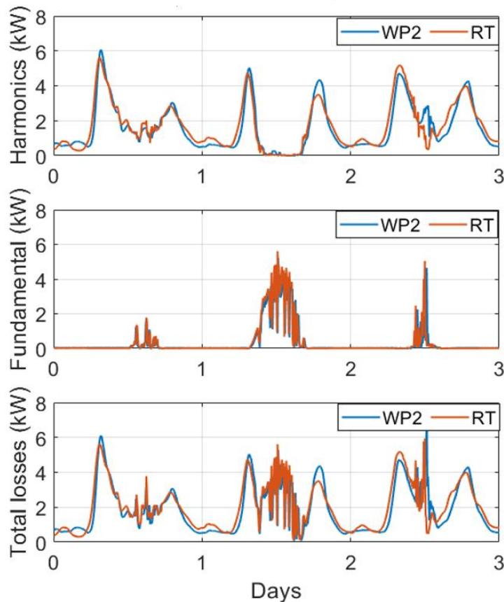
Figure 44: Comparison of transformer losses in a) WP2 and b) HIL. Average loss value: 2.22 kW for HIL and 2.21 kW for WP2.
