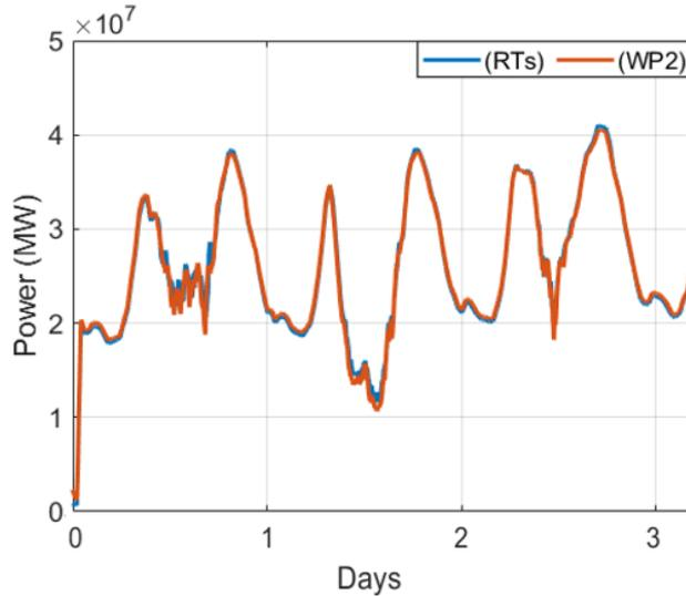
Figure 30: Power comparison at TIVE3 between WP2 and the simplified OPAL-RT model.
