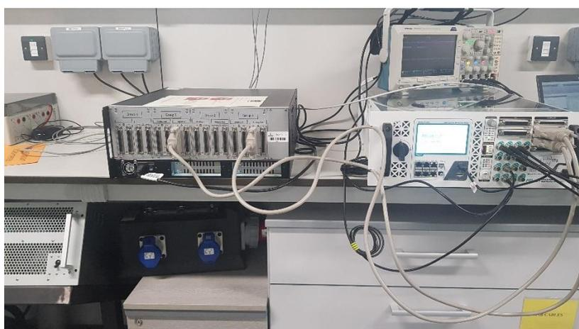
Figure 2: The DB37 cables are used to connect the back ports of the OPAL-RT and the inverter.
