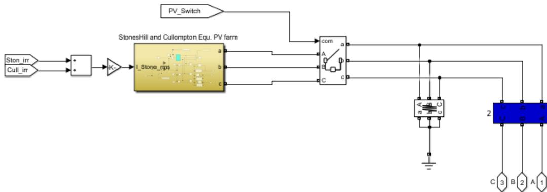
Figure 37: Additional shunt resistance added in parallel to the dynamic PV farm model.
