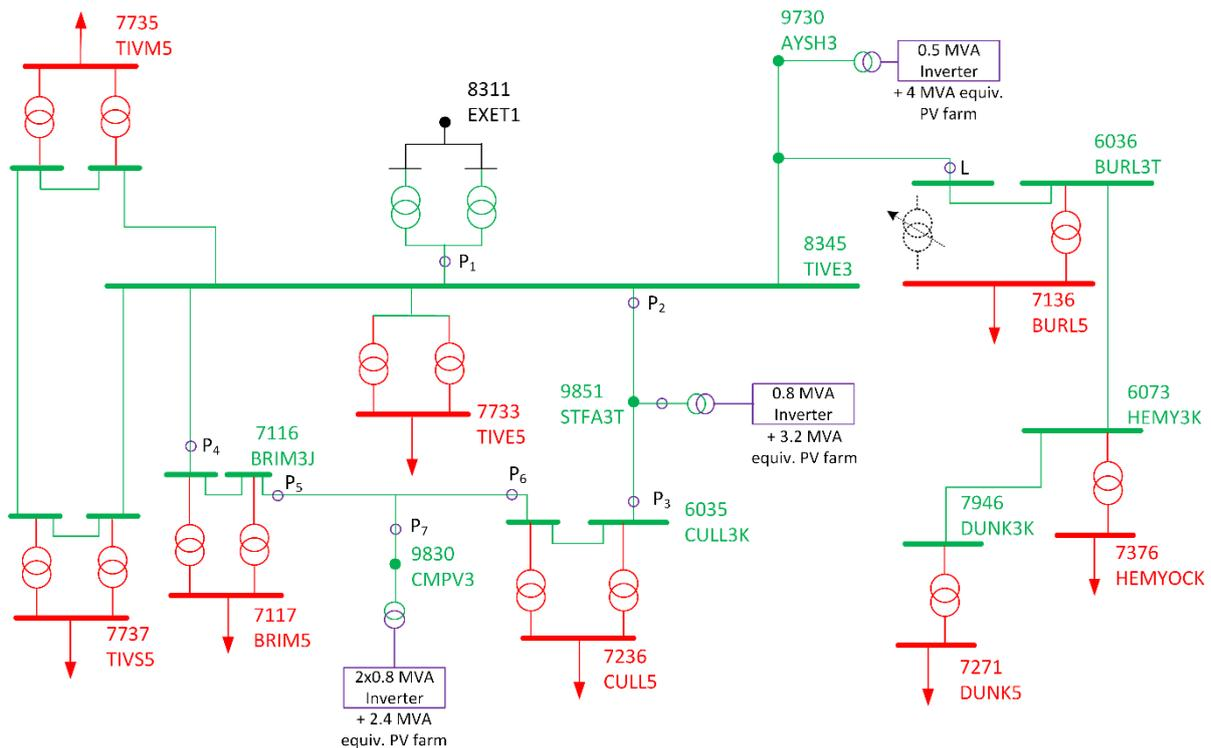
Figure 19: Overview of the Tiverton network, including the PV farms and the measurement points (P<sub>1</sub>-P<sub>7</sub> and L).
