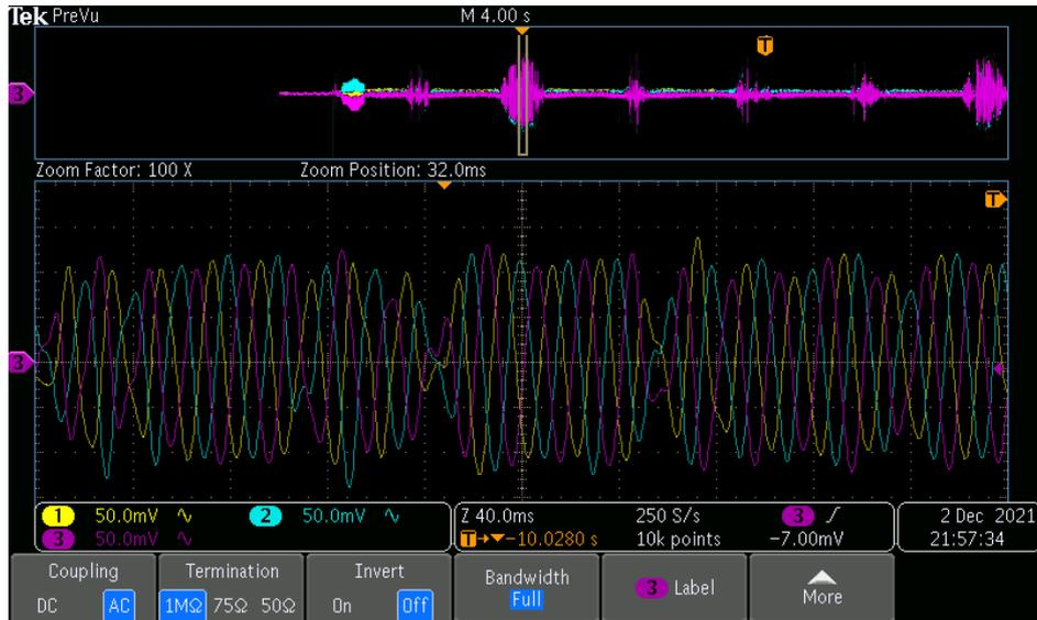
Figure 39: Inverter current from the oscilloscope when AF operation is not active – the zoomed in window in the second plot shows large fundamental current during the night.
