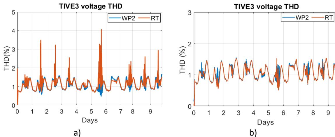
Figure 36: Comparison of voltage THD a) before and b) after adding the shunt resistance in parallel to the equivalent farm models.
