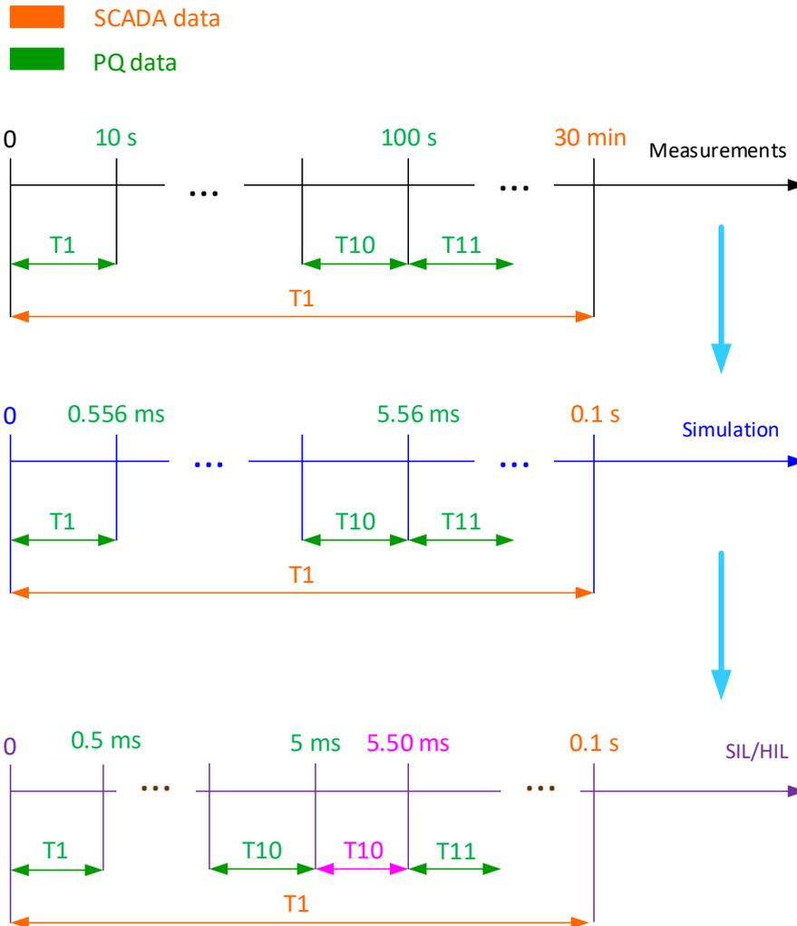
Figure 21: Mapping of SCADA data and PQ data in different domains.
