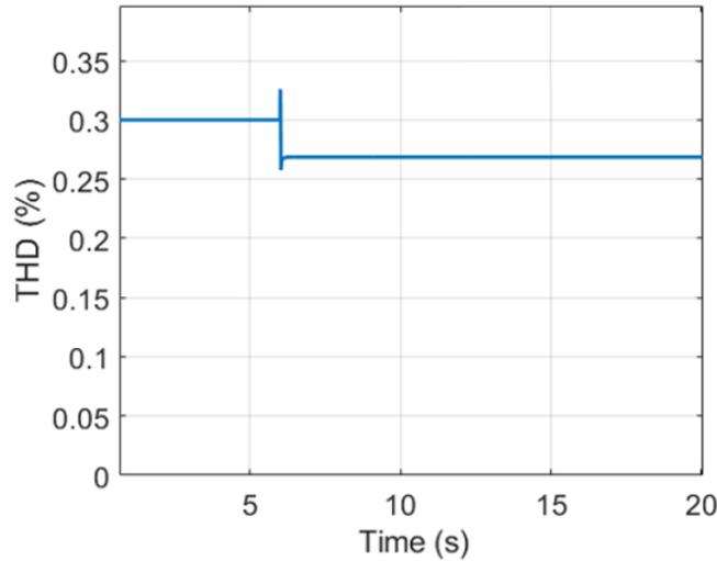
Figure 34: Voltage THD at TIVE3, when harmonic mitigation from the PELab is activated at t = 6 s.
