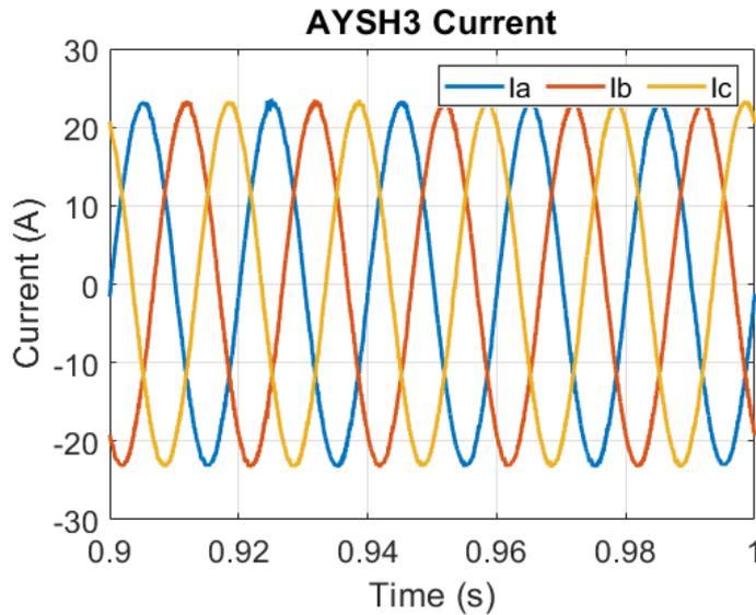
Figure 15: Inverter current at Ayshford 33 kV (workspace).
