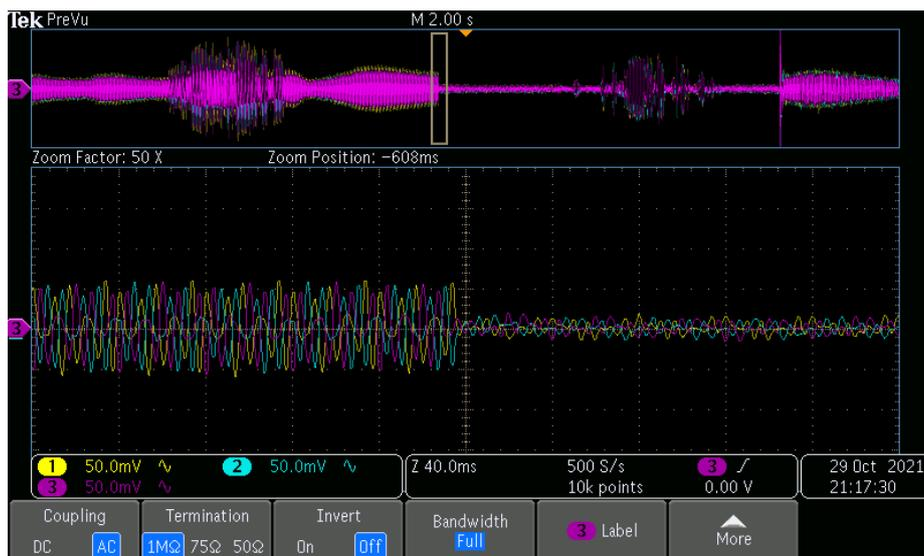
Figure 40: Inverter current, showing the transition between AF operation, and normal operation.
