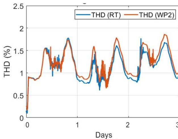
Figure 24: Voltage THD at TIVE3 – significant error due to time shift.
