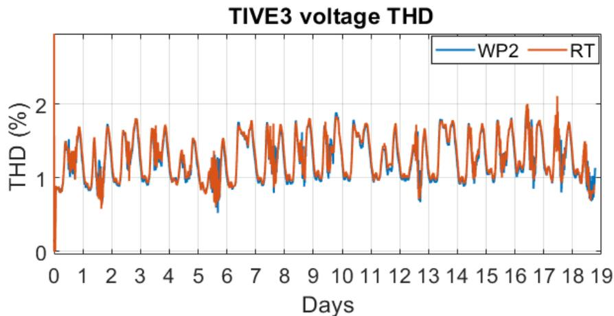
Figure 31: Voltage THD comparison between WP2 results and real-time with concentrated load without compensation.
