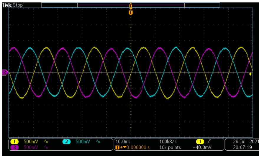
Figure 16: Inverter current at Ayshford 33 kV.
