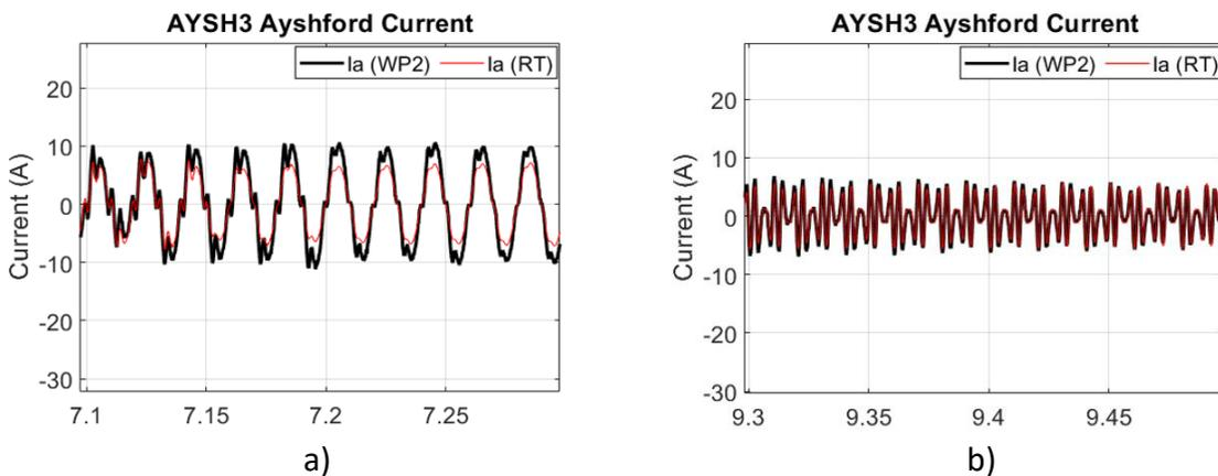
Figure 42: Detailed comparison of phase a current during the day (a) and the night (b).
