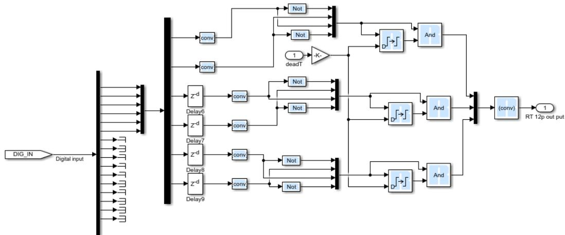
Figure 11: Duplication of the digital signals from the inverter to generate 12 switching pulses.
