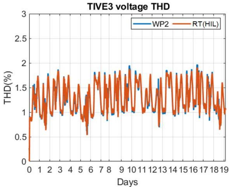
Figure 32: Final THD results in HIL (without compensation).
