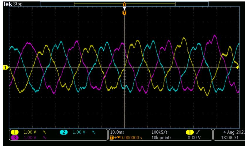
Figure 17: Inverter current from the oscilloscope when all harmonics are included.
