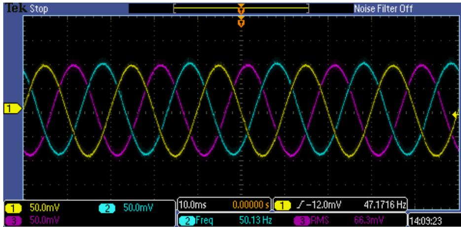
Figure 14: Voltage at Ayshford 33 kV (Oscilloscope 1).
