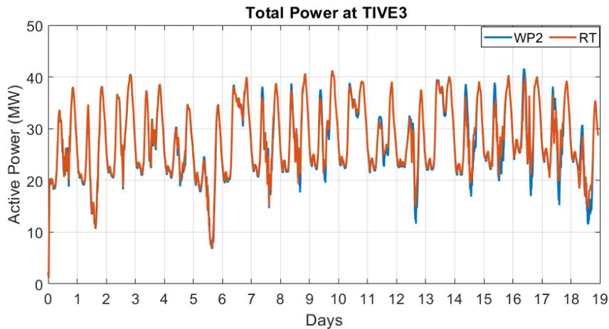
Figure 26: Total power at TIVE3 for entire observation period after correction of the PQ data.
