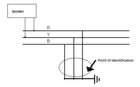
**Test 2** - With an **Earth** re-applied to the leg to be identified, remove the **Earths** from the alternative leg(s) and ensure a signal is detected in the leg to be identified.
