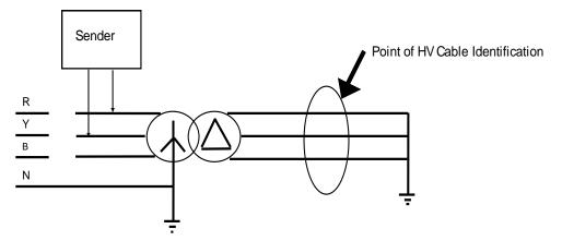
If it is not possible to make direct connection to the cable a signal may be injected through a distribution transformer.
