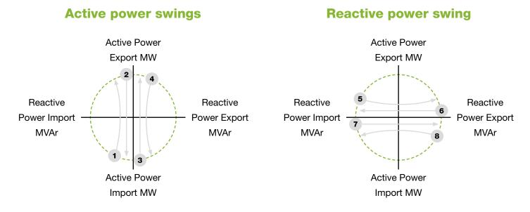
These diagrams assume the other vector (MW or MVAr) does not change during the power swing.
